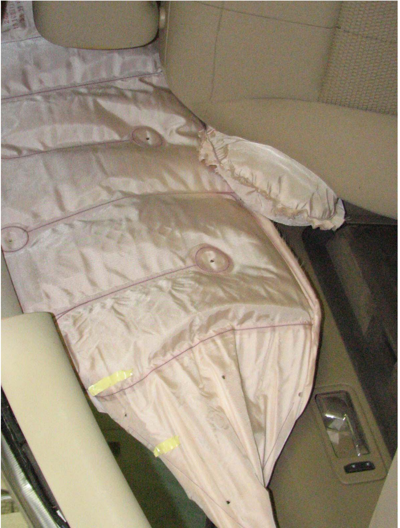
Figure A-10: Post-Test Airbags, Close-up View
