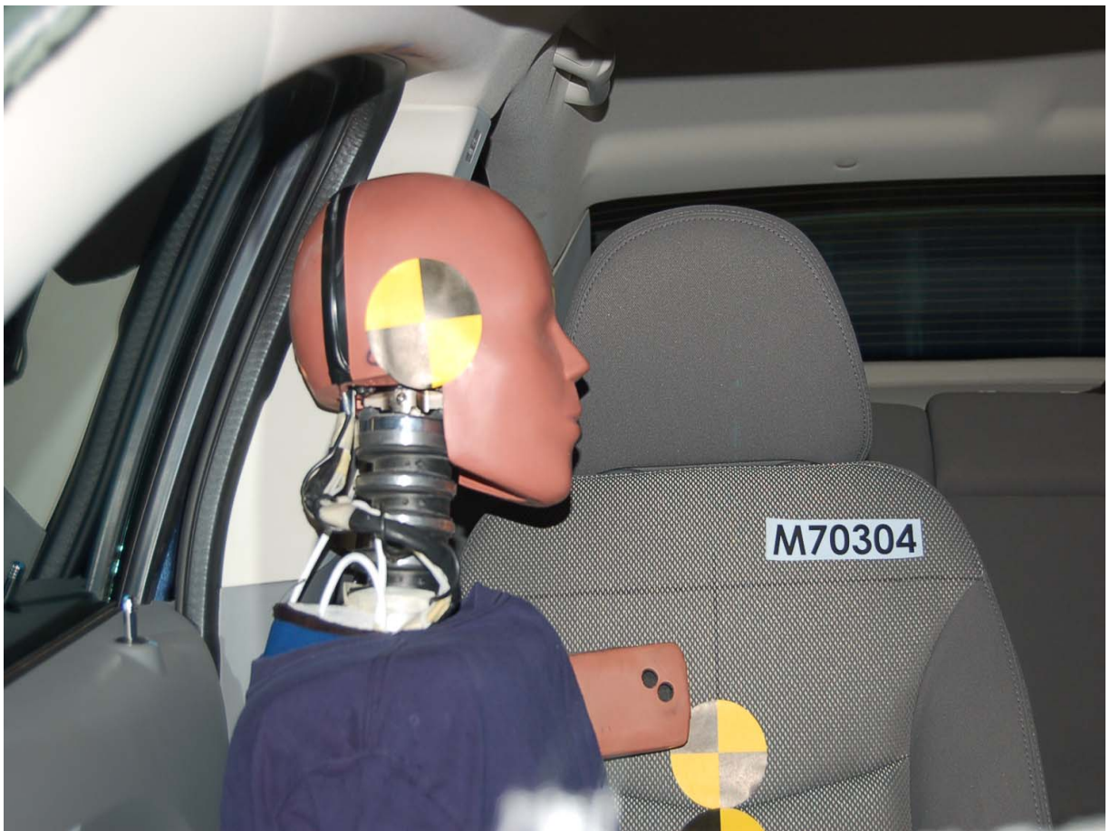
Pre-Test SID-IIs Dummy Right Side Head View
