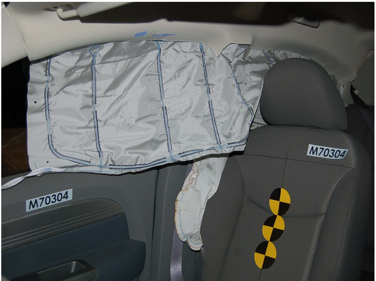
Post-Test Curtain and Torso Airbag View
