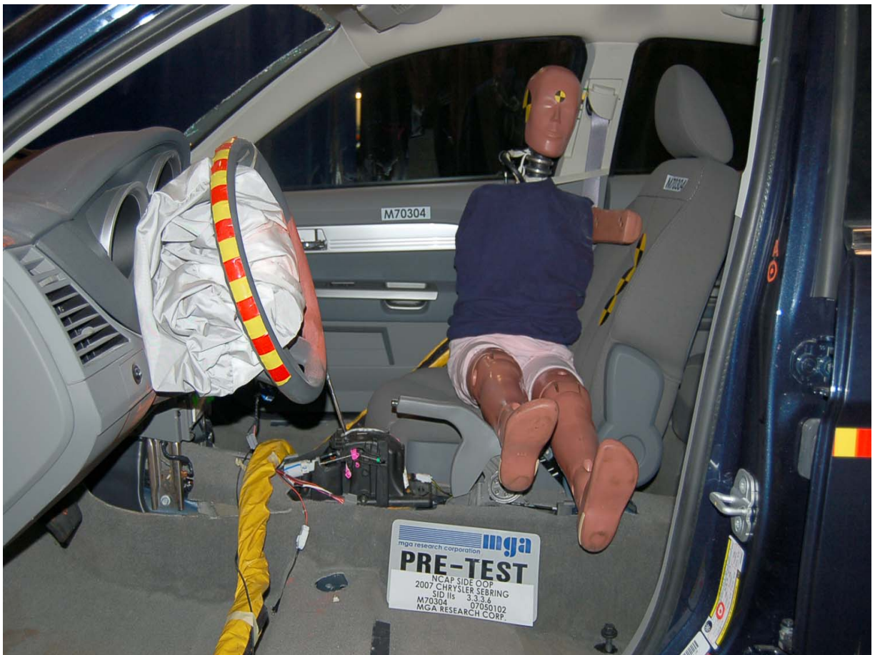
Pre-Test SID-IIs Dummy Frontal View
