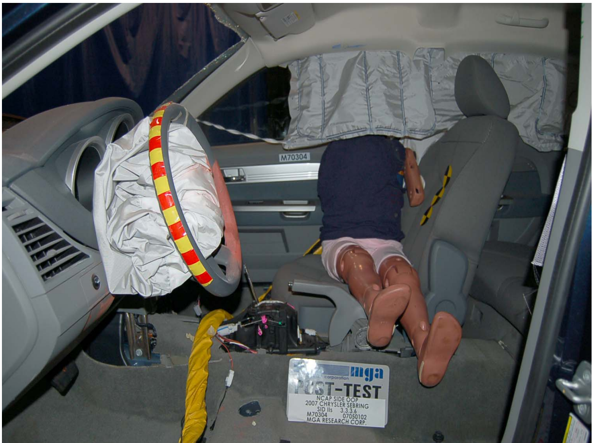
Post-Test SID-IIs Dummy Frontal View
