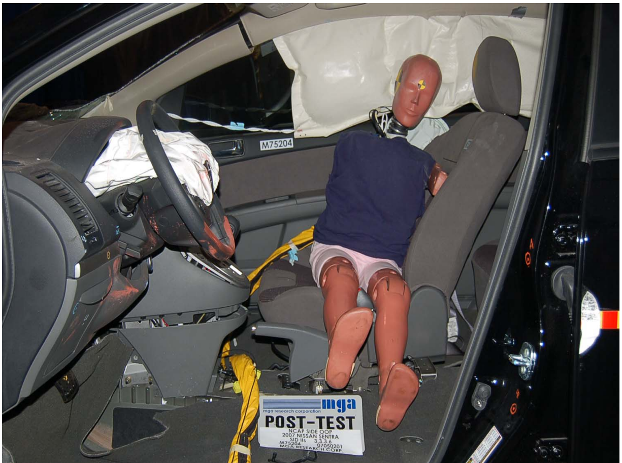
Post-Test SID-IIs Dummy Frontal View
