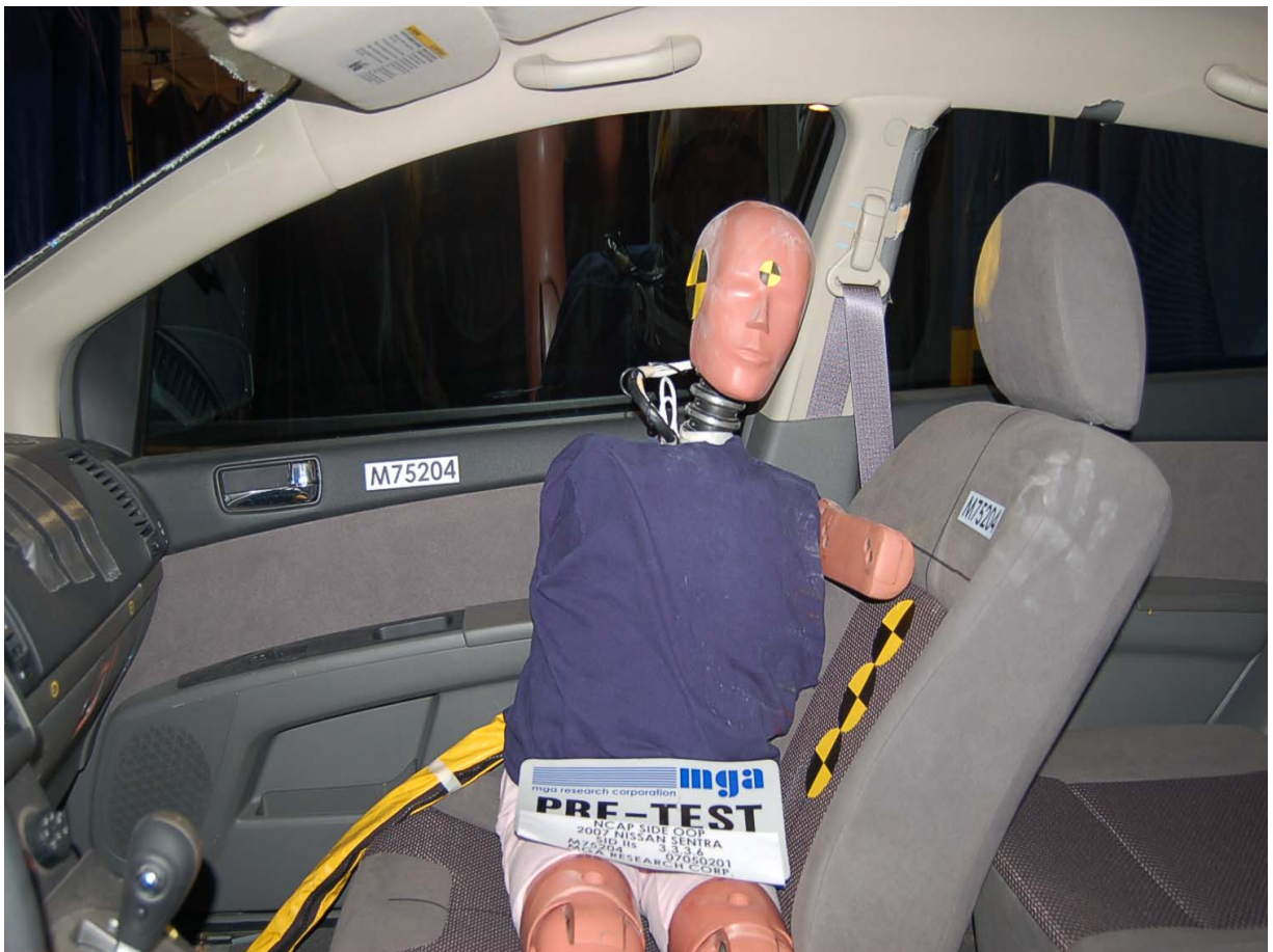
Pre-Test SID-IIs Dummy Frontal Closeup View
