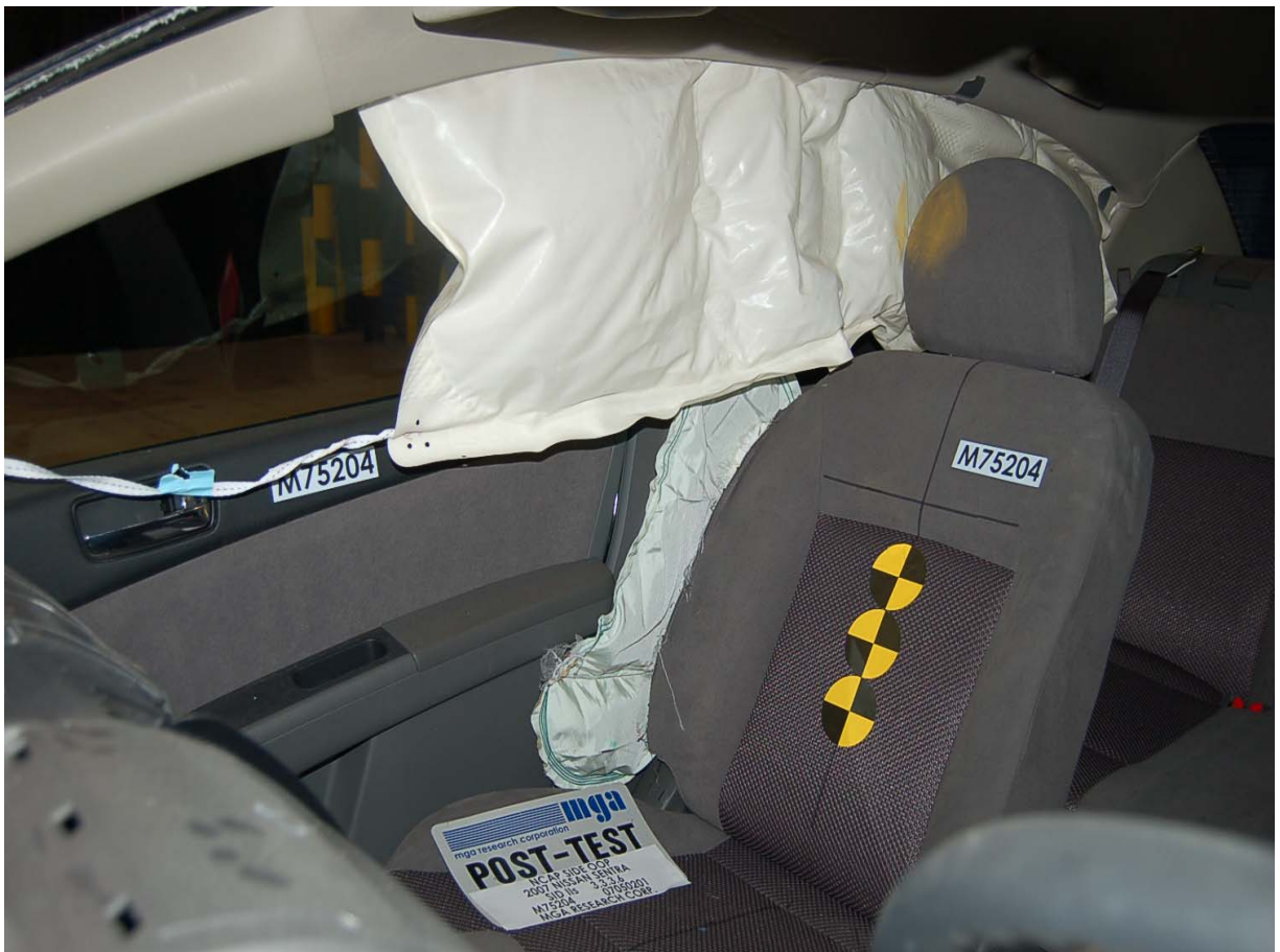
Post-Test Curtain and Torso Airbag View
