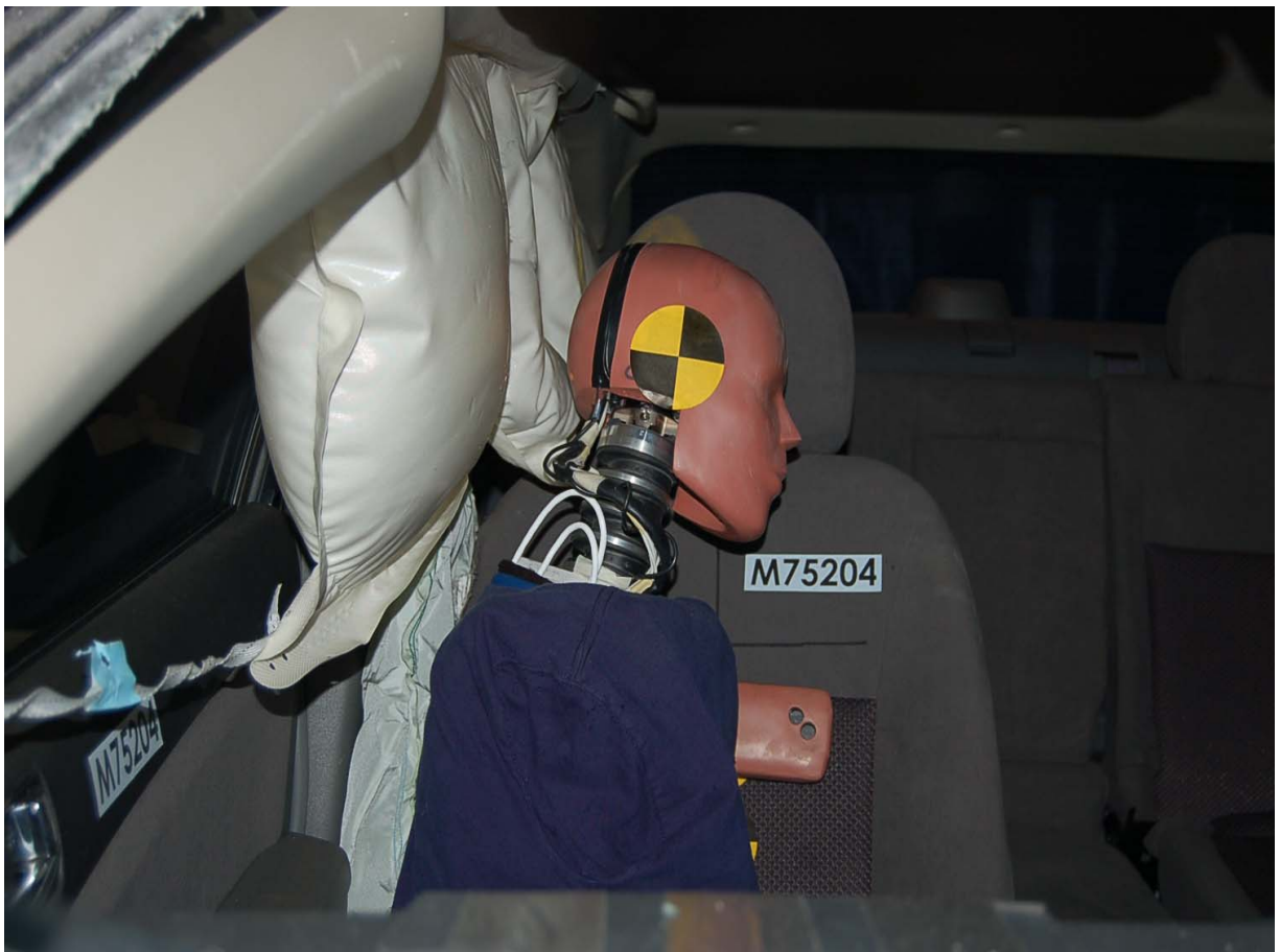
Post-Test SID-III Dummy Right Side Head View
