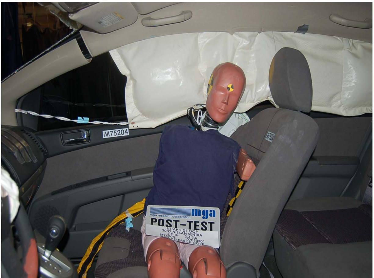
Post-Test SID-IIs Dummy Frontal Closeup View
