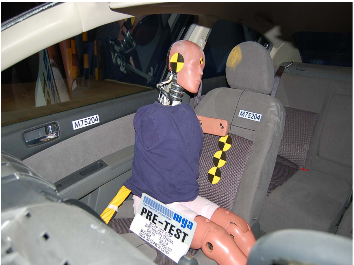
Pre-Test SID-11s Dummy Right 3/4 Front View
