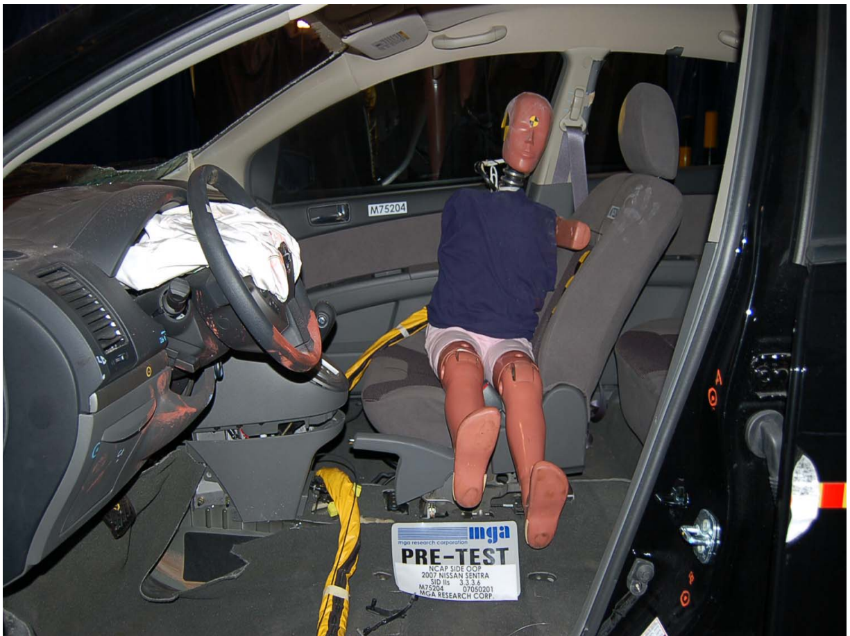
Pre-Test SID-IIs Dummy Frontal View
