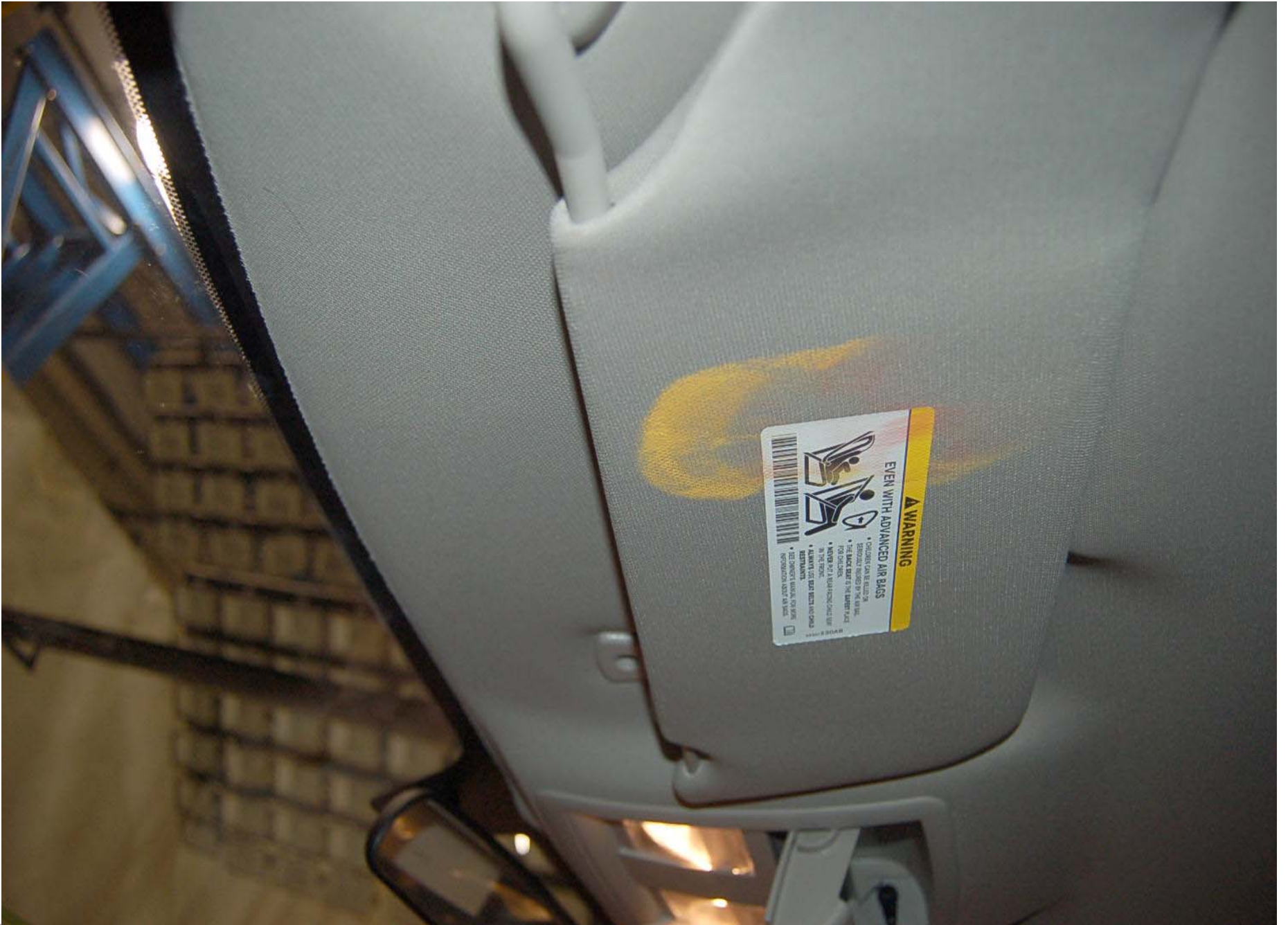
Post-Test Driver Dummy Head Contact (visor)
