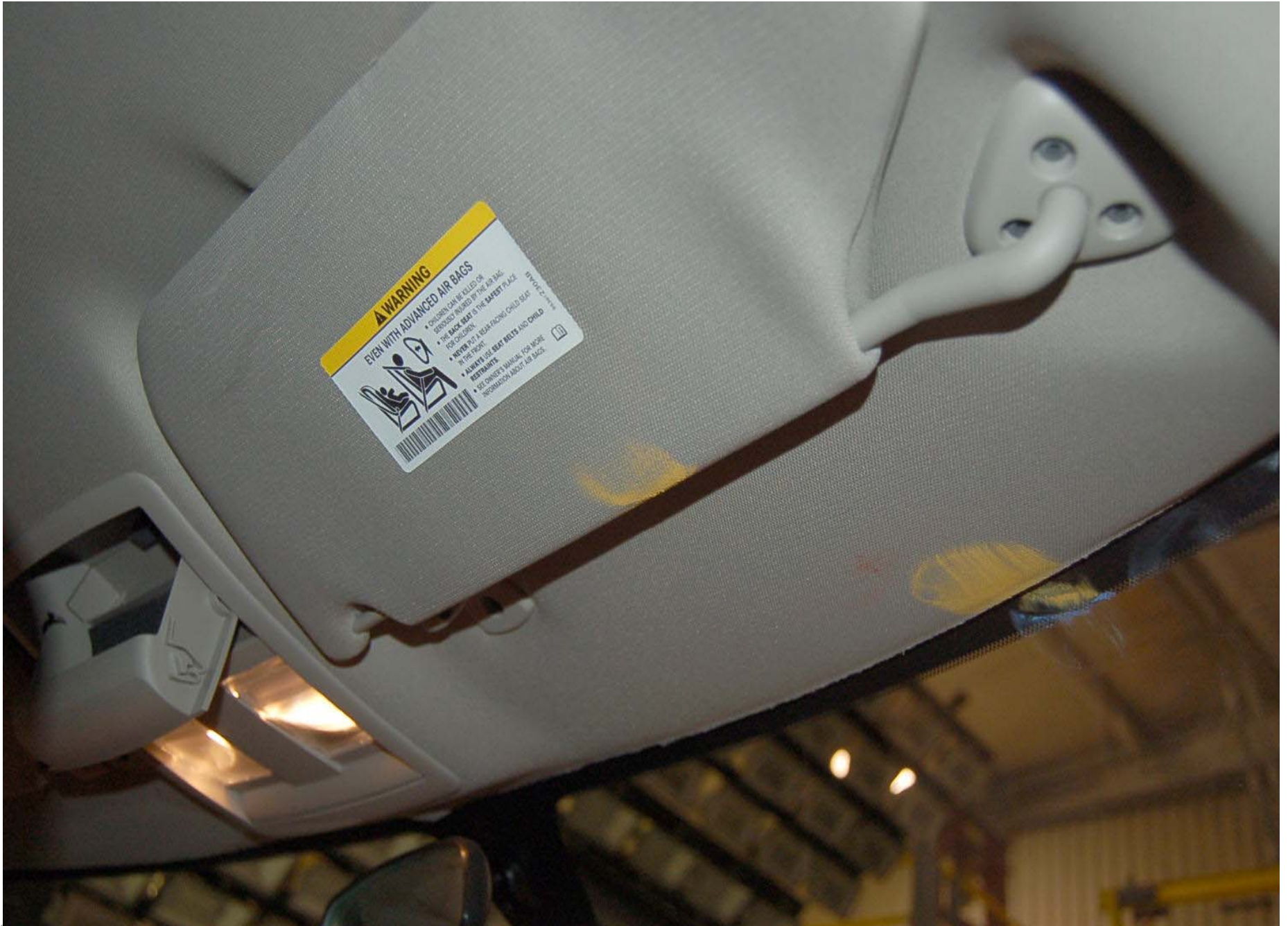
Post-Test Passenger Dummy Head Contact View (visor, header & Windshield)
