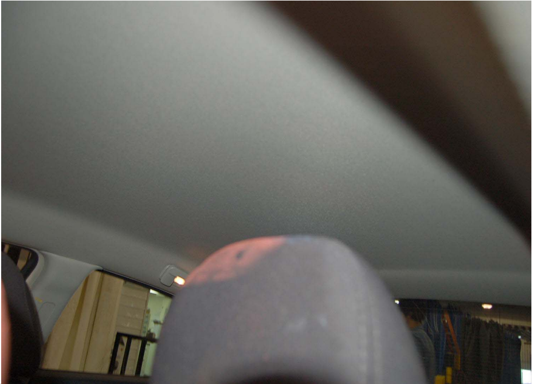
Post-Test Driver Dummy Head Contact (head rest)
