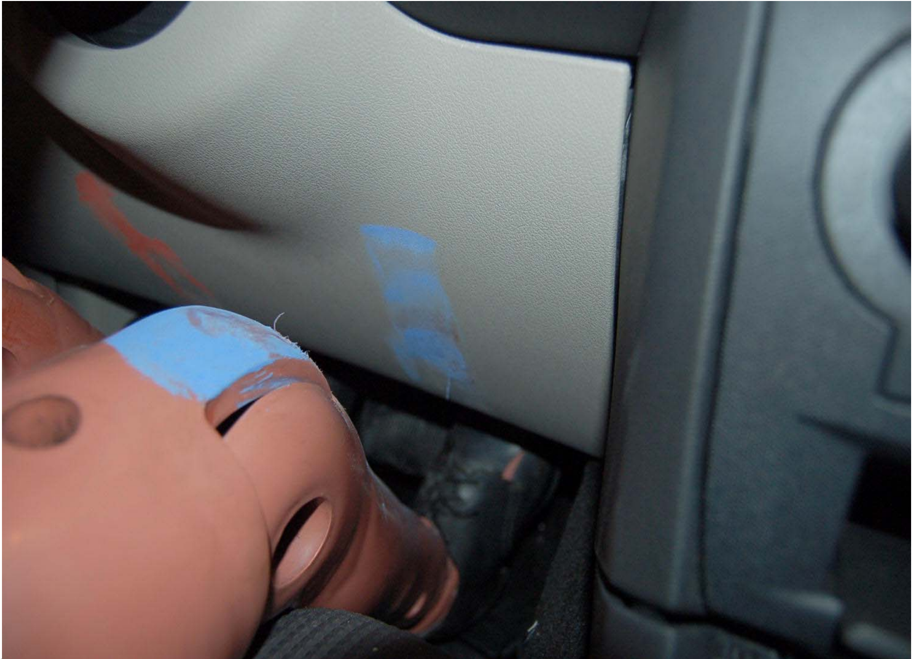
Post-Test Driver Dummy Knee Contact (right side)
