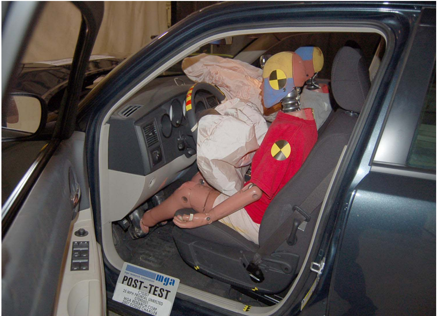
Post-Test Driver Dummy Position Left Side View (Door Open)
