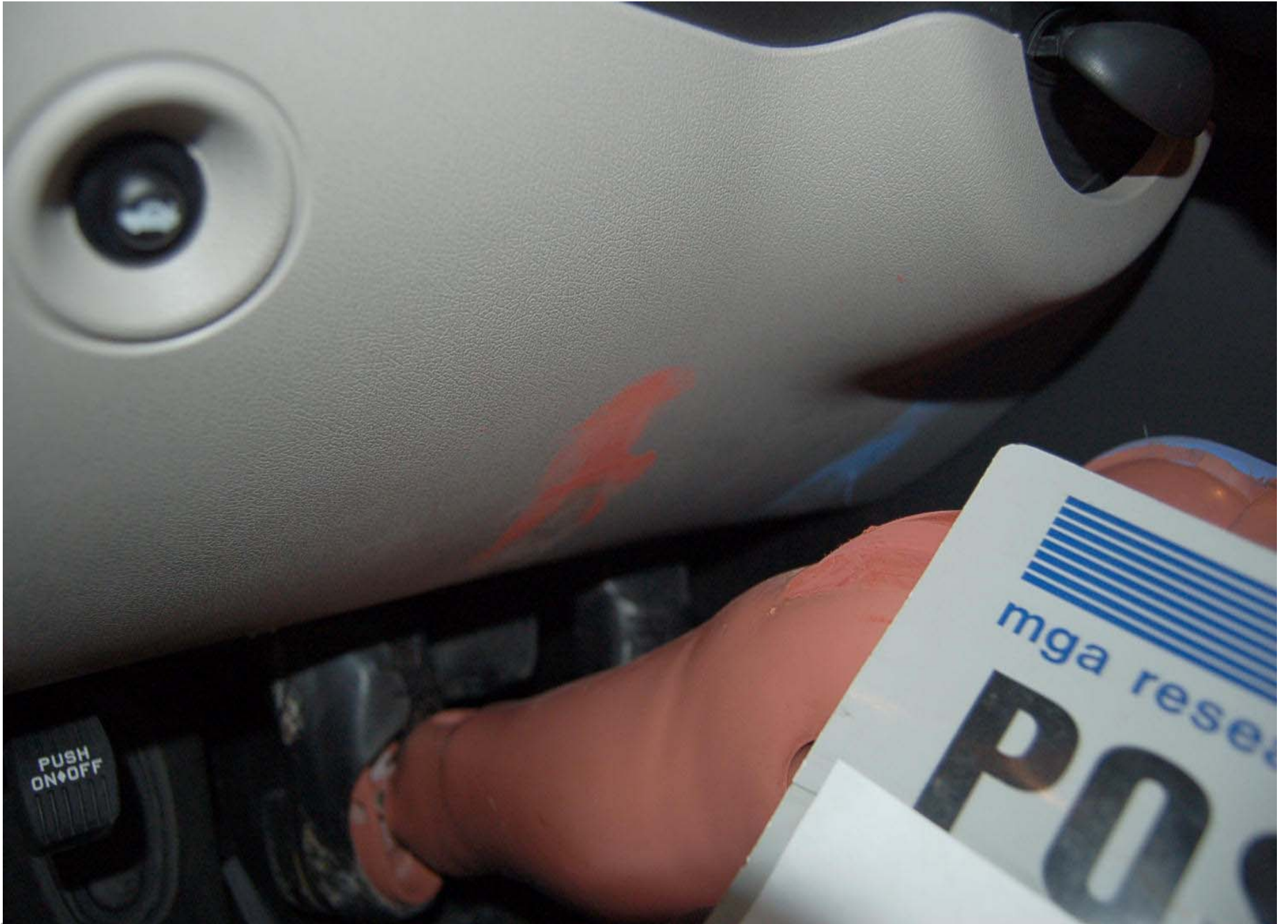
Post-Test Driver Dummy Knee Contact (left side)
