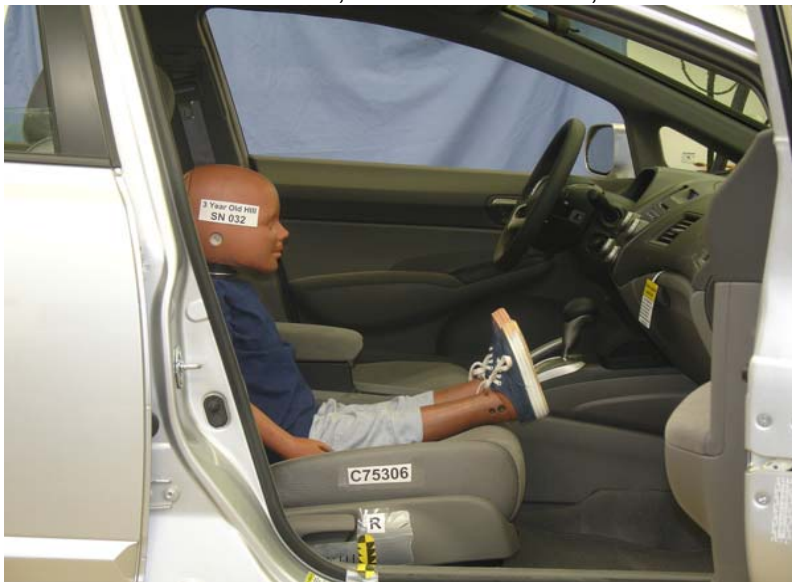
3-Year-Old Unbelted, Rearward Seat Track, Position 1
