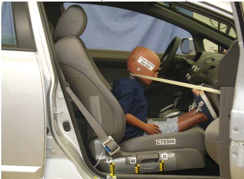
3-Year-Old Unbelted, Forward Seat Track, Position 3
