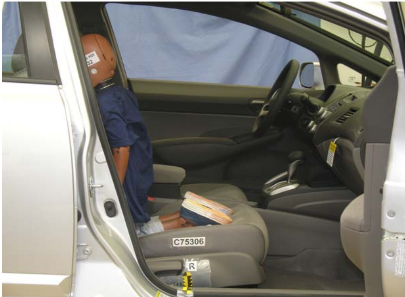
3-Year-Old Unbelted, Rearward Seat Track, Position 7
