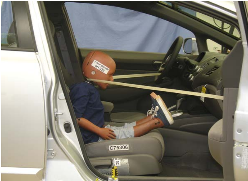
3-Year-Old Unbelted, Rearward Seat Track, Position 3
