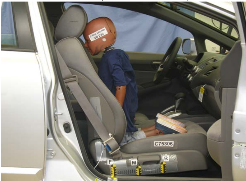
3-Year-Old Unbelted, Forward Seat Track, Position 7
