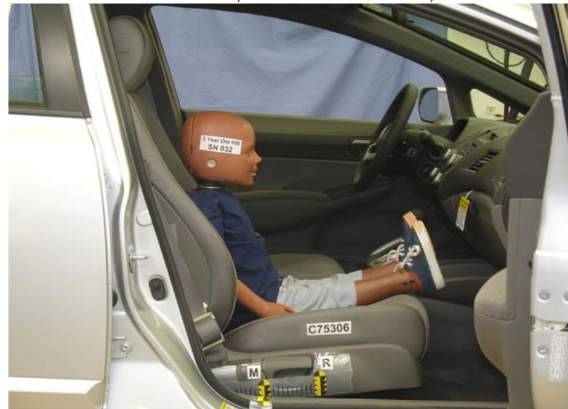
3-Year-Old Unbelted, Middle Seat Track, Position 1
