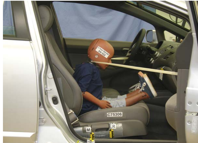
3-Year-Old Unbelted, Middle Seat Track, Position 3
