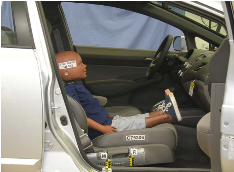
3-Year-Old Unbelted, Middle Seat Track, Position 2
