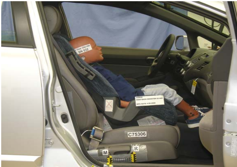
3-Year-Old Cosco High Back Booster Cinched With Harness, Middle Seat Track
