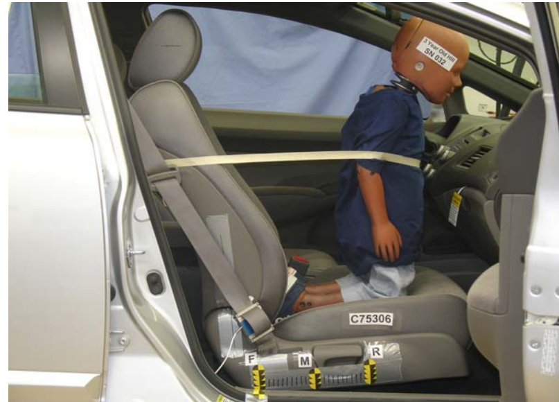
3-Year-Old Unbelted, Forward Seat Track, Position 6
