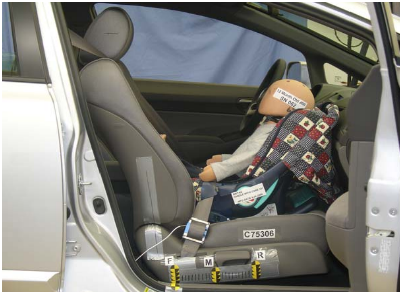
Britax Handle With Care 191 Belted, Forward Seat Track
