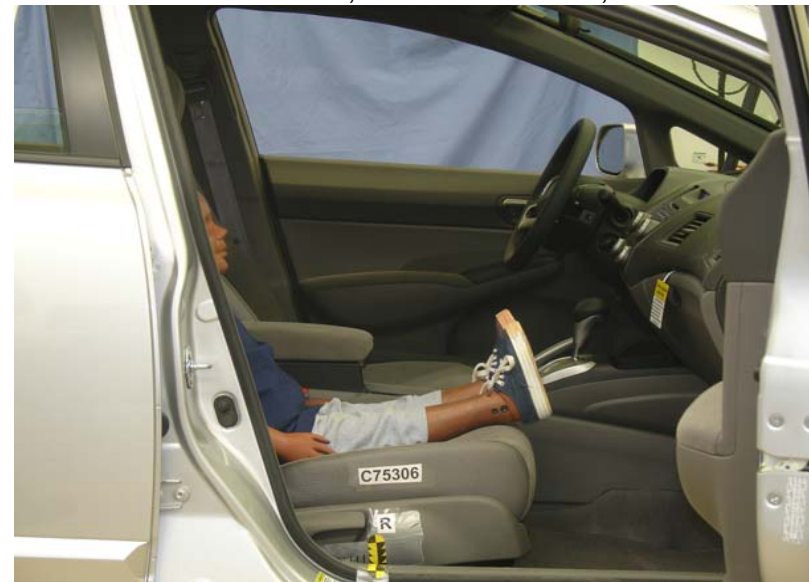
3-Year-Old Unbelted, Rearward Seat Track, Position 2
