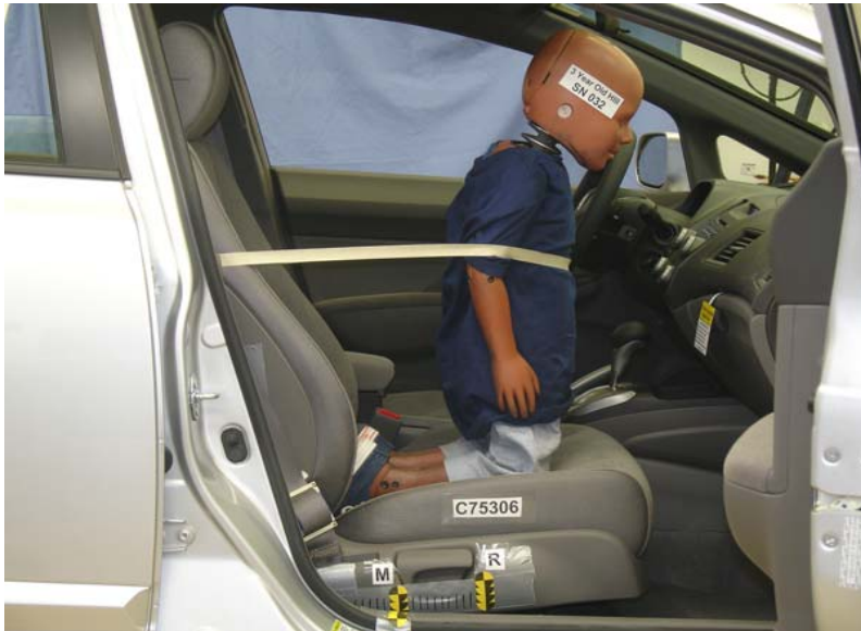
3-Year-Old Unbelted, Middle Seat Track, Position 6
