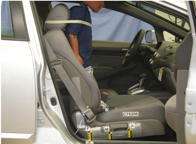
3-Year-Old Unbelted, Forward Seat Track, Position 5
