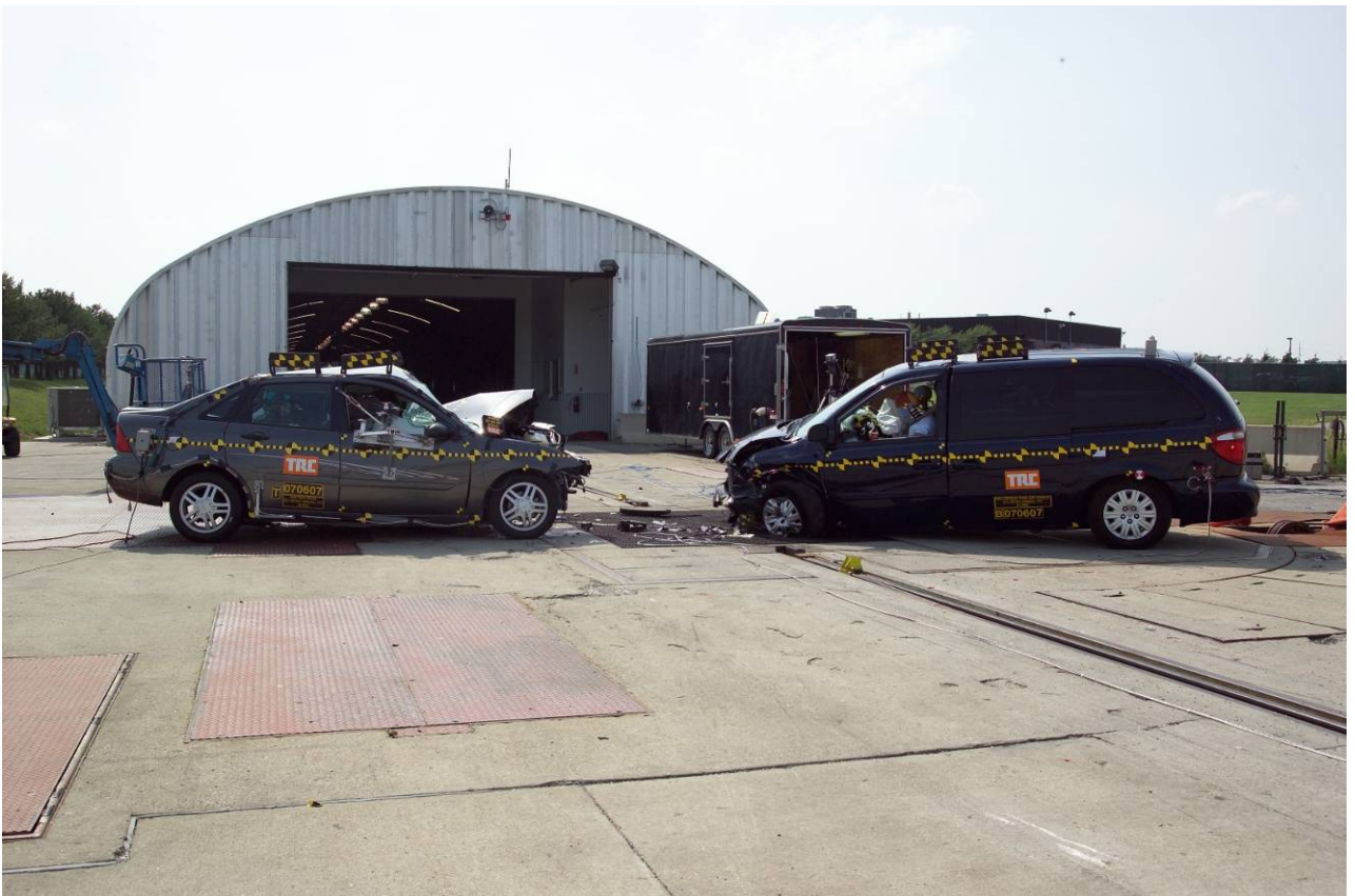
Figure A-4 Post-Test Overall - View 2
