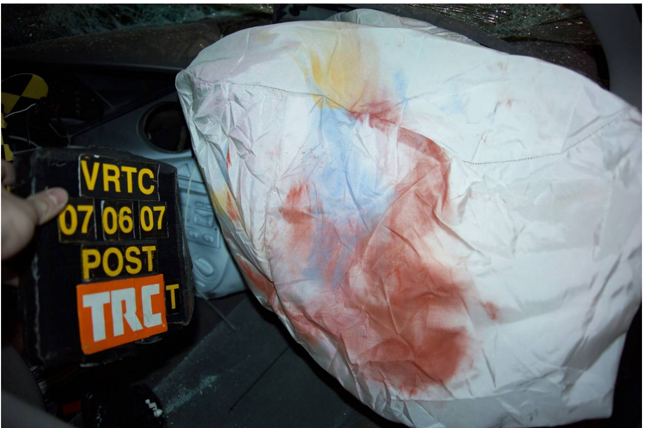
Figure A-122 Post-Test Target Vehicle Passenger Dummy Head Contact - View 1
