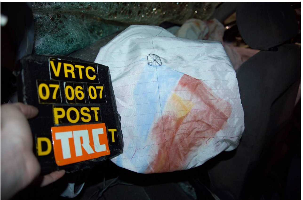
Figure A-118 Post-Test Target Vehicle Driver Dummy Head Contact View
