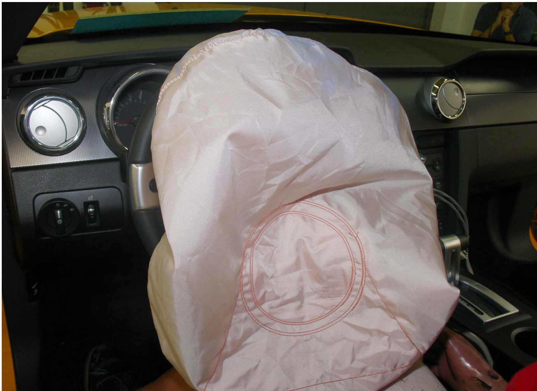
Post-Test 5th Fem. P2 Driver Dummy Airbag Contact Left Side View
