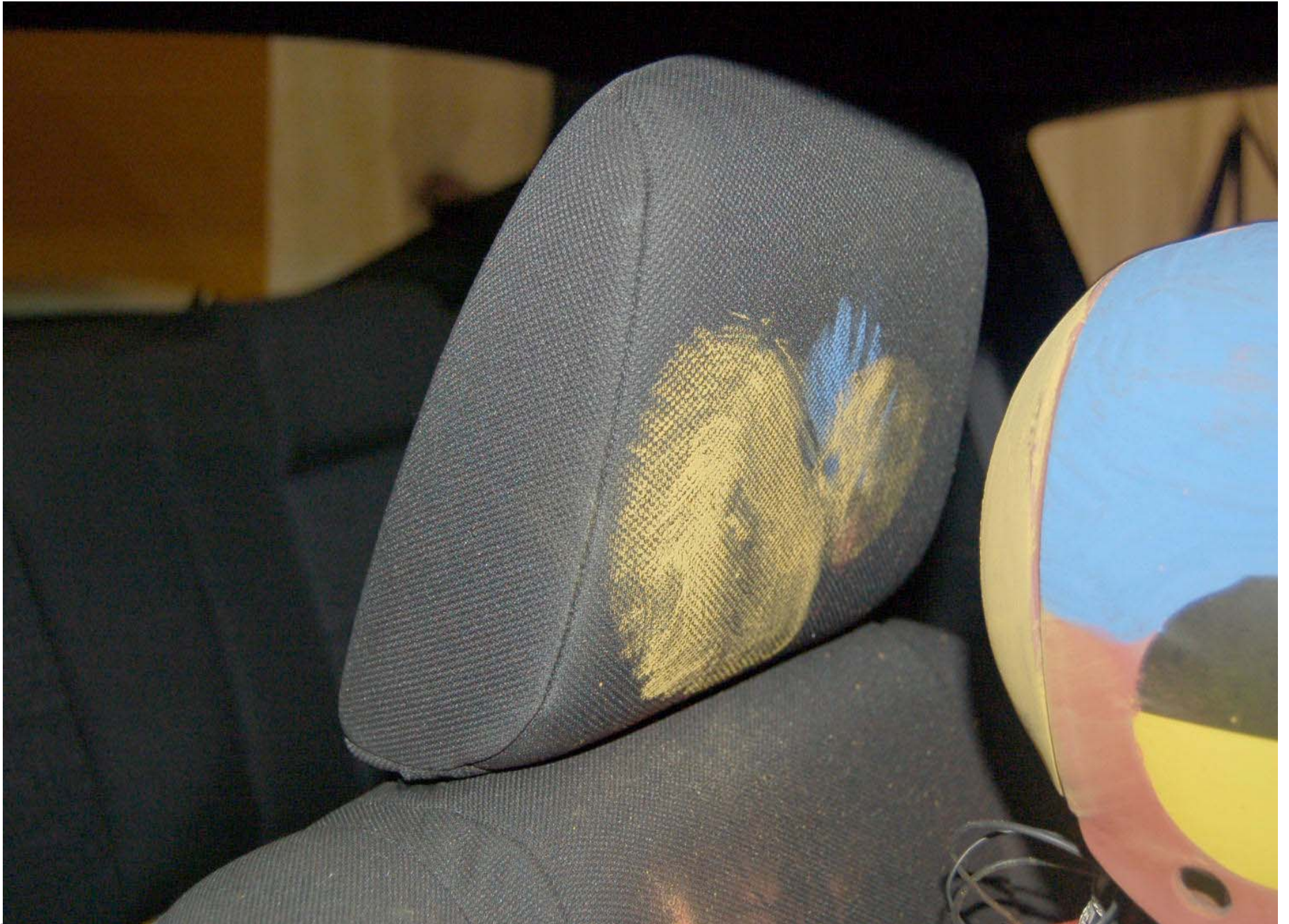
Post-Test Passenger Dummy Head Contact (headrest)
