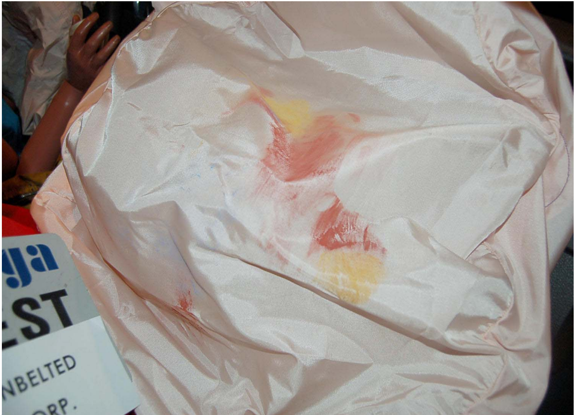
Post-Test Passenger Dummy Airbag Contact
