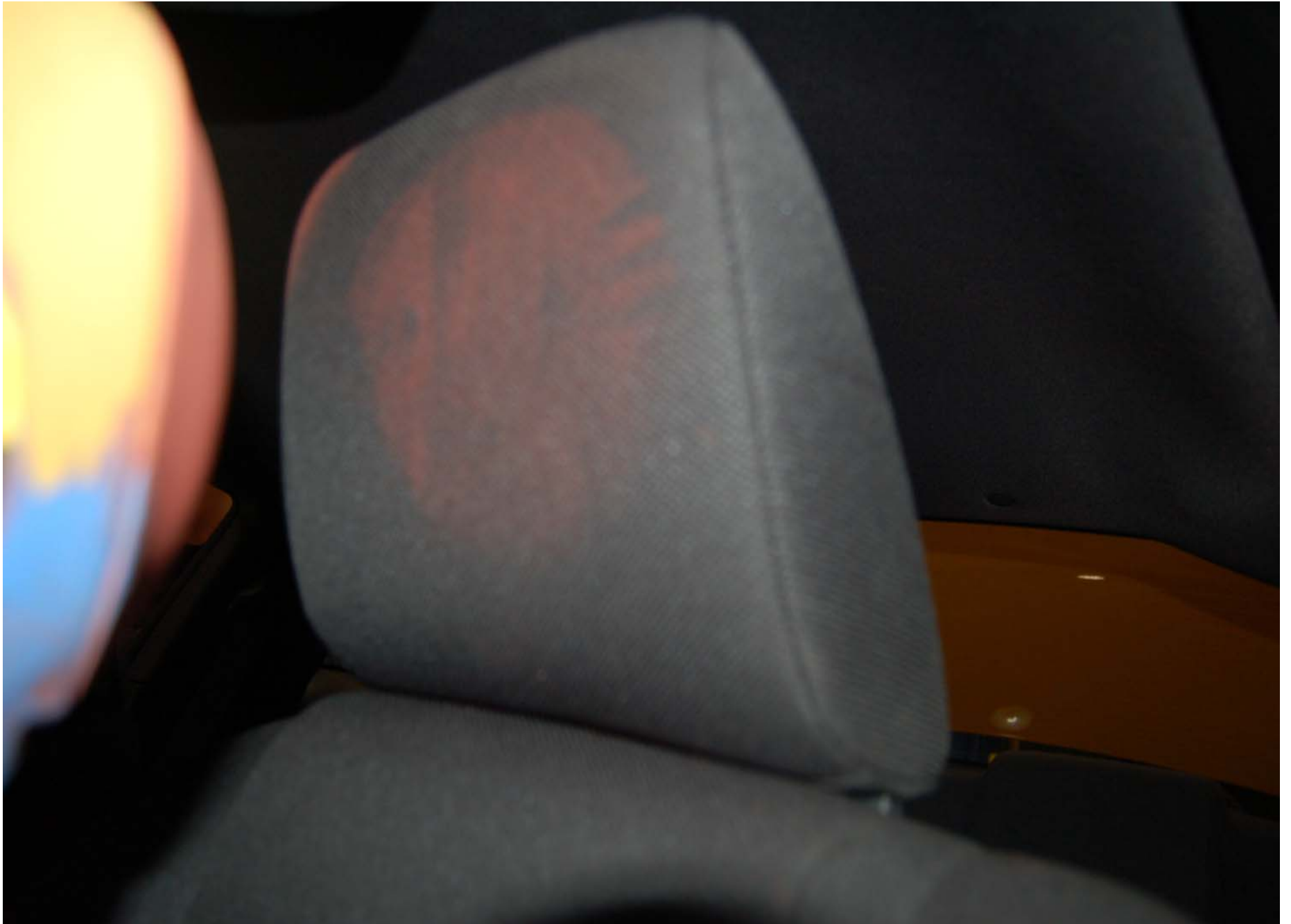
Post-Test Driver Dummy Head Contact (headrest)
