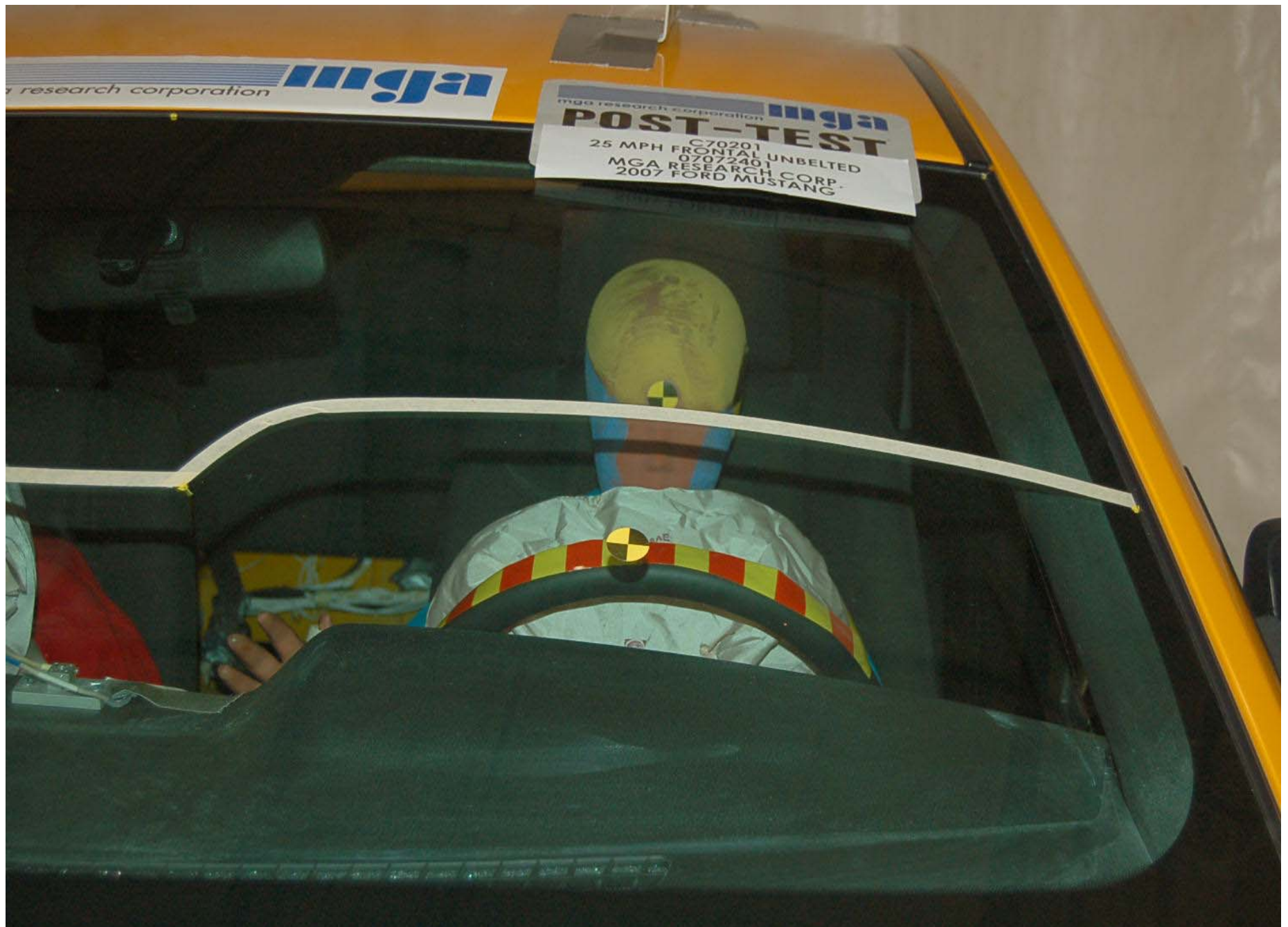
Post-Test Driver Dummy Front View (head position)
