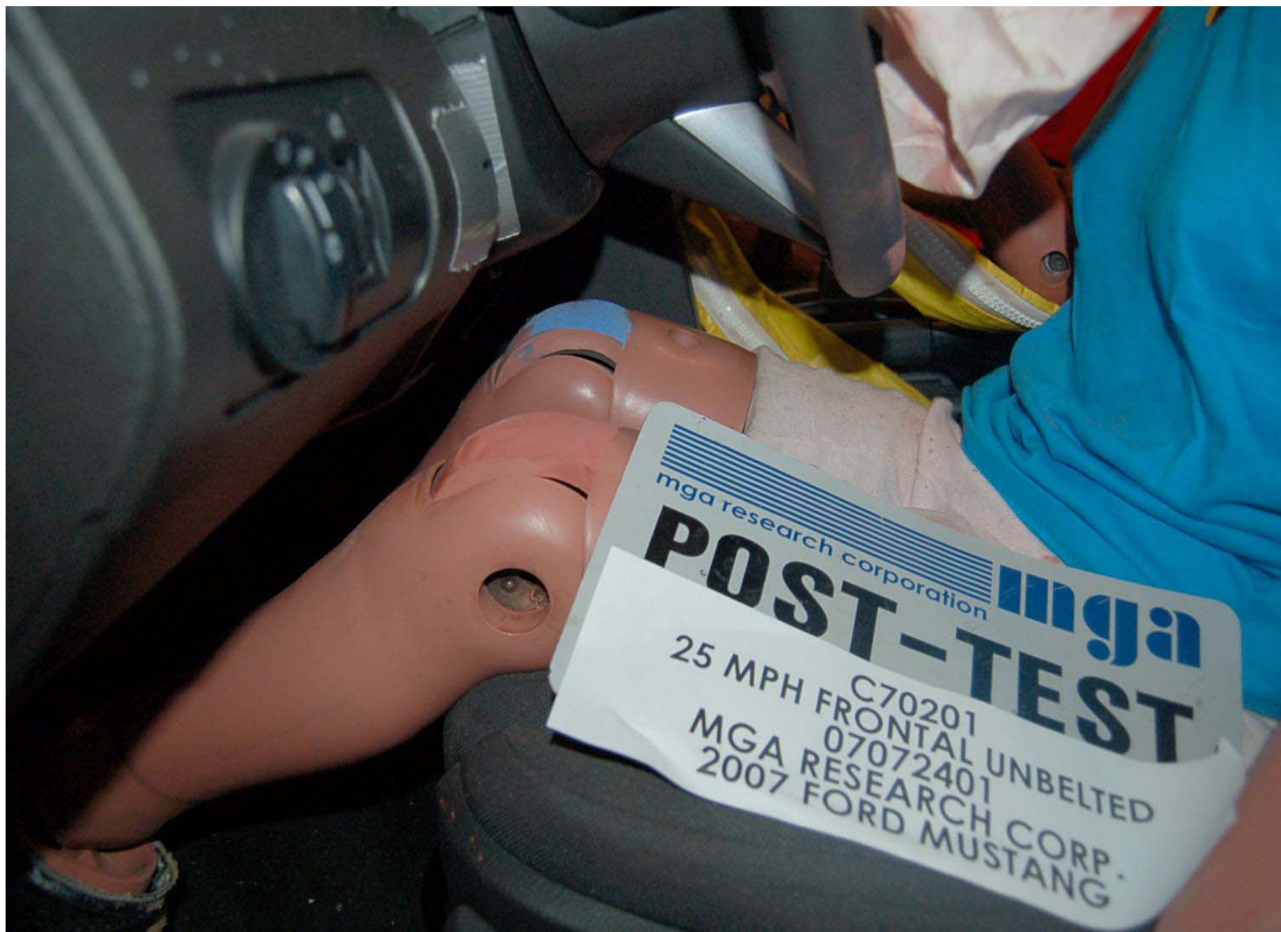
Post-Test Driver Side Knee Bolster View
