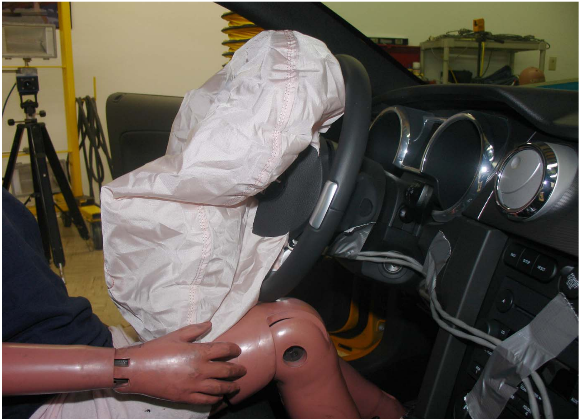
Post-Test 5th Fem. P1 Driver Dummy Airbag Contact Right Side View
