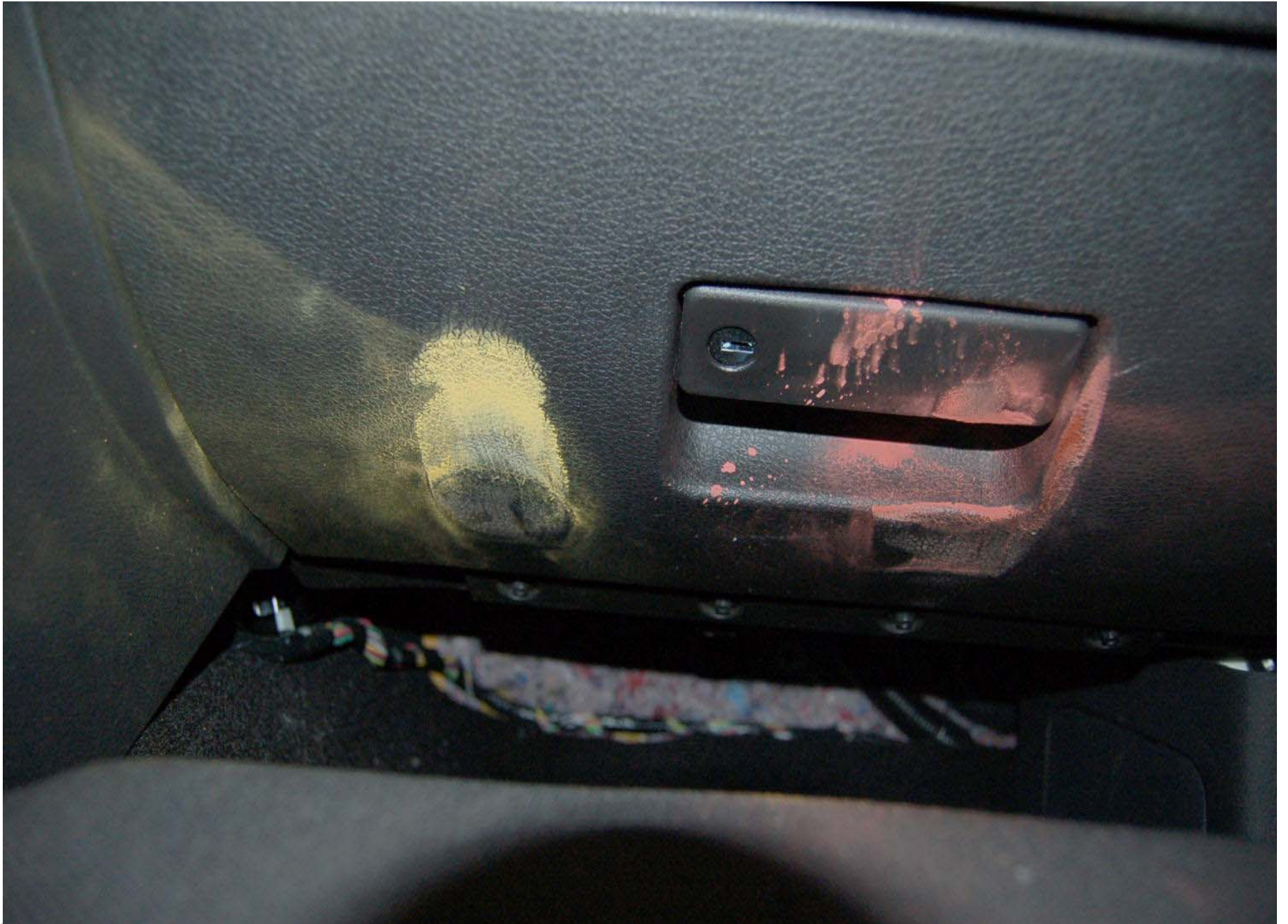
Post-Test Passenger Dummy Knee Contact
