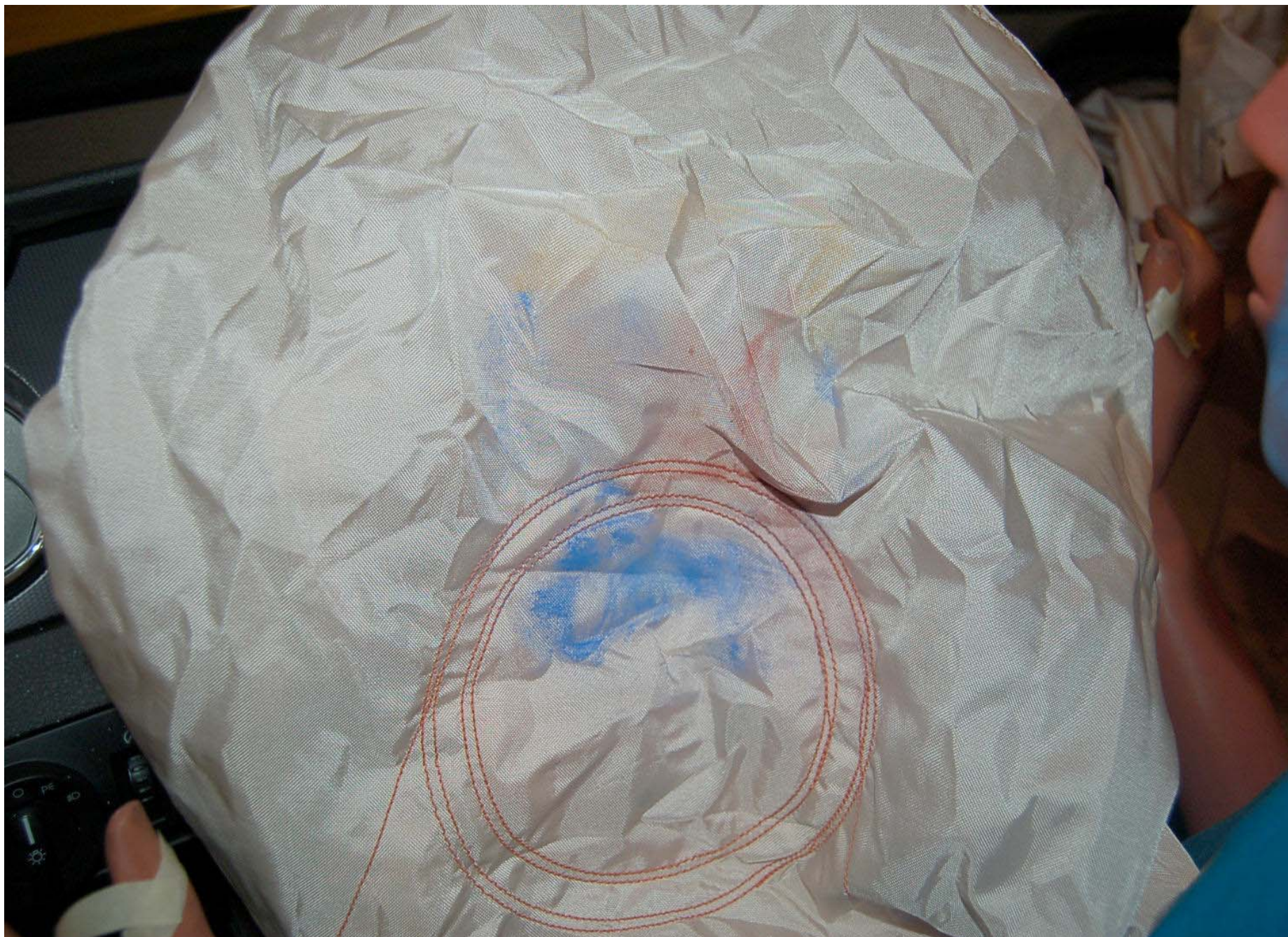
Post-Test Driver Dummy Airbag Contact
