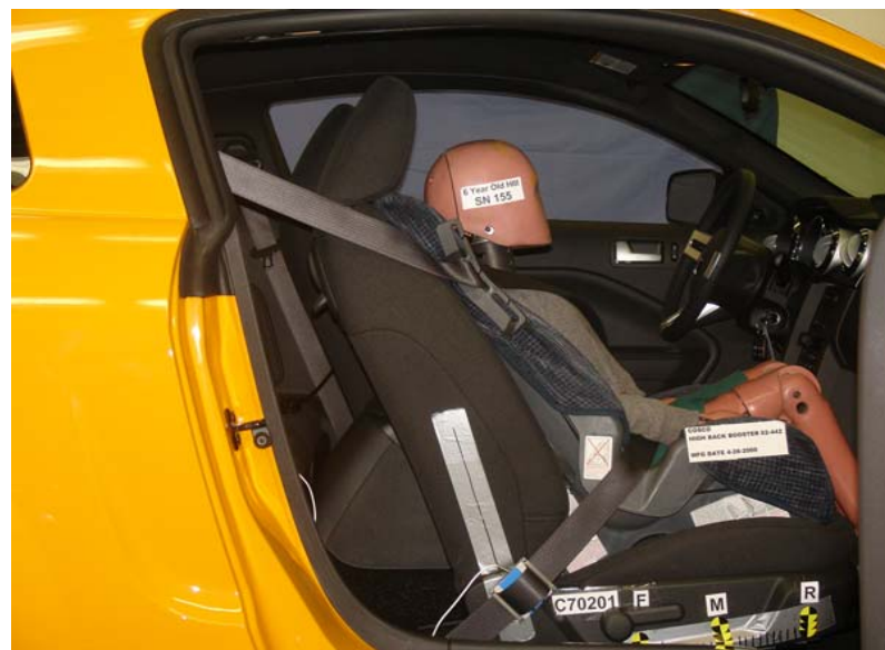
6-Year-Old Cosco High Back Booster Belted, Middle Seat Track
