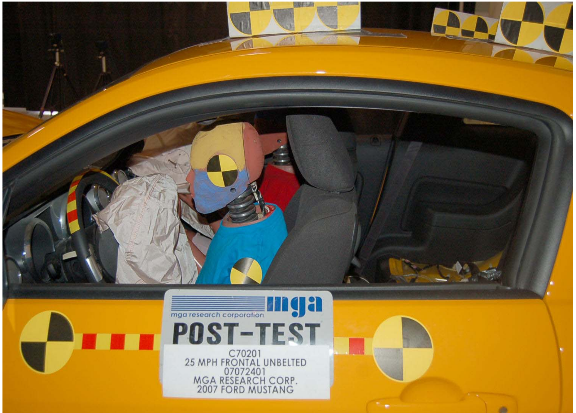
Post-Test Driver Dummy Position Left Side View
