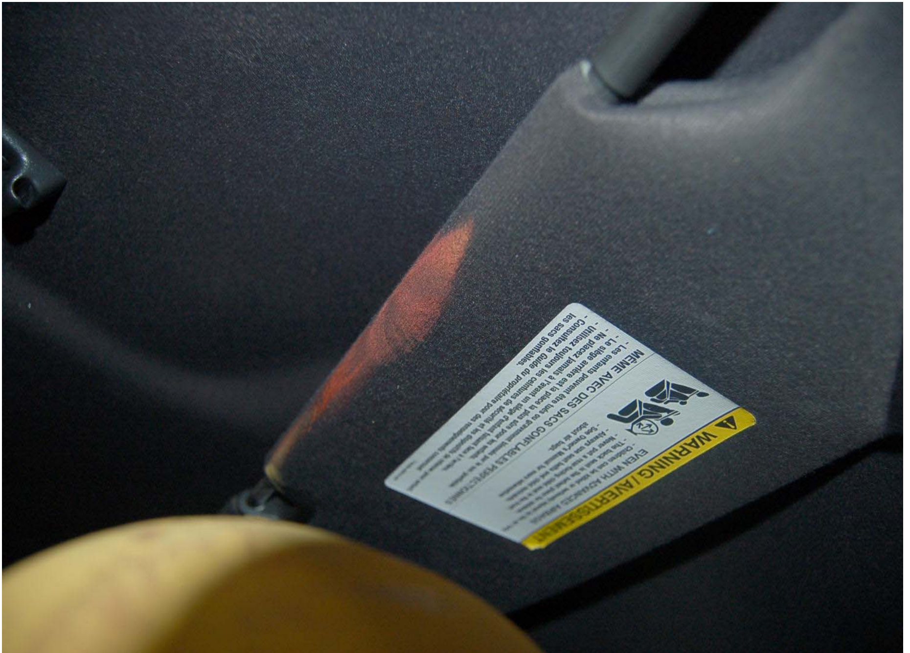
Post-Test Driver Dummy Head Contact (visor)
