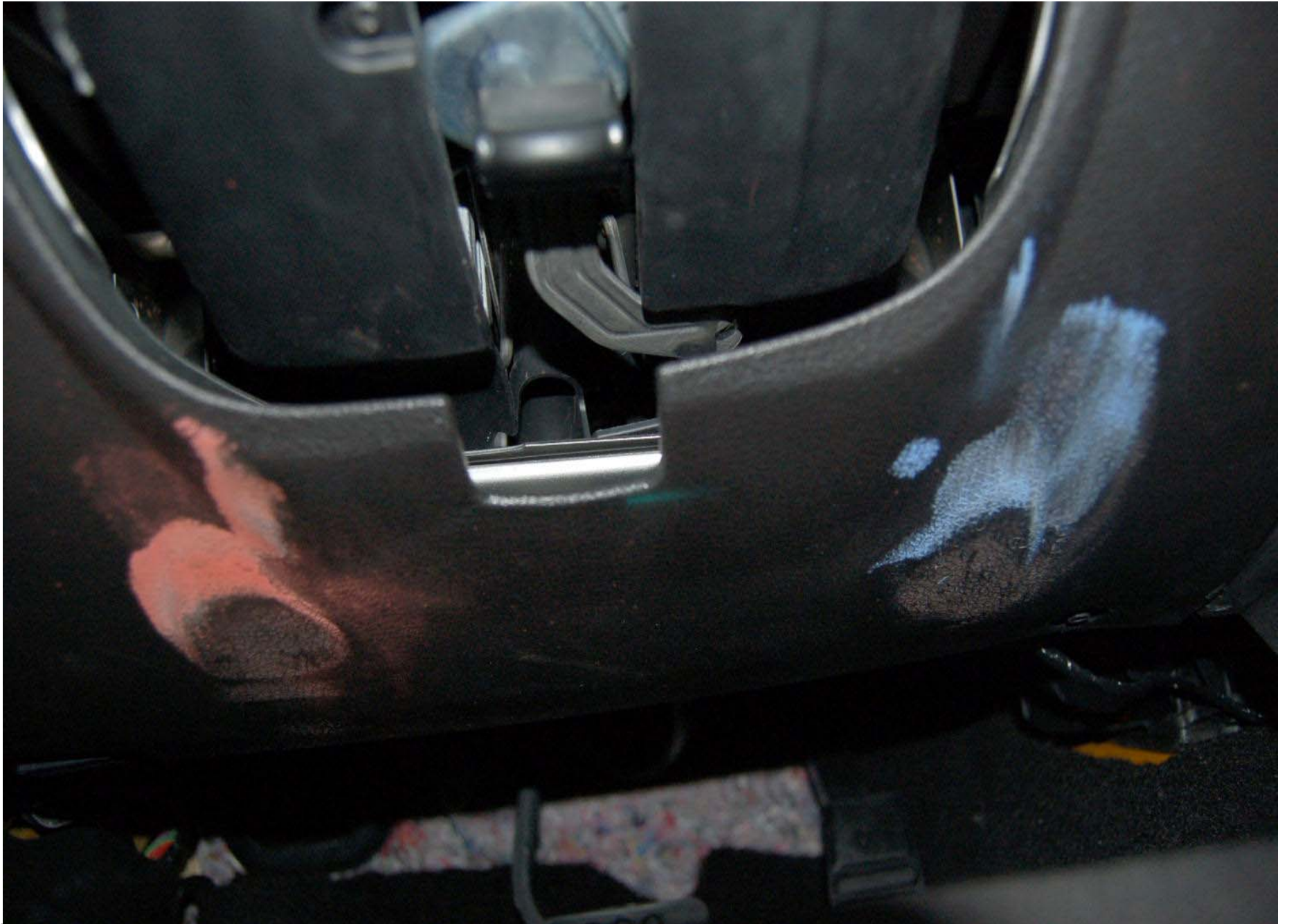
Post-Test Driver Dummy Knee Contact
