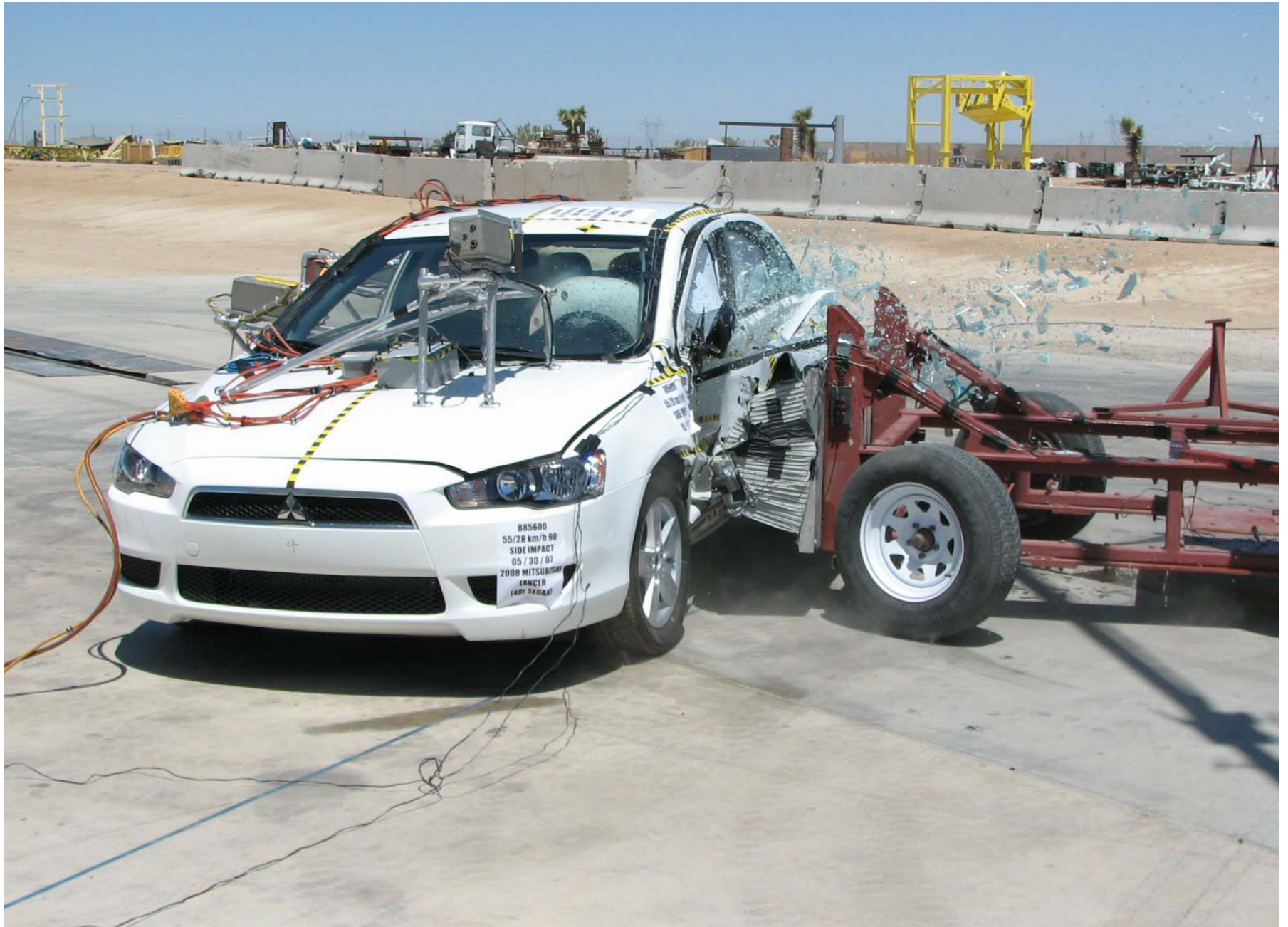
Figure A-65: Vehicle Impact
