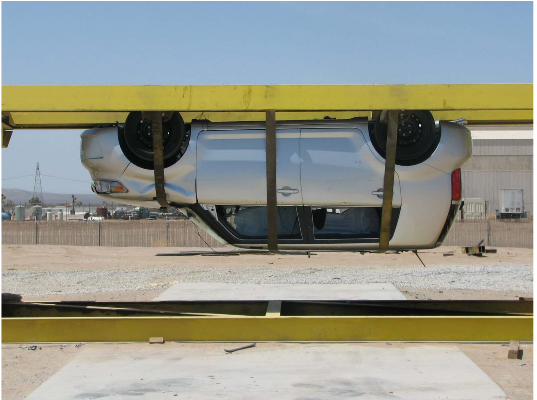
Figure A-63: Vehicle on Rollover Device (180°)
