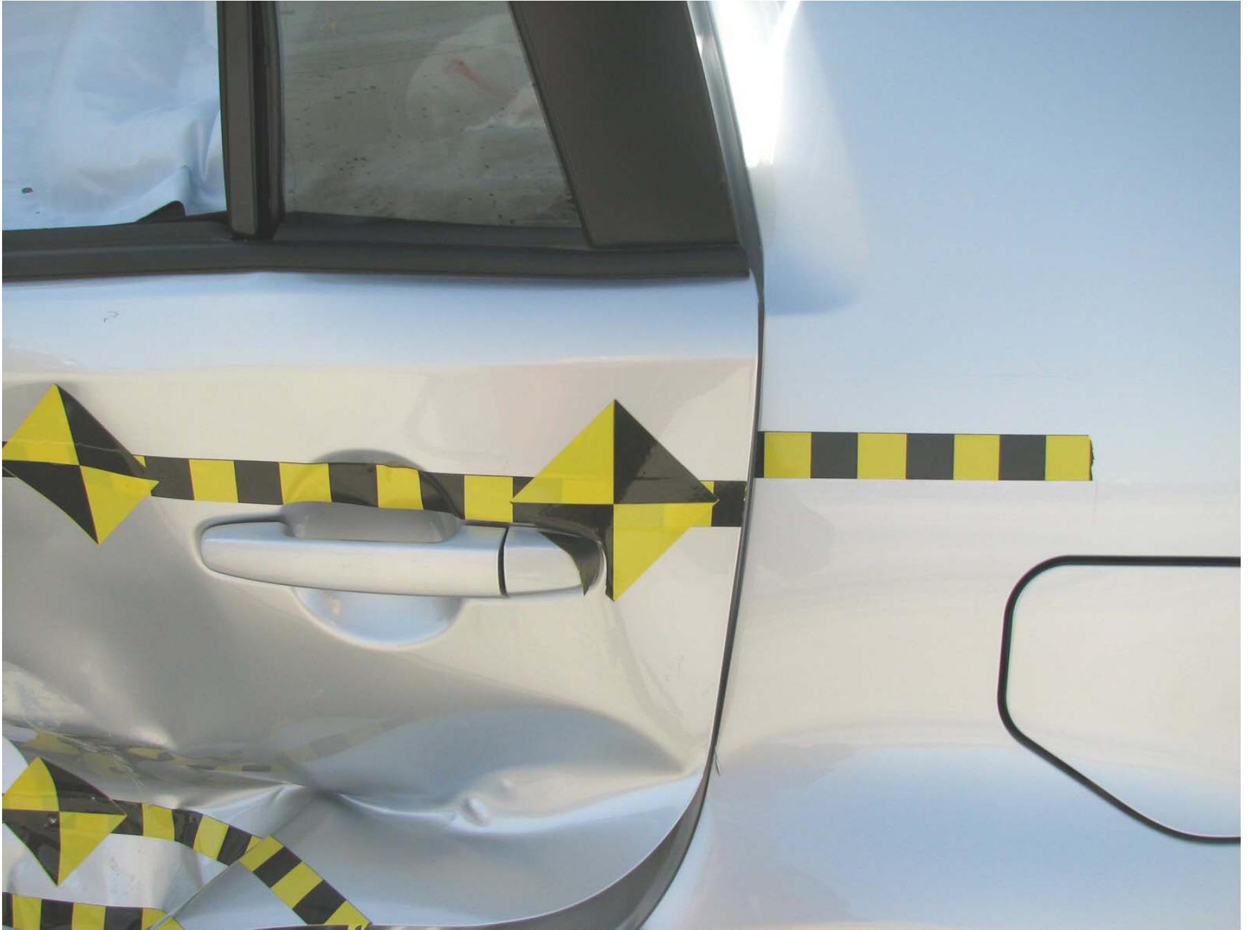
Figure A-34: Post-Test Left Rear Door
