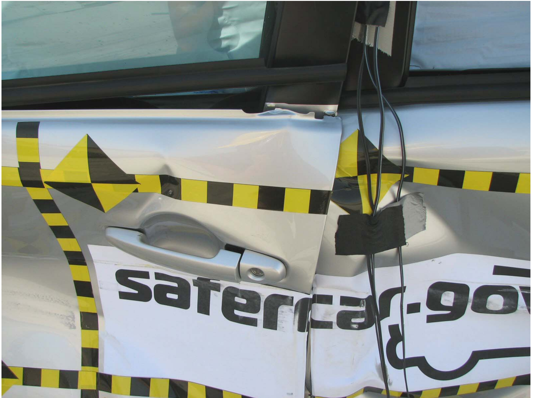
Figure A-32: Post-Test Left Front Door
