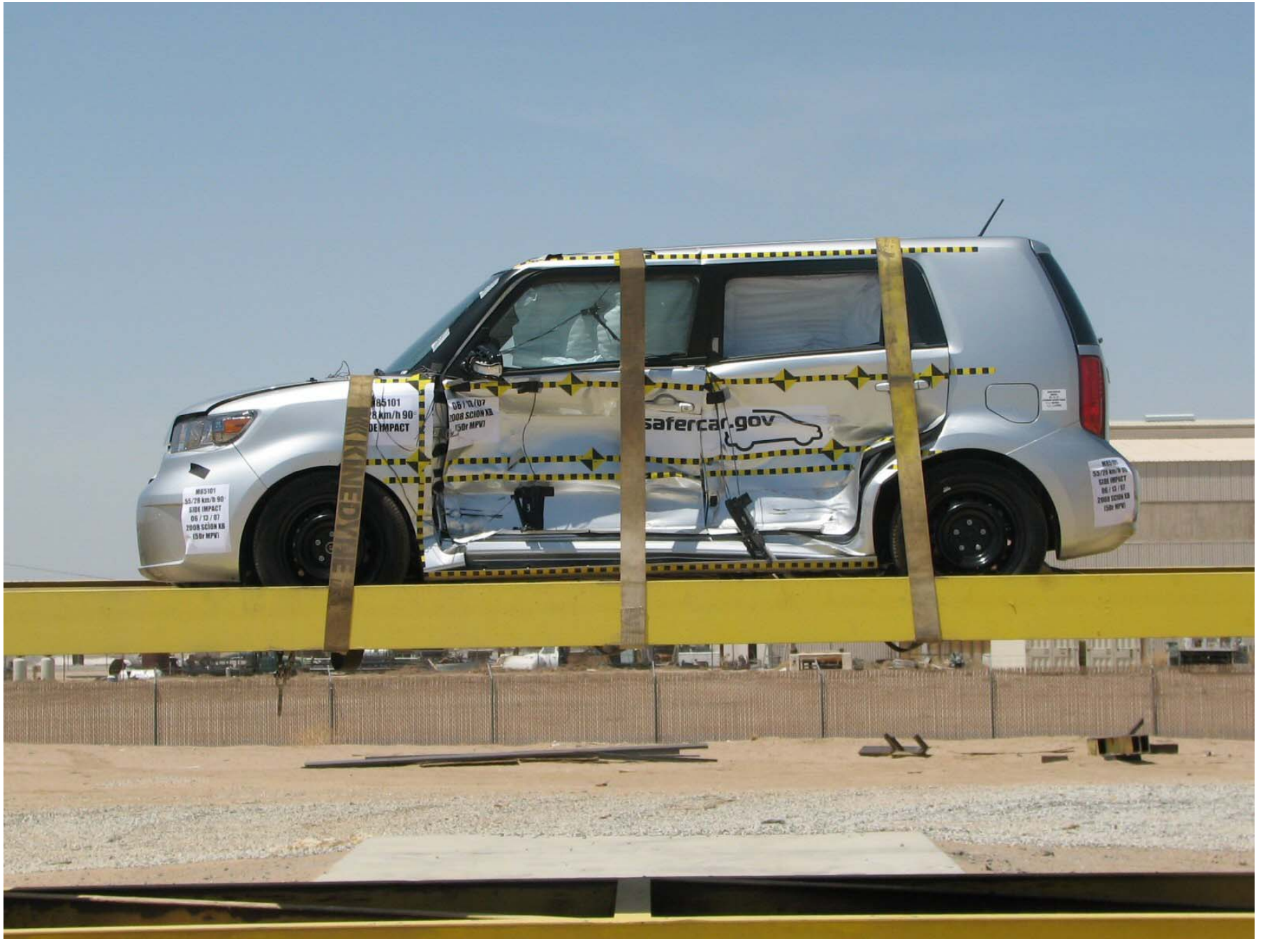
Figure A-61: Vehicle on Rollover Device (0°)
