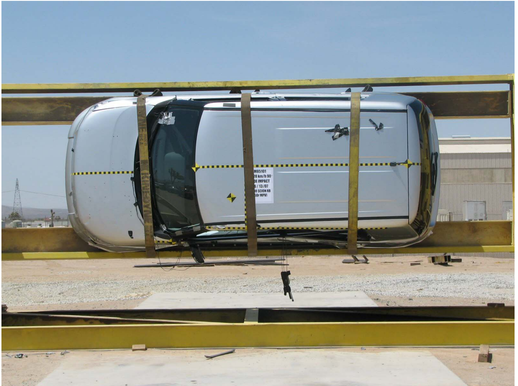
Figure A-62: Vehicle on Rollover Device (90°)
