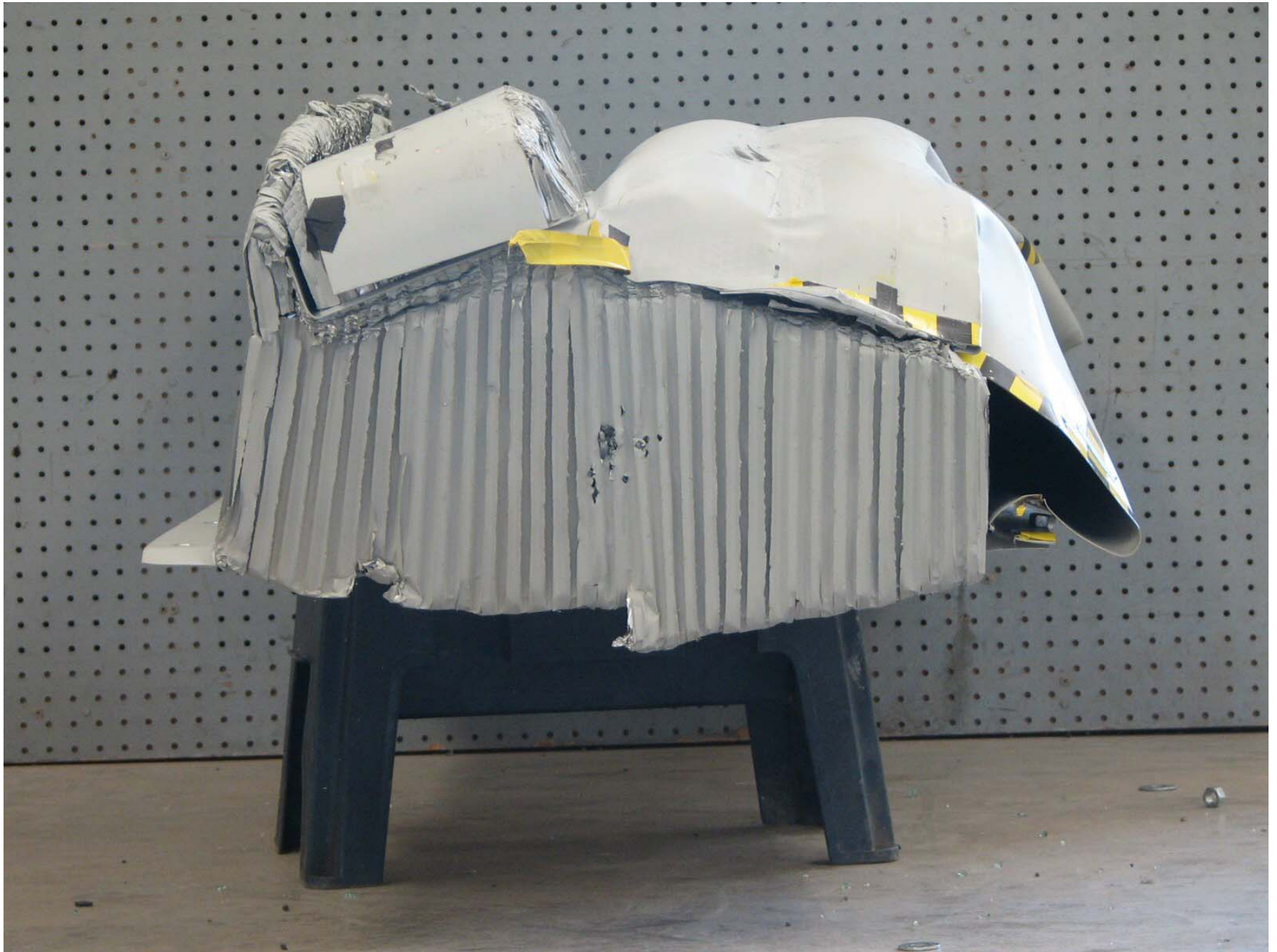
Figure A-60: Post-Test Left Side View of Deformable Barrier
