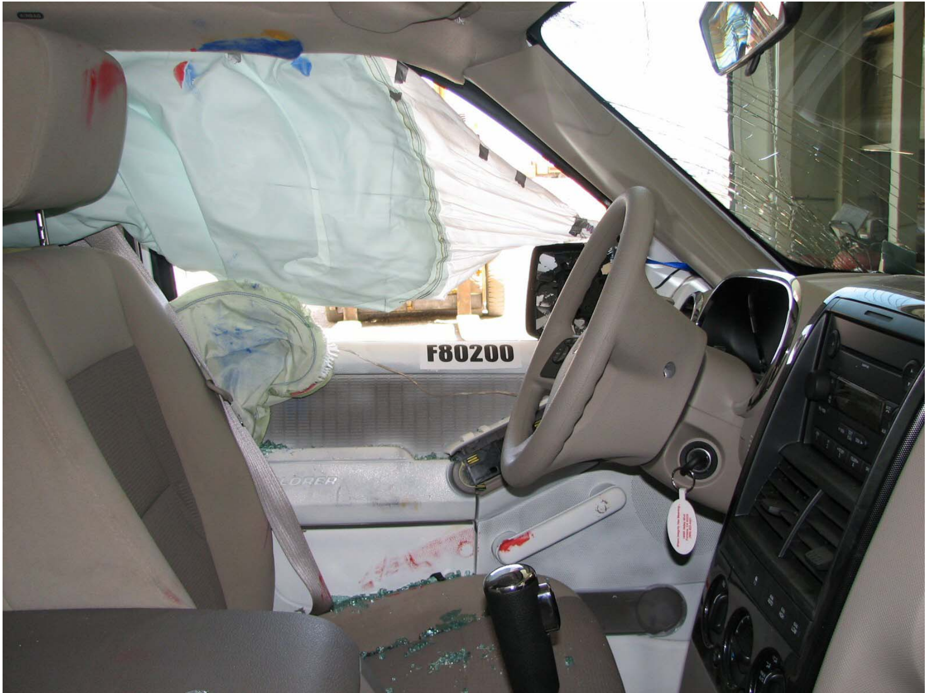
Figure A-43: Post-Test Front Door Panel (Interior)
