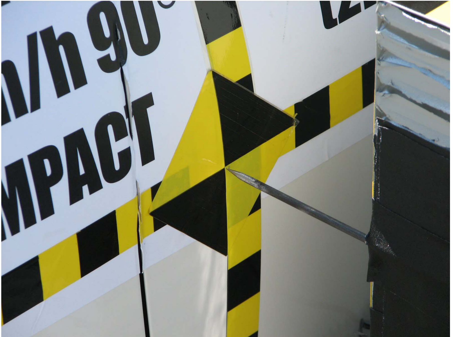
Figure A-25: Pre-Test Left Impact Point
