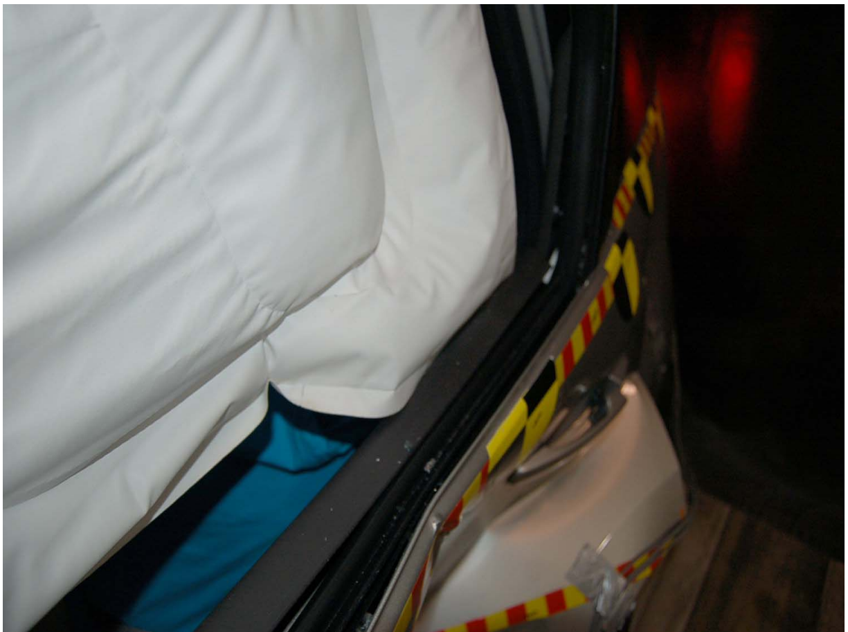
Post-Test Passenger Dummy Clearance From Door
