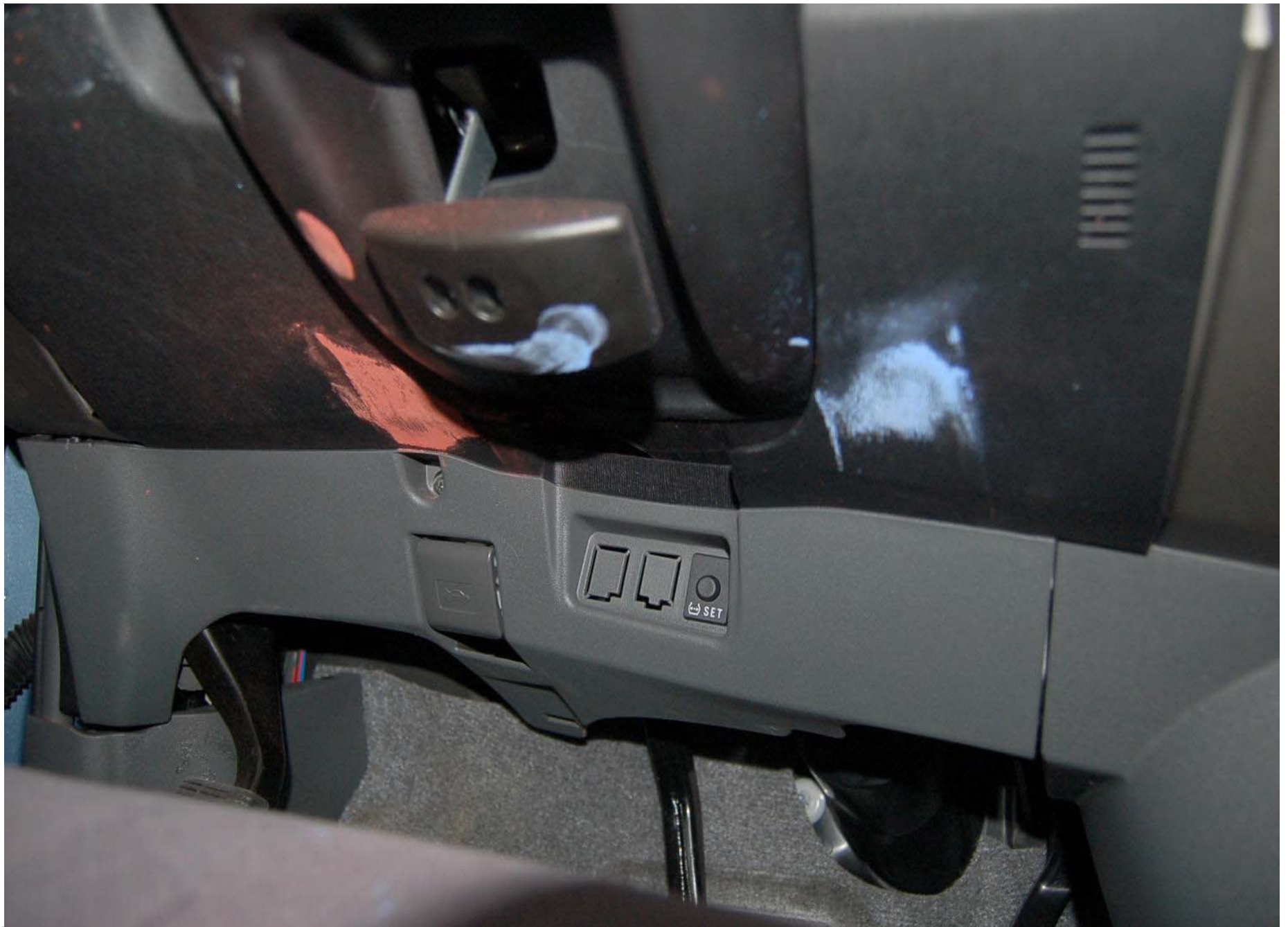
Post-Test Driver Dummy Knee Contact (view 1)
