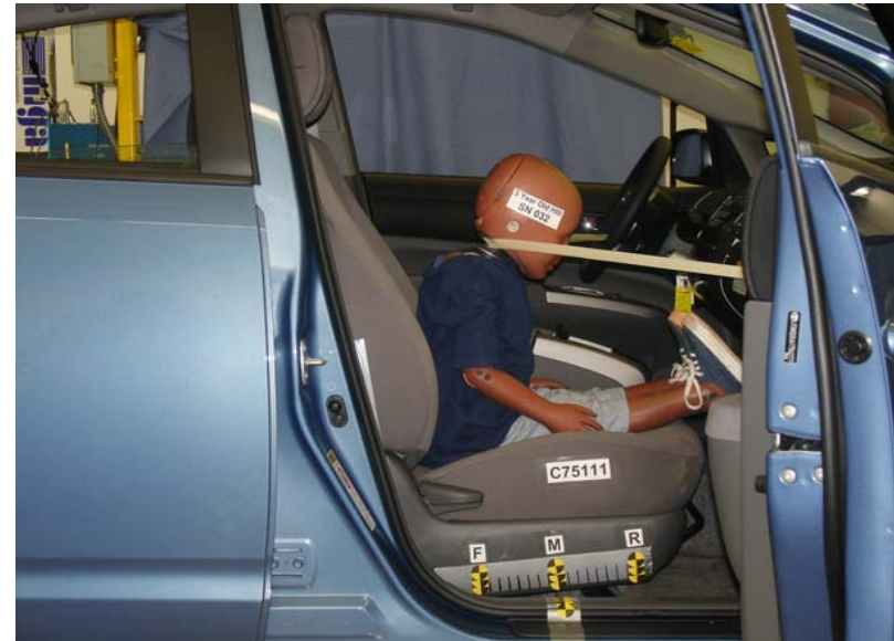
3-Year-Old Unbelted, Middle Seat Track, Position 3
