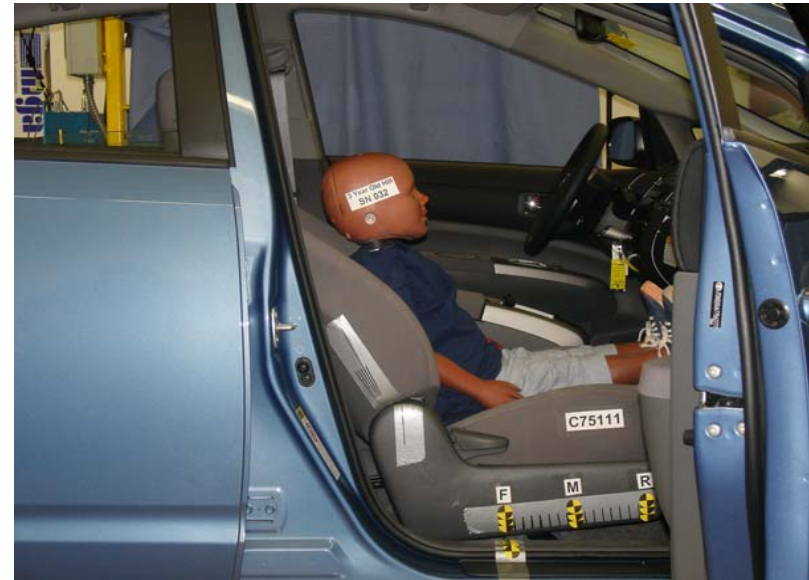
3-Year-Old Unbelted, Forward Seat Track, Position 2
