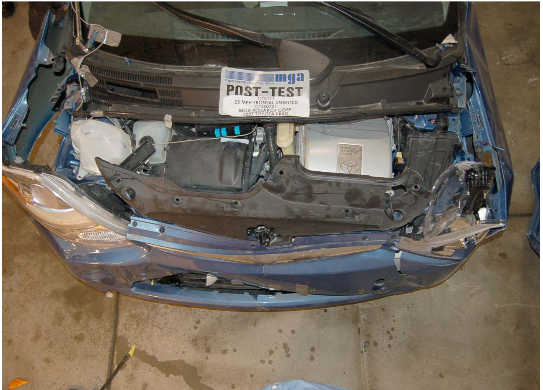
Post-Test Electrical Propulsion Components
