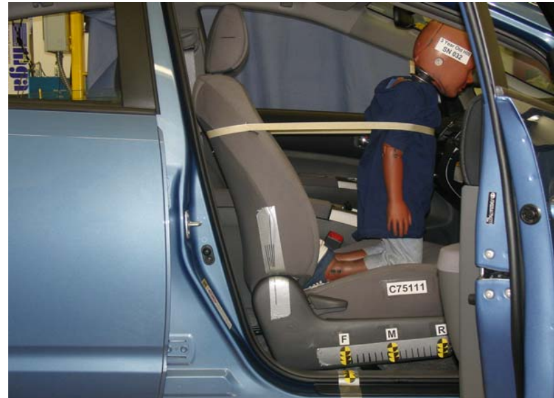
3-Year-Old Unbelted, Forward Seat Track, Position 6
