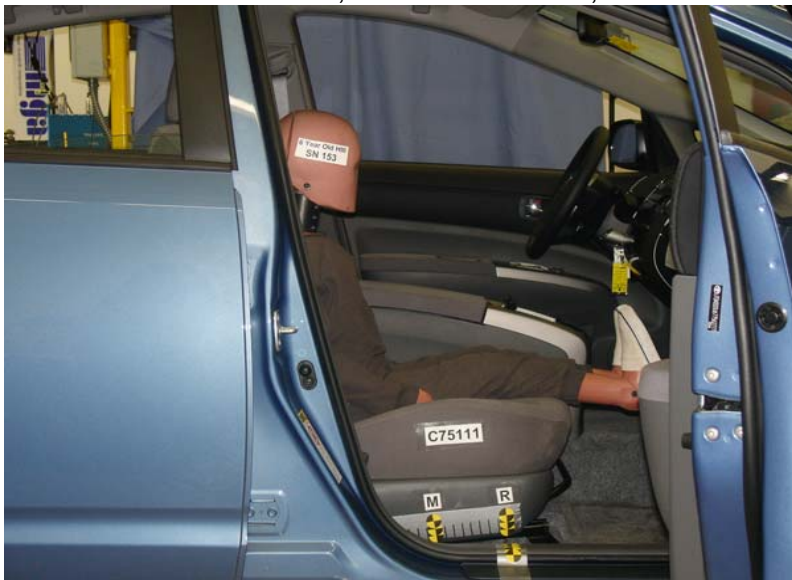
6-Year-Old Unbelted, Rearward Seat Track, Position 1
