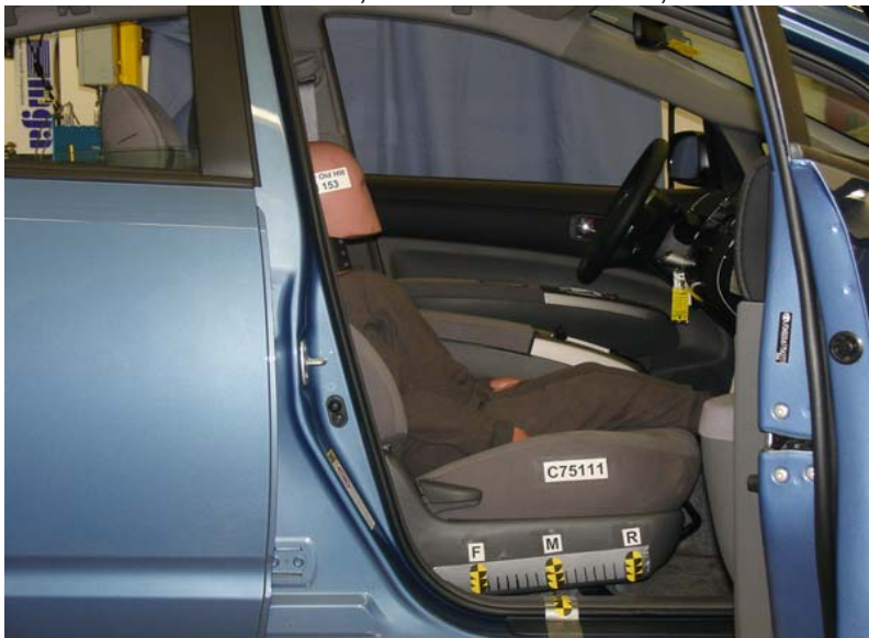
6-Year-Old Unbelted, Middle Seat Track, Position 2
