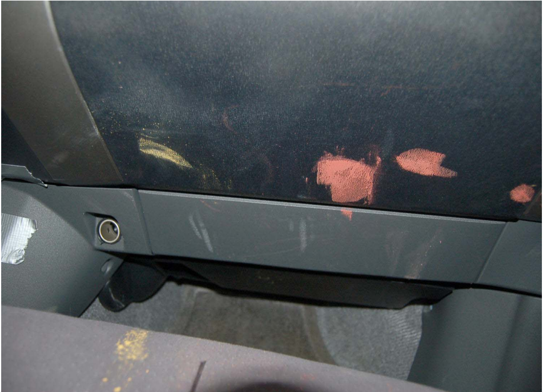
Post-Test Passenger Dummy Knee Contact
