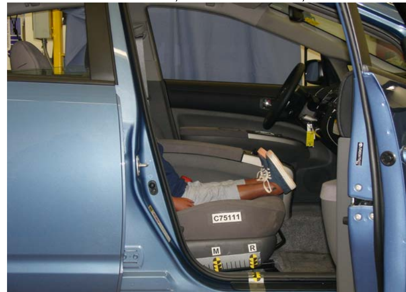
3-Year-Old Unbelted, Rearward Seat Track, Position 2
