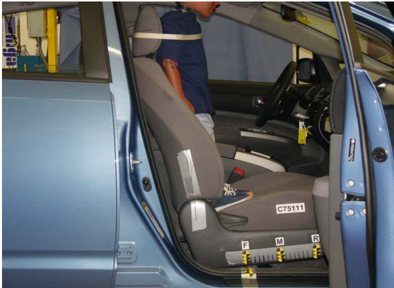
3-Year-Old Unbelted, Forward Seat Track, Position 5
