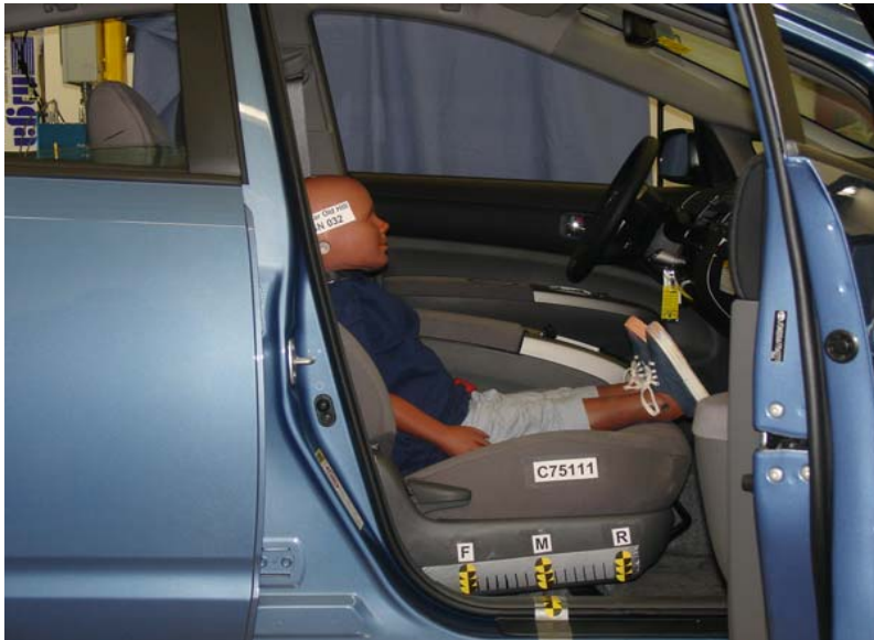
3-Year-Old Unbelted, Middle Seat Track, Position 2
