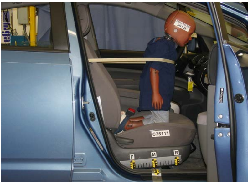
3-Year-Old Unbelted, Middle Seat Track, Position 6
