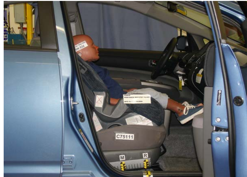
3-Year-Old Cosco High Back Booster Cinched With Harness, Rearward Seat Track
