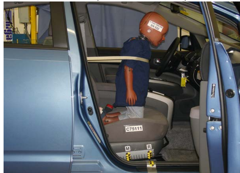
3-Year-Old Unbelted, Rearward Seat Track, Position 6
