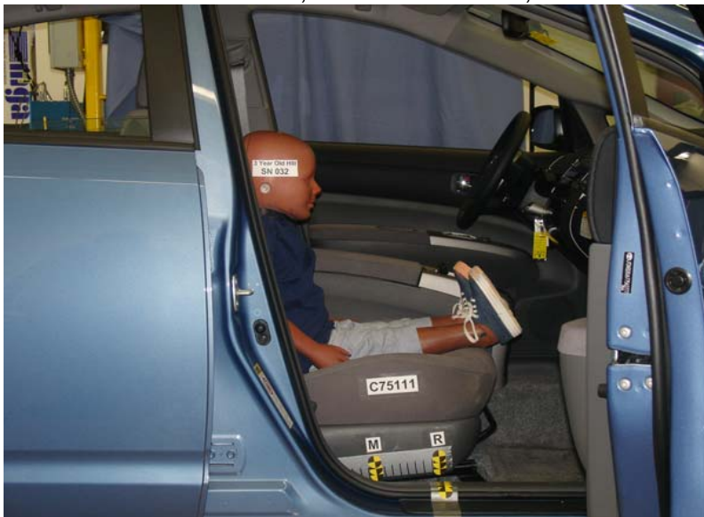
3-Year-Old Unbelted, Rearward Seat Track, Position 1
