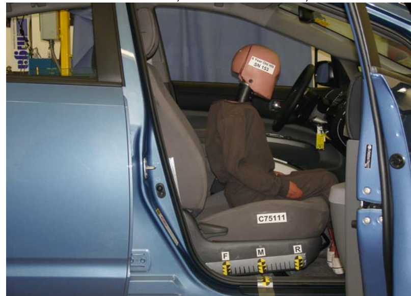
6-Year-Old Unbelted, Middle Seat Track, Position 3
