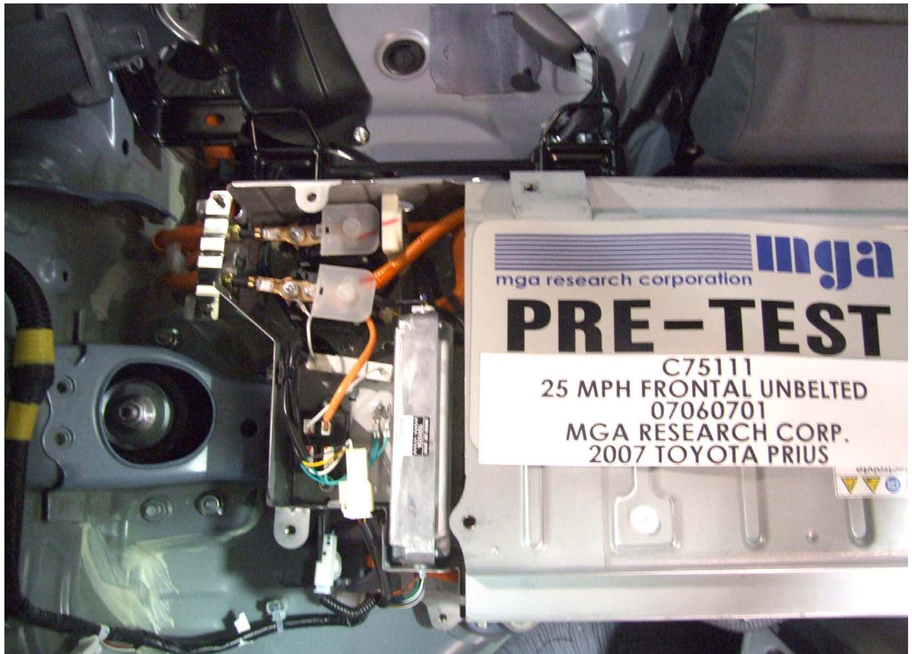
Pre-Test High Voltage Interconnect
