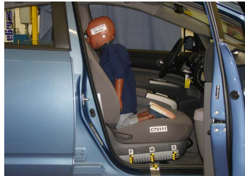
3-Year-Old Unbelted, Middle Seat Track, Position 7
