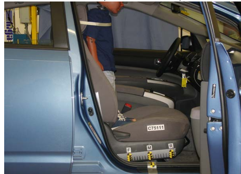
3-Year-Old Unbelted, Middle Seat Track, Position 5
