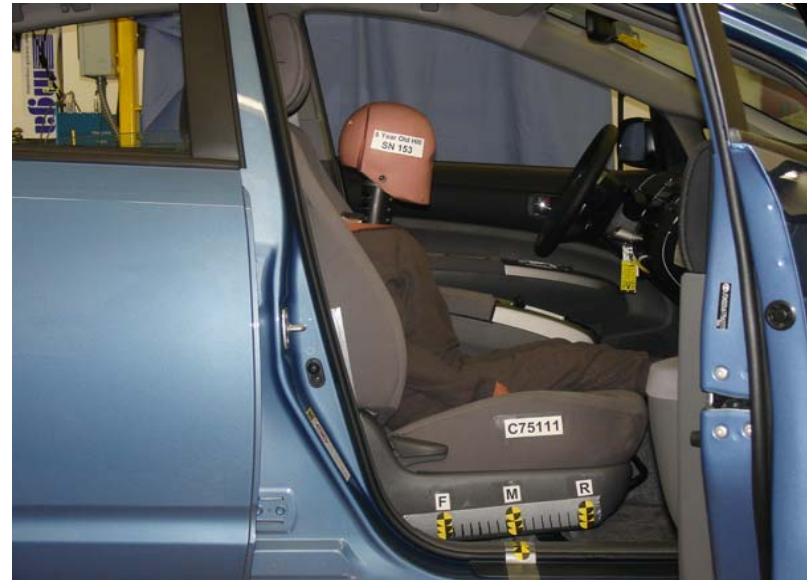
6-Year-Old Unbelted, Middle Seat Track, Position 1
