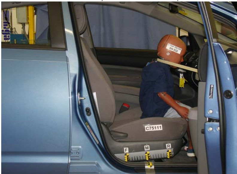
3-Year-Old Unbelted, Middle Seat Track, Position 4
