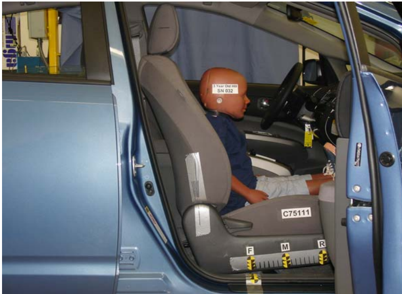
3-Year-Old Unbelted, Forward Seat Track, Position 1
