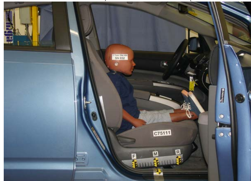
3-Year-Old Unbelted, Middle Seat Track, Position 1
