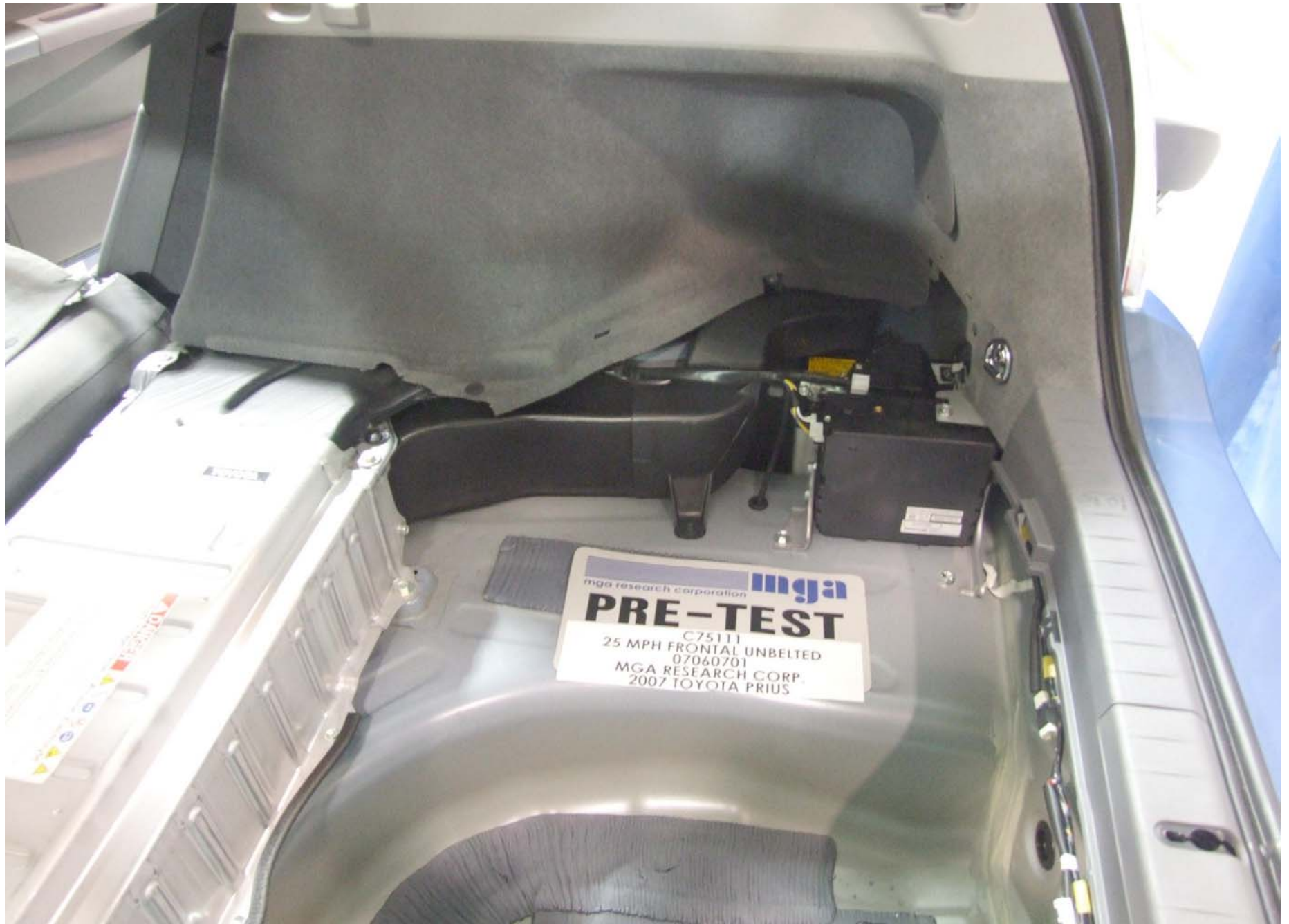
Pre-Test Propulsion Battery Venting System
