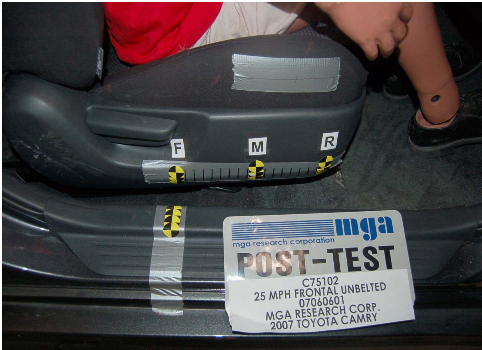
Post-Test Passenger Dummy Seat Position
