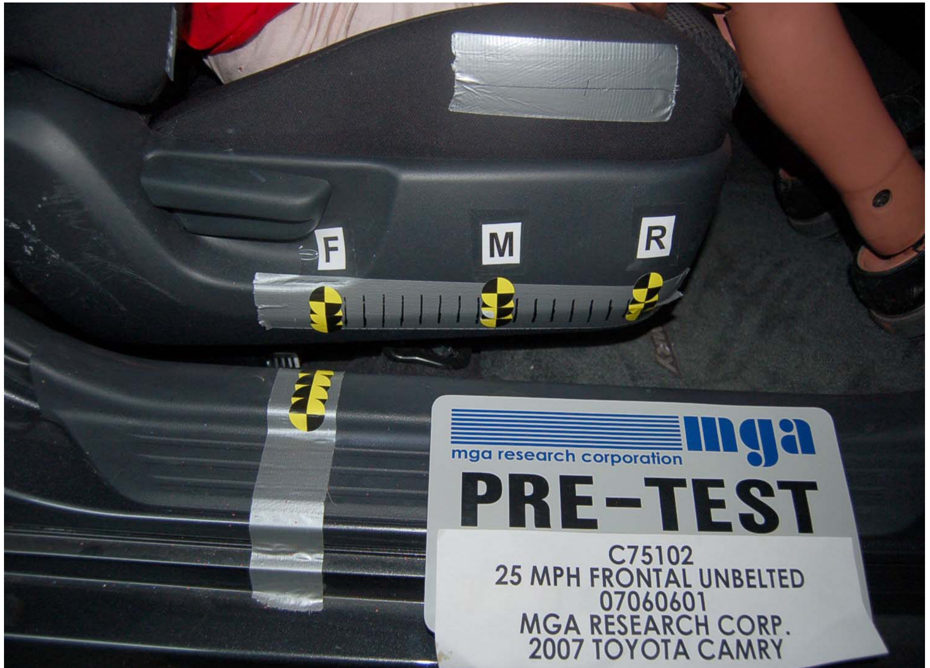
Pre-Test Passenger Dummy Seat Position
