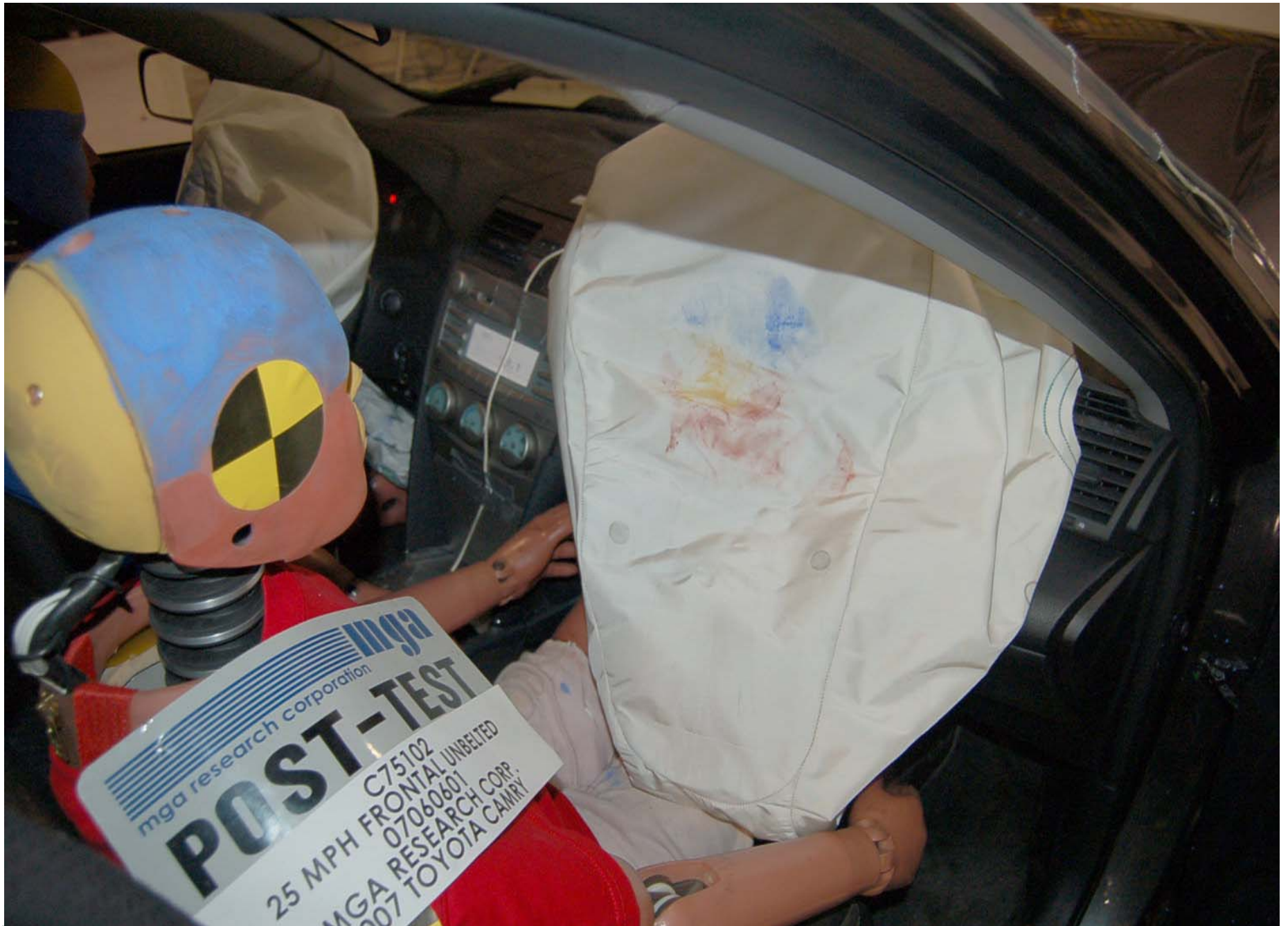
Post-Test Passenger Dummy Airbag Contact
