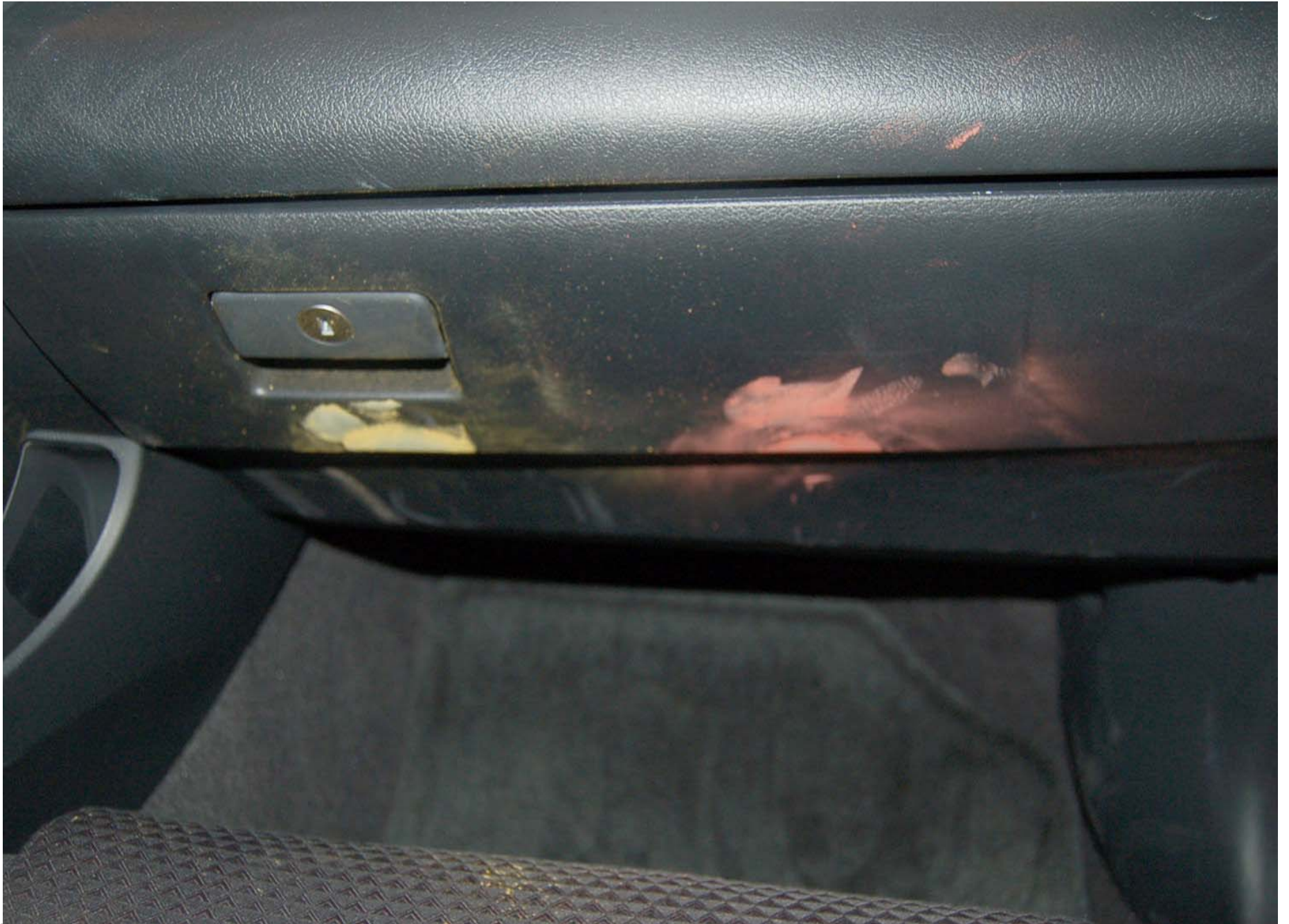
Post-Test Passenger Dummy Knee Contact
