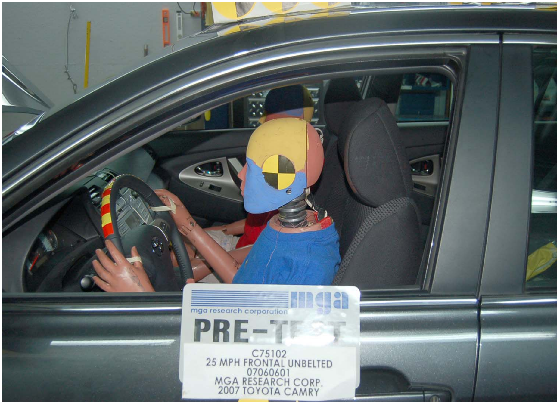
Pre-Test Driver Dummy Position Left Side View
