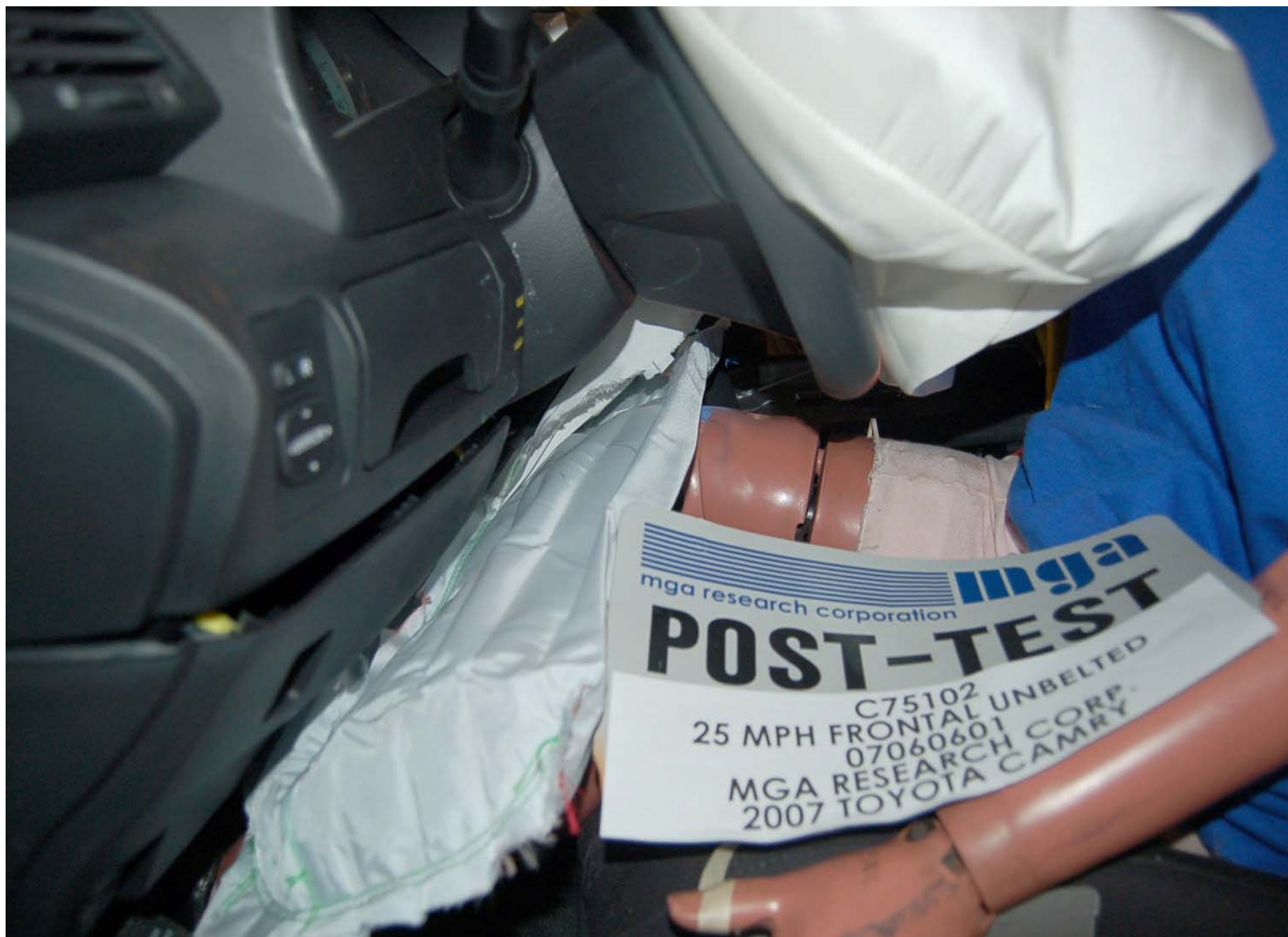
Post-Test Driver Side Knee Bolster View
