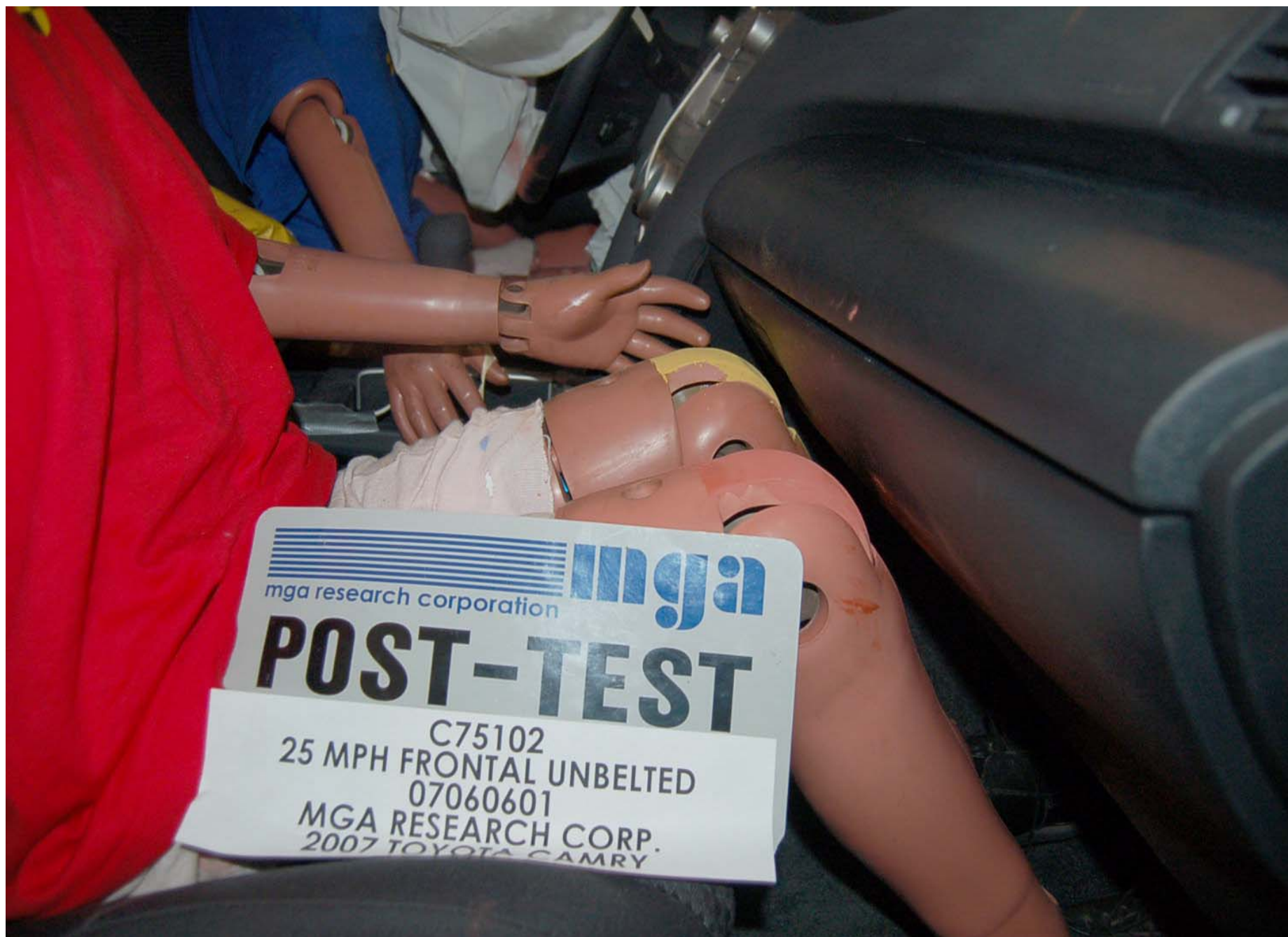
Post-Test Passenger Side Knee Bolster View
