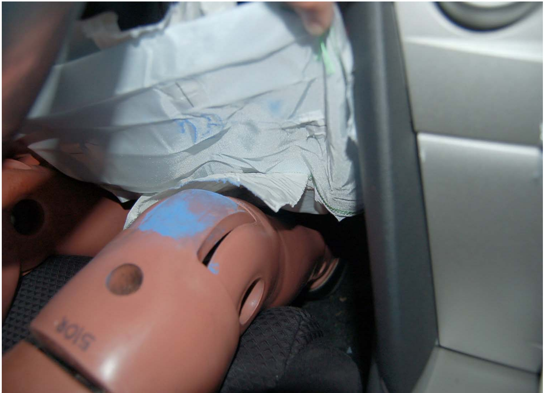
Post-Test Driver Dummy Knee Contact (view 2)
