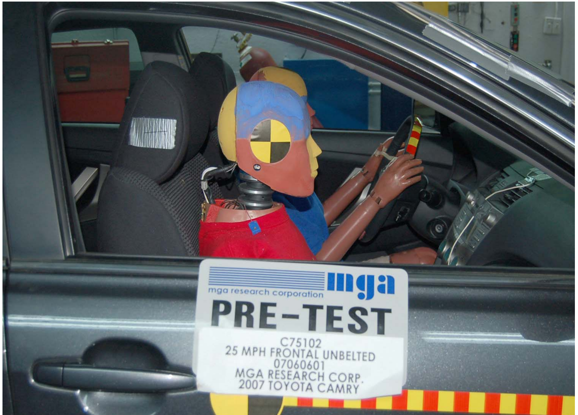
Pre-Test Passenger Dummy Position Right Side View
