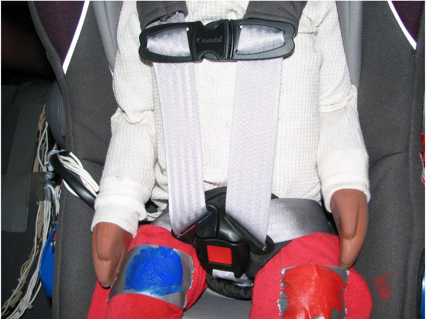
Figure D2-12: Pre-Test Position 3 Front View (Seat Belt Position)
