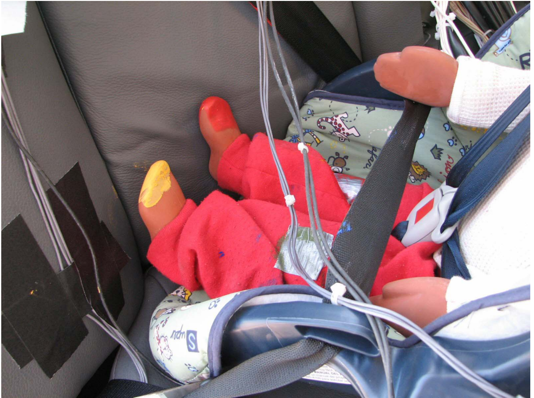
Figure D2-18: Post-Test Position 3 Dummy Legs
