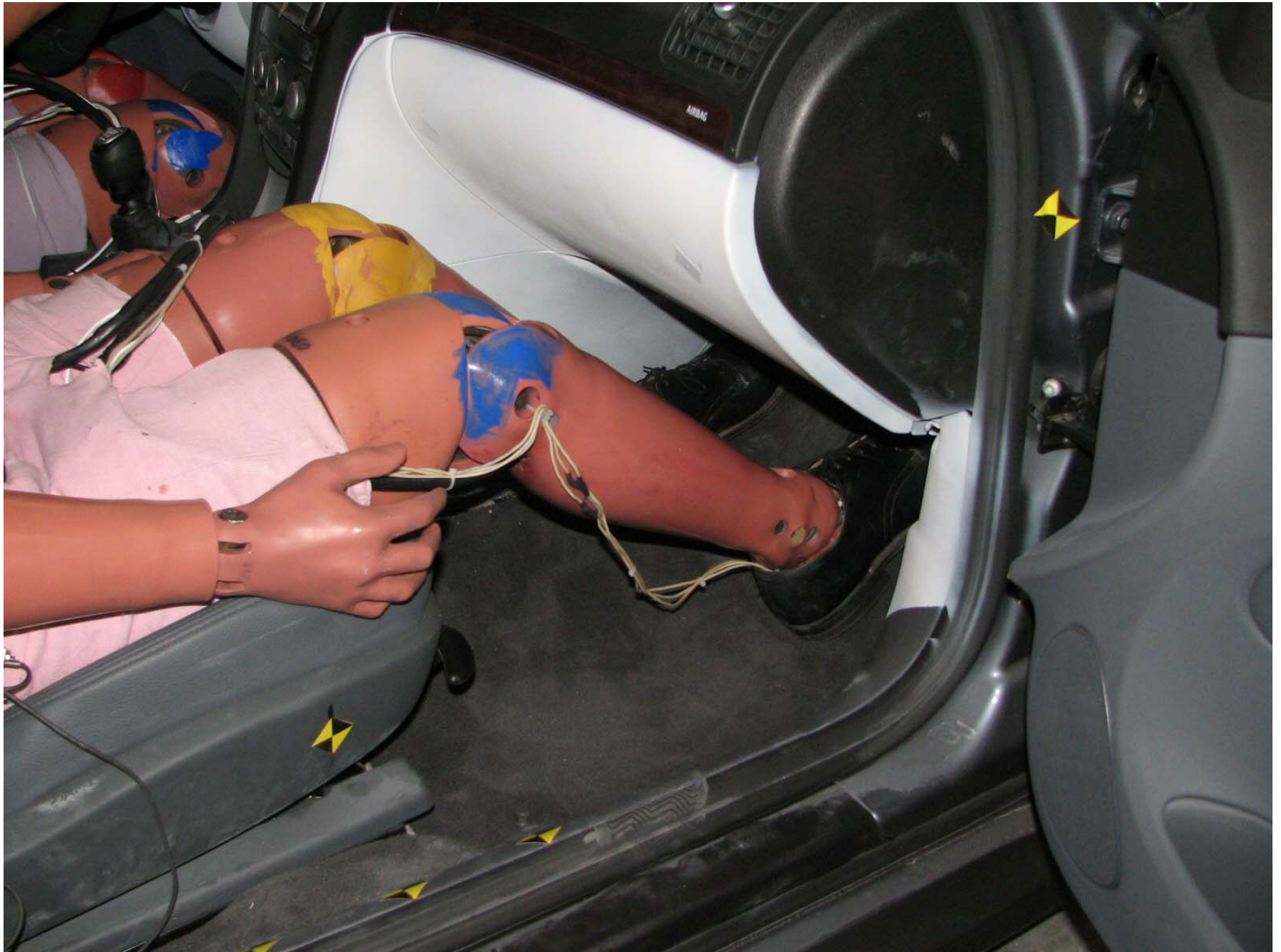
Figure A-50: Pre-Test Passenger Dummy Feet
