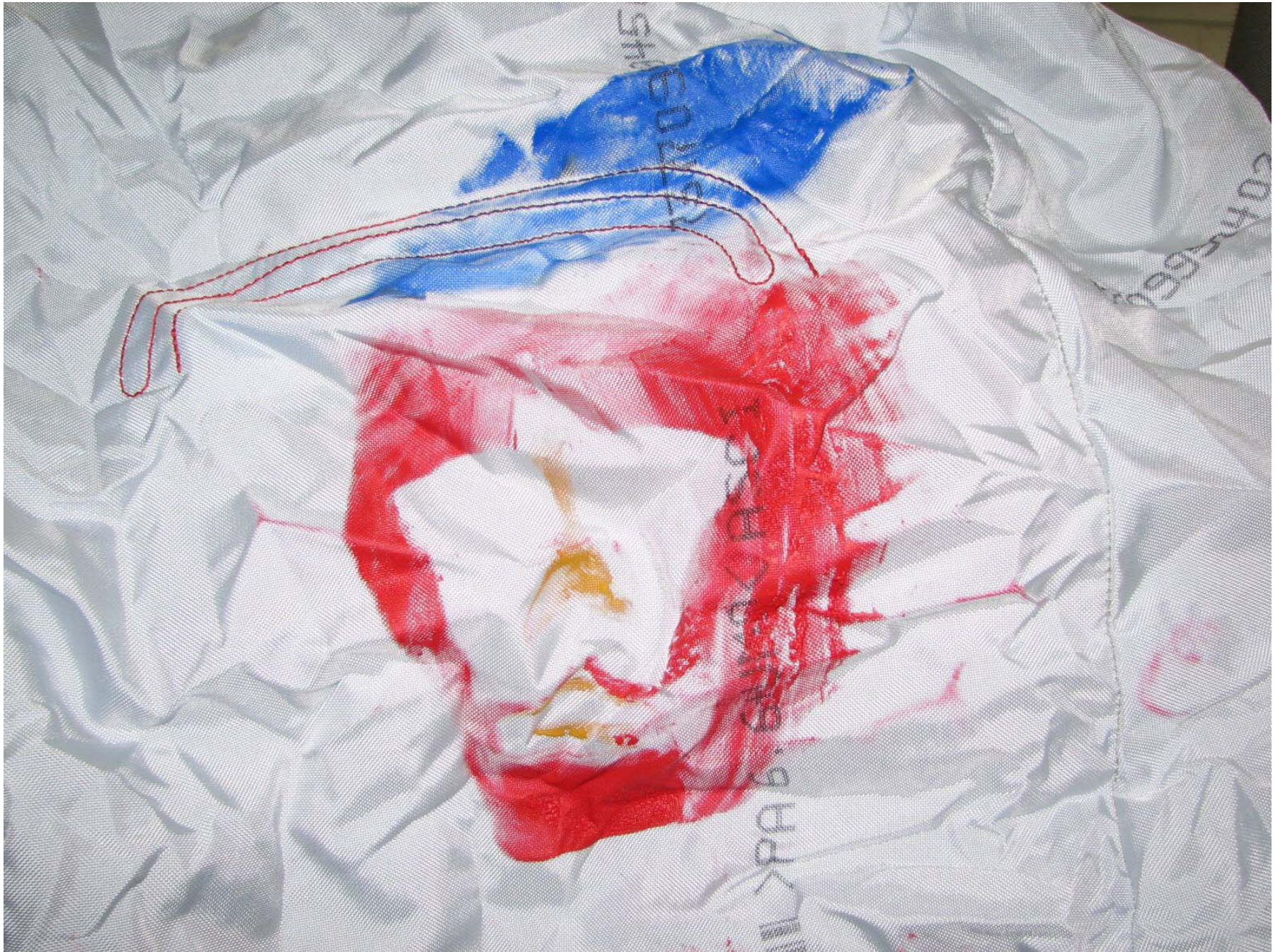
Figure A-57: Post-Test Passenger Dummy Airbag Contact
