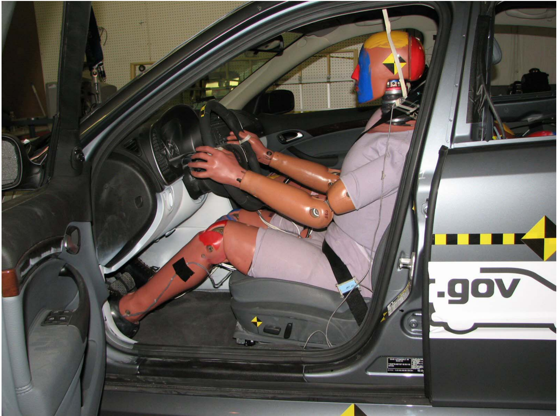
Figure A-34: Pre-Test Driver Dummy (Door Open)
