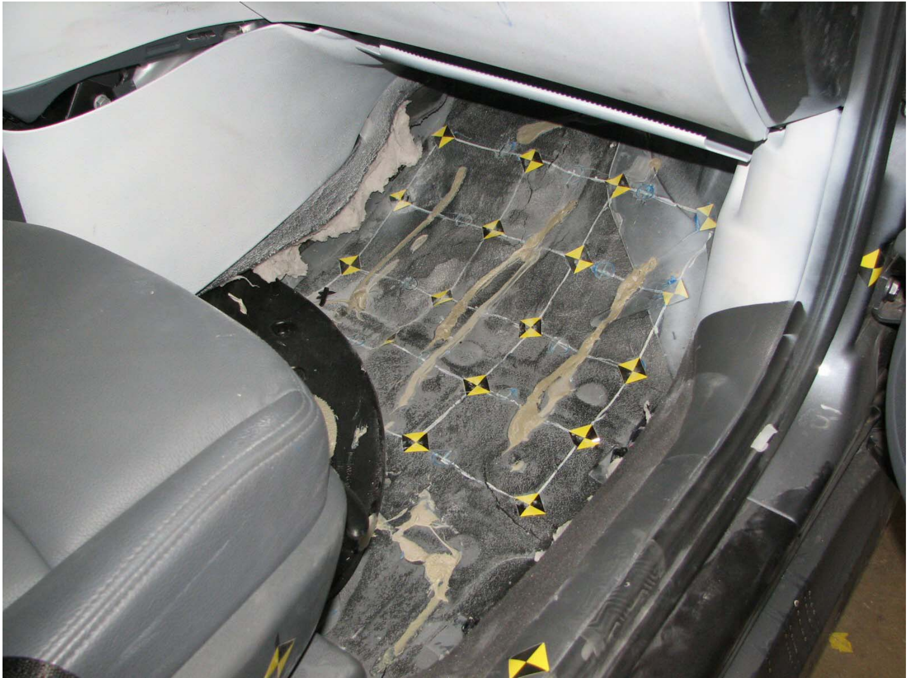
Figure A-55: Post-Test Passenger Side Floor Pan
