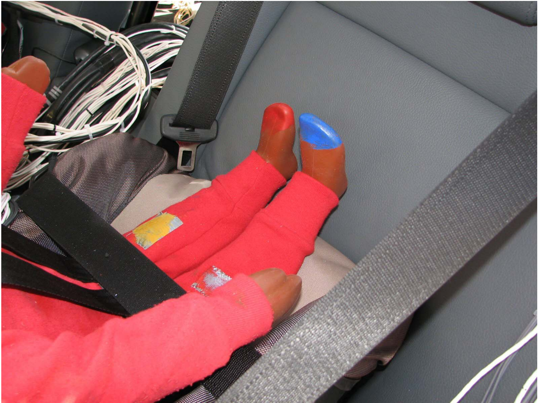
Figure D2-36: Post-Test Position 4 Dummy Legs
