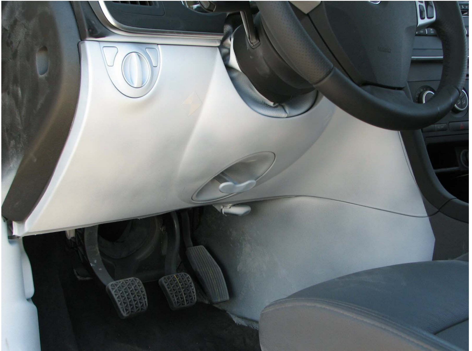
Figure A-38: Pre-Test Driver Side Knee Bolster
