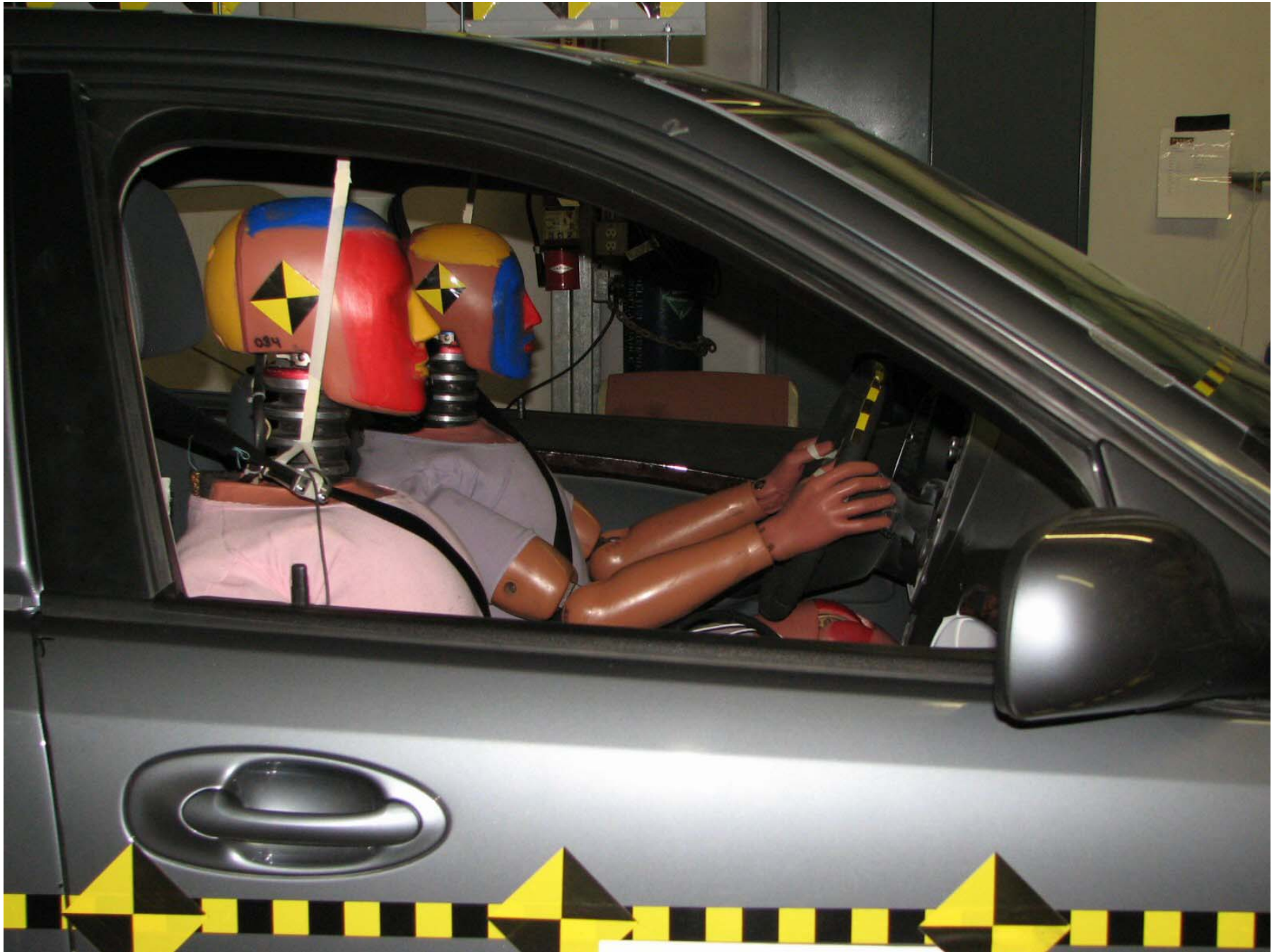
Figure A-46: Pre-Test Passenger Dummy (Through Window)
