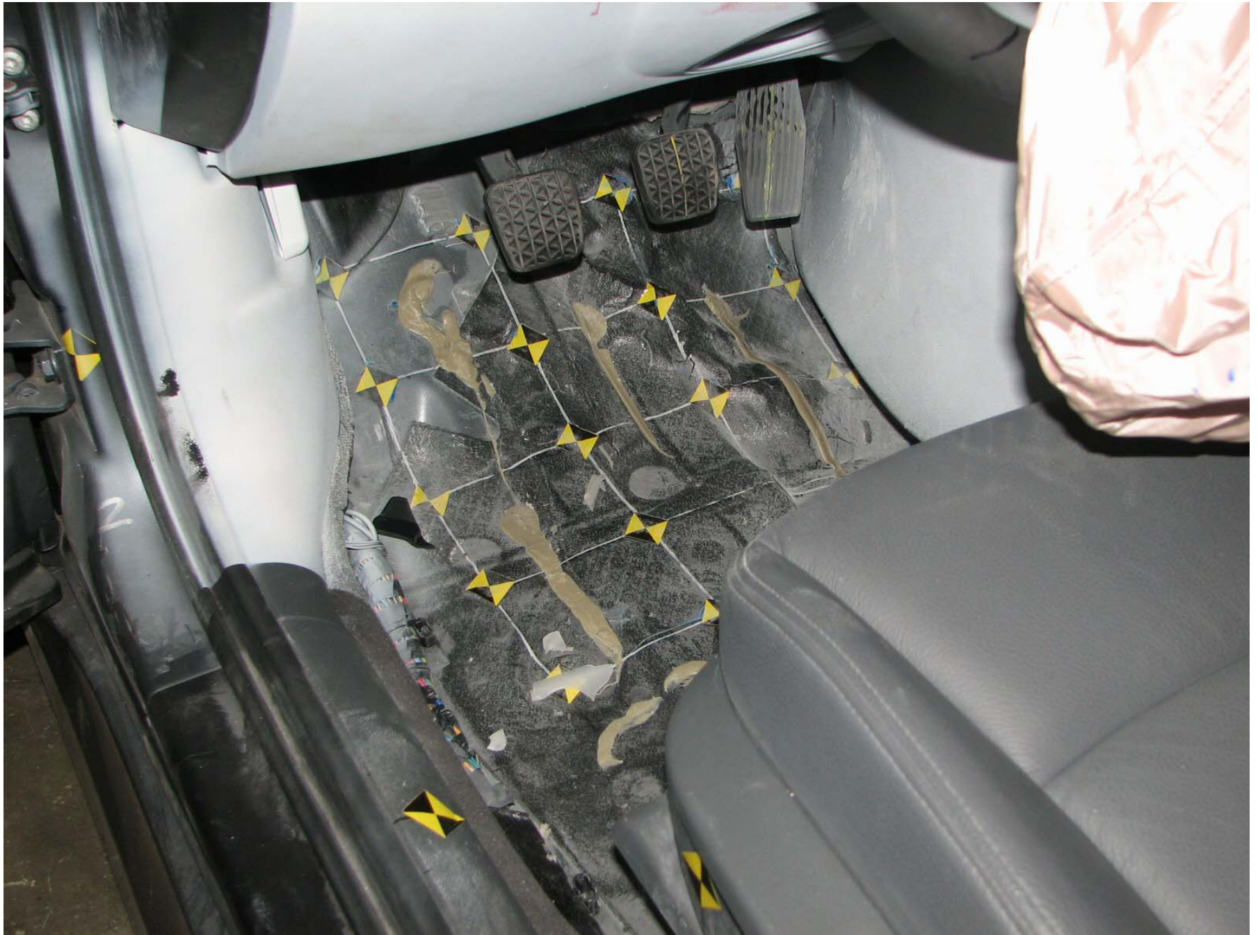
Figure A-41: Post-Test Driver Side Floor Pan
