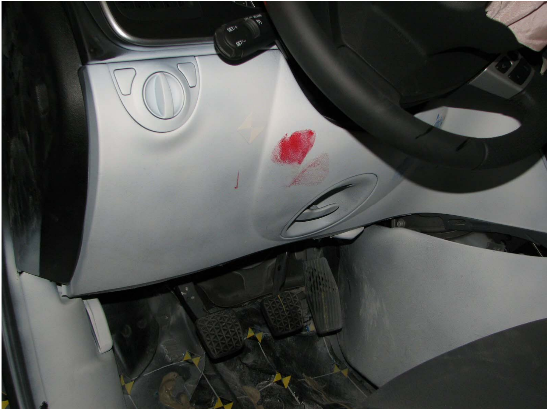
Figure A-39: Post-Test Driver Side Knee Bolster
