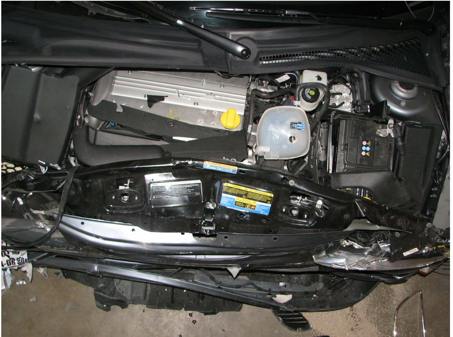
Figure A-21: Post-Test Engine Compartment (Vehicle Moved)
