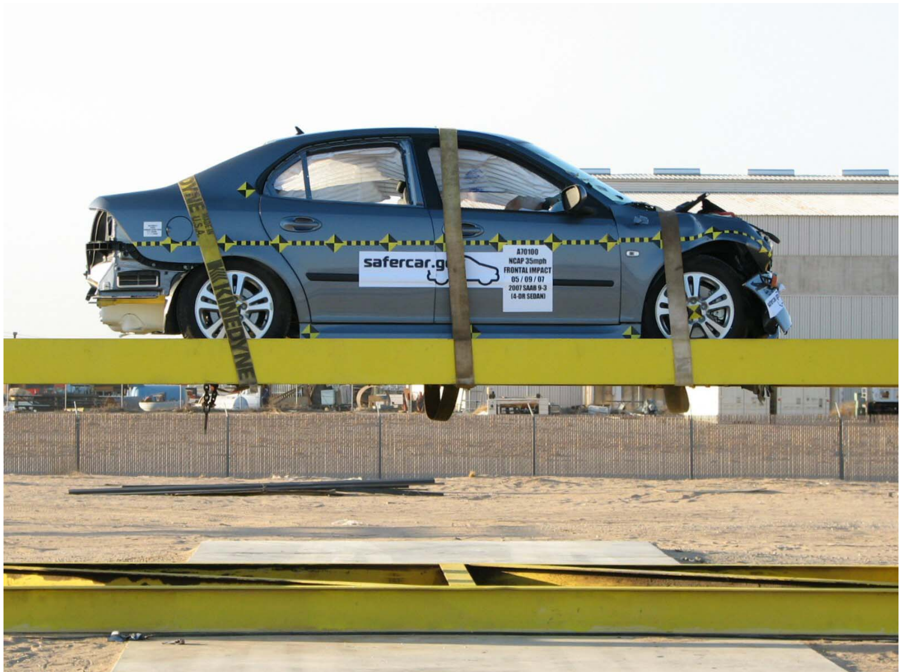
Figure A-58: Vehicle on Rollover Device (0°)
