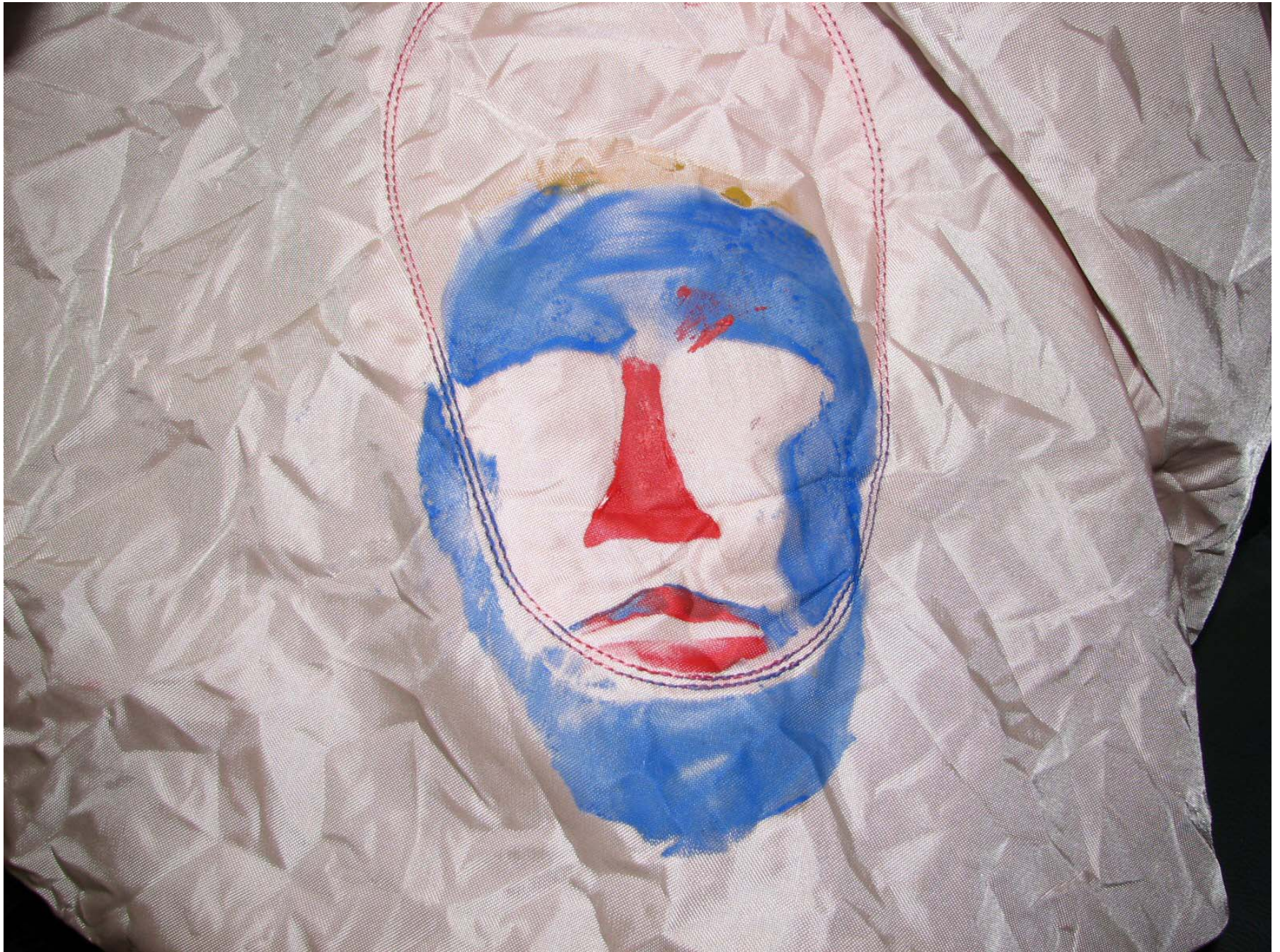
Figure A-43: Post-Test Driver Dummy Airbag Contact
