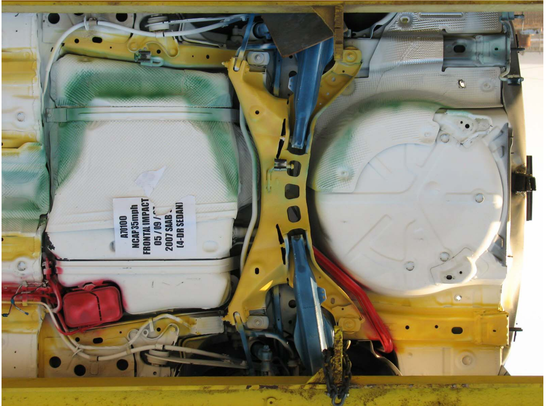
Figure A-29: Post-Test Rear Underbody
