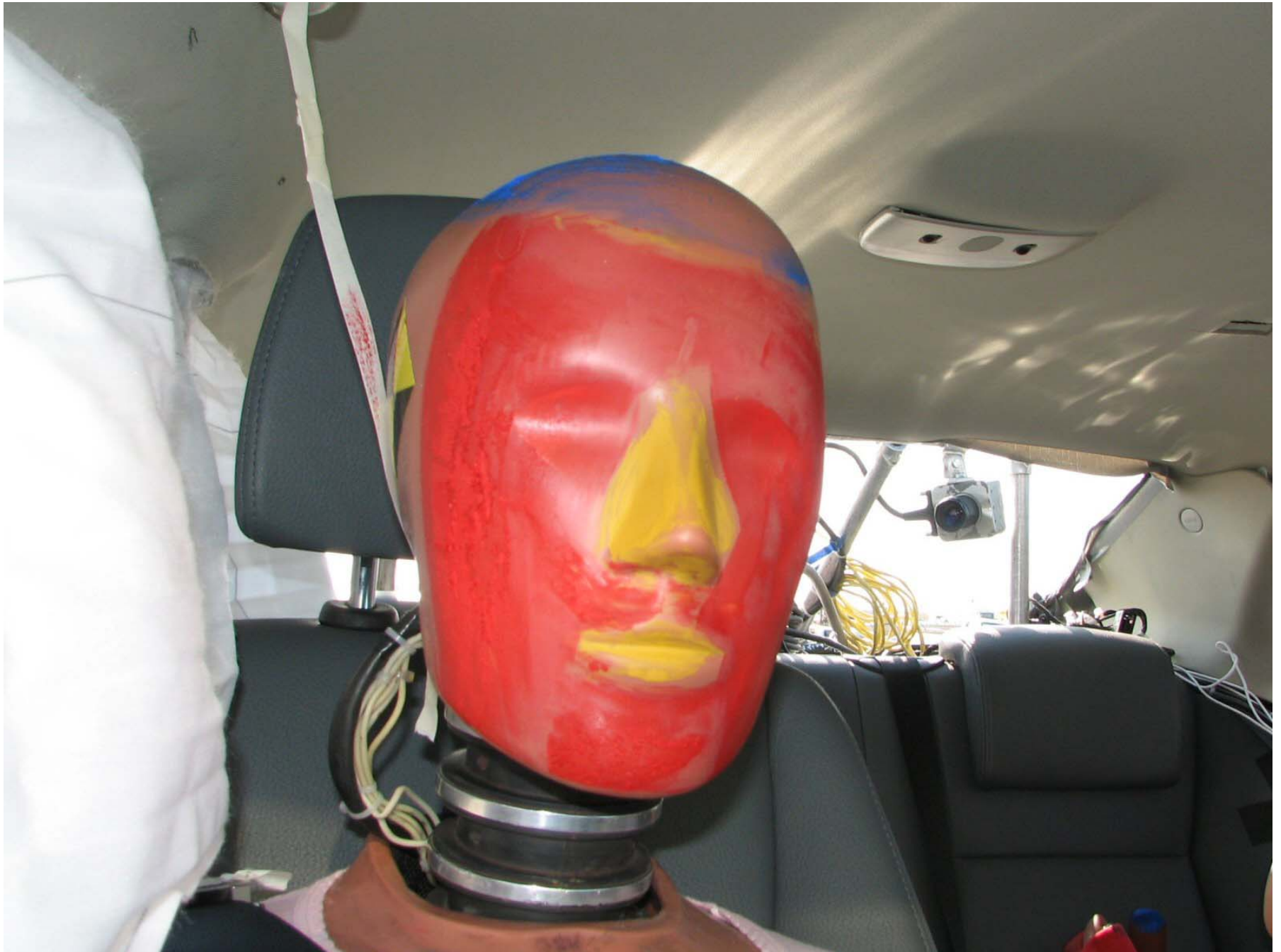
Figure A-56: Post-Test Passenger Dummy Head
