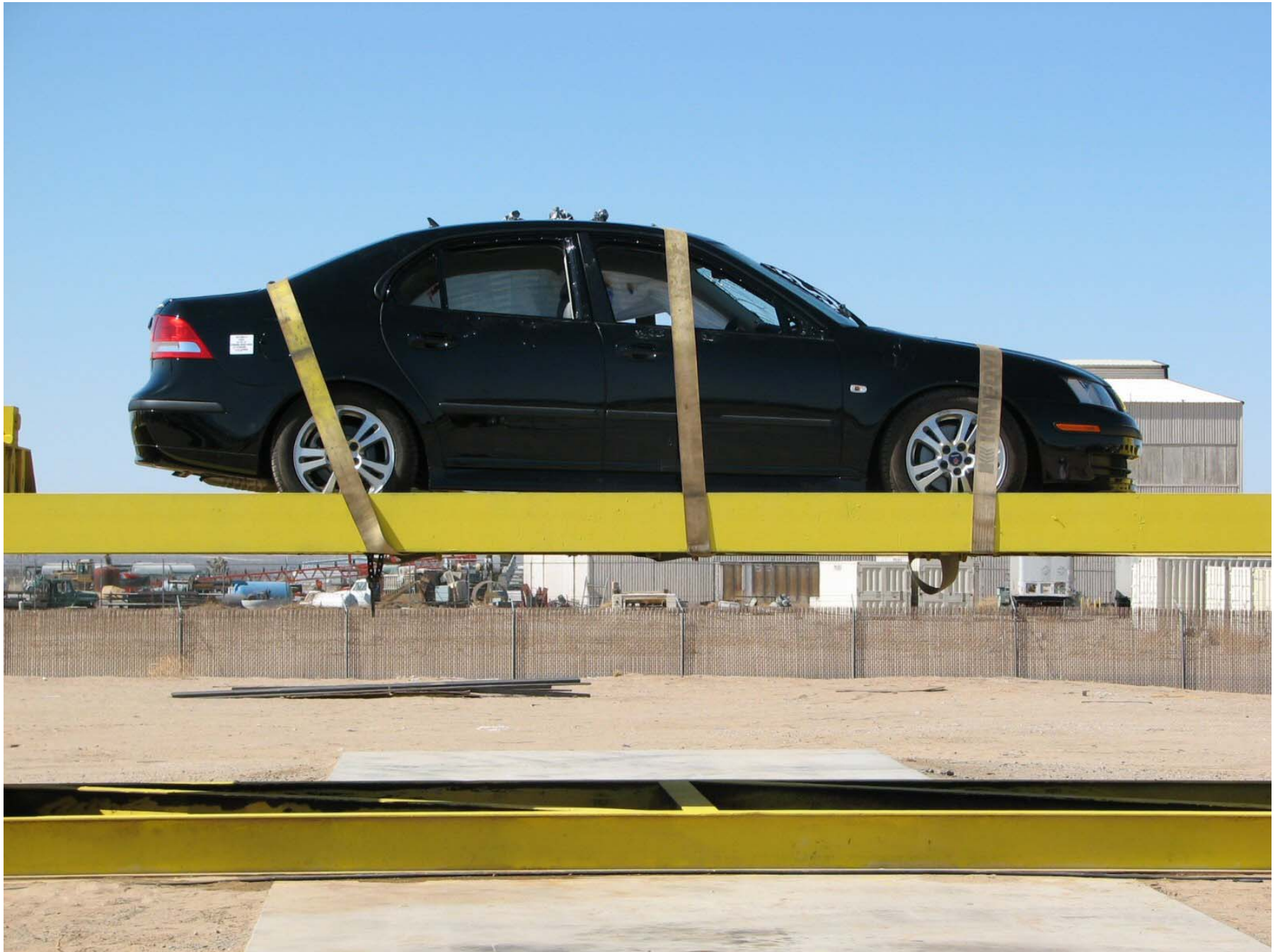
Figure A-61: Vehicle on Rollover Device (0°)
