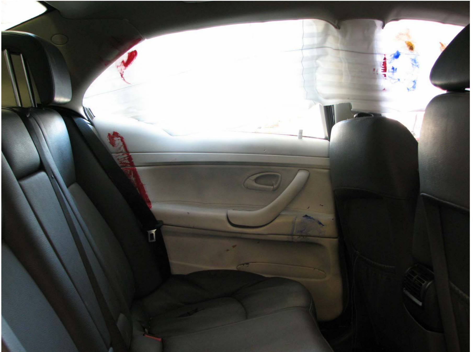
Figure A-52: Post-Test Rear Door Panel (Interior)
