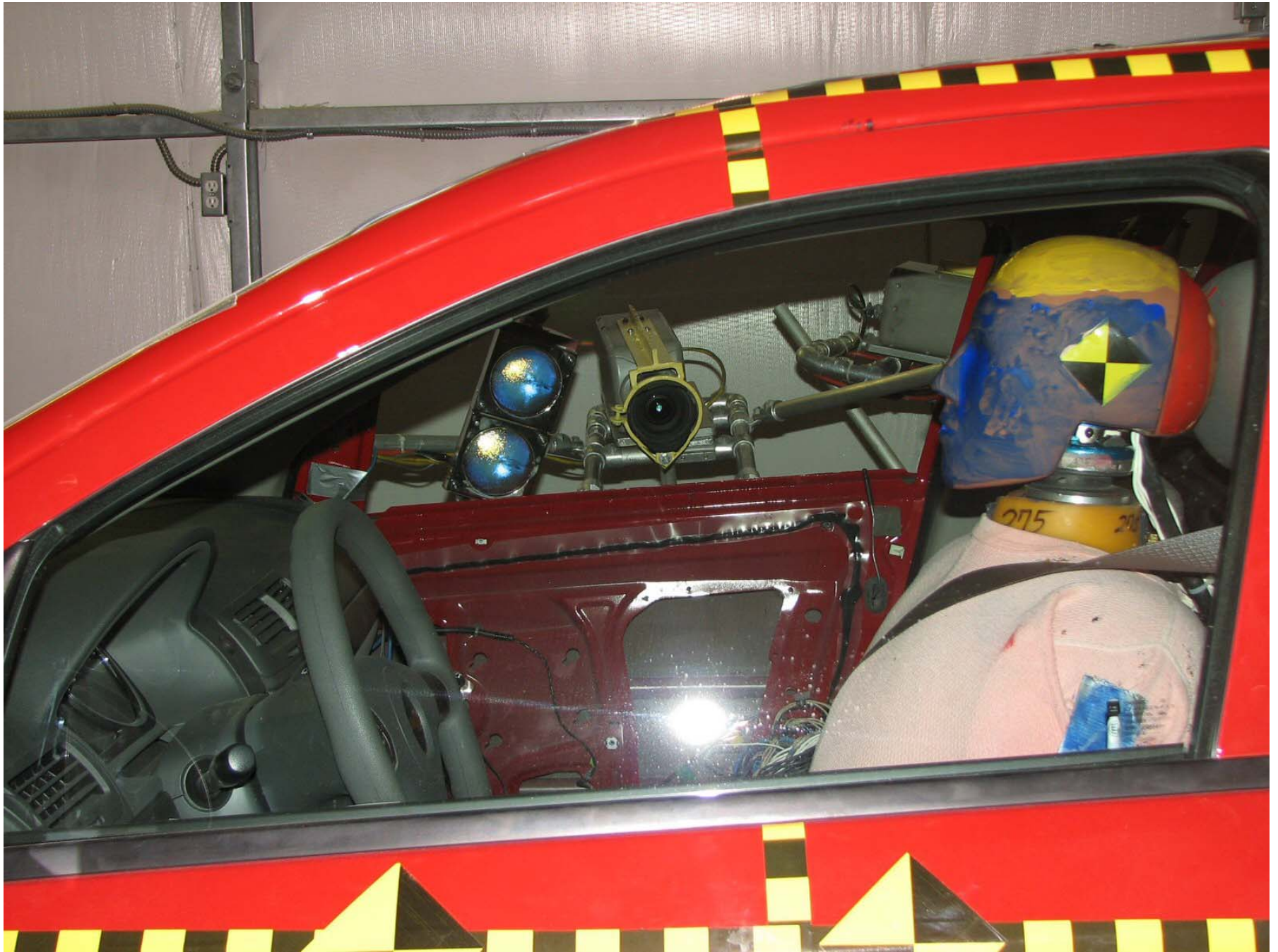
Figure A-36: Pre-Test Driver Dummy (Through Window)
