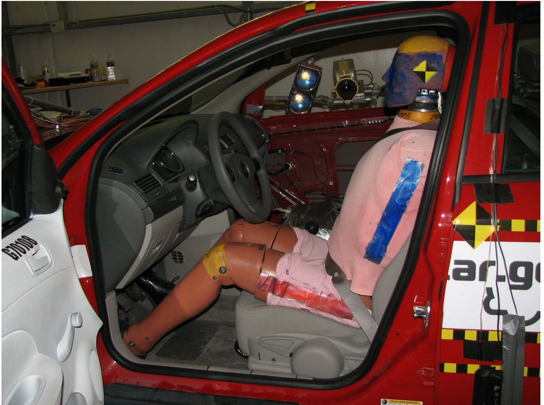
Figure A-35: Pre-Test Driver Dummy (Door Open)
