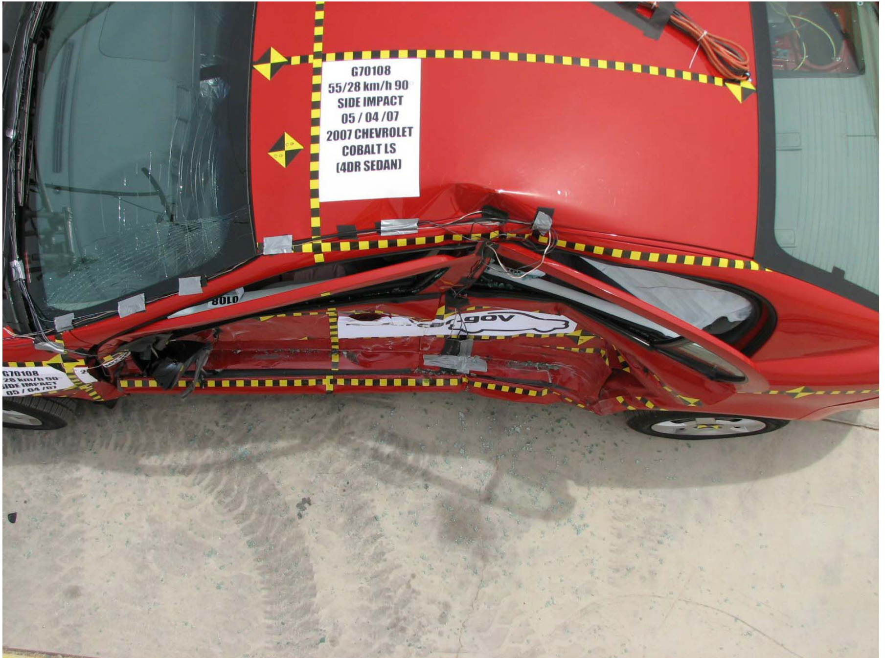
Figure A-24: Post-Test Overhead Close-up View
