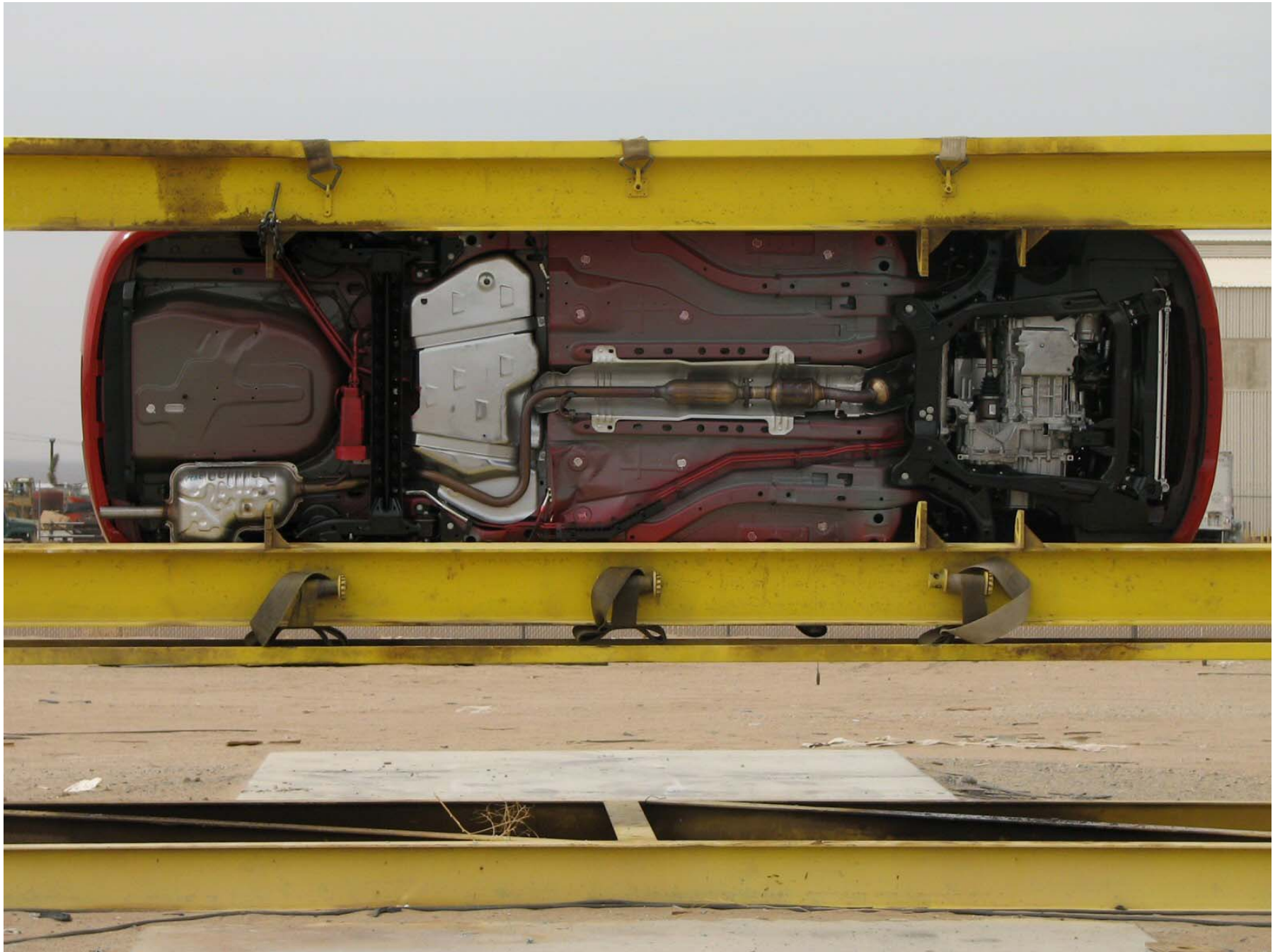
Figure A-64: Vehicle on Rollover Device (270°)
