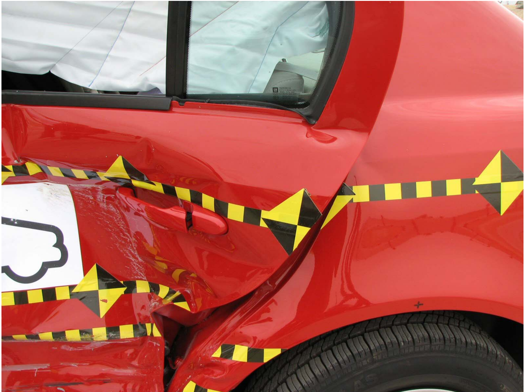
Figure A-34: Post-Test Left Rear Door
