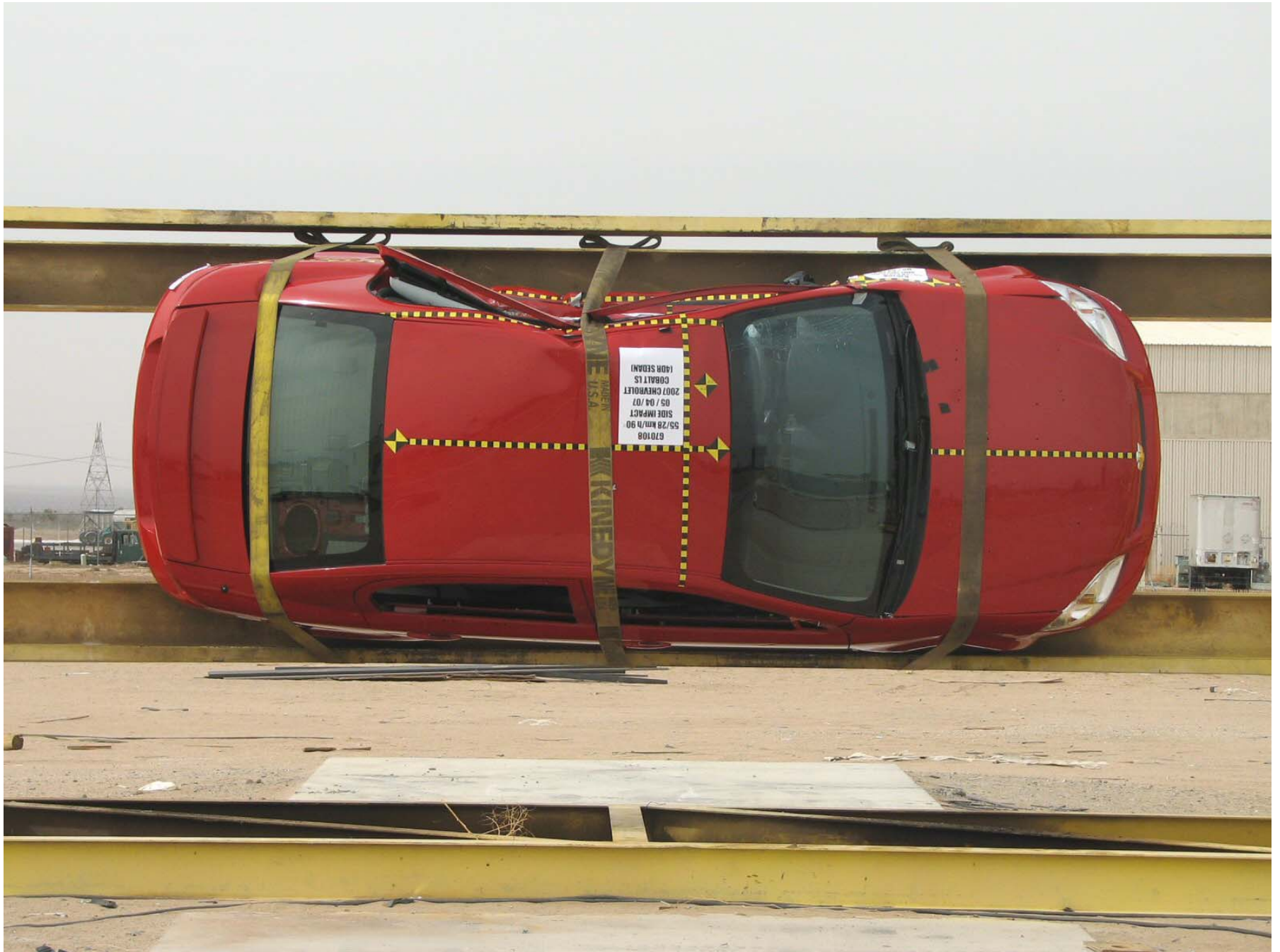
Figure A-62: Vehicle on Rollover Device (90°)
