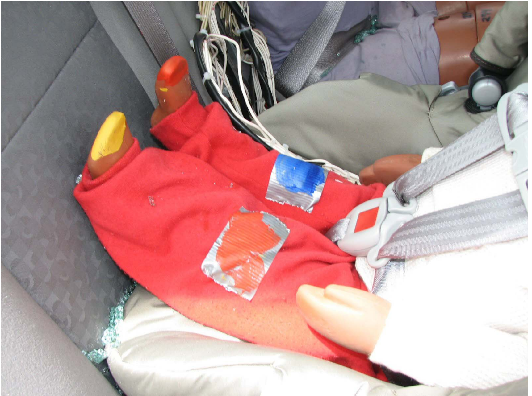
Figure D2-18: Post-Test Position 3 Dummy Legs
