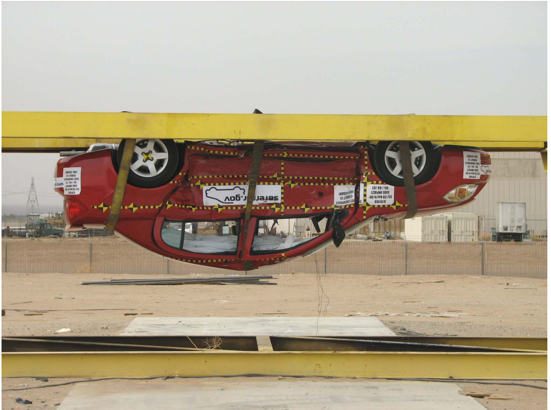
Figure A-63: Vehicle on Rollover Device (180°)
