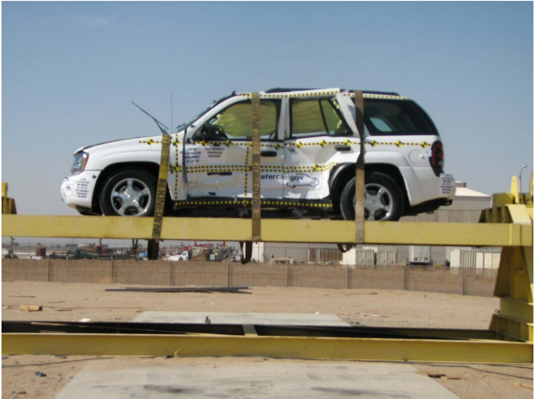
Figure A-61: Vehicle on Rollover Device (0°)
