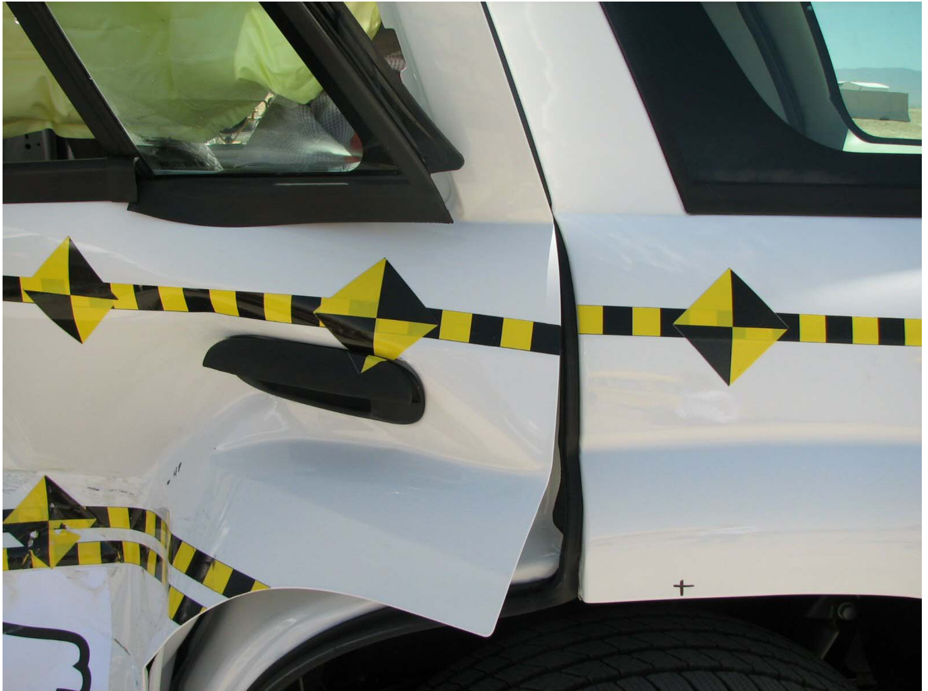
Figure A-34: Post-Test Left Rear Door
