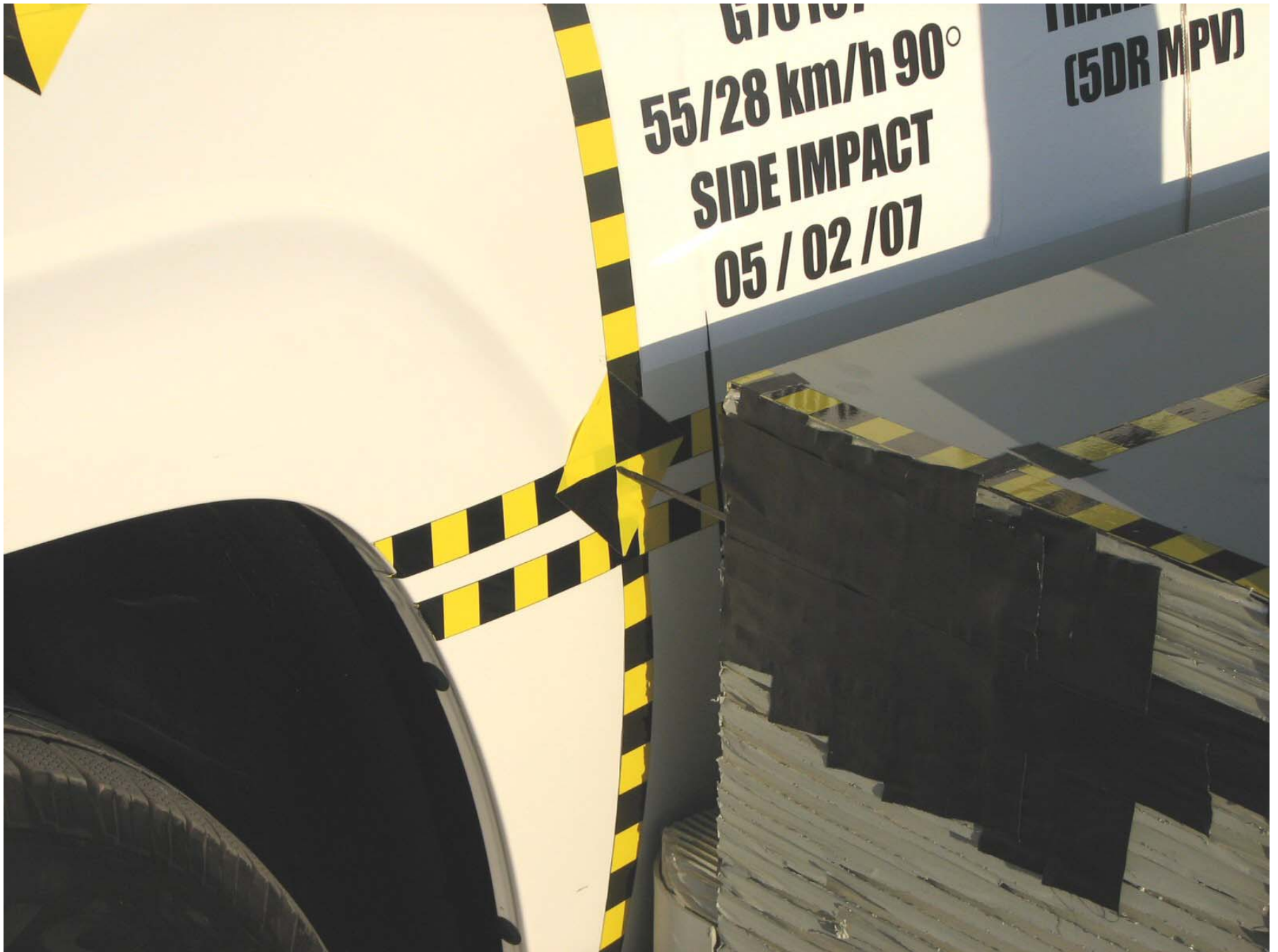
Figure A-25: Pre-Test Left Impact Point
