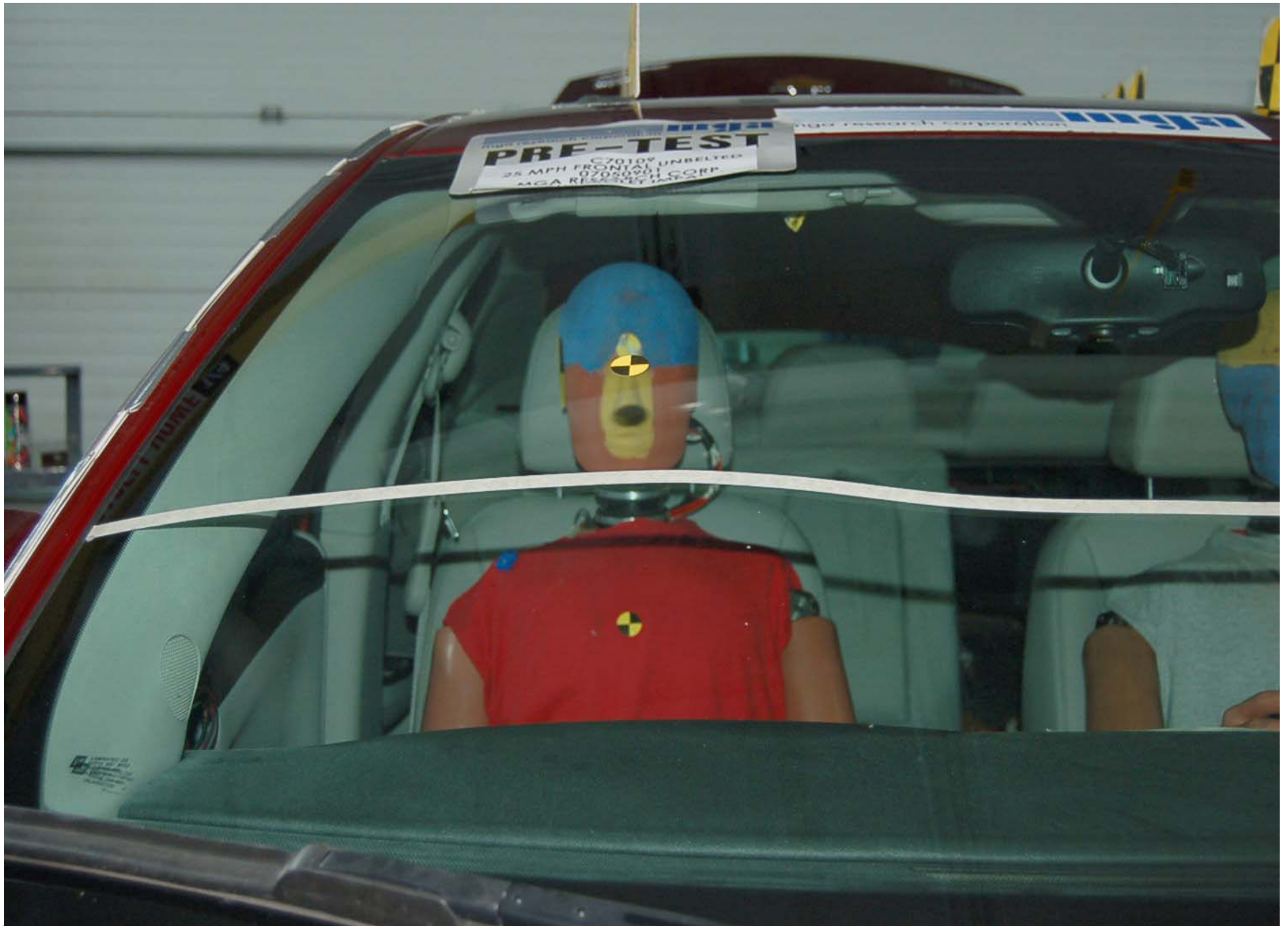
Pre-Test Passenger Dummy Front View (head position)
