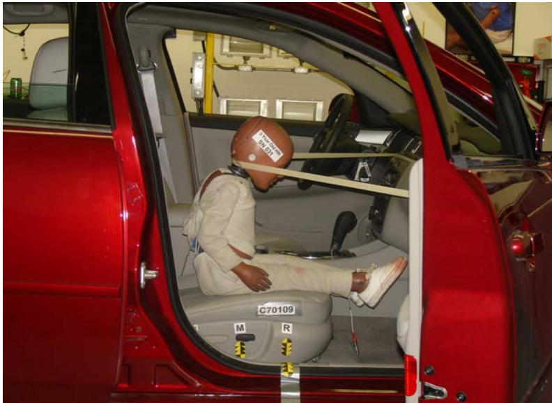
3-Year-Old Unbelted, Rearward Seat Track, Position 3
