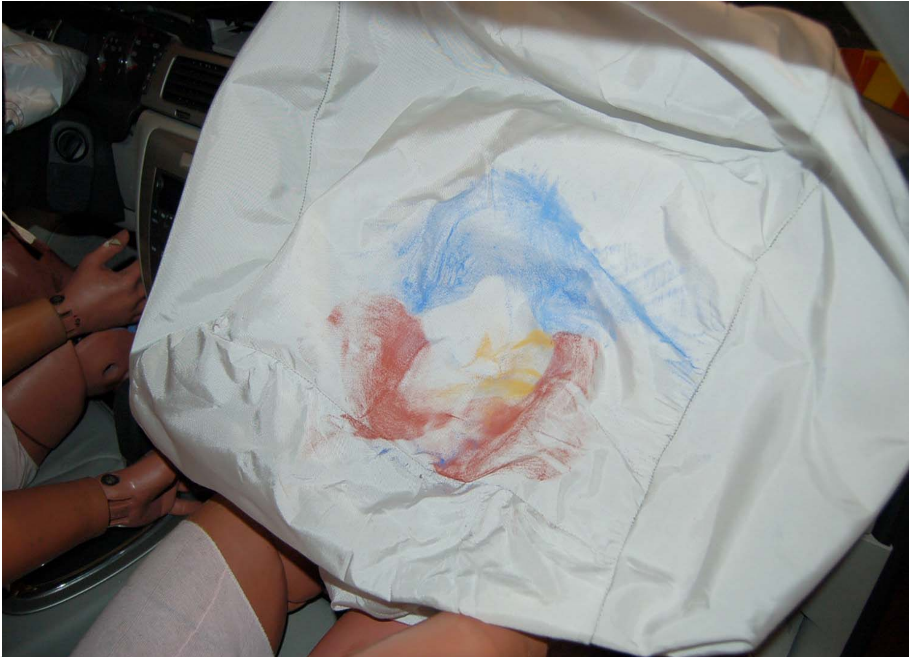
Post-Test Passenger Dummy Airbag Contact
