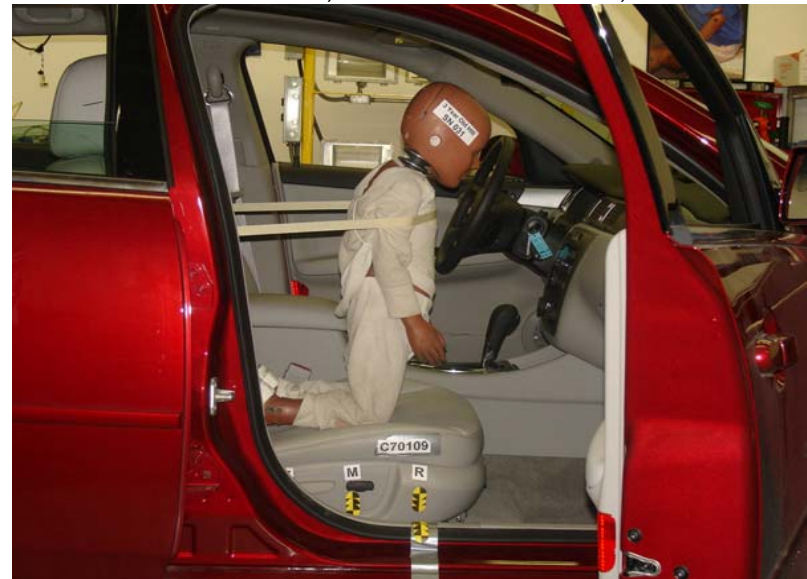
3-Year-Old Unbelted, Rearward Seat Track, Position 6
