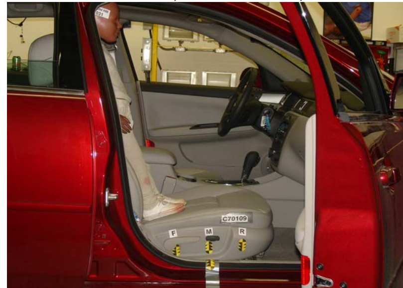
3-Year-Old Unbelted, Middle Seat Track, Position 5
