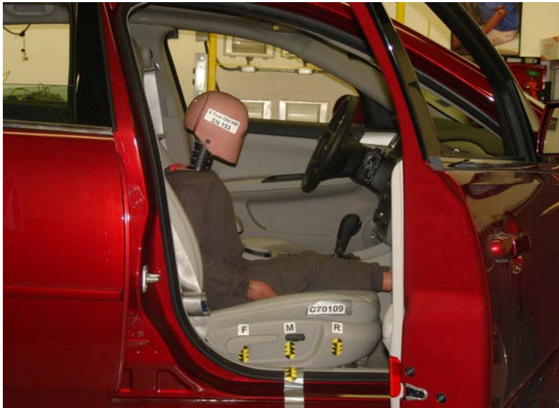
6-Year-Old Unbelted, Middle Seat Track, Position 1
