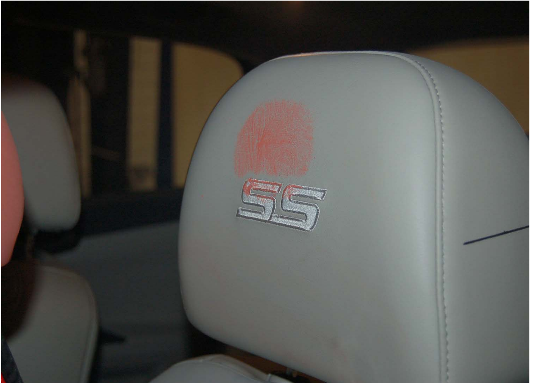
Post-Test Driver Dummy Head Contact (headrest)
