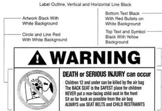
Figure 6a. Sun Visor Label Visible When Visor is in Down Position.
