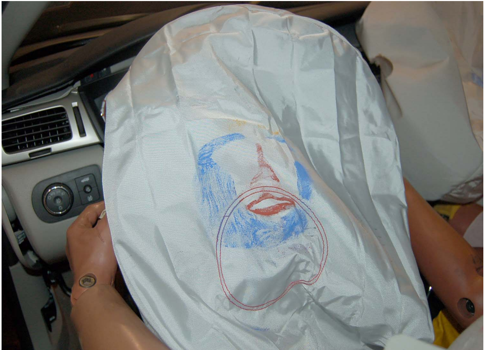
Post-Test Driver Dummy Airbag Contact
