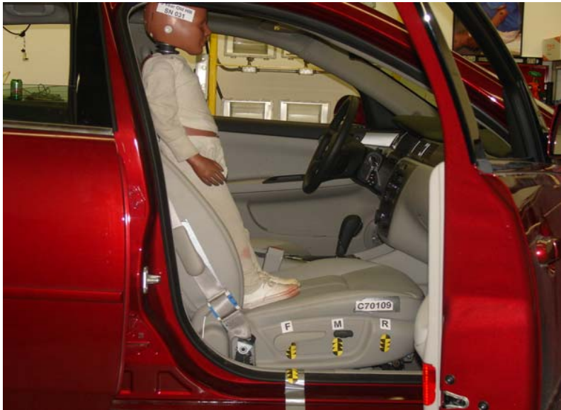
3-Year-Old Unbelted, Forward Seat Track, Position 5
