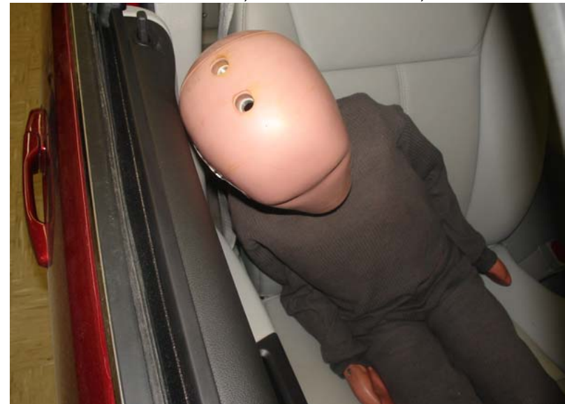
6-Year-Old Unbelted, Middle Seat Track, Position 4
