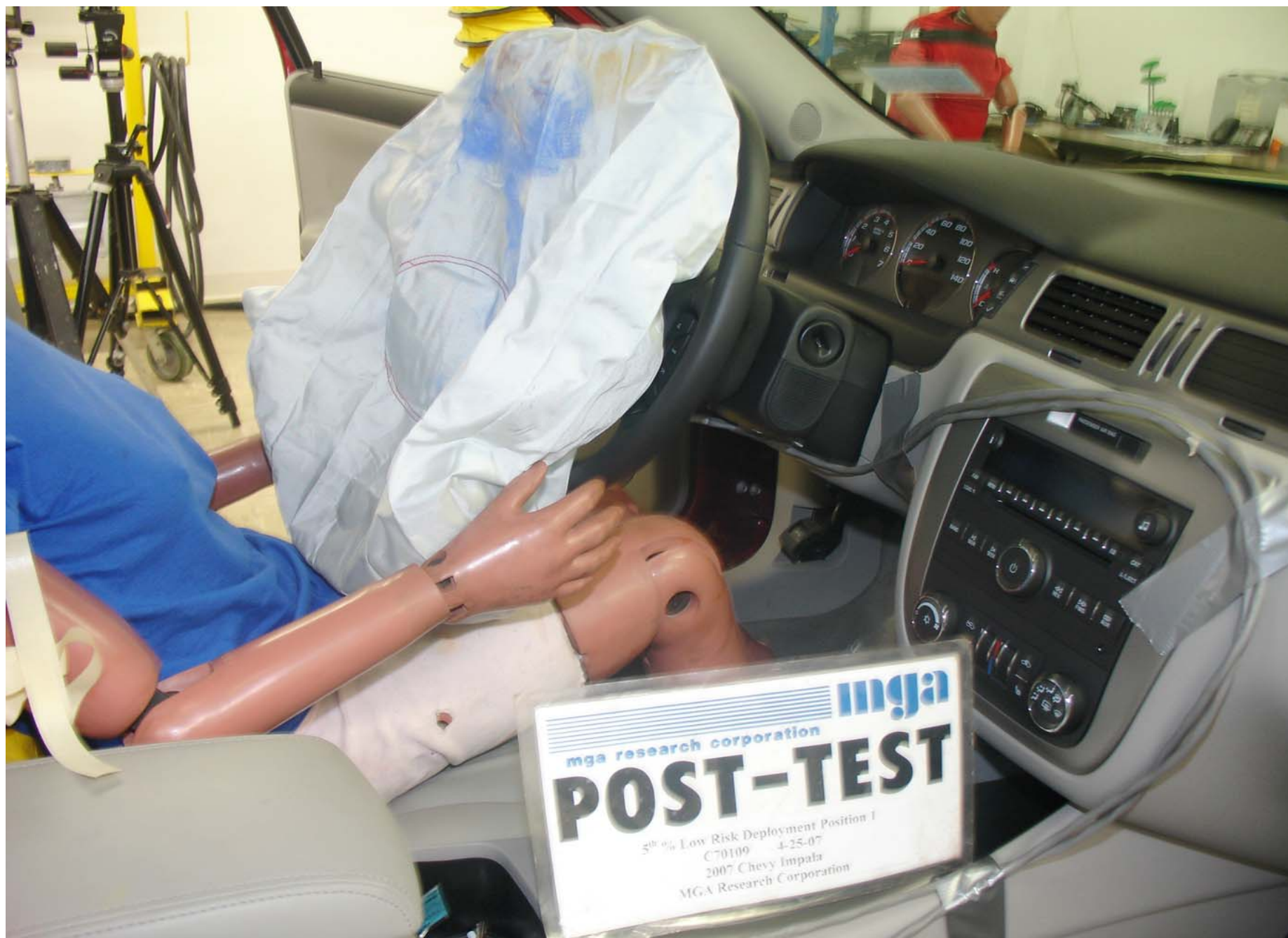
Post-Test 5th Fem. P1 Driver Dummy Airbag Contact Right Side View
