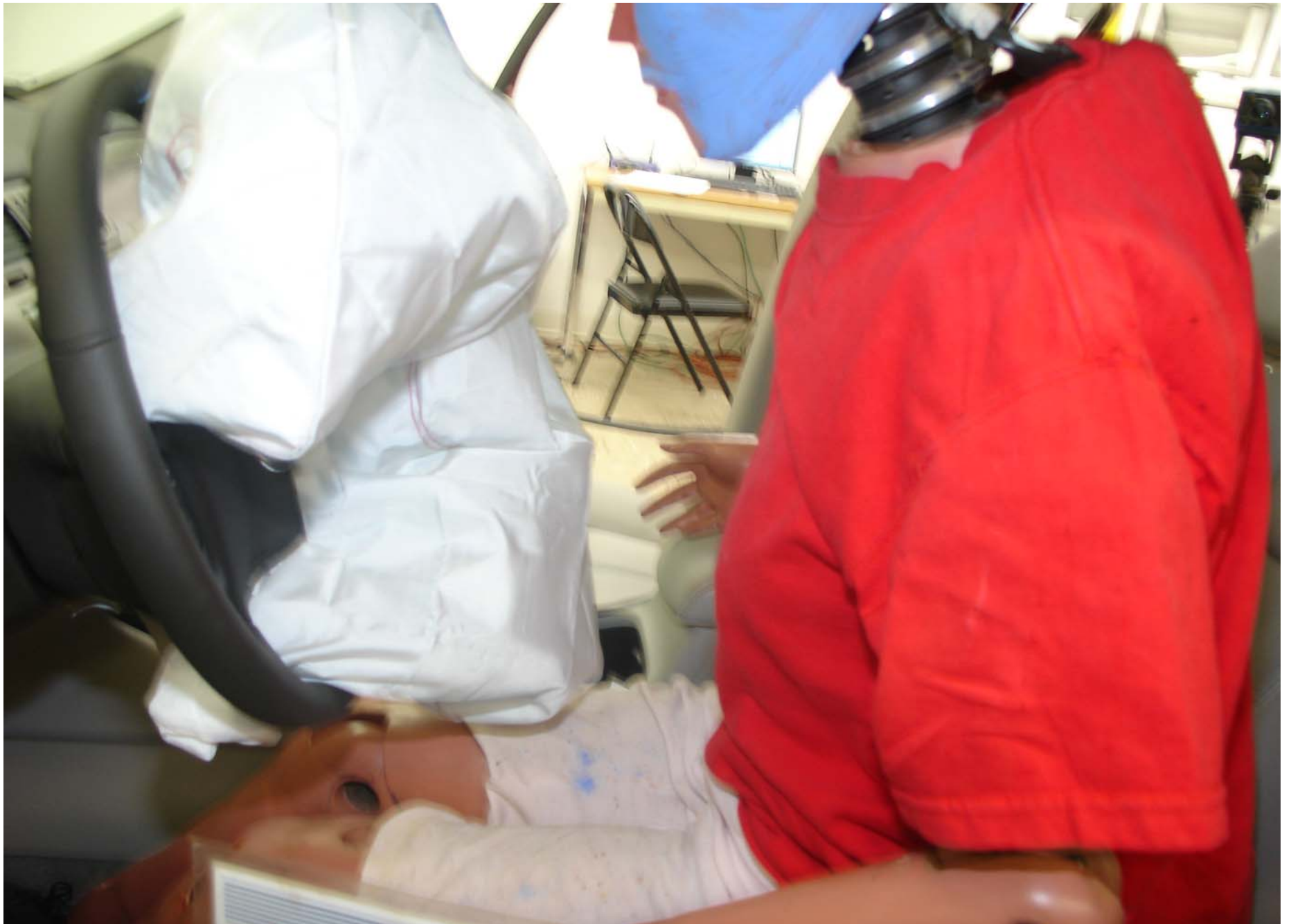
Post-Test 5th Fem. P2 Driver Dummy Airbag Contact Left Side View
