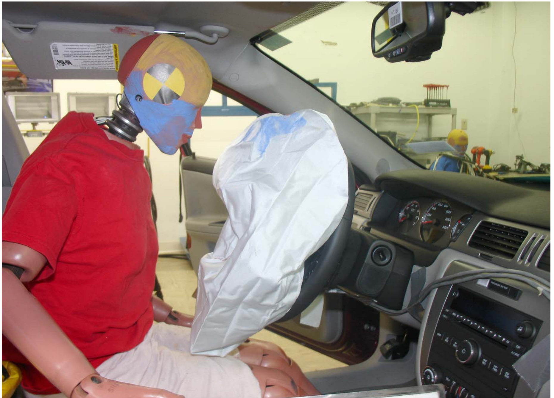
Post-Test 5th Fem. P2 Driver Dummy Airbag Contact Right Side View
