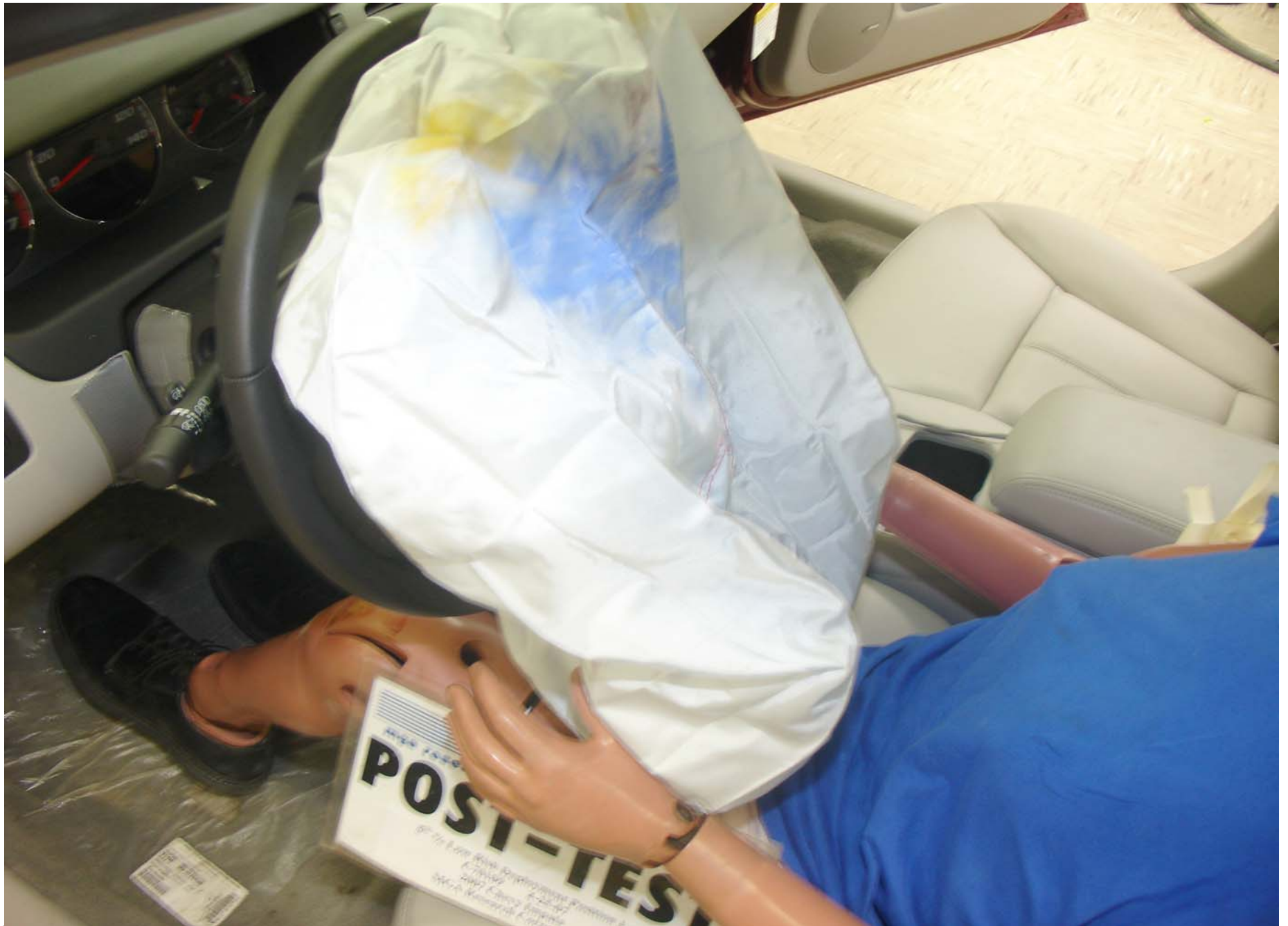
Post-Test 5th Fem. P1 Driver Dummy Airbag Contact Left Side View
