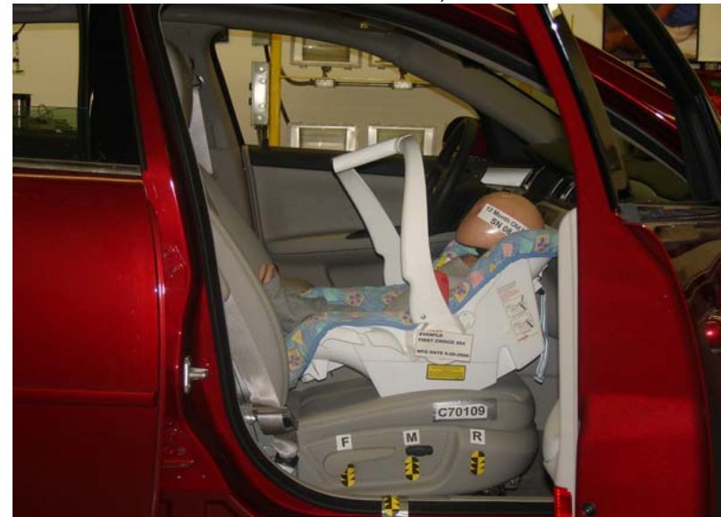
Evenflo First Choice 204 Unbelted, Forward Seat Track
