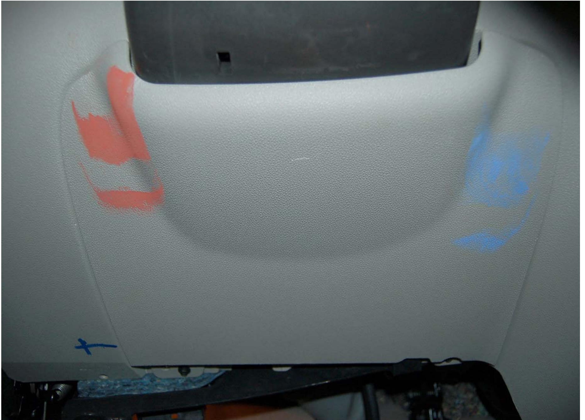
Post-Test Driver Dummy Knee Contact
