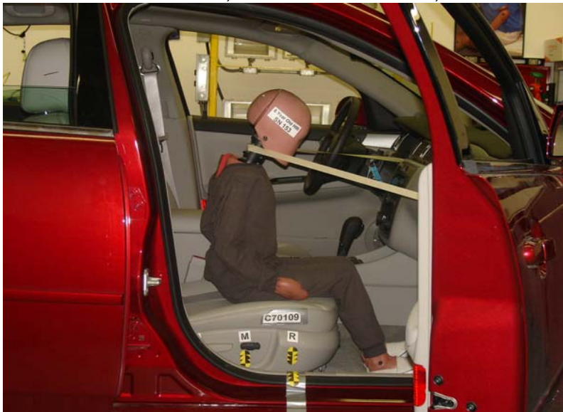
6-Year-Old Unbelted, Rearward Seat Track, Position 3
