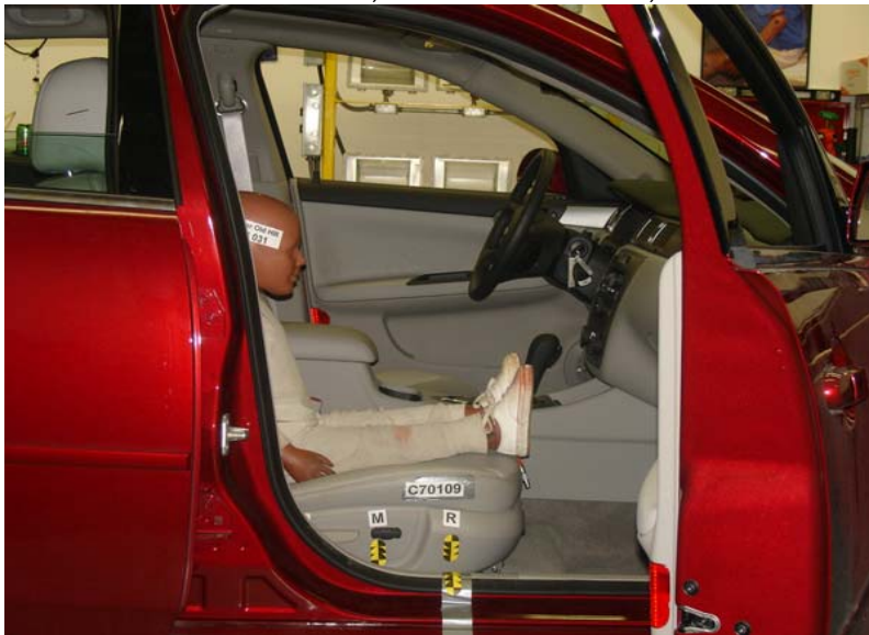
3-Year-Old Unbelted, Rearward Seat Track, Position 1
