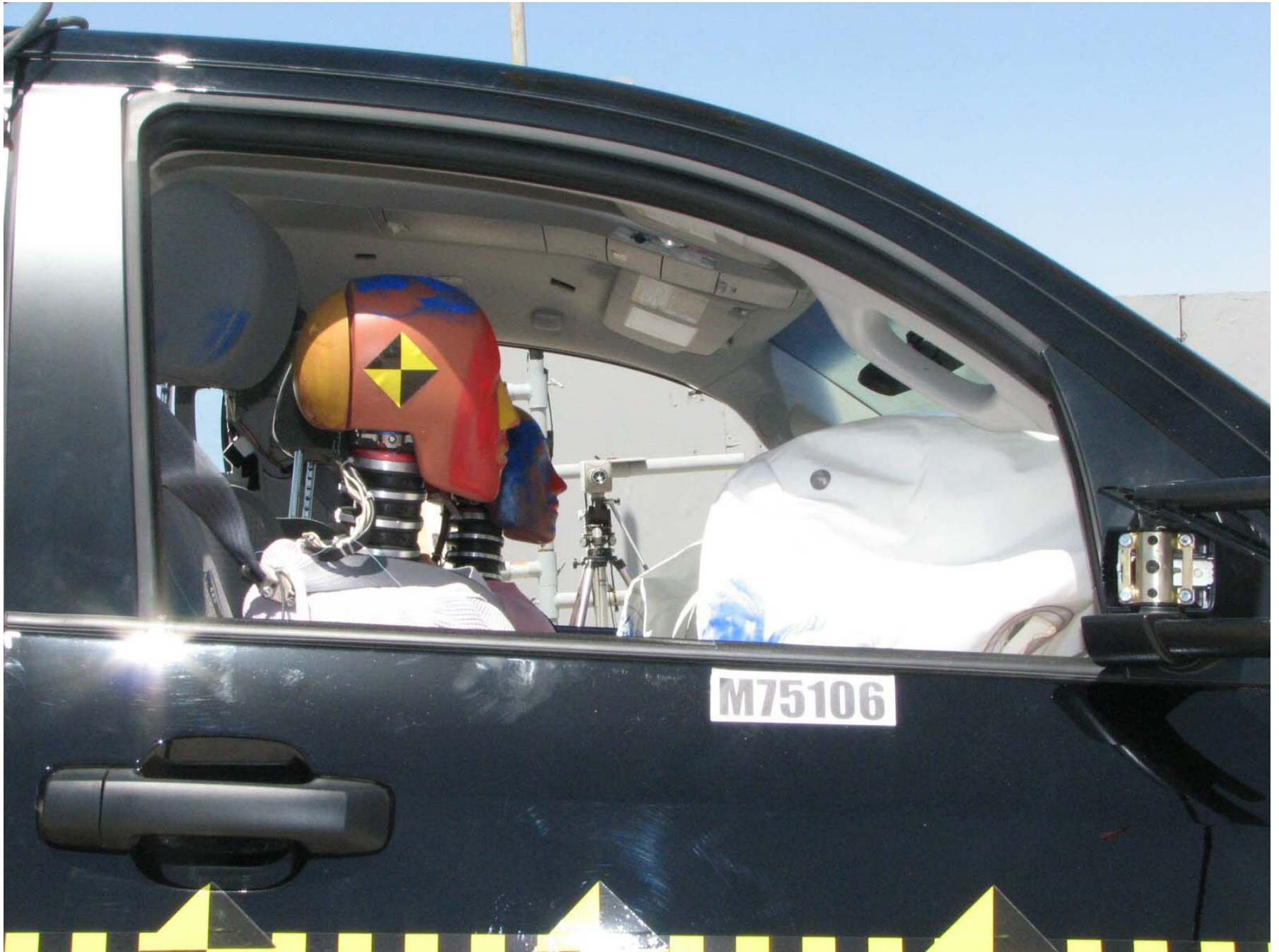
Figure A-47: Post-Test Passenger Dummy (Through Window)
