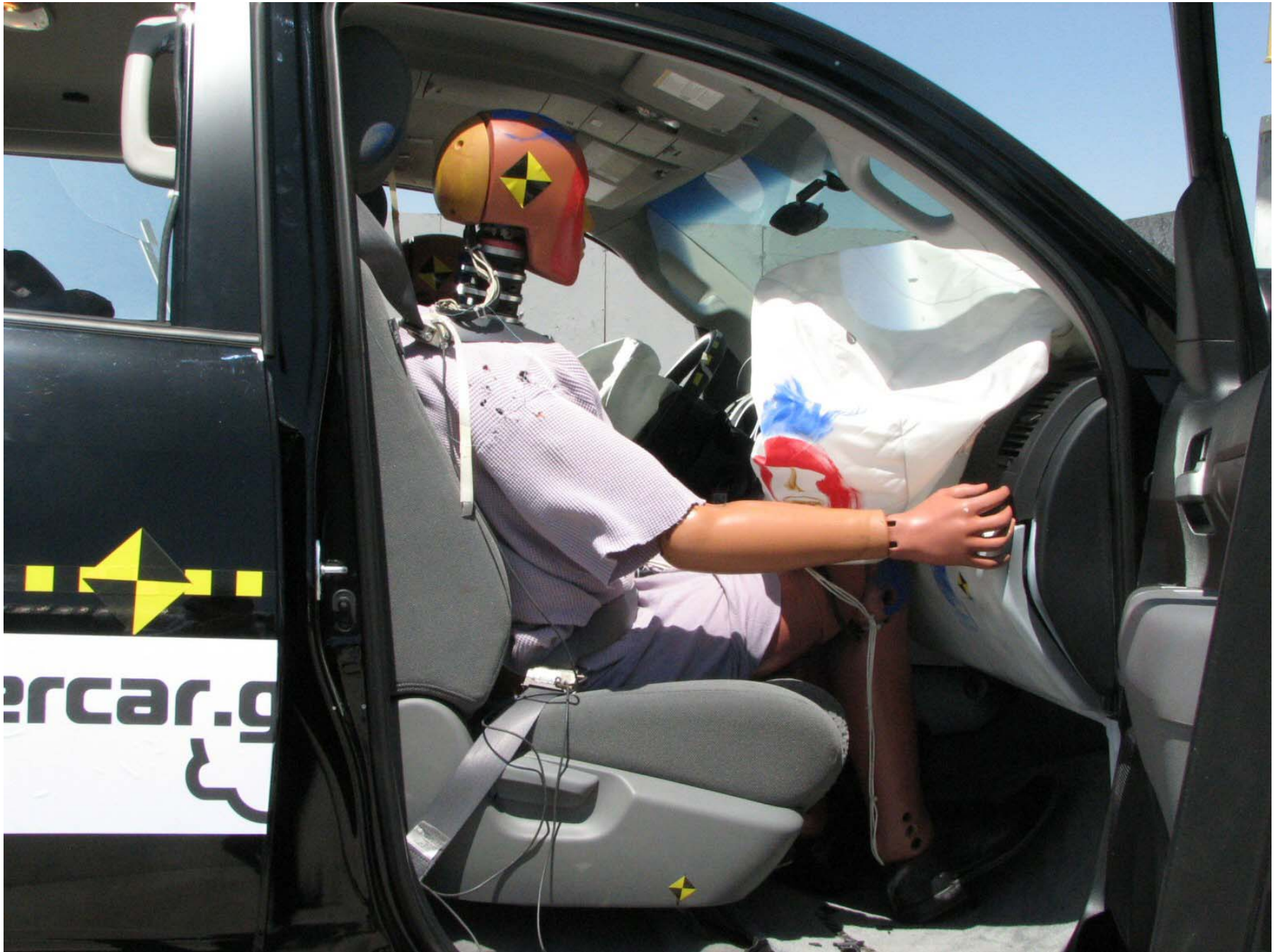
Figure A-49: Post-Test Passenger Dummy (Door Open)
