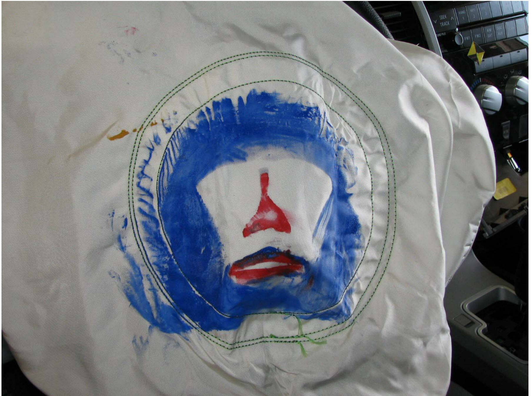
Figure A-43: Post-Test Driver Dummy Airbag Contact
