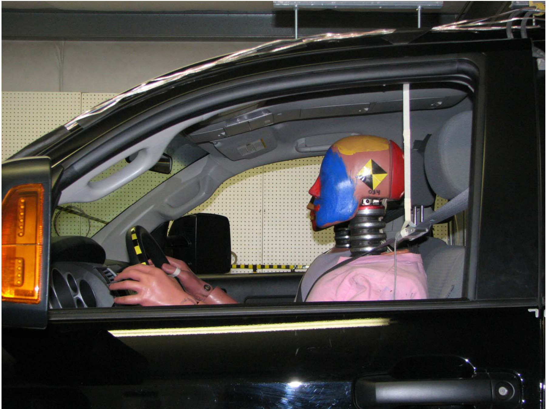
Figure A-32: Pre-Test Driver Dummy (Through Window)
