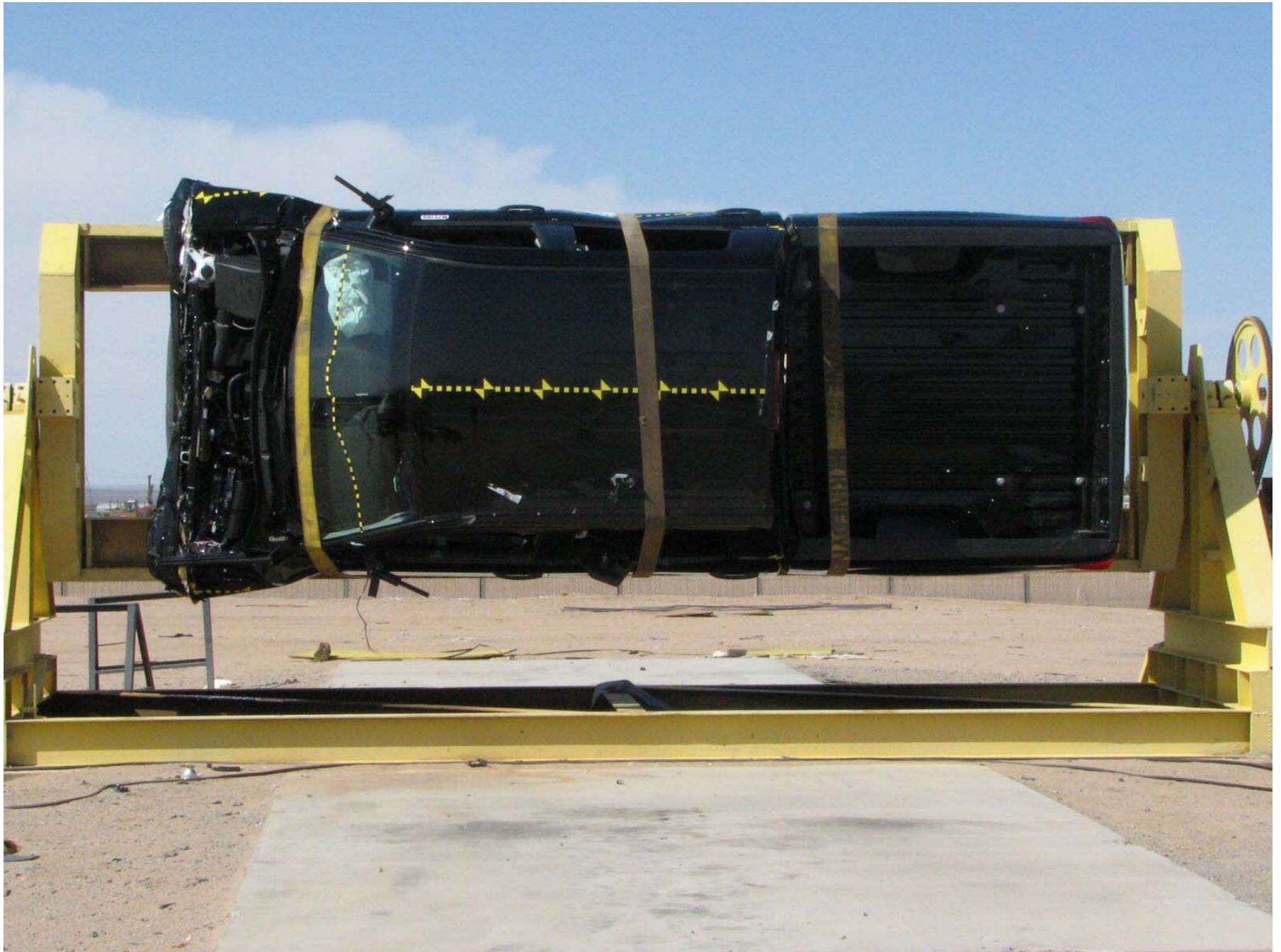
Figure A-59: Vehicle on Rollover Device (90°)
