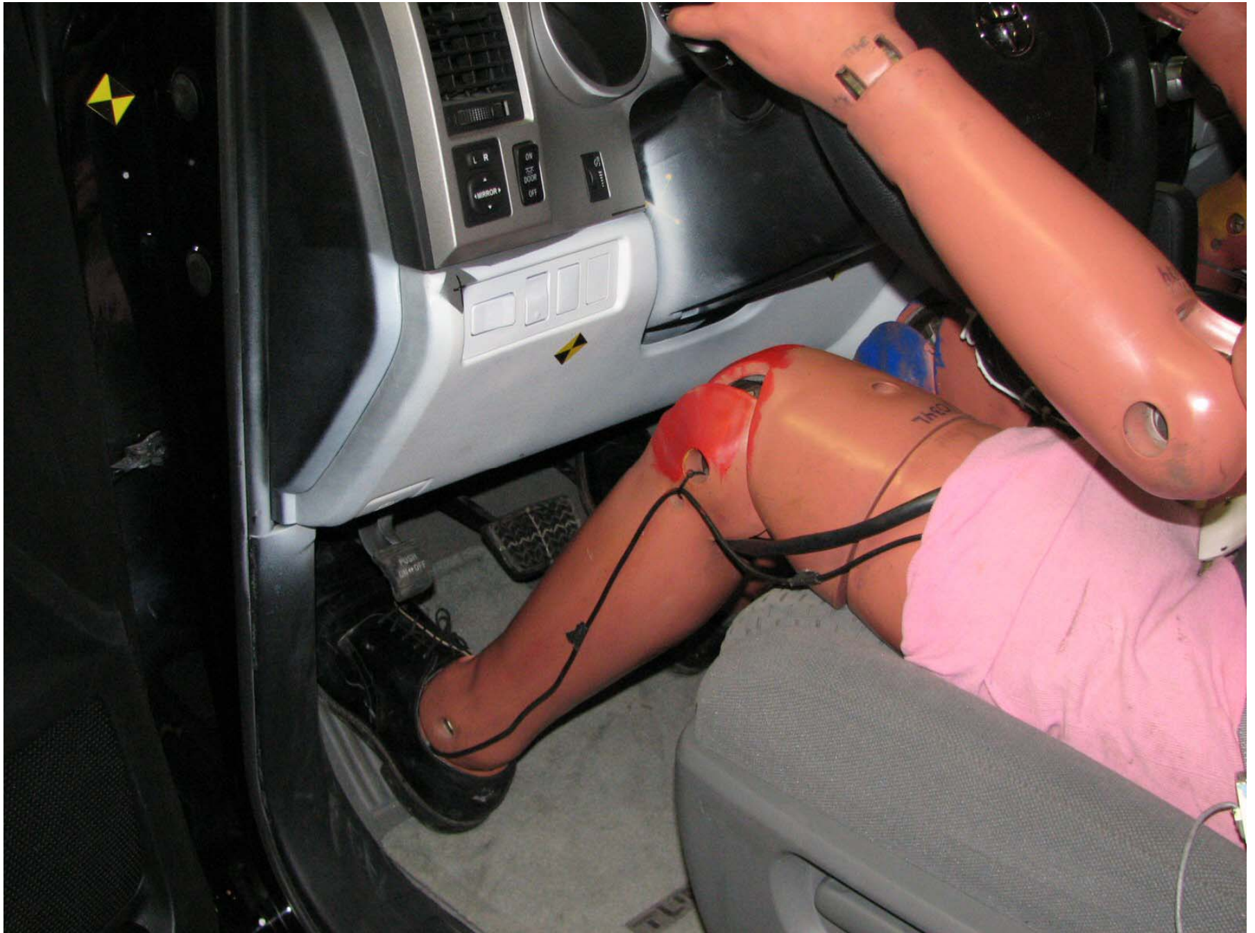
Figure A-36: Pre-Test Driver Dummy Feet
