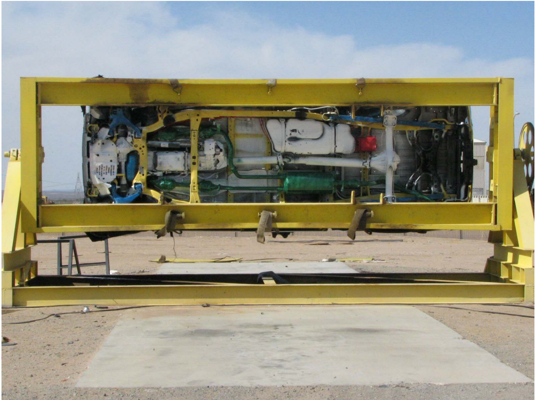
Figure A-61: Vehicle on Rollover Device (270°)
