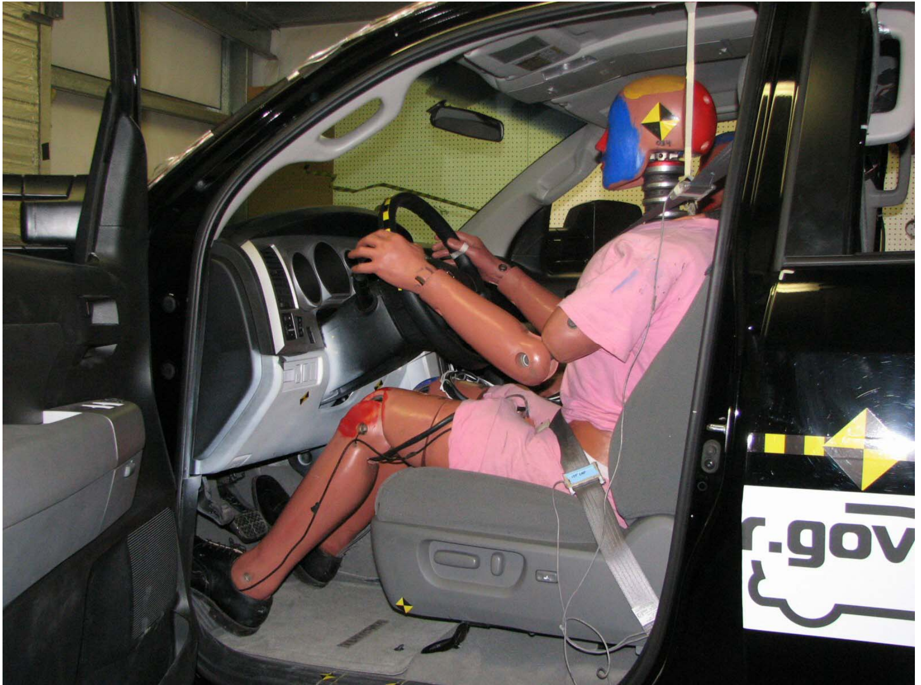
Figure A-34: Pre-Test Driver Dummy (Door Open)
