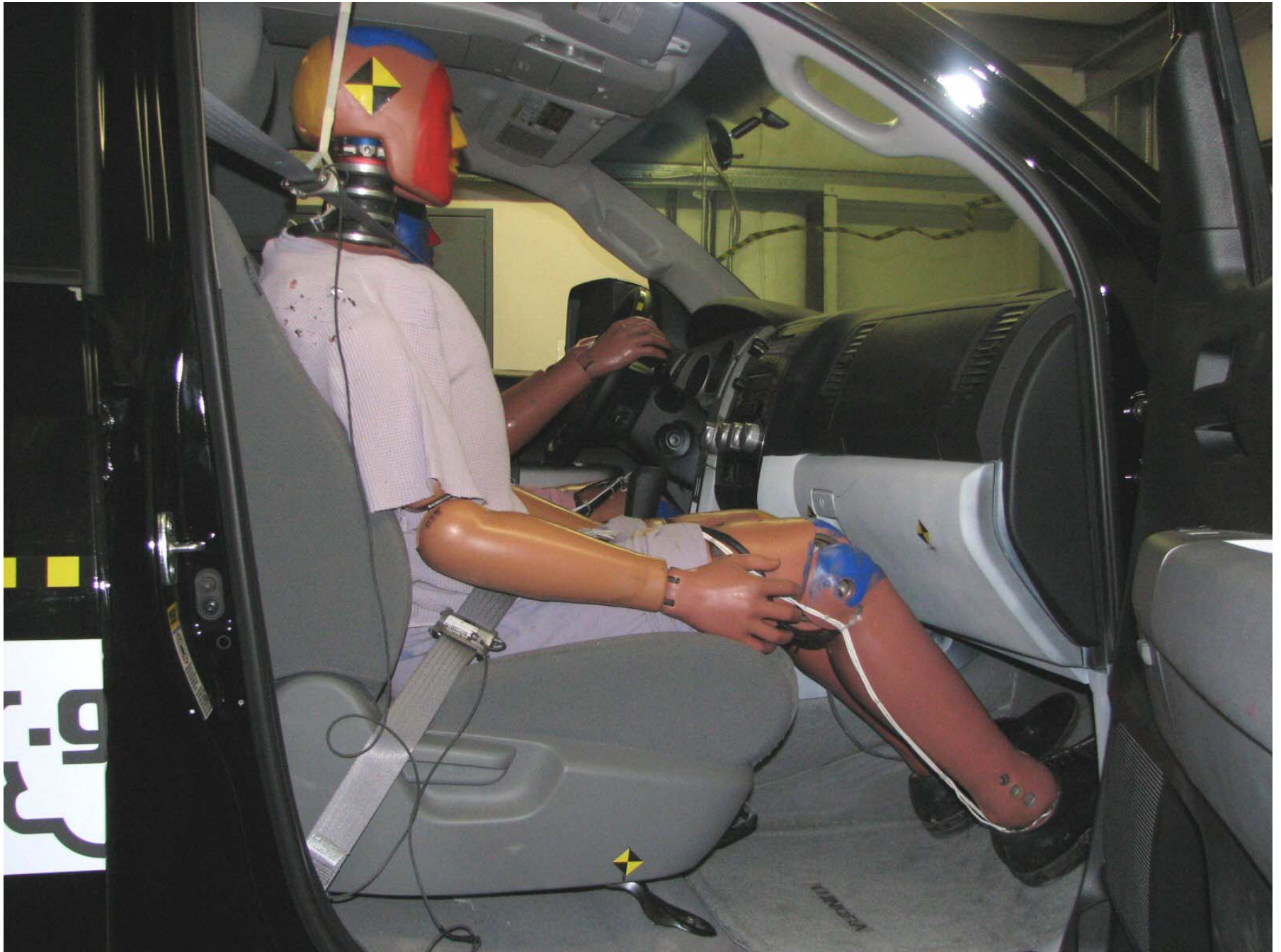
Figure A-48: Pre-Test Passenger Dummy (Door Open)
