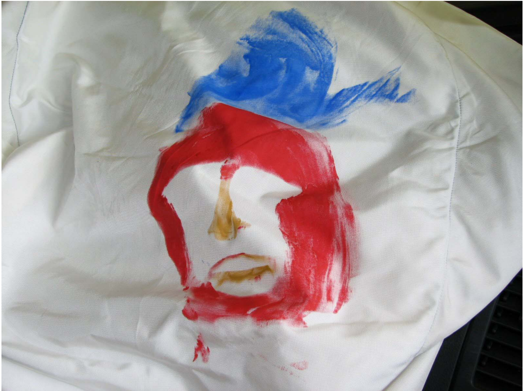
Figure A-57: Post-Test Passenger Dummy Airbag Contact
