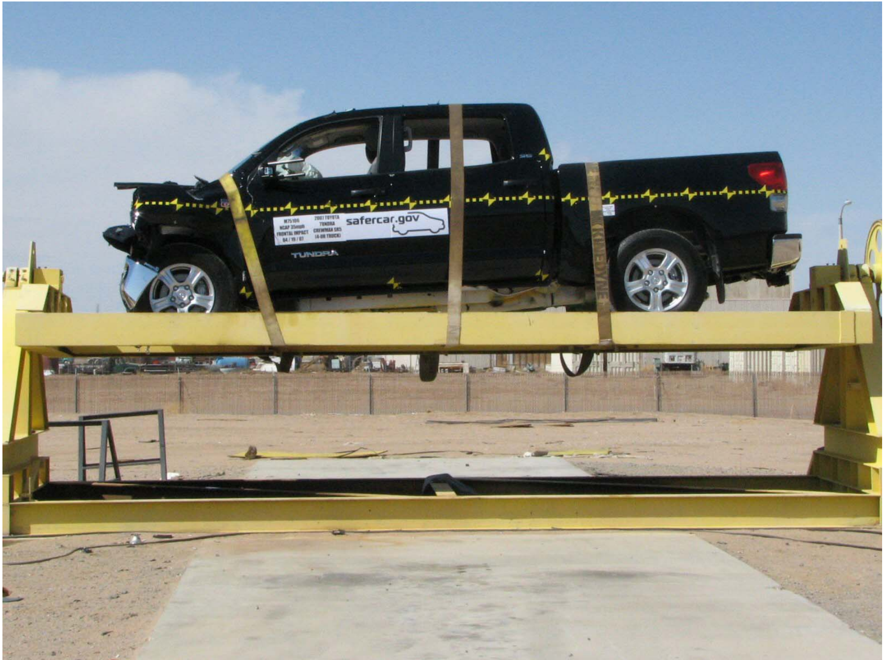
Figure A-58: Vehicle on Rollover Device (0°)
