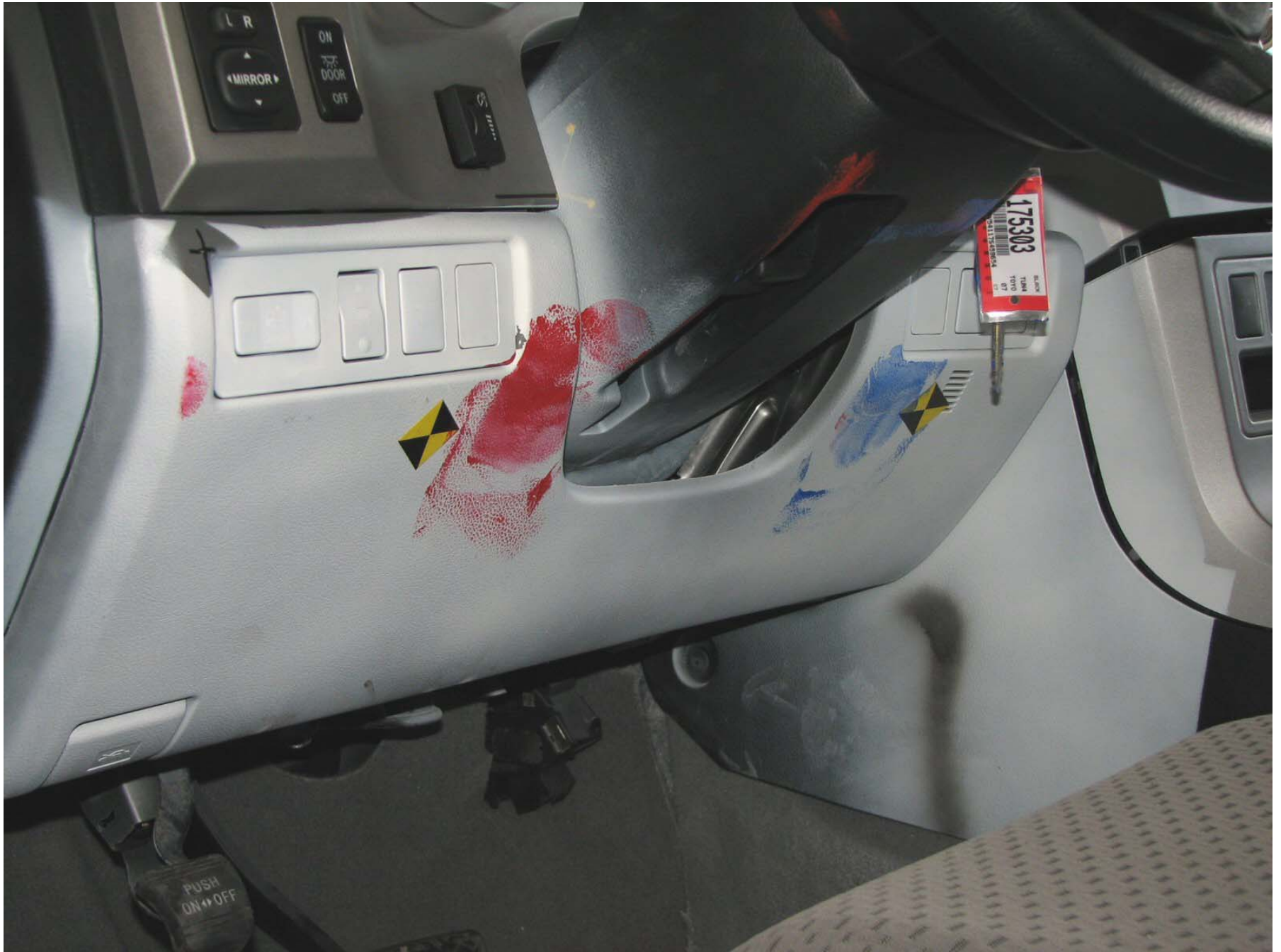
Figure A-39: Post-Test Driver Side Knee Bolster
