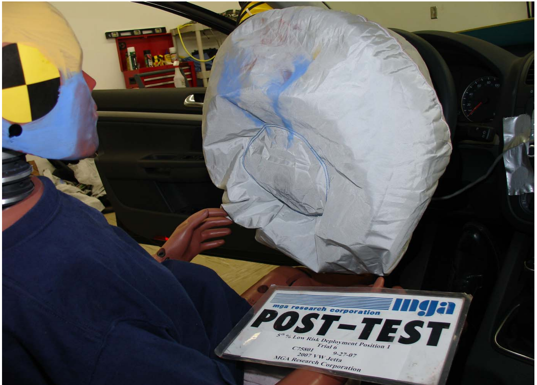
Post-Test 5th Fem. P1 Driver Dummy Airbag Right Side View (Trial 6)
