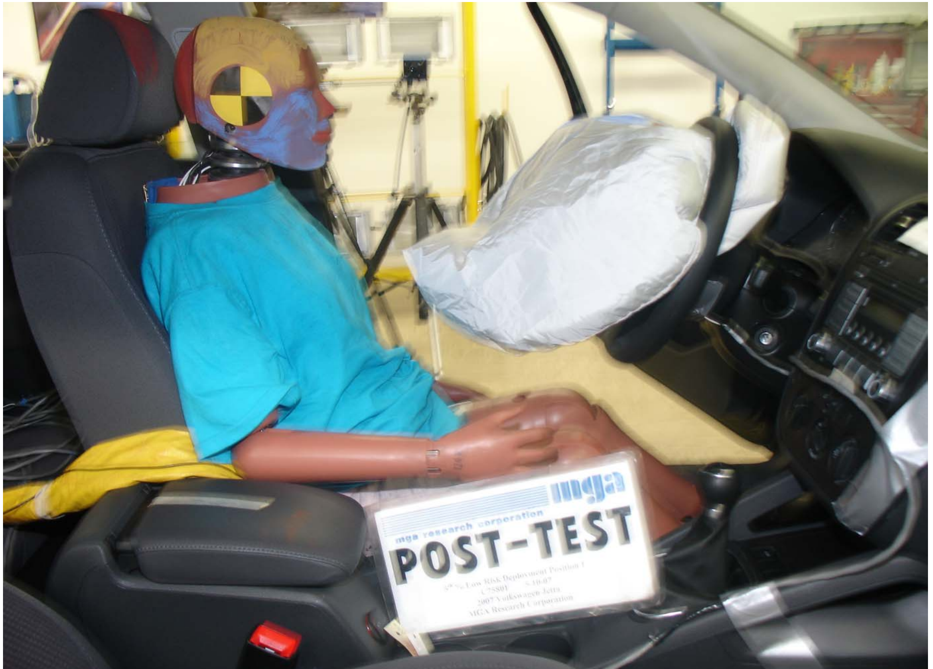
Post-Test 5th Fem. P1 Driver Dummy Right Side View (Trial 1)
