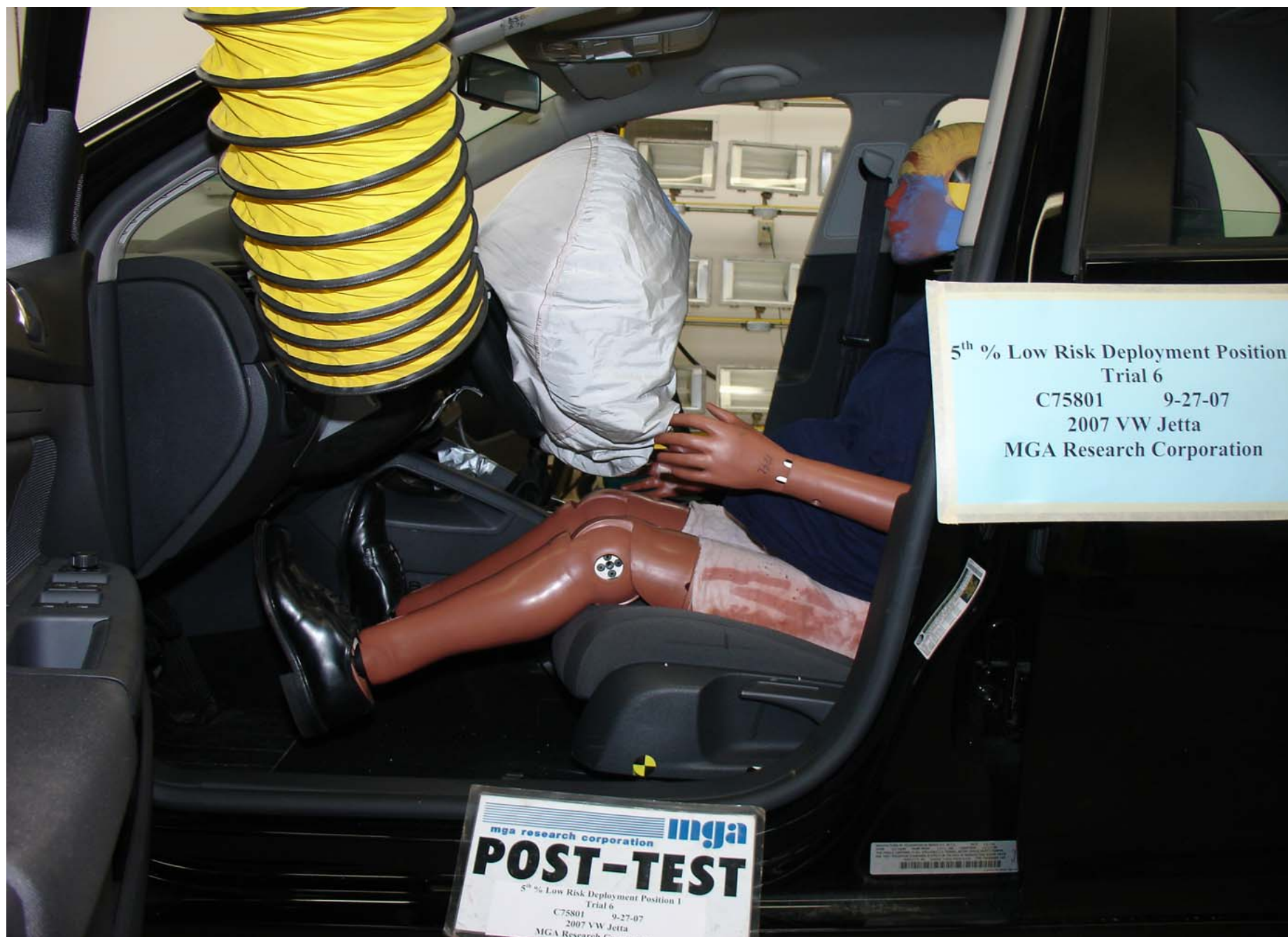
Post-Test 5th Fem. P1 Driver Dummy Left Side View (Trial 6)
