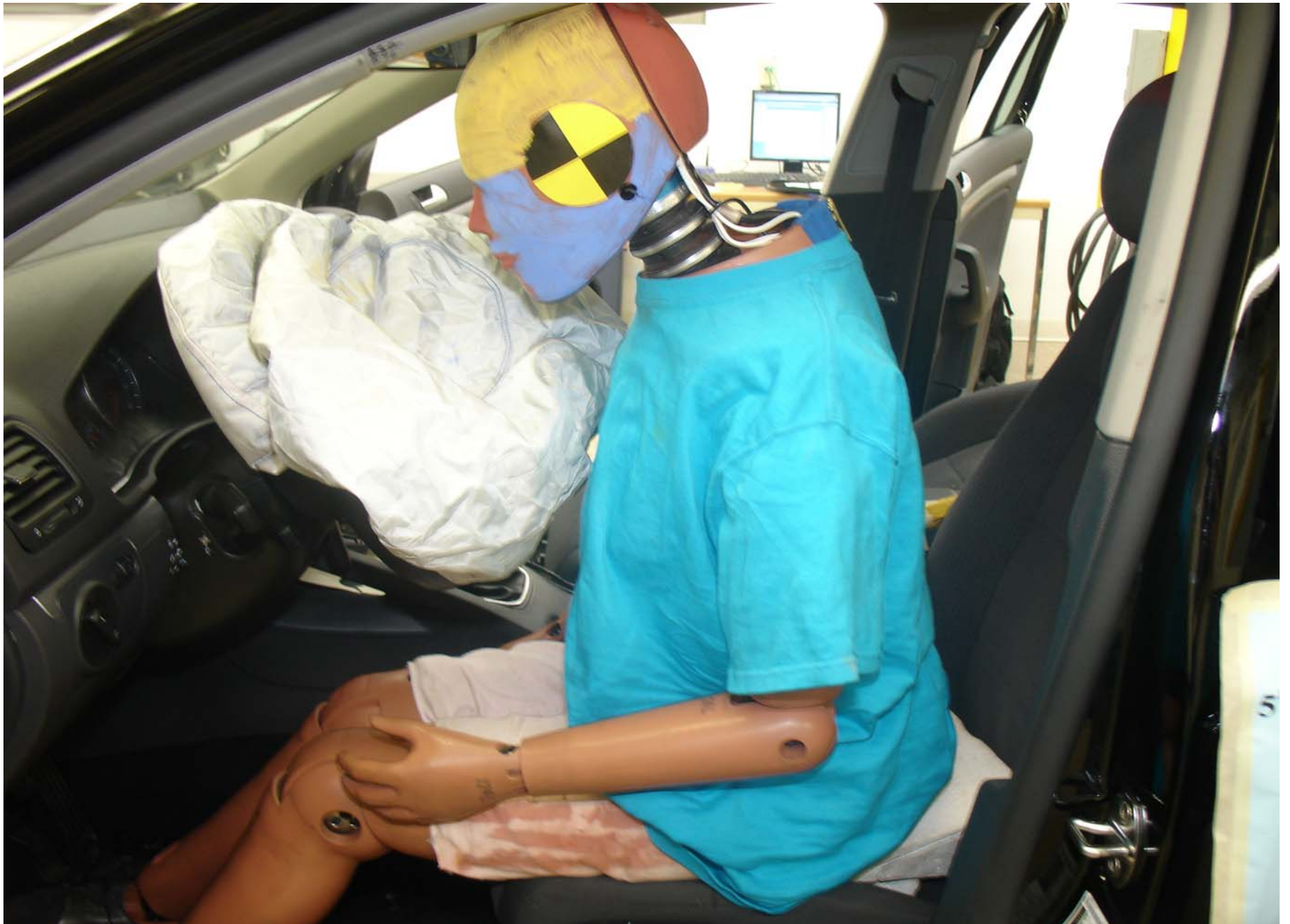
Post-Test 5th Fem. P2 Driver Dummy Left Side View (Trial 2)
