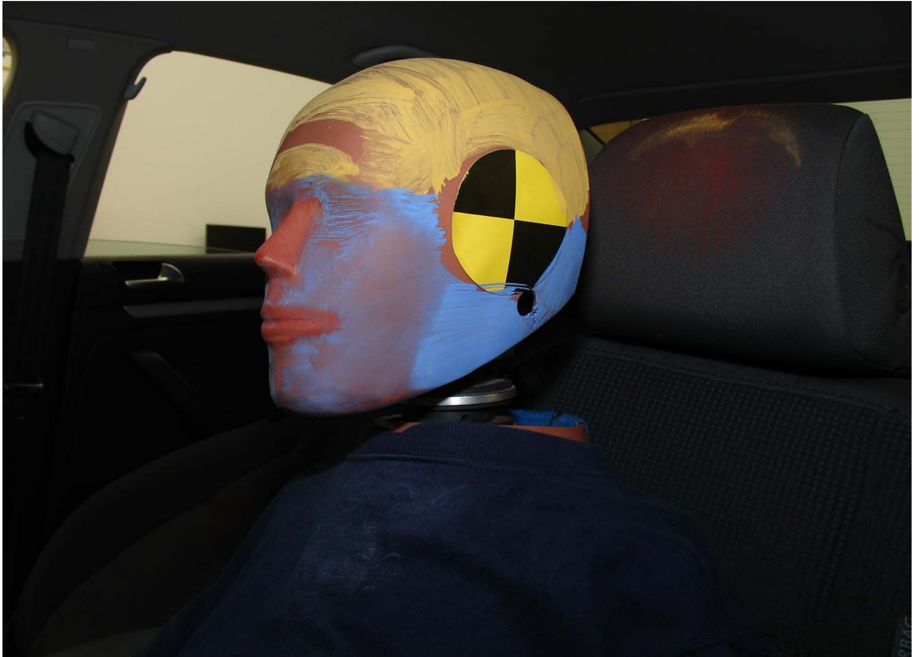
Post-Test 5th Fem. P1 Driver Dummy Head Contact (Headrest) (Trial 6)
