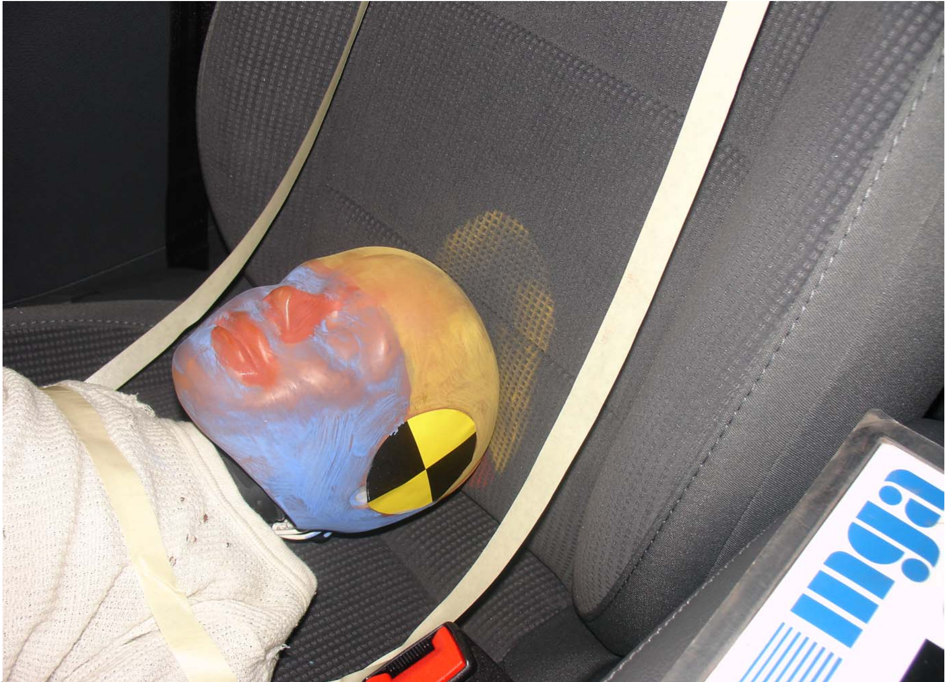
Post-Test 3YO P1 Passenger Dummy Head Contact View
