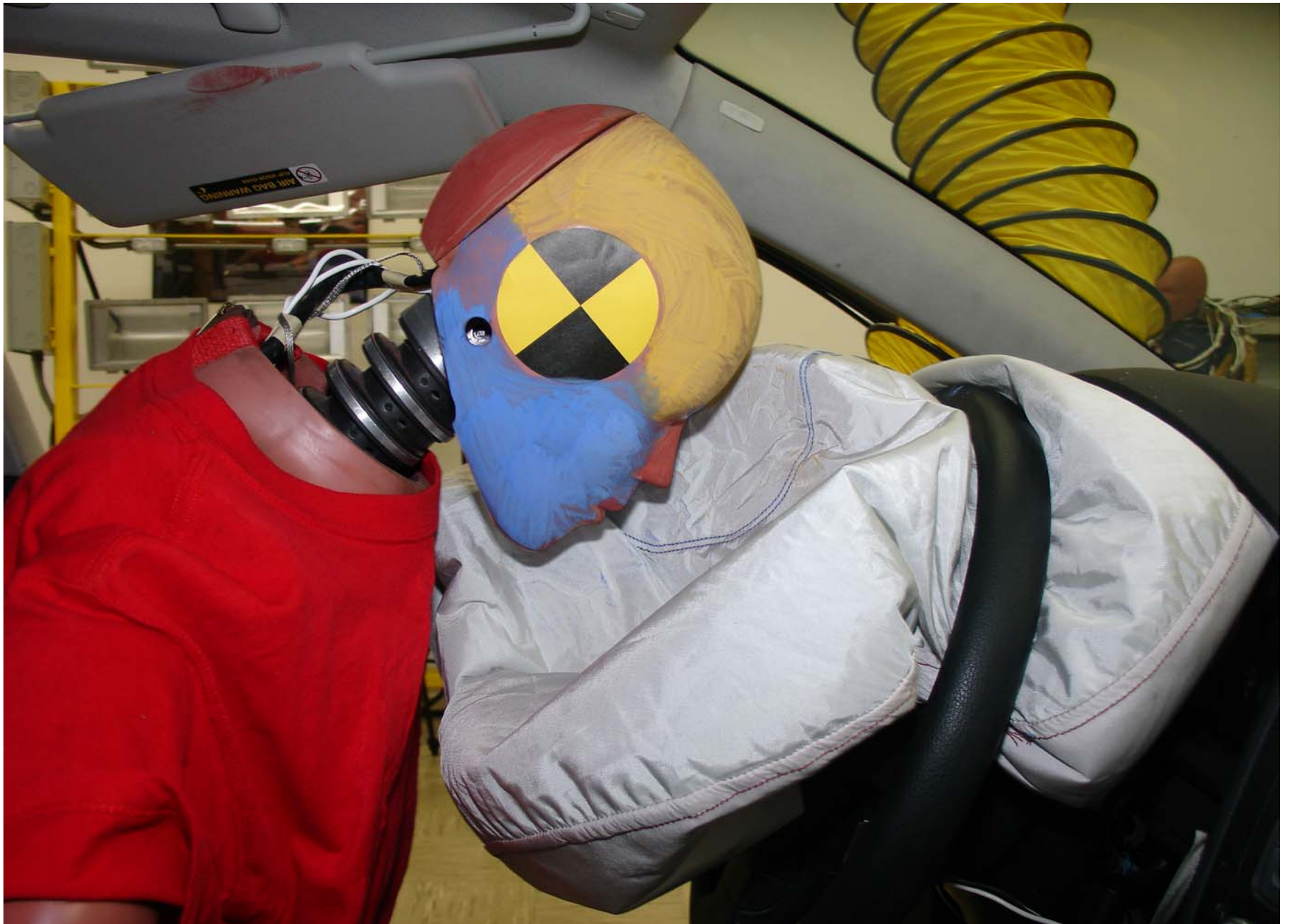
Post-Test 5th Fem. P2 Driver Dummy Airbag Right Side View (Trial 3)
