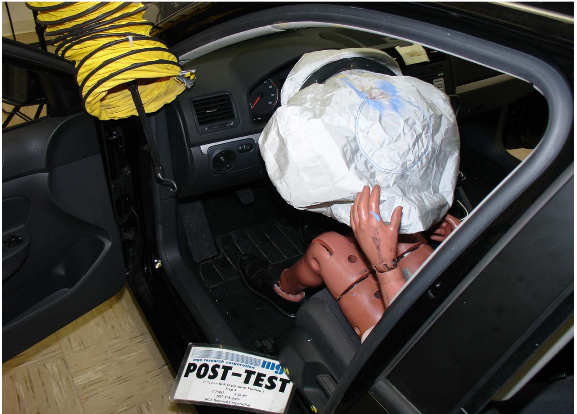
Post-Test 5th Fem. P1 Driver Dummy Airbag Left Side View (Trial 4)
