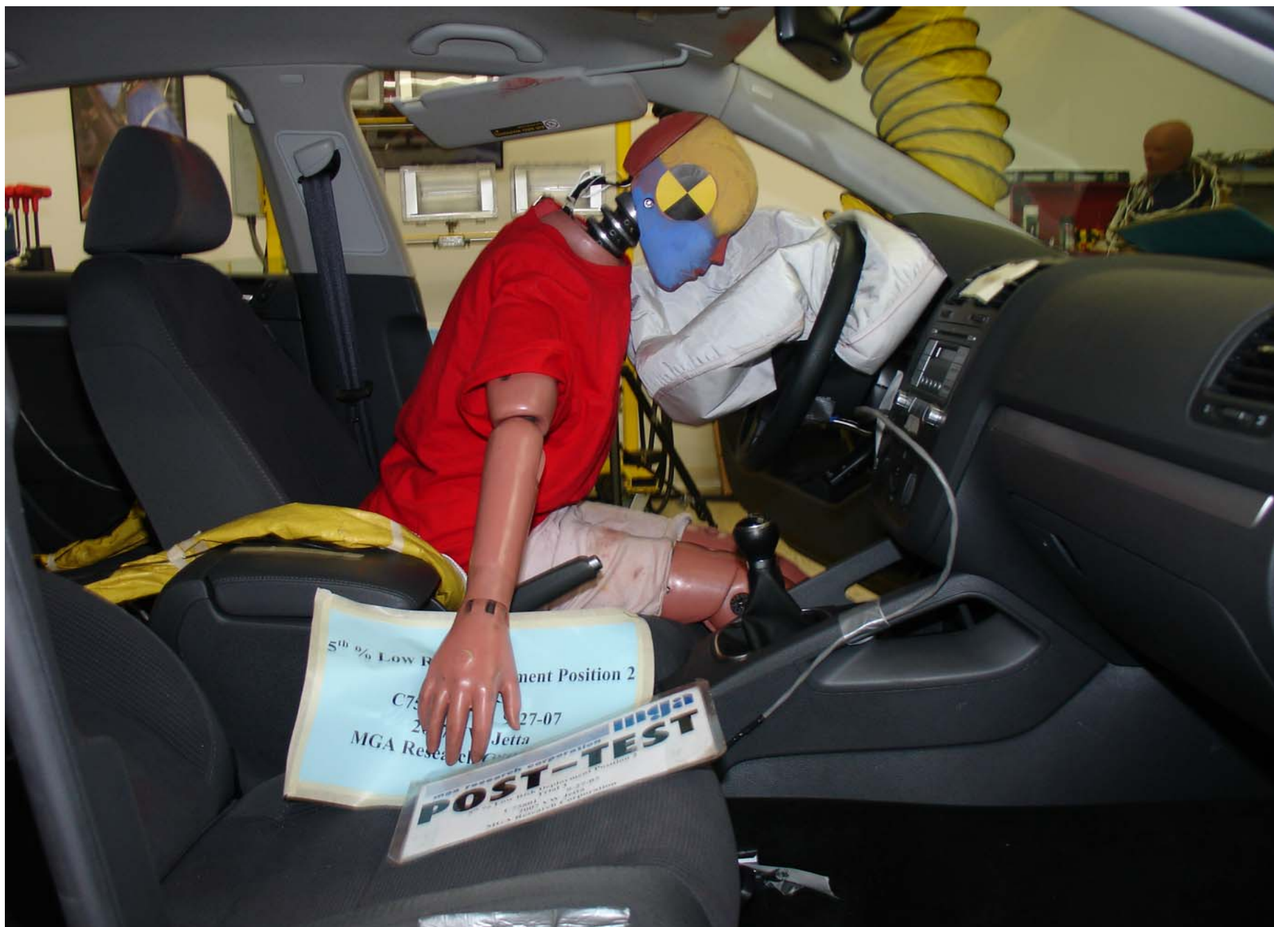
Post-Test 5th Fem. P2 Driver Dummy Right Side View (Trial 3)
