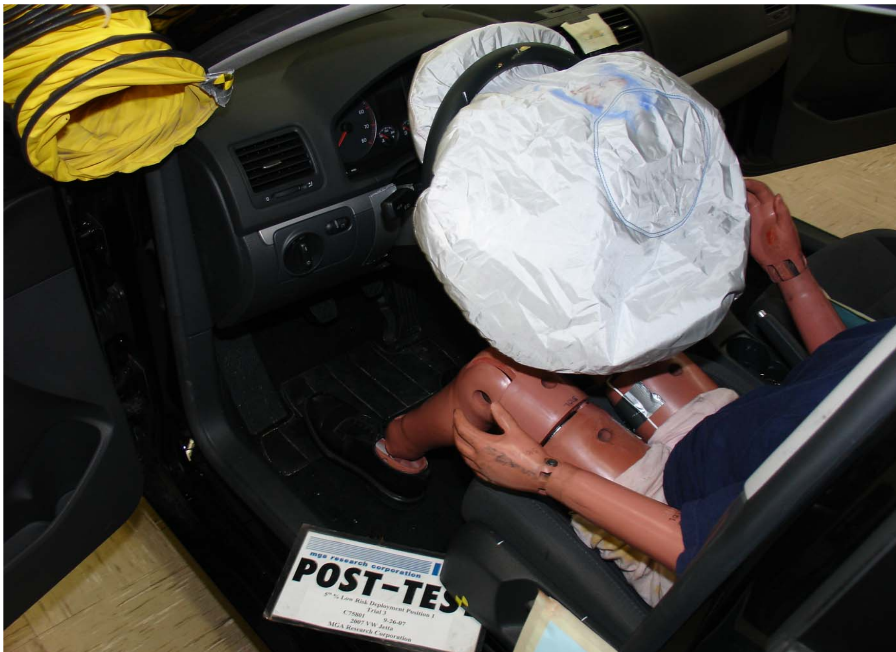
Post-Test 5th Fem. P1 Driver Dummy Airbag Left Side View (Trial 3)
