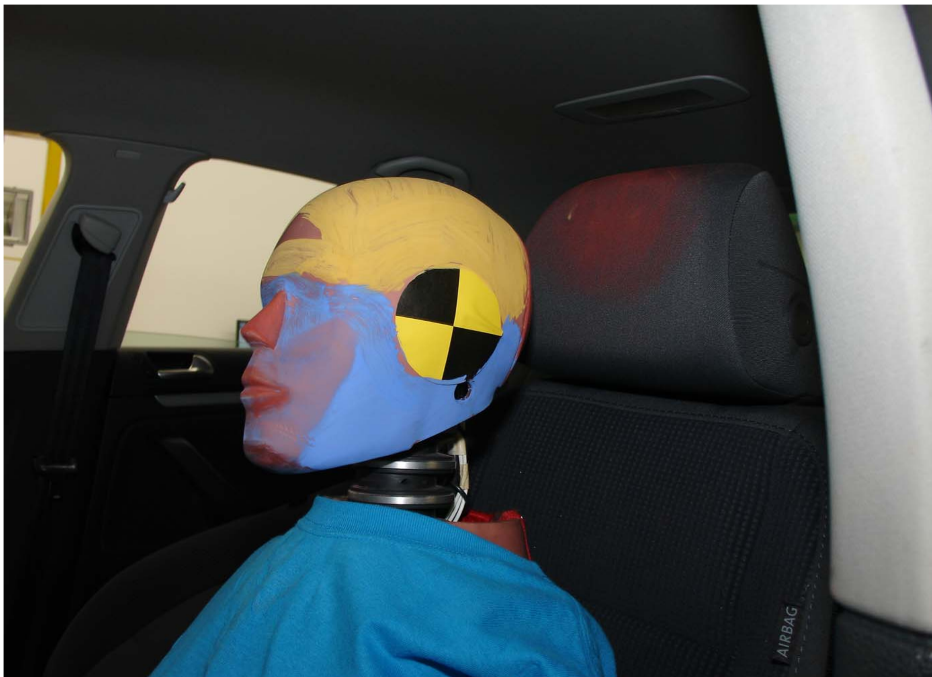
Post-Test 5th Fem. P1 Driver Dummy Head Contact (Headrest) (Trial 5)
