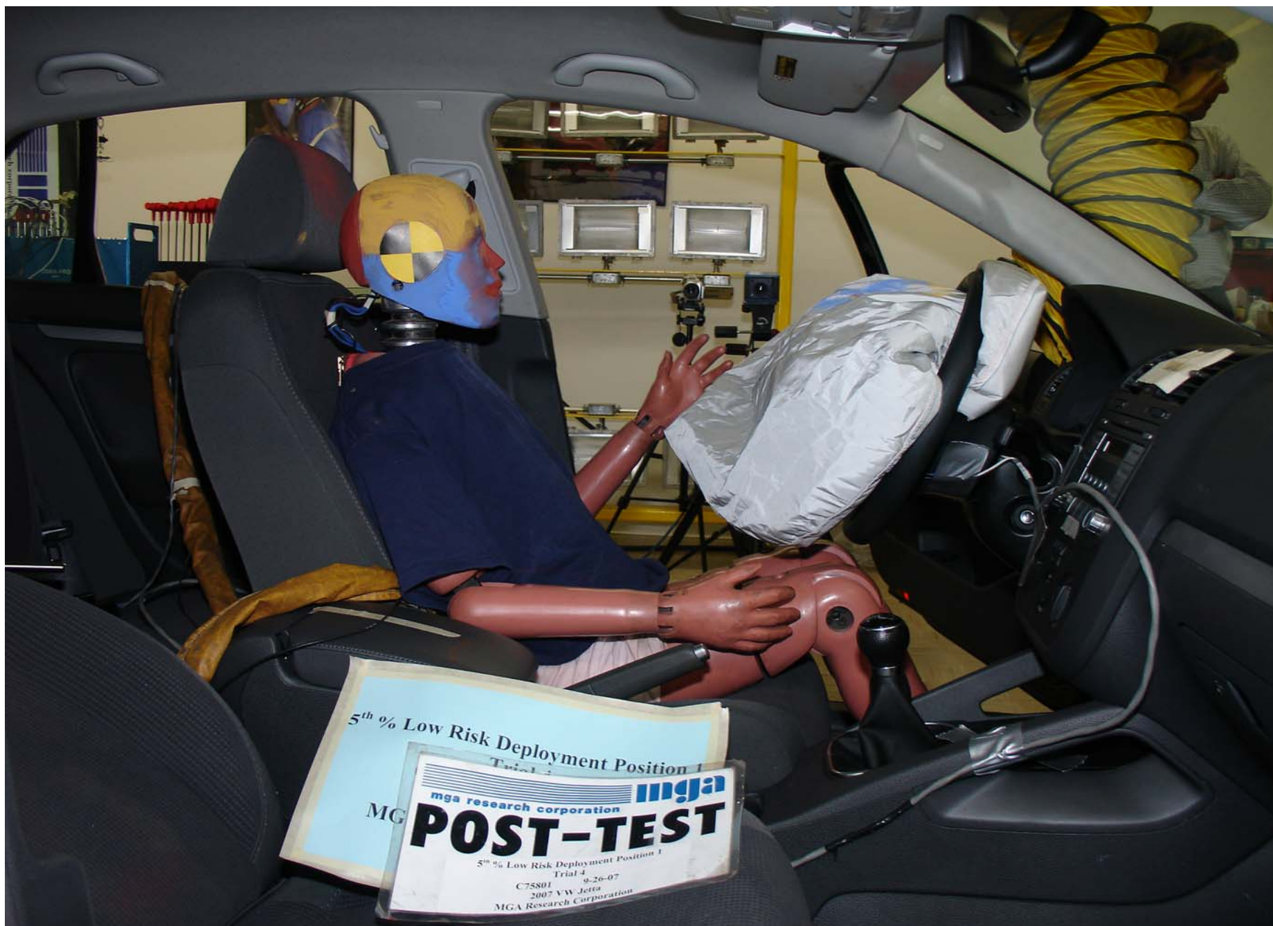
Post-Test 5th Fem. P1 Driver Dummy Right Side View (Trial 4)
