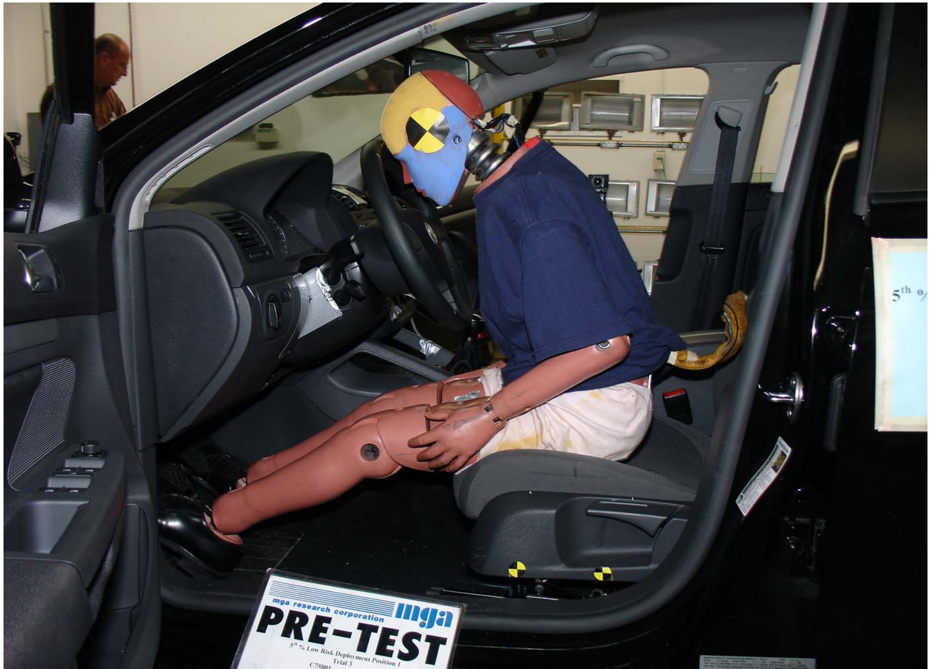
Pre-Test 5th Fem. P1 Driver Dummy Left Side View (Trial 3)
