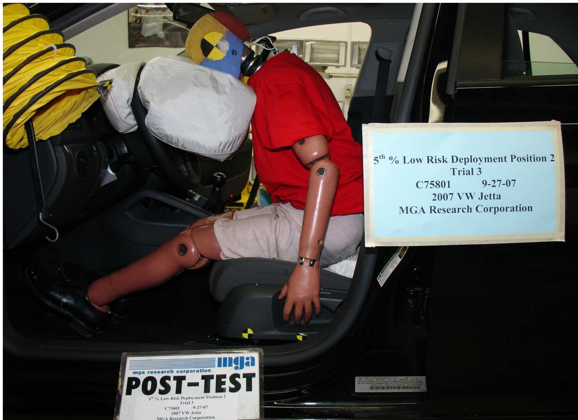
Post-Test 5th Fem. P2 Driver Dummy Left Side View (Trial 3)
