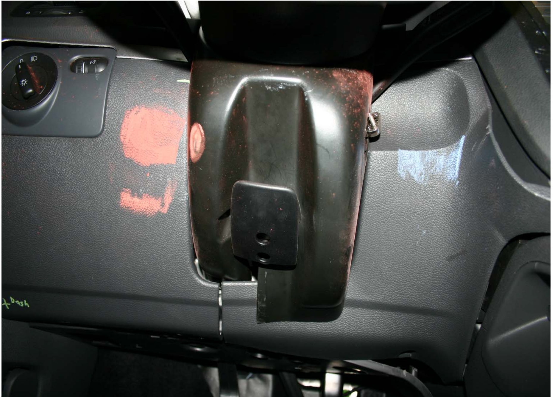
Post-Test Driver Dummy Knee Contact
