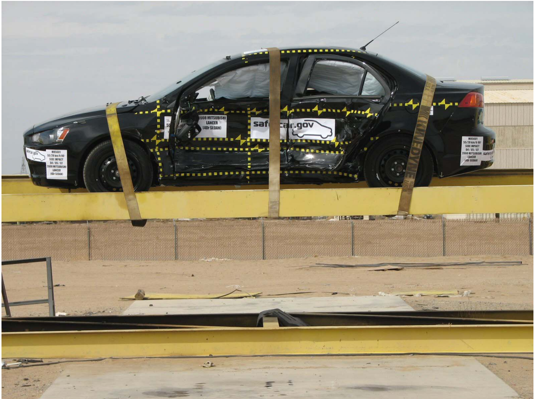
Figure A-61: Vehicle on Rollover Device (0°)
