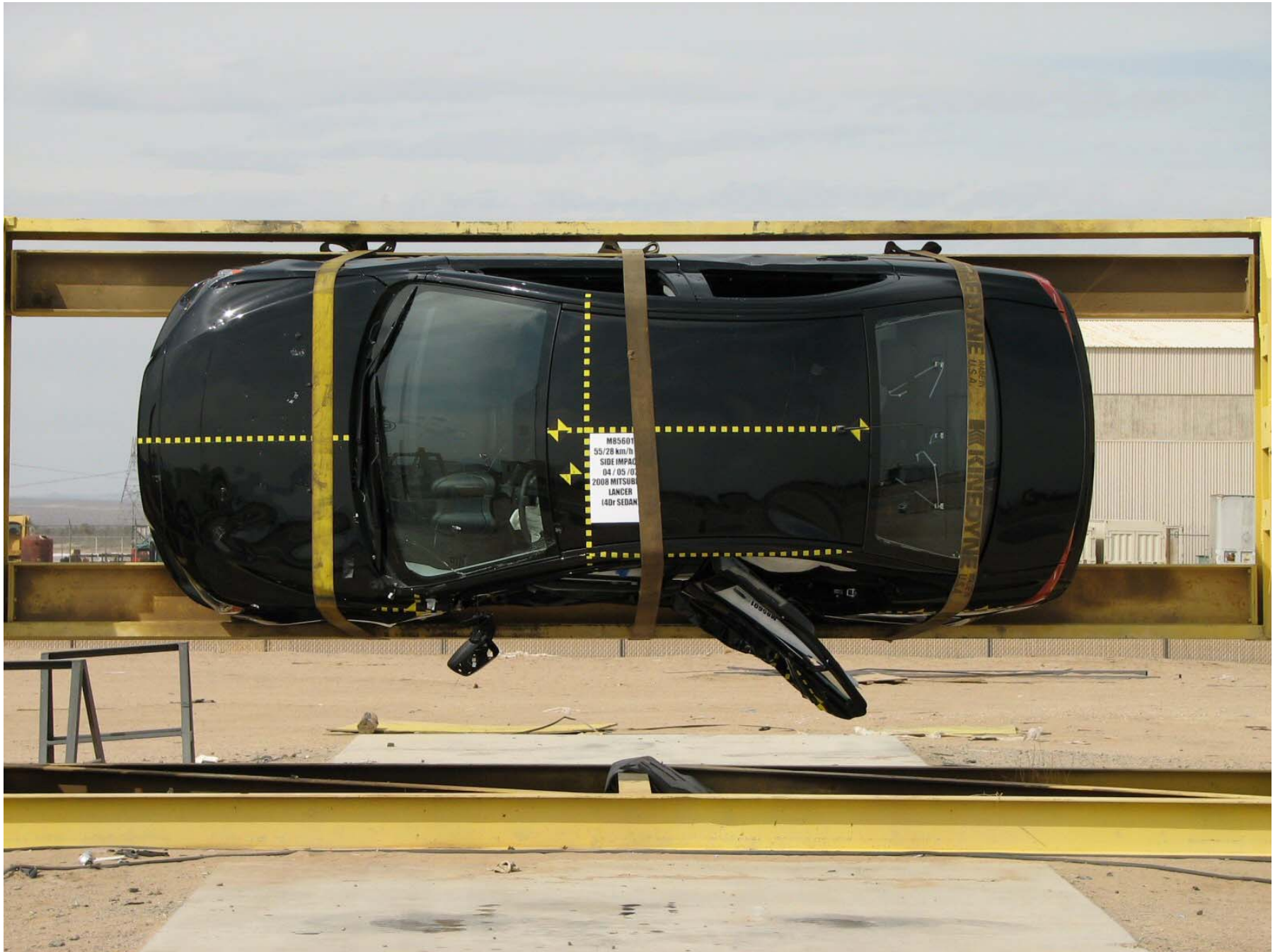
Figure A-62: Vehicle on Rollover Device (90°)
