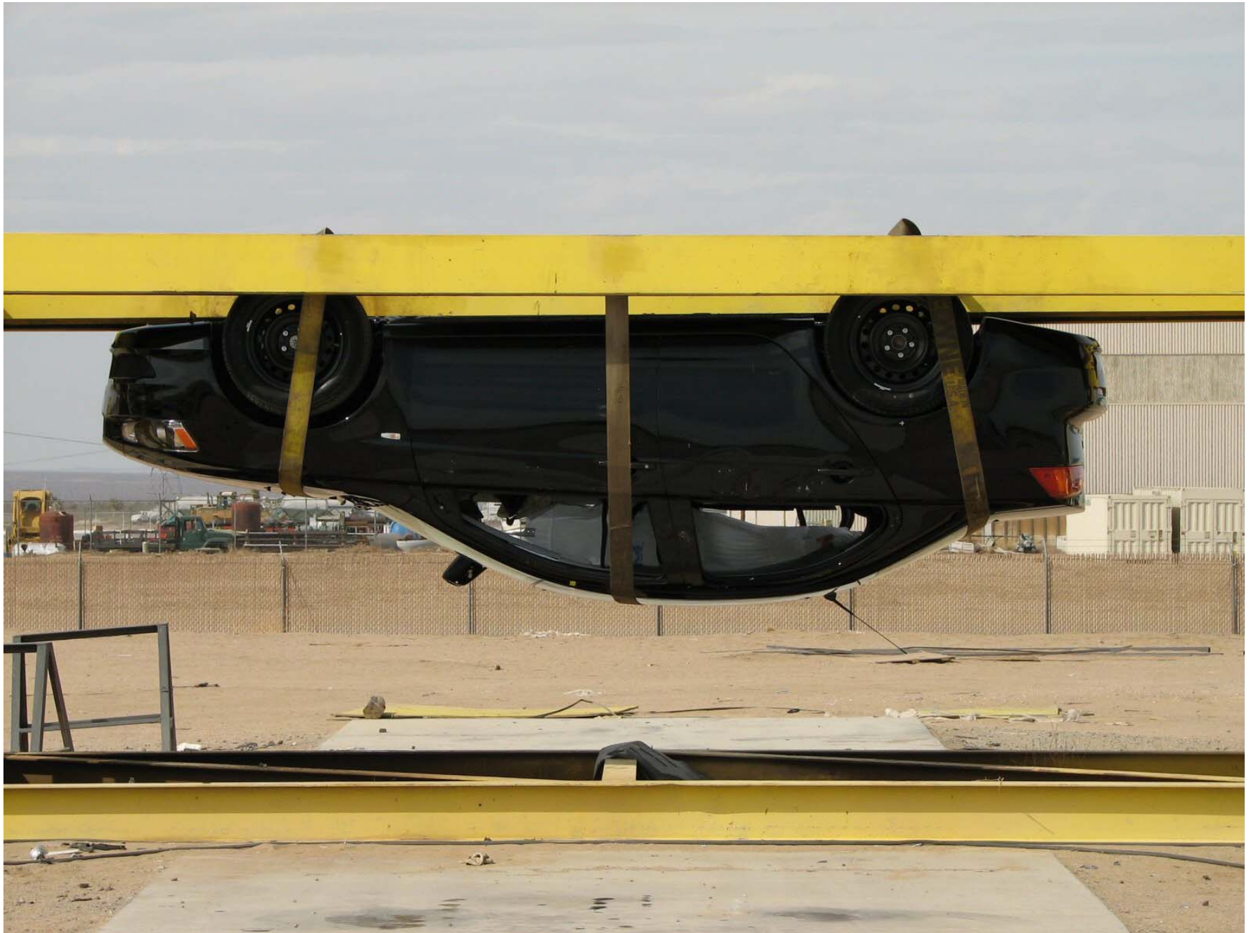
Figure A-63: Vehicle on Rollover Device (180°)
