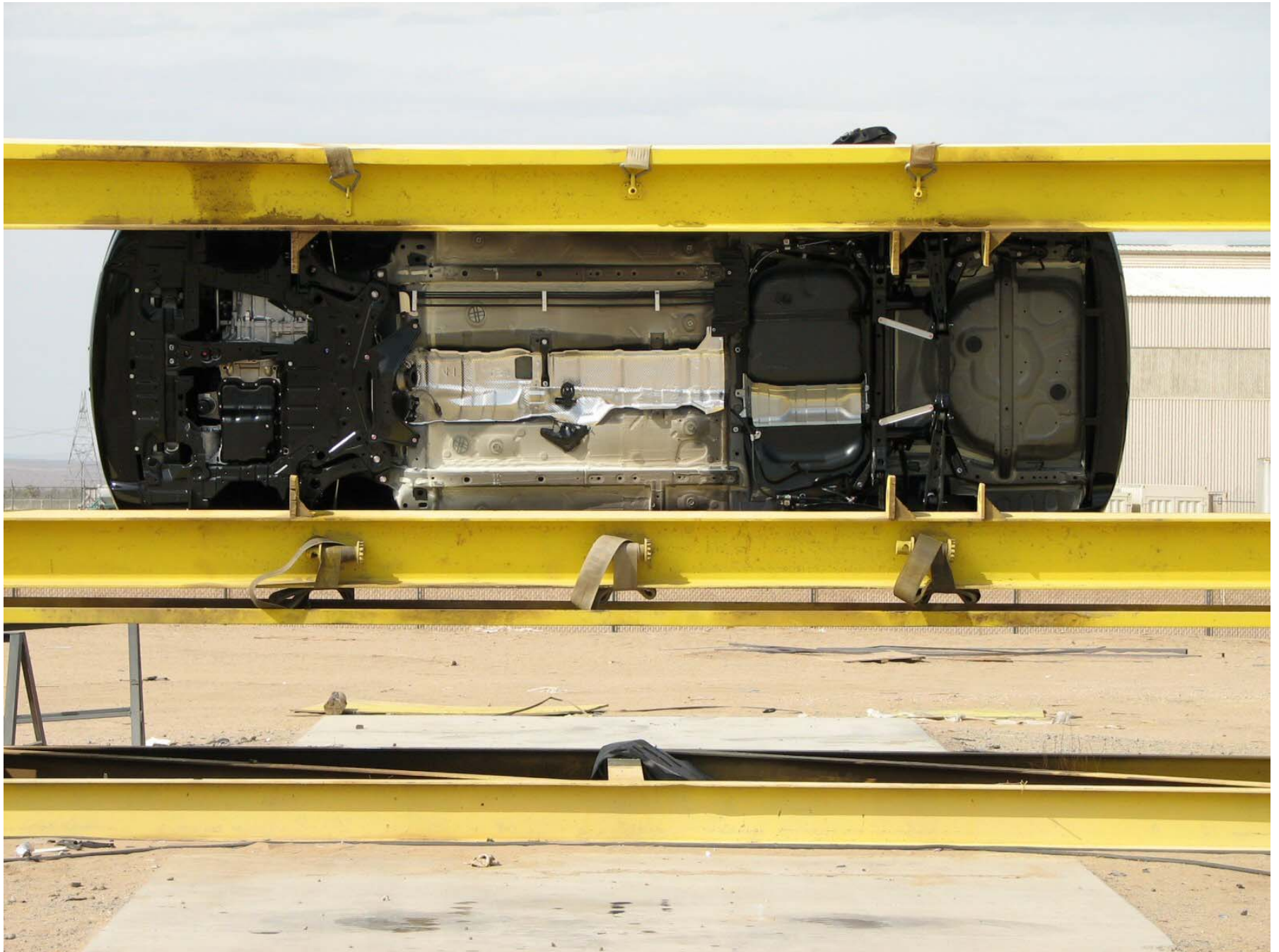
Figure A-64: Vehicle on Rollover Device (270°)
