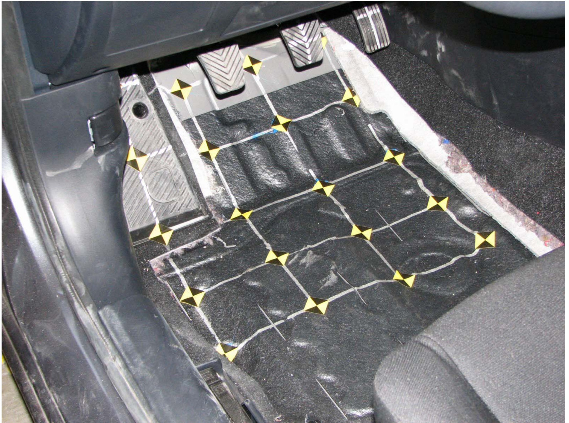
Figure A-40: Pre-Test Driver Side Floor Pan
