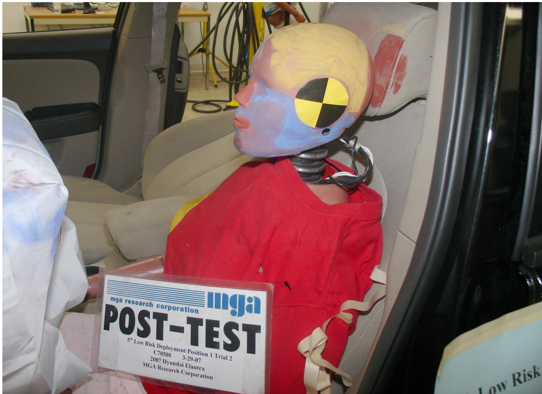
Post-Test 5th Fem. P1 Trial 2 Driver Dummy Airbag Left View
