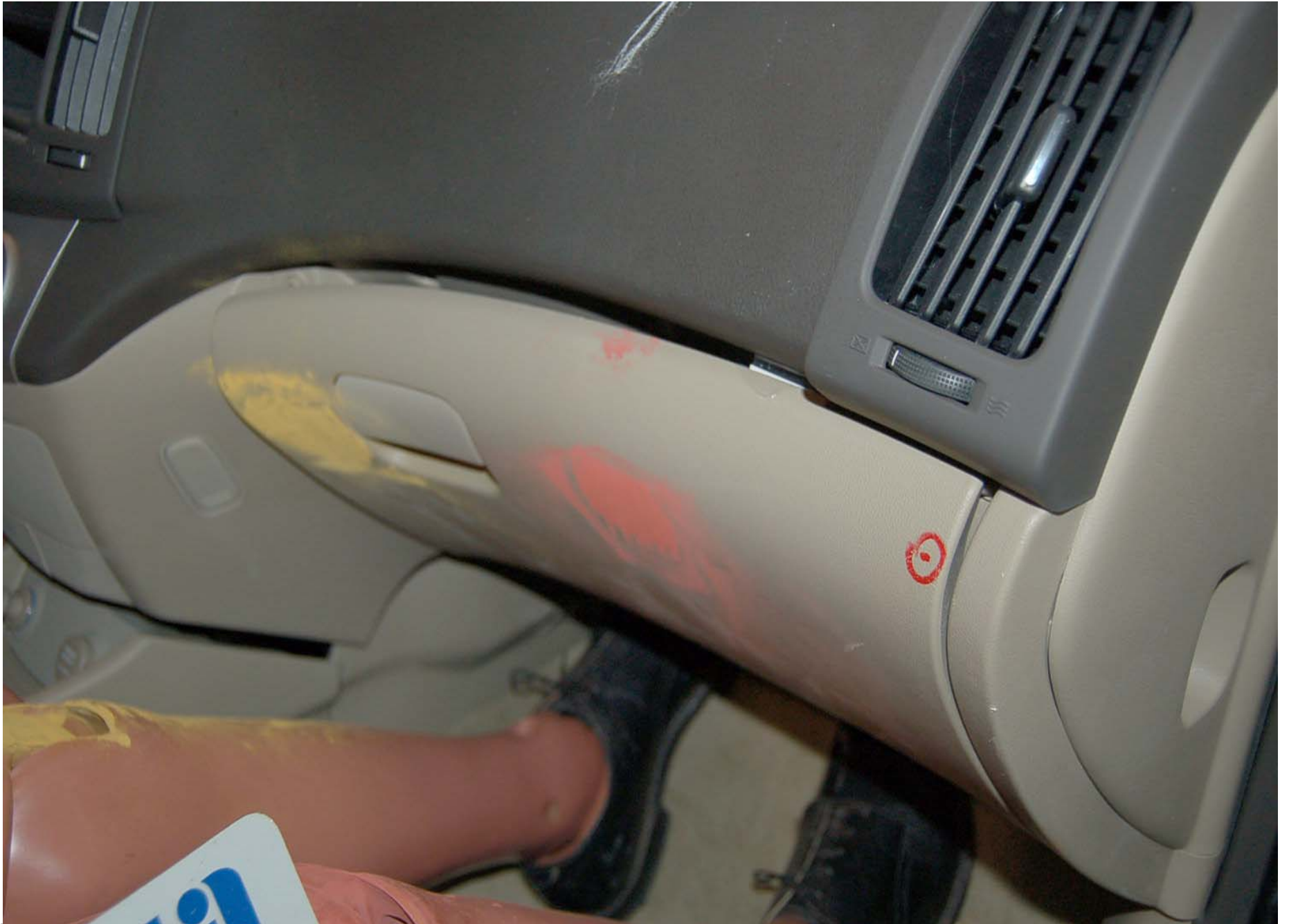
Post-Test Passenger Dummy Knee Contact
