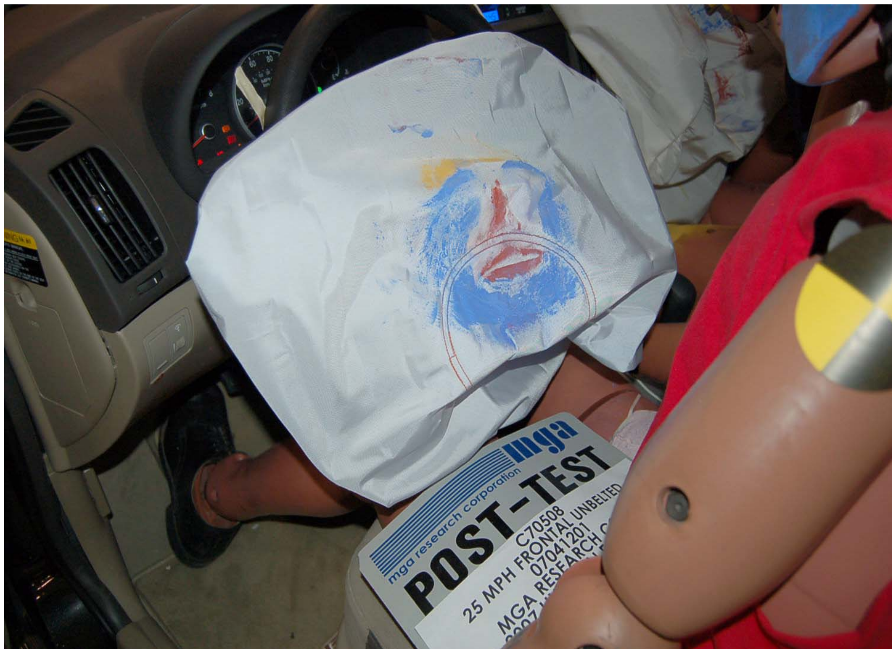
Post-Test Driver Dummy Airbag Contact
