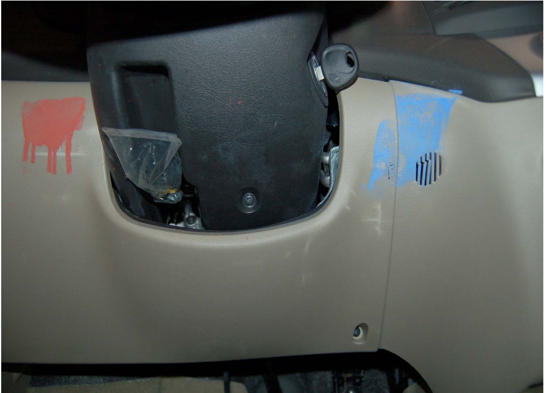
Post-Test Driver Dummy Knee Contact
