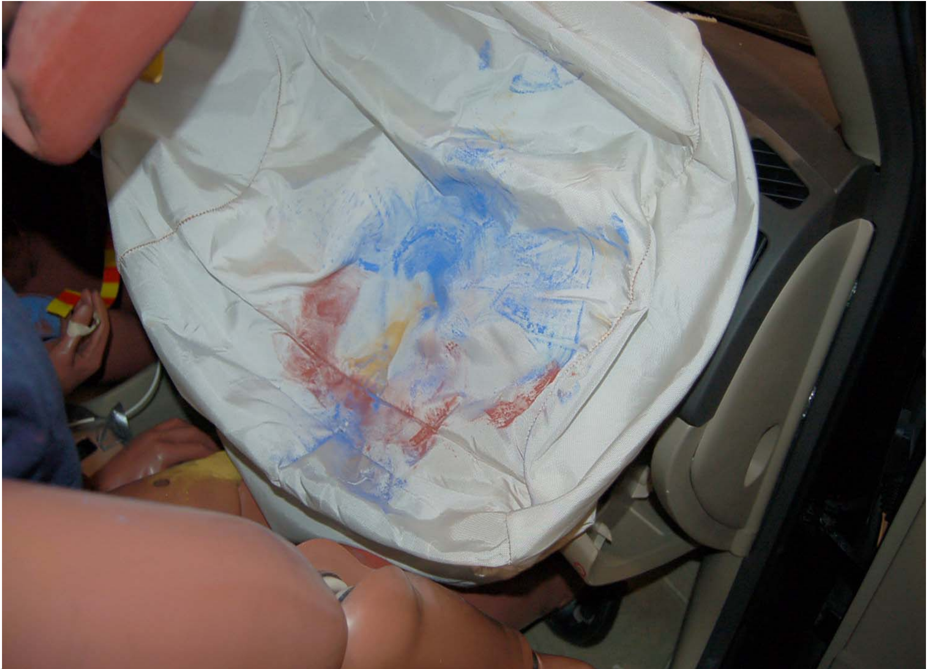
Post-Test Passenger Dummy Airbag Contact
