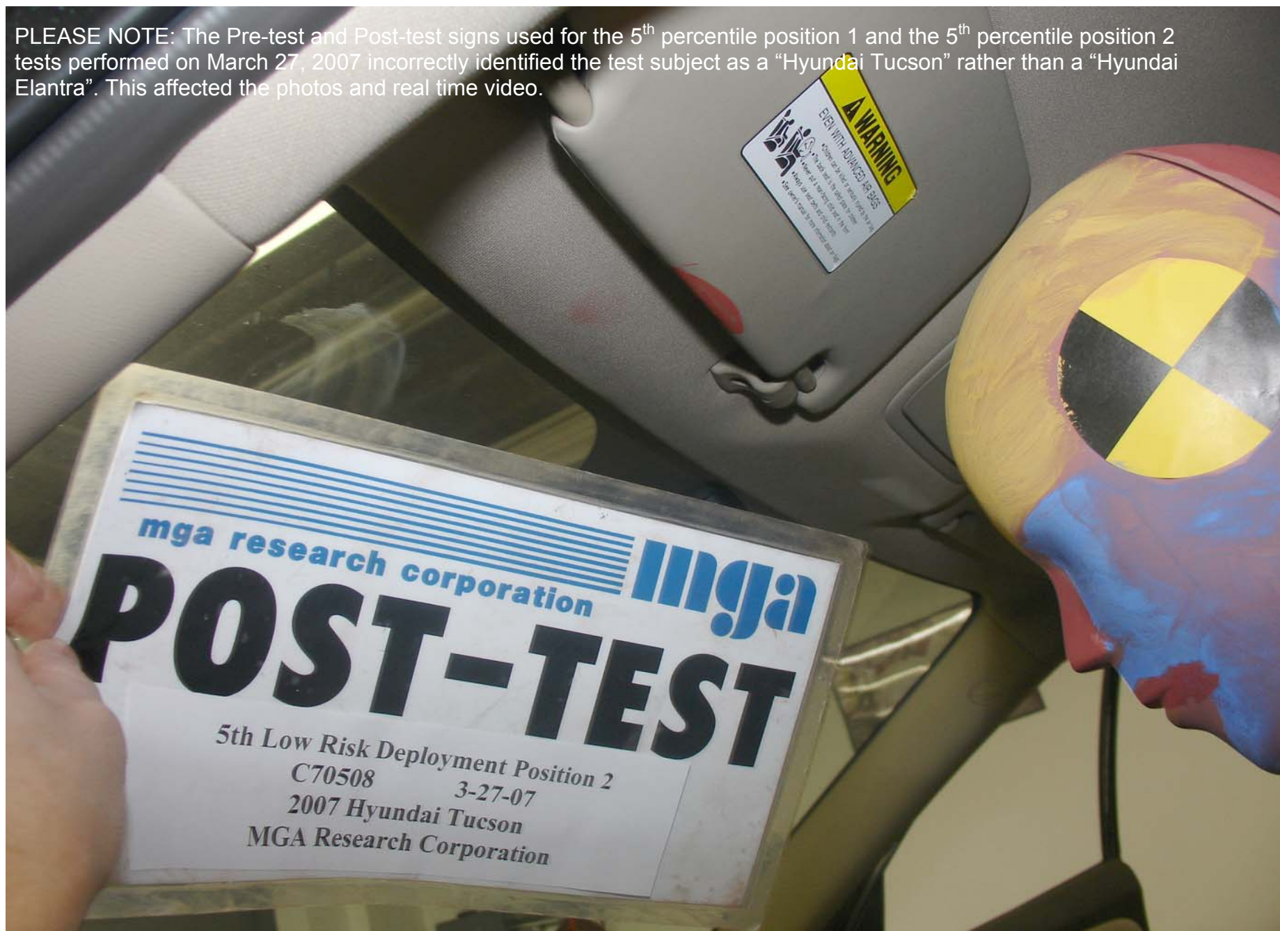
Post-Test 5th Fem. P2 Driver Dummy Head Contact
