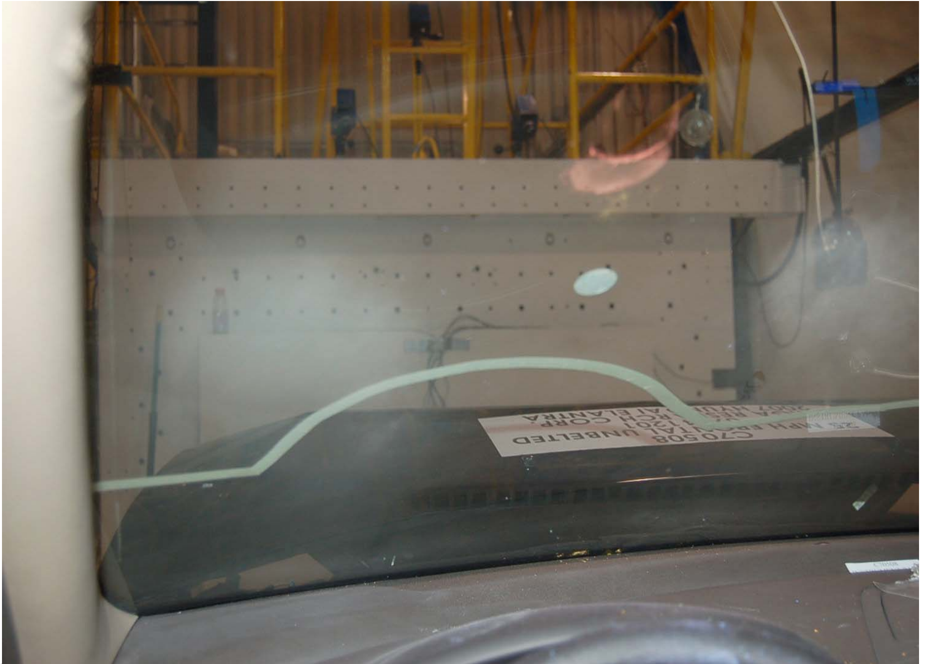
Post-Test Driver Dummy Head Contact (windshield)
