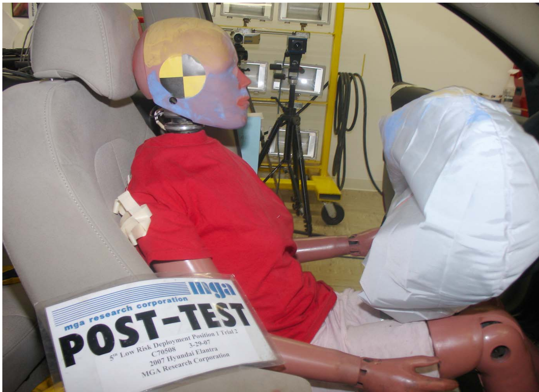
Post-Test 5th Fem. P1 Trial 2 Driver Dummy Airbag Right View
