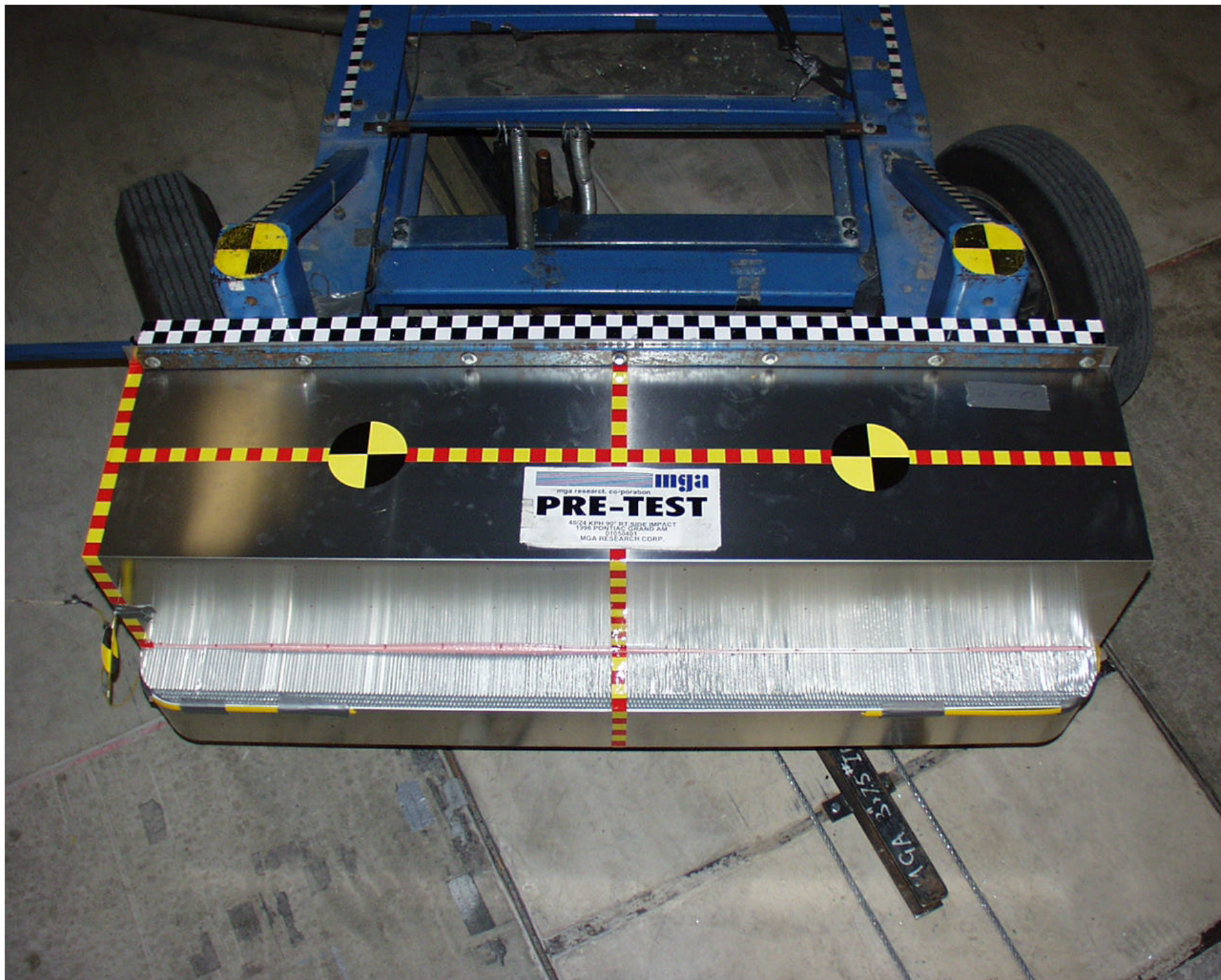
Photo No. A-10 - Pre-Test MDB Top View
