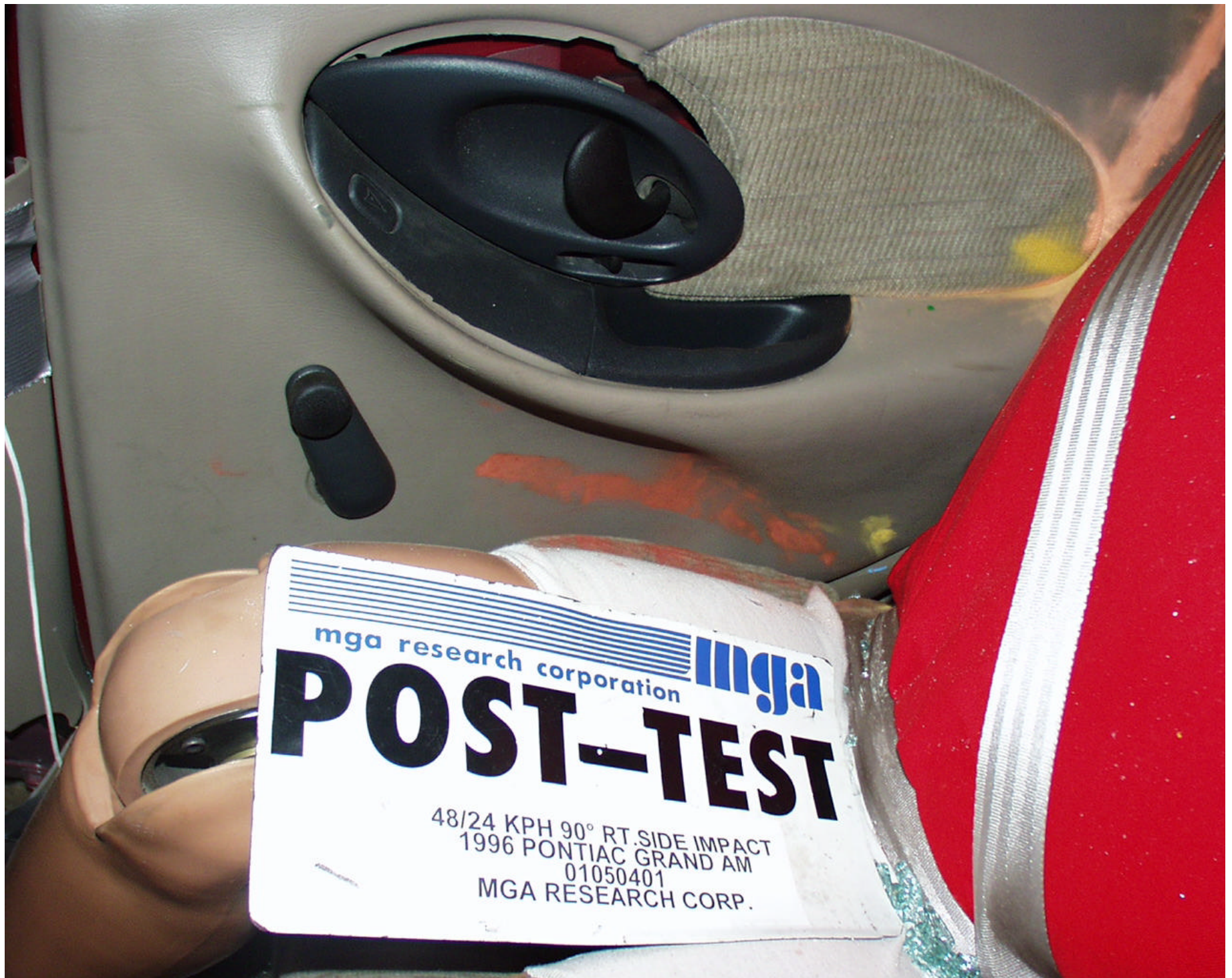
Photo No. A-33 - Post-Test RRP Dummy Contact
