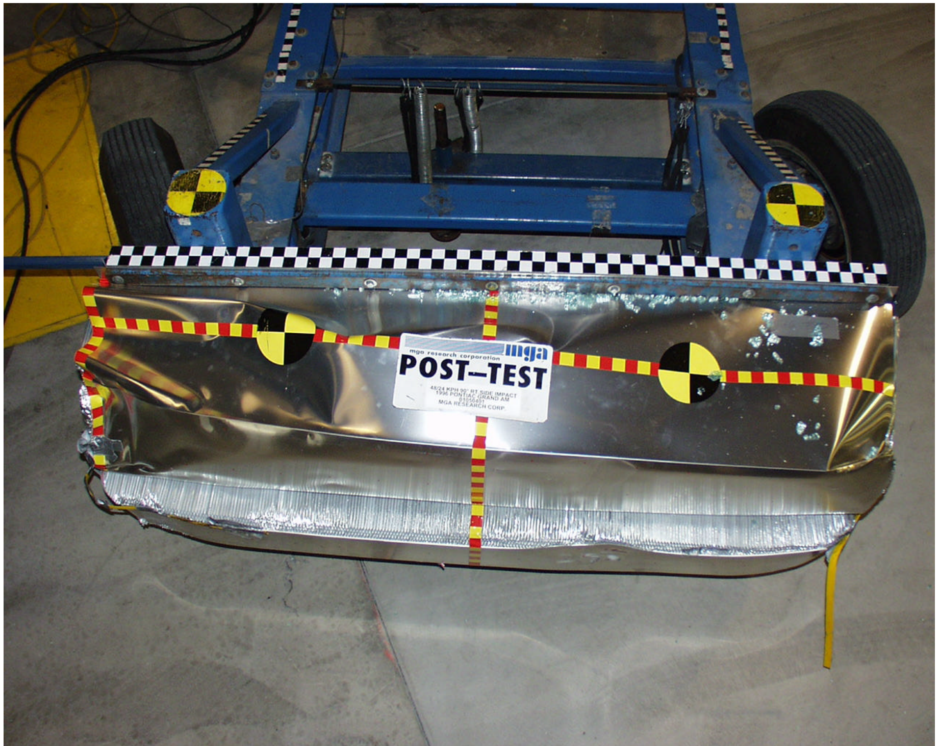
Photo No. A-11 - Post-Test MDB Top View
