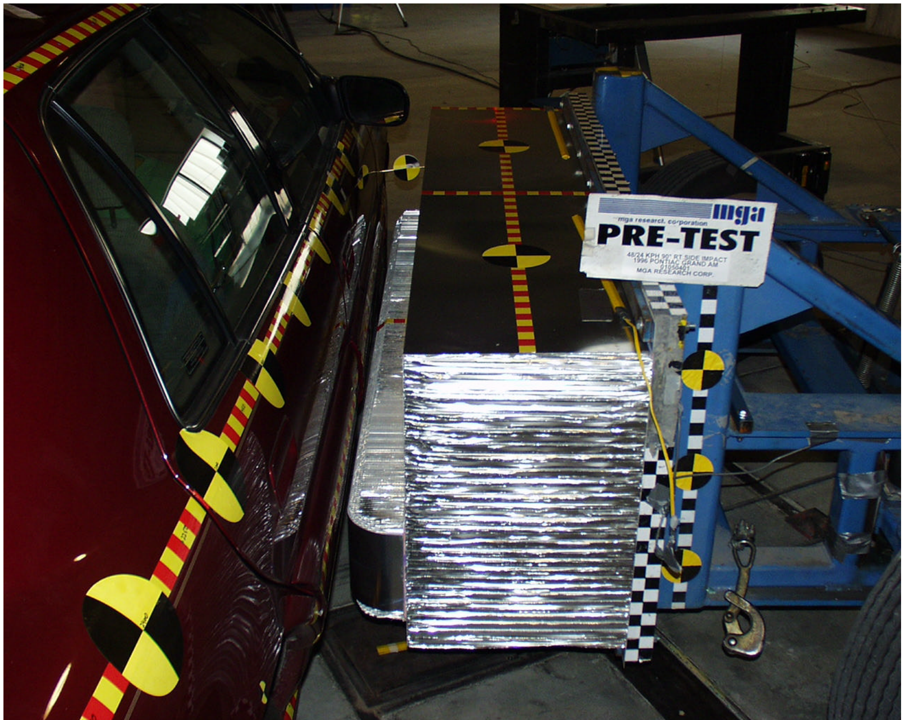
Photo No. A-5 - Pre-Test MDB Positioned Against Vehicle (left side)
