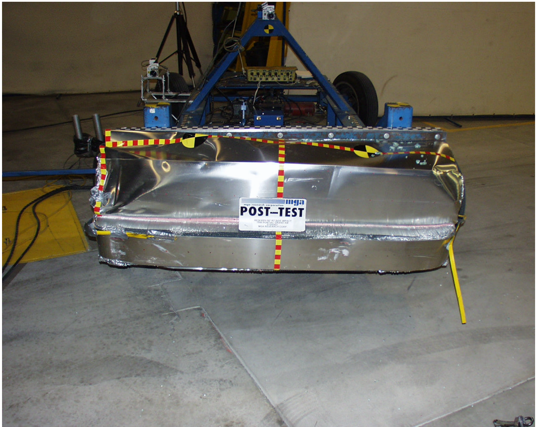
Photo No. A-13 - Post-Test MDB Front View
