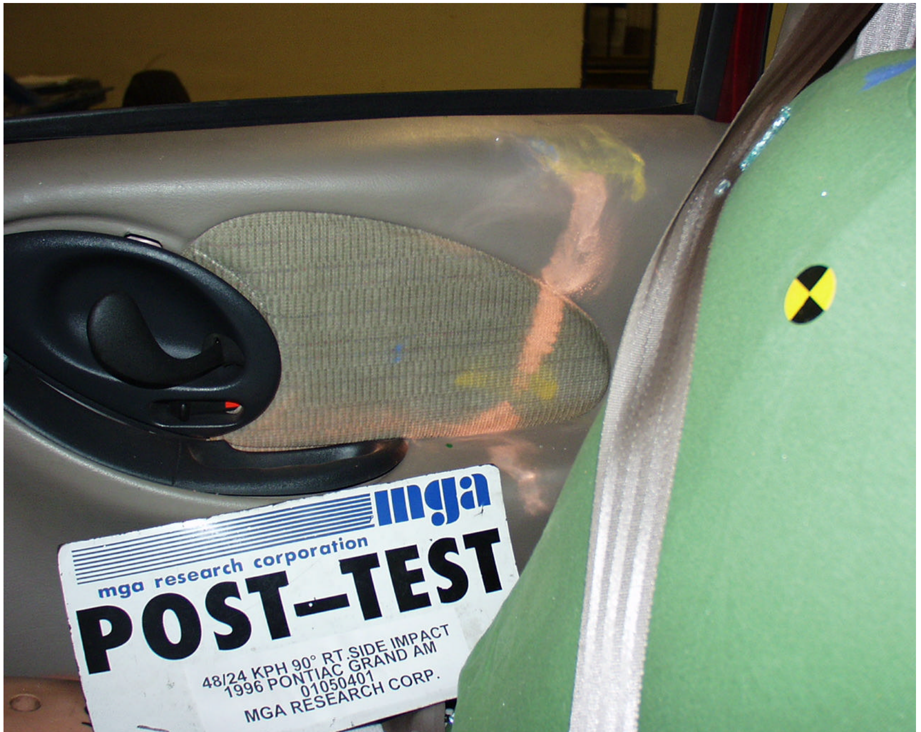
Photo No. A-25 - Post-Test RFP Dummy Contact
