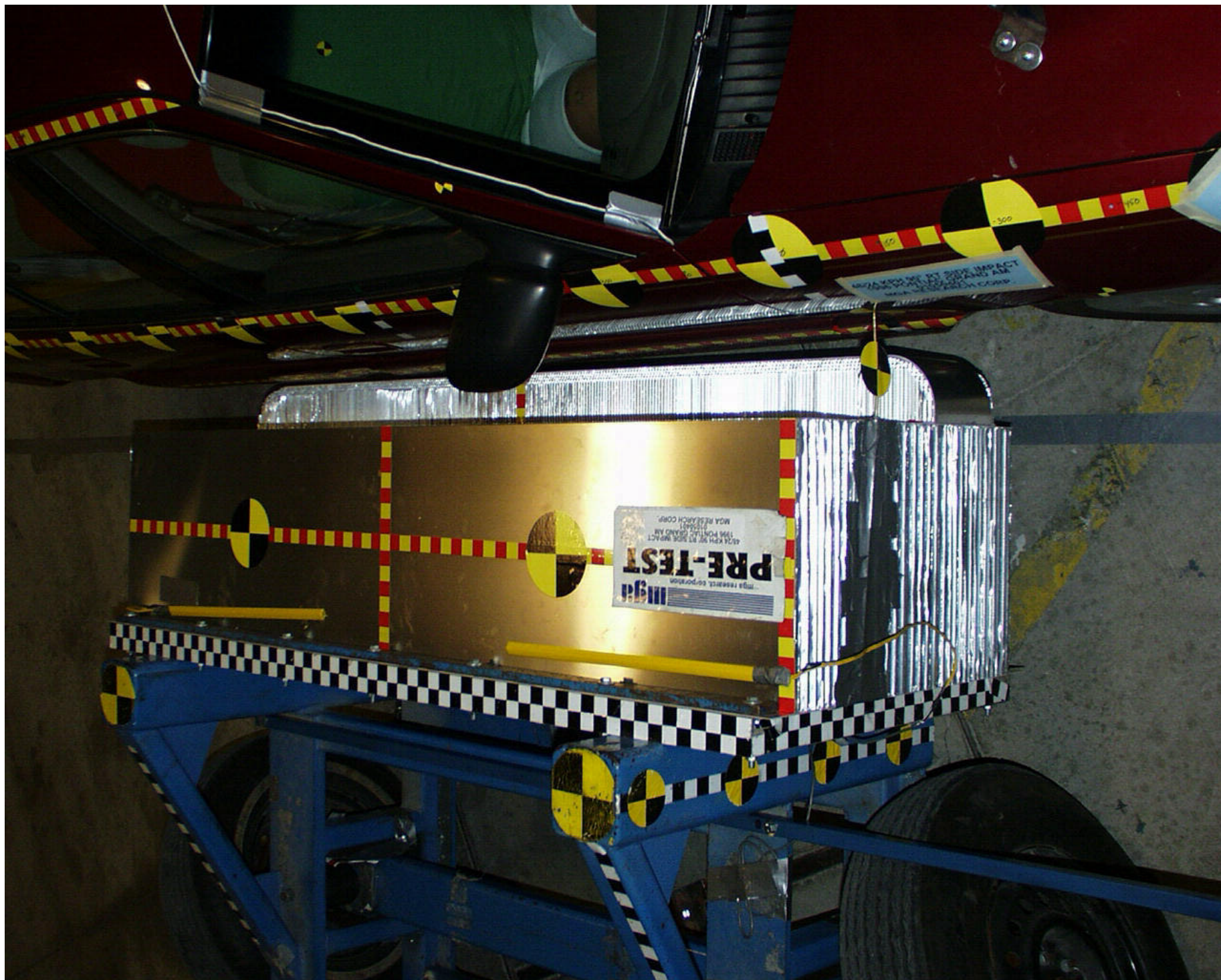
Photo No. A-7 - Pre-Test MDB Positioned Against Vehicle (overhead view)
