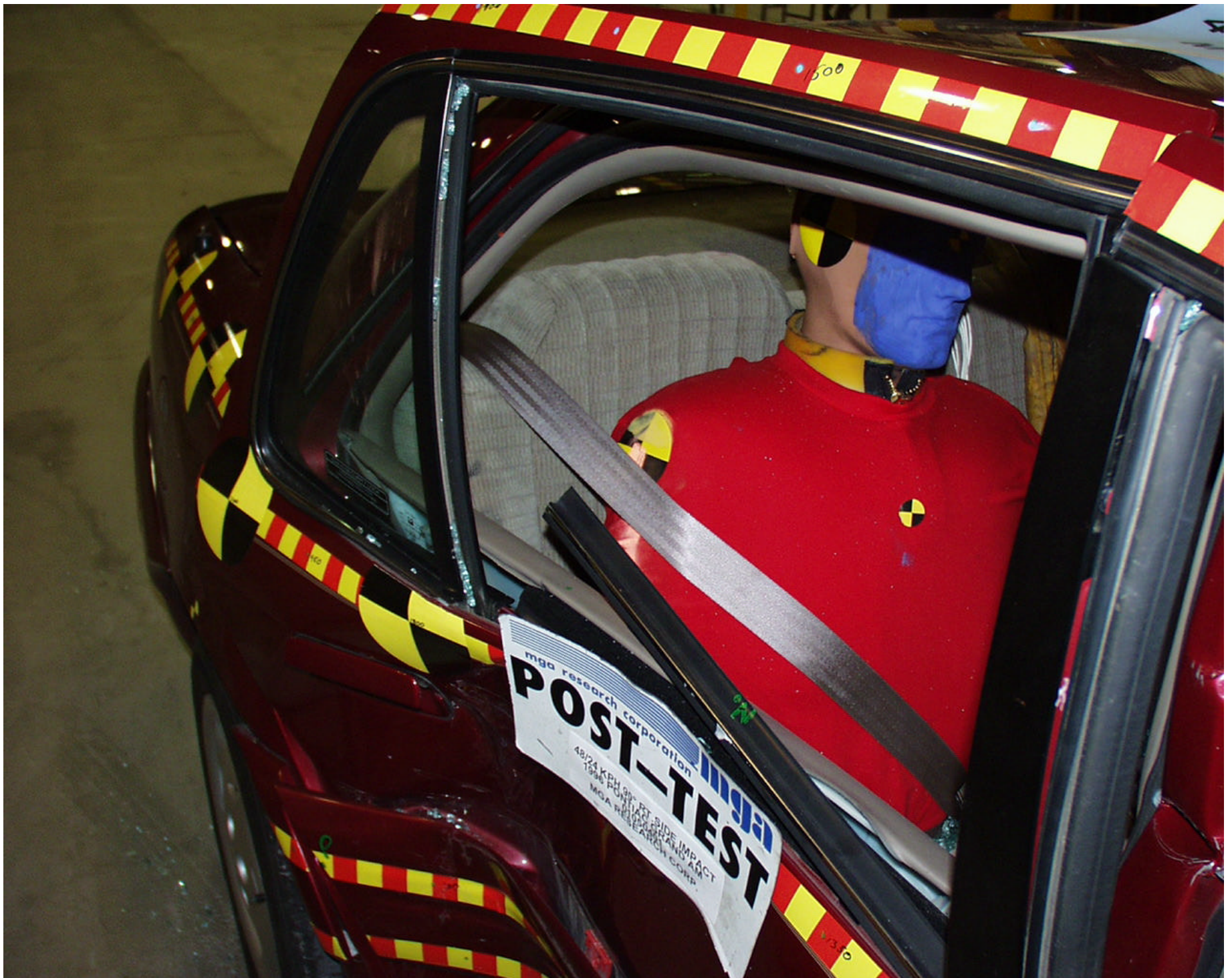
Photo No. A-32 - Post-Test RRP Dummy Shoulder and Door Top View
