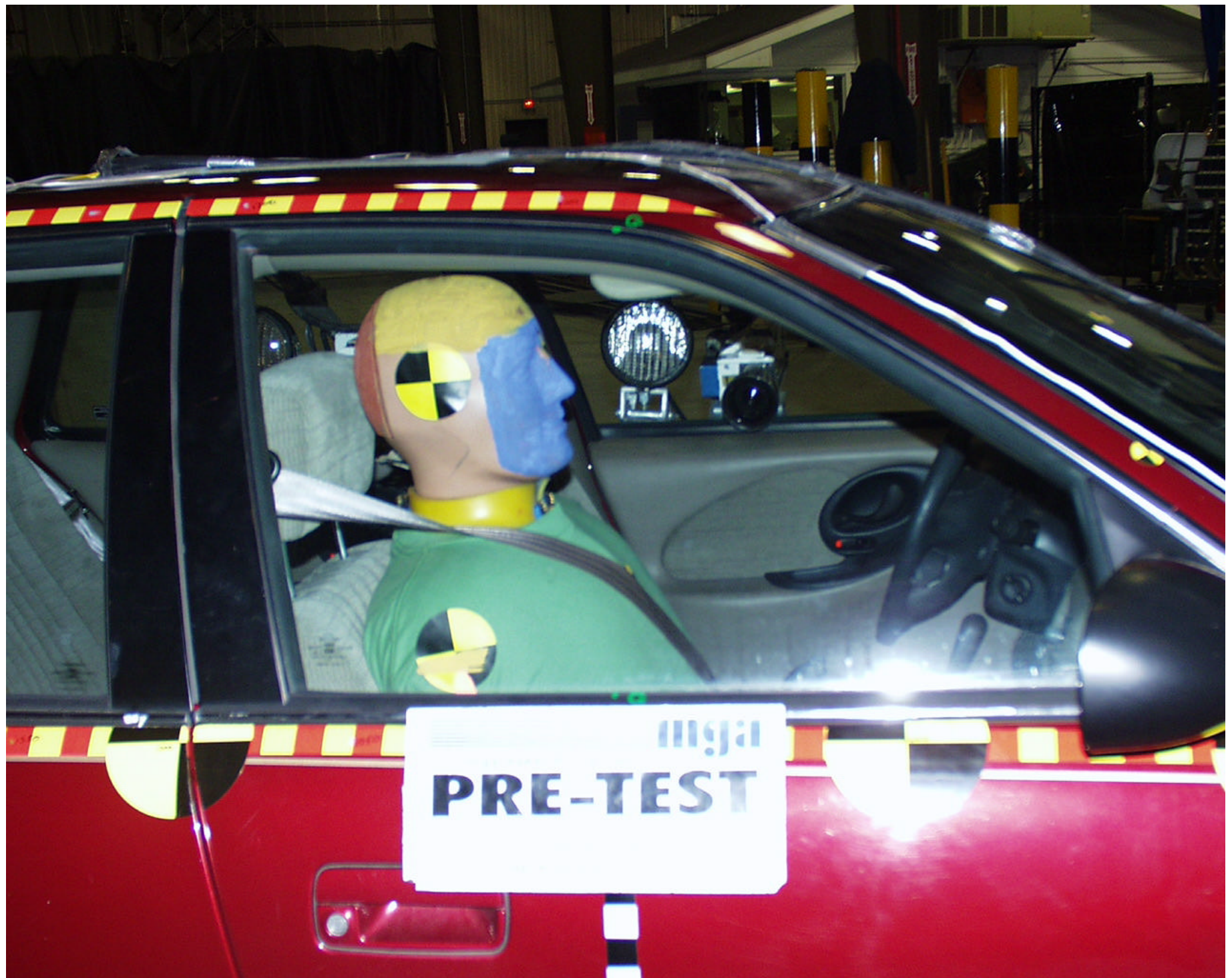
Photo No. A-18 - Pre-Test RFP Dummy Right Side View
