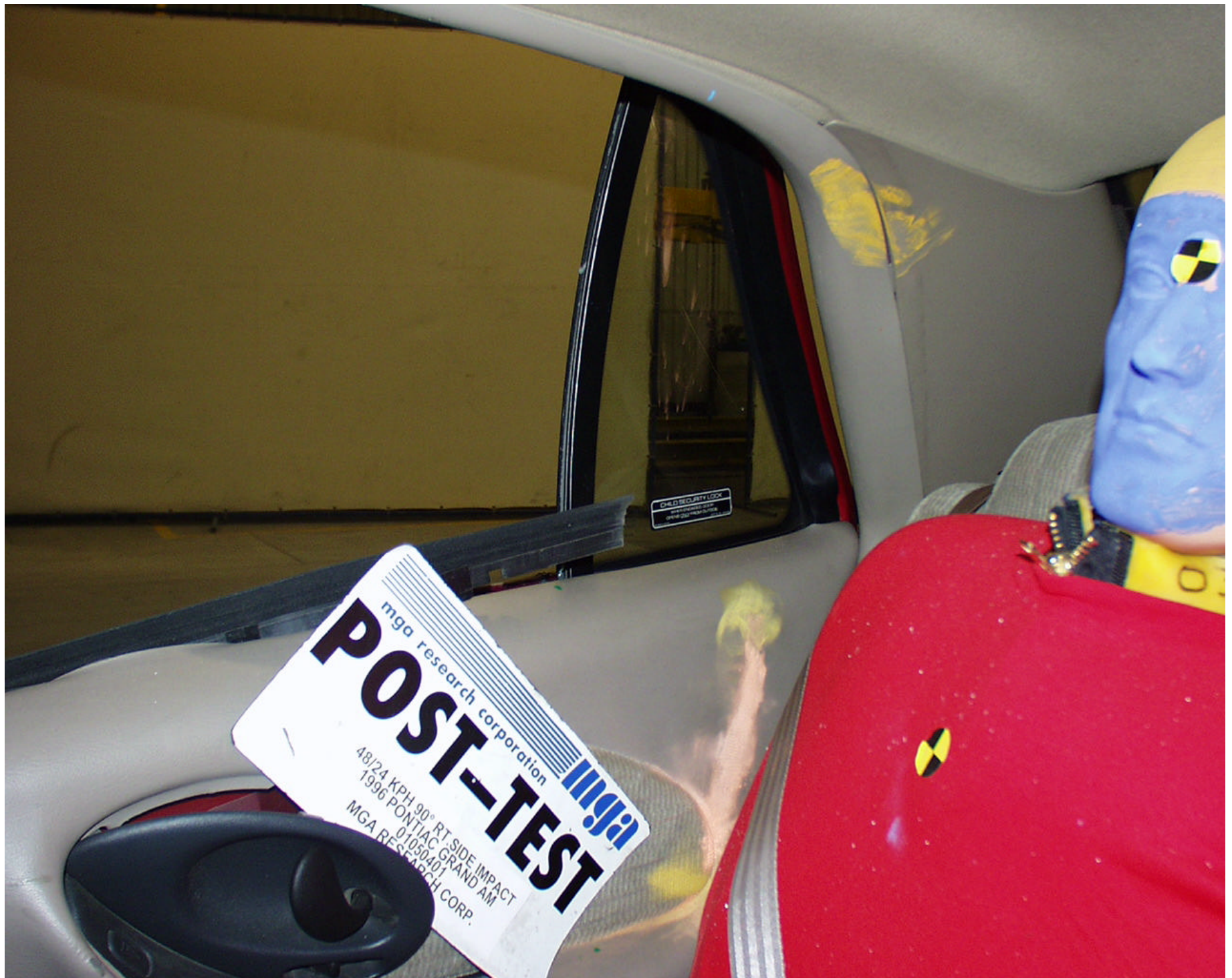
Photo No. A-34 - Post-Test RRP Dummy Head Contact
