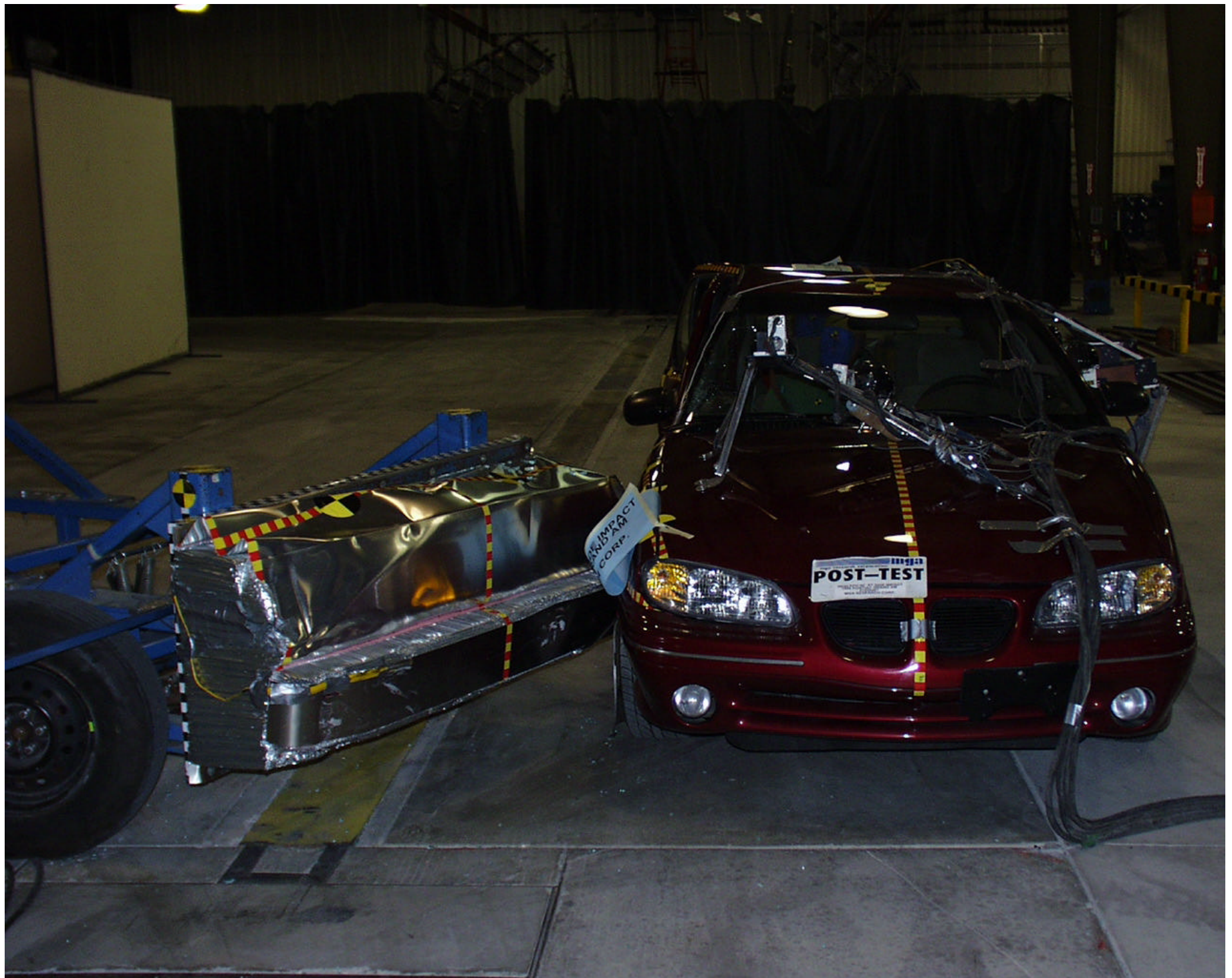
Photo No. A-8 - Post-Test MDB and Vehicle (right side)
