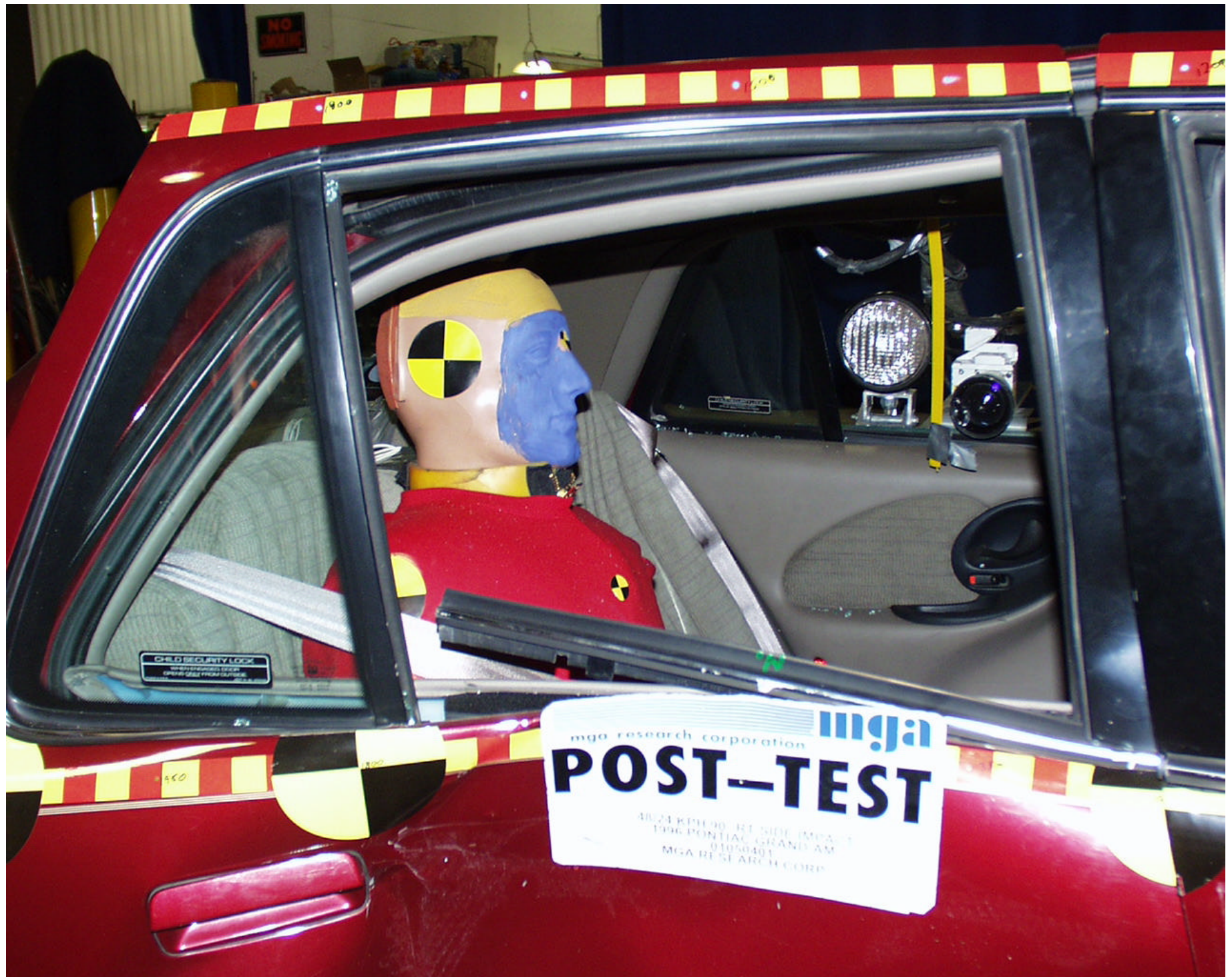
Photo No. A-27 - Post-Test RRP Dummy Right Side View
