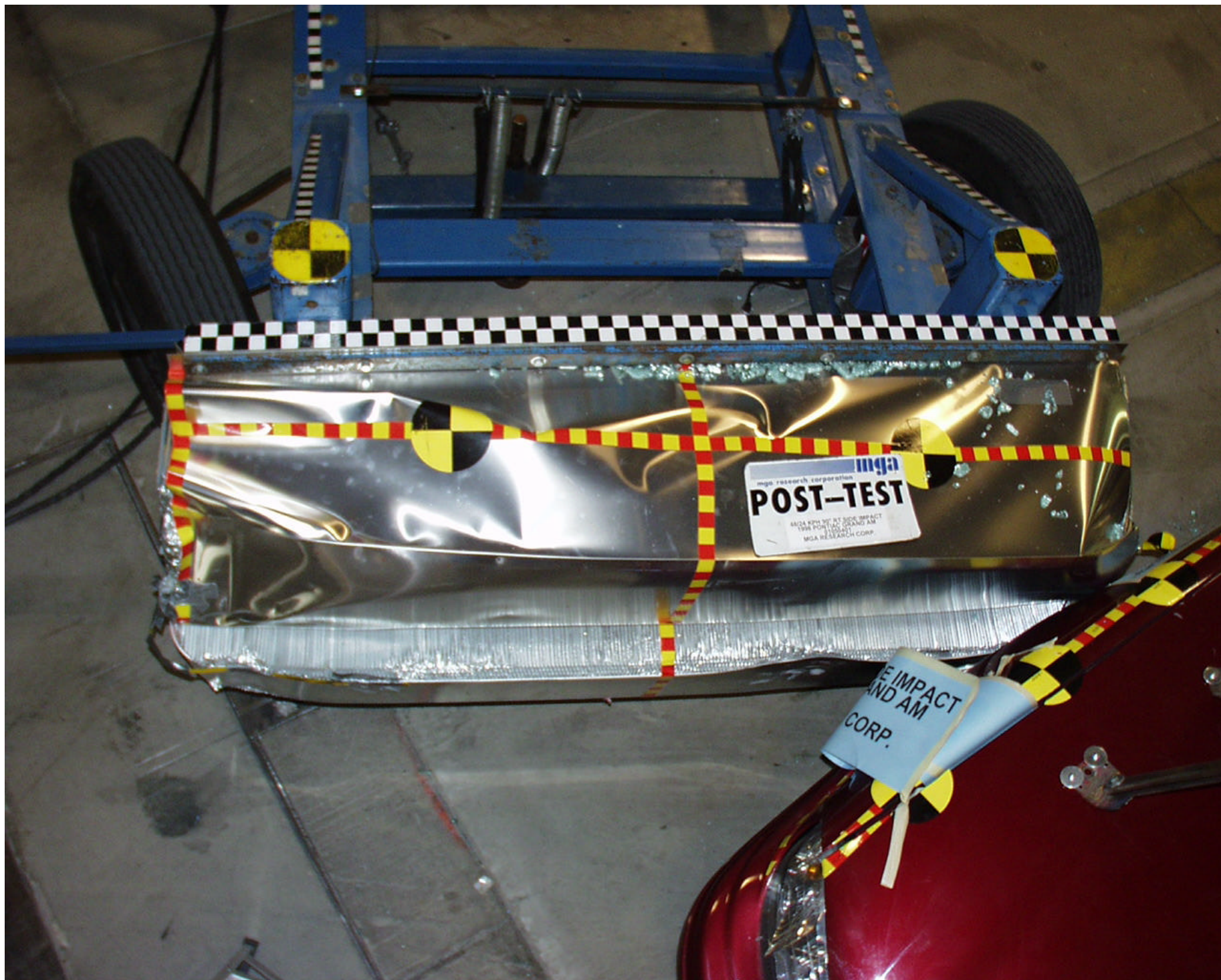
Photo No. A-9 – Post-Test MDB and Vehicle (overhead view)
