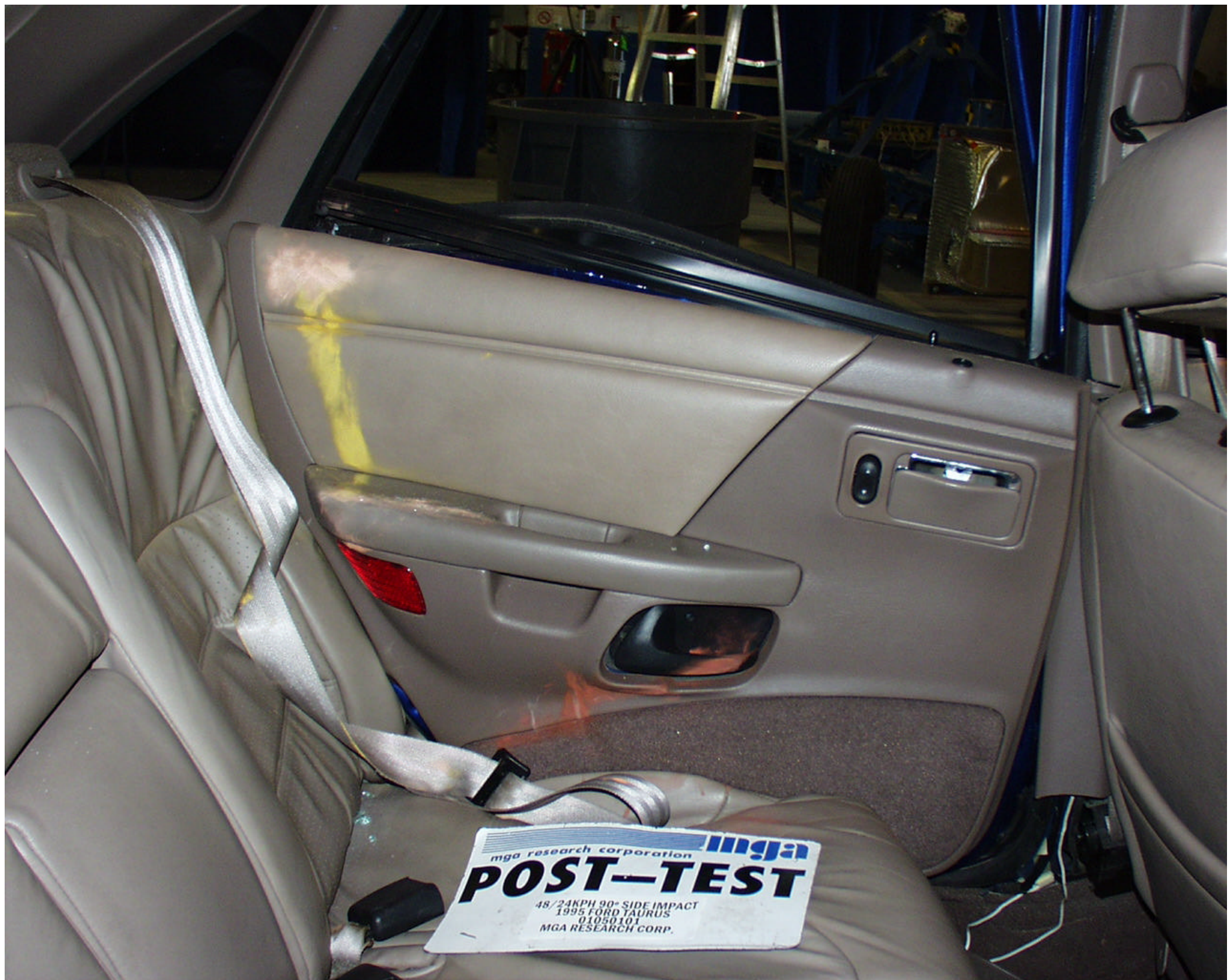
Photo No. A-34 - Post-Test Left Rear Passenger Contact
