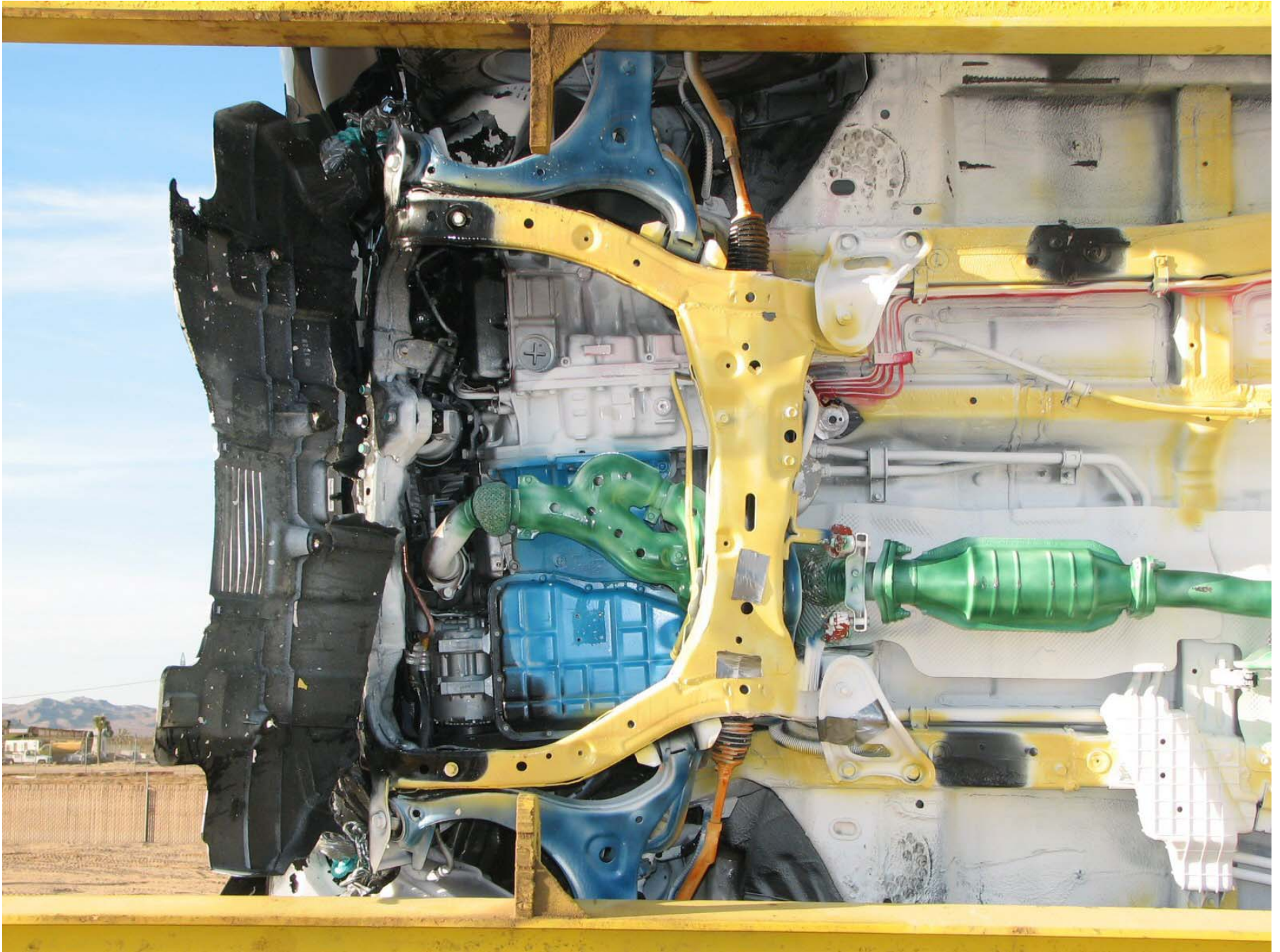
Figure A-25: Post-Test Front Underbody
