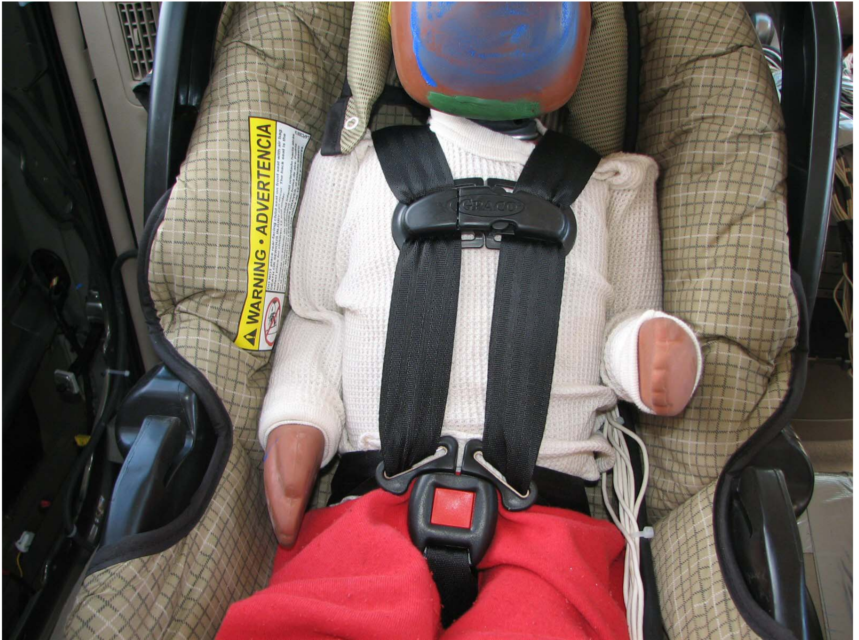
Figure D2-31: Post-Test Position 4 Front View (Seat Belt Position)
