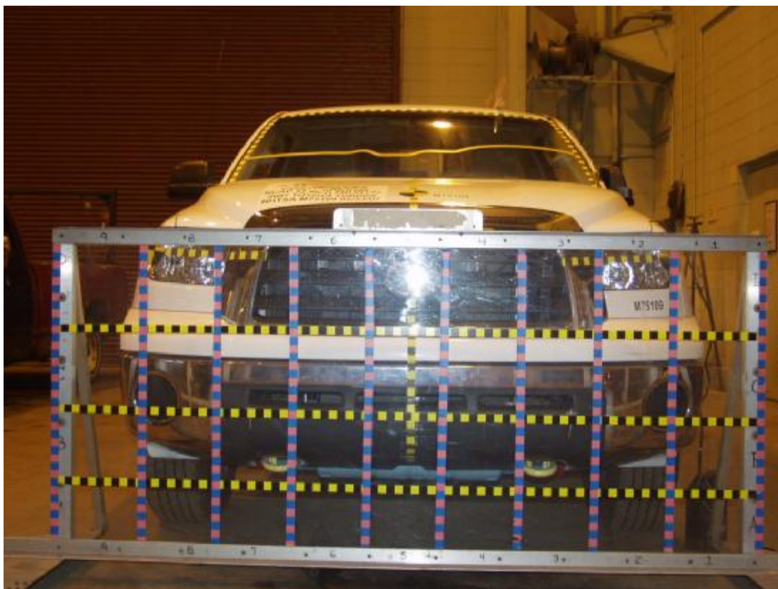
Figure A-1: Load Cell Locations
