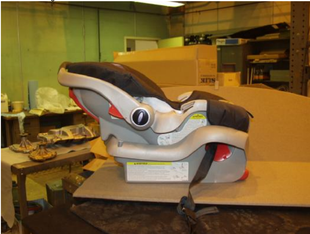
Figure 3-10: POST-TEST RIGHT SIDE VIEW OF POSITION 3CRS
