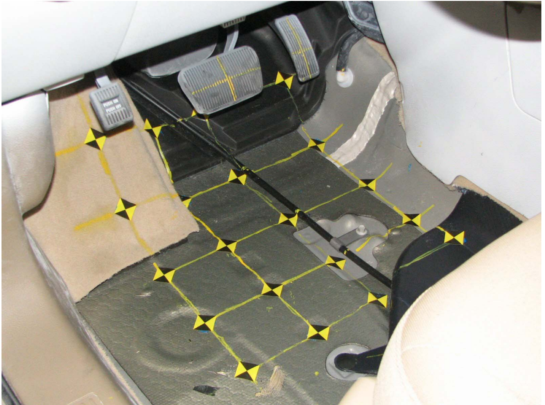
Figure A-40: Pre-Test Driver Side Floor Pan
