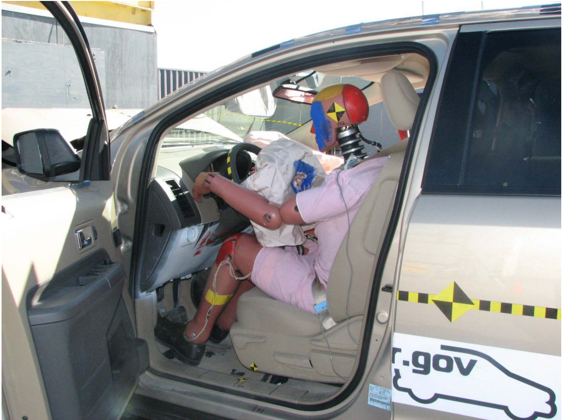
Figure A-35: Post-Test Driver Dummy (Door Open)
