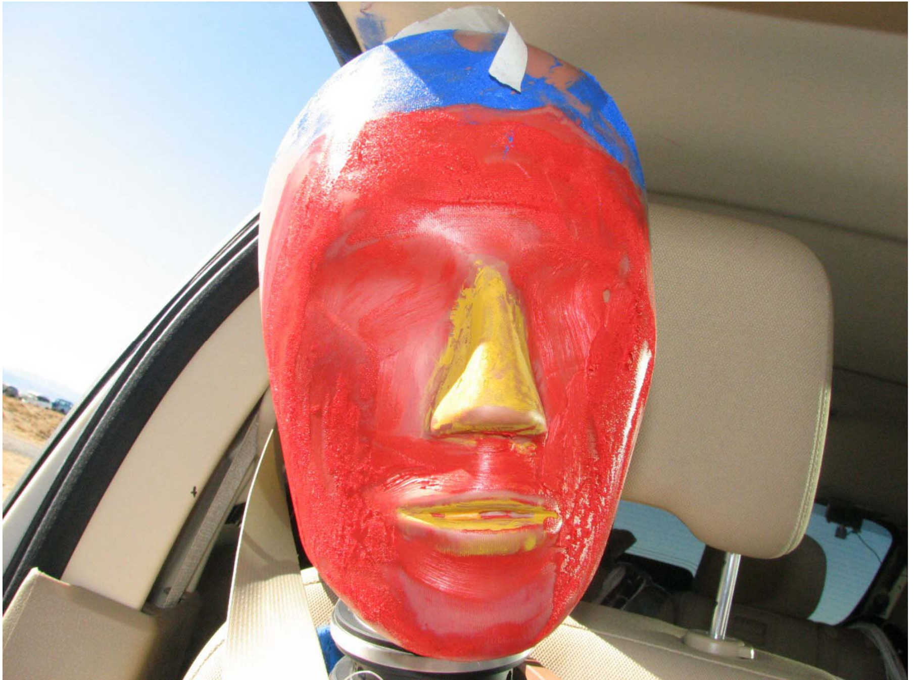
Figure A-56: Post-Test Passenger Dummy Head
