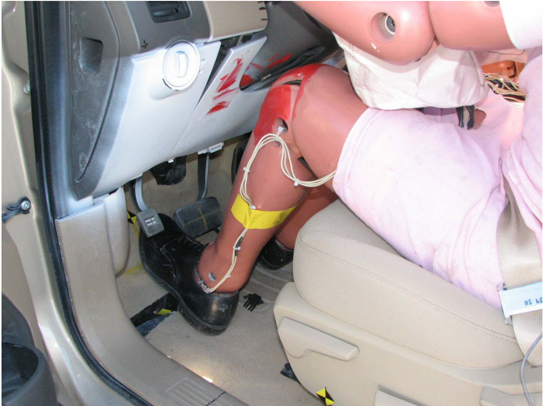
Figure A-37: Post-Test Driver Dummy Feet
