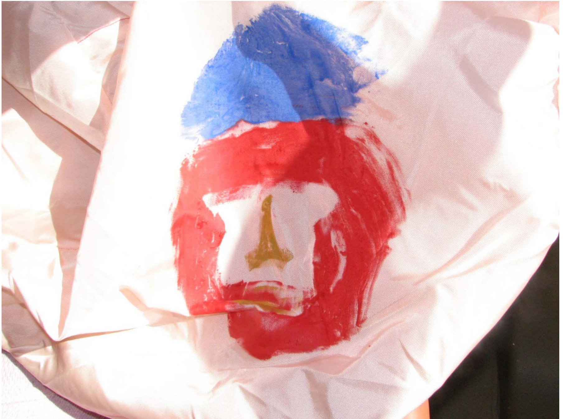
Figure A-57: Post-Test Passenger Dummy Airbag Contact
