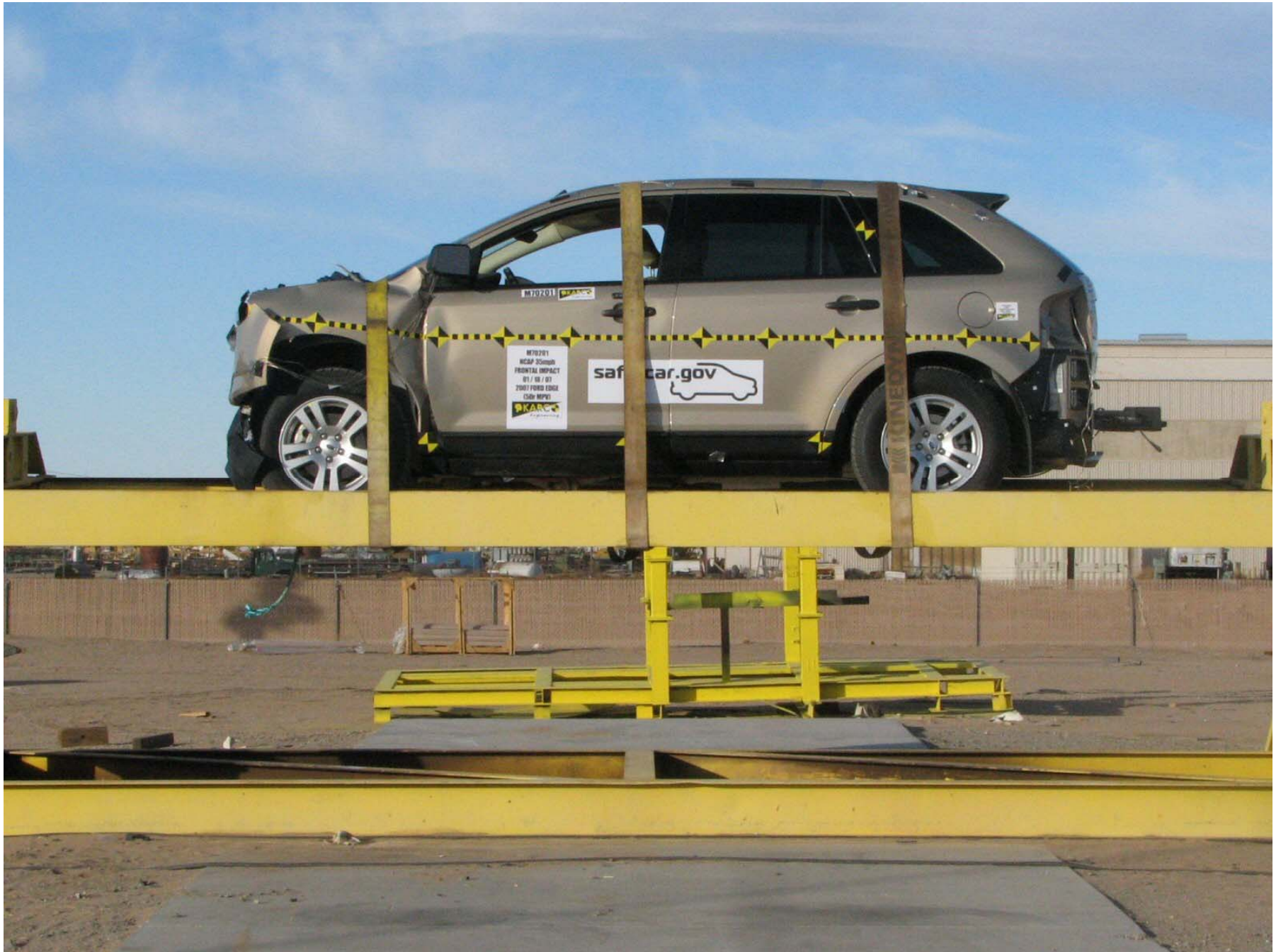
Figure A-58: Vehicle on Rollover Device (0°)
