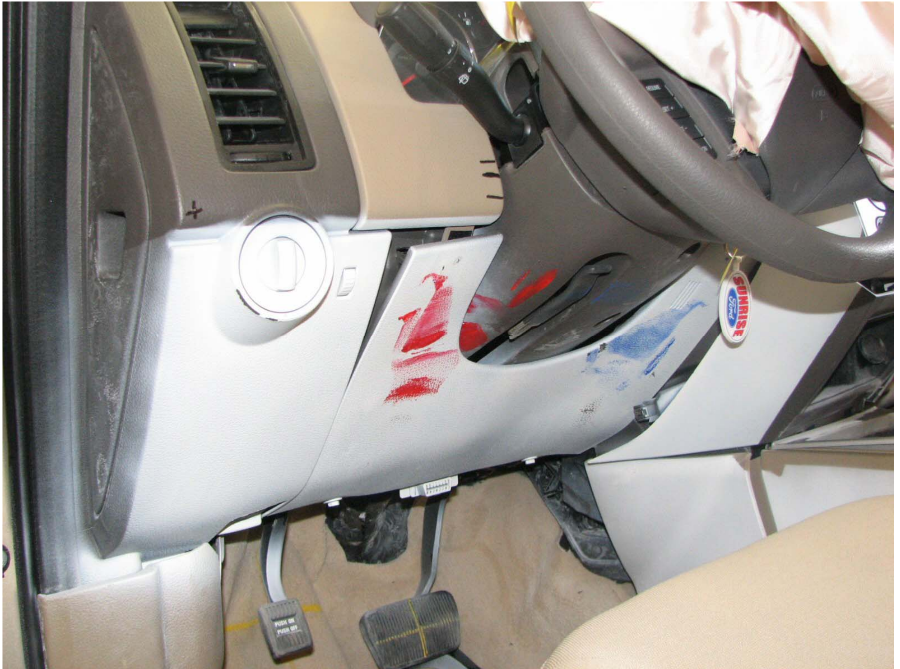
Figure A-39: Post-Test Driver Side Knee Bolster
