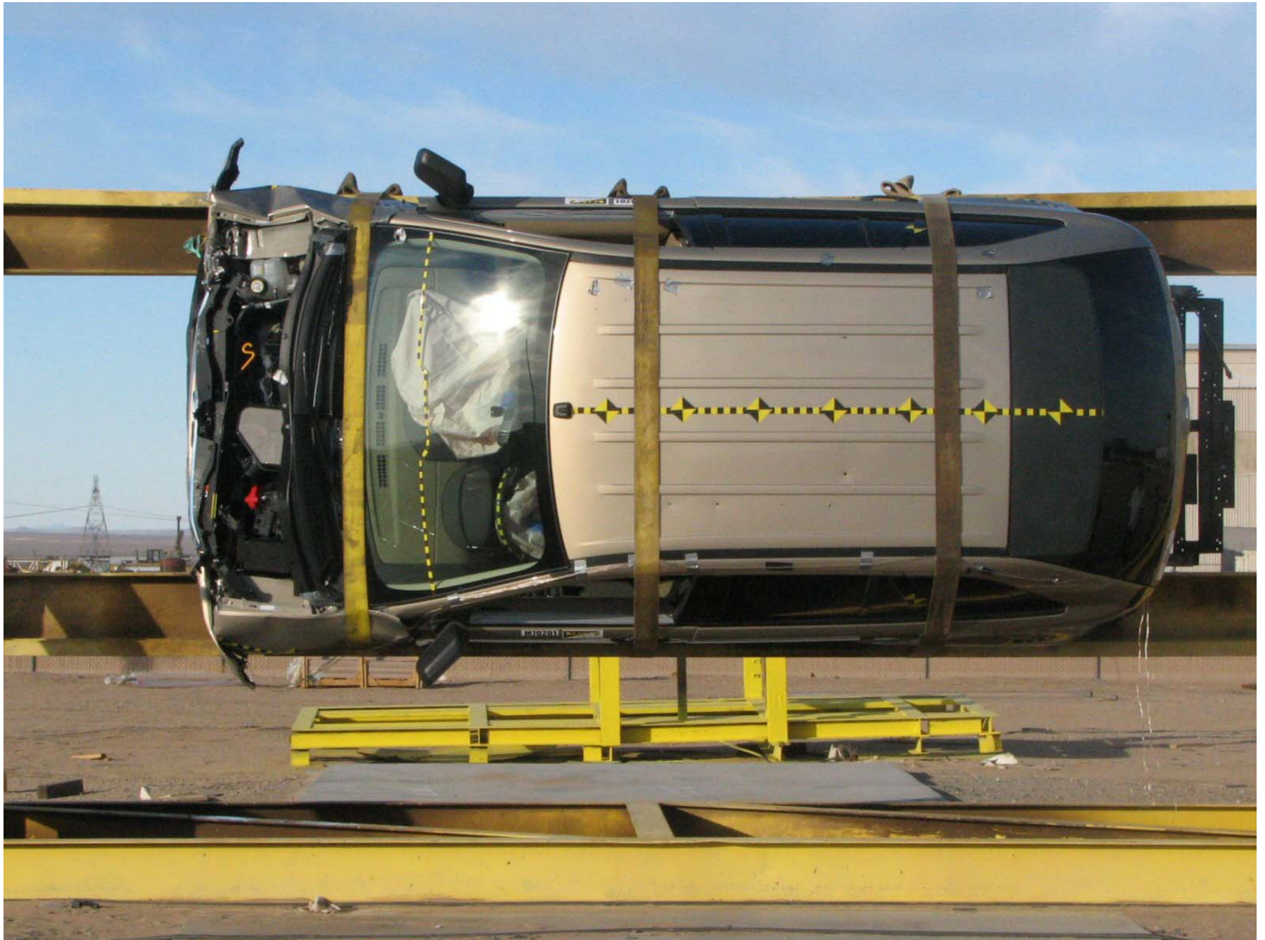
Figure A-59: Vehicle on Rollover Device (90°)
