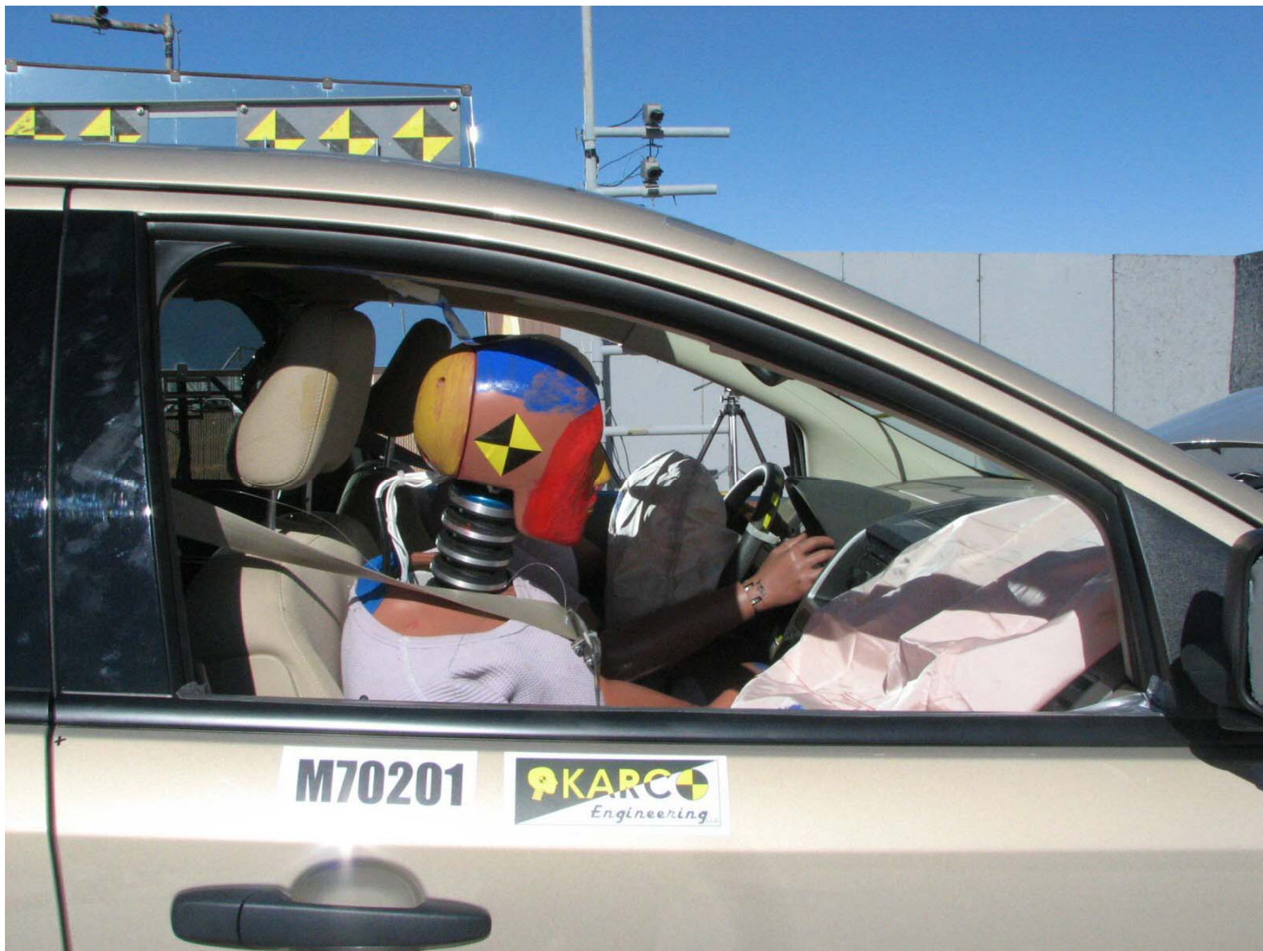
Figure A-47: Post-Test Passenger Dummy (Through Window)
