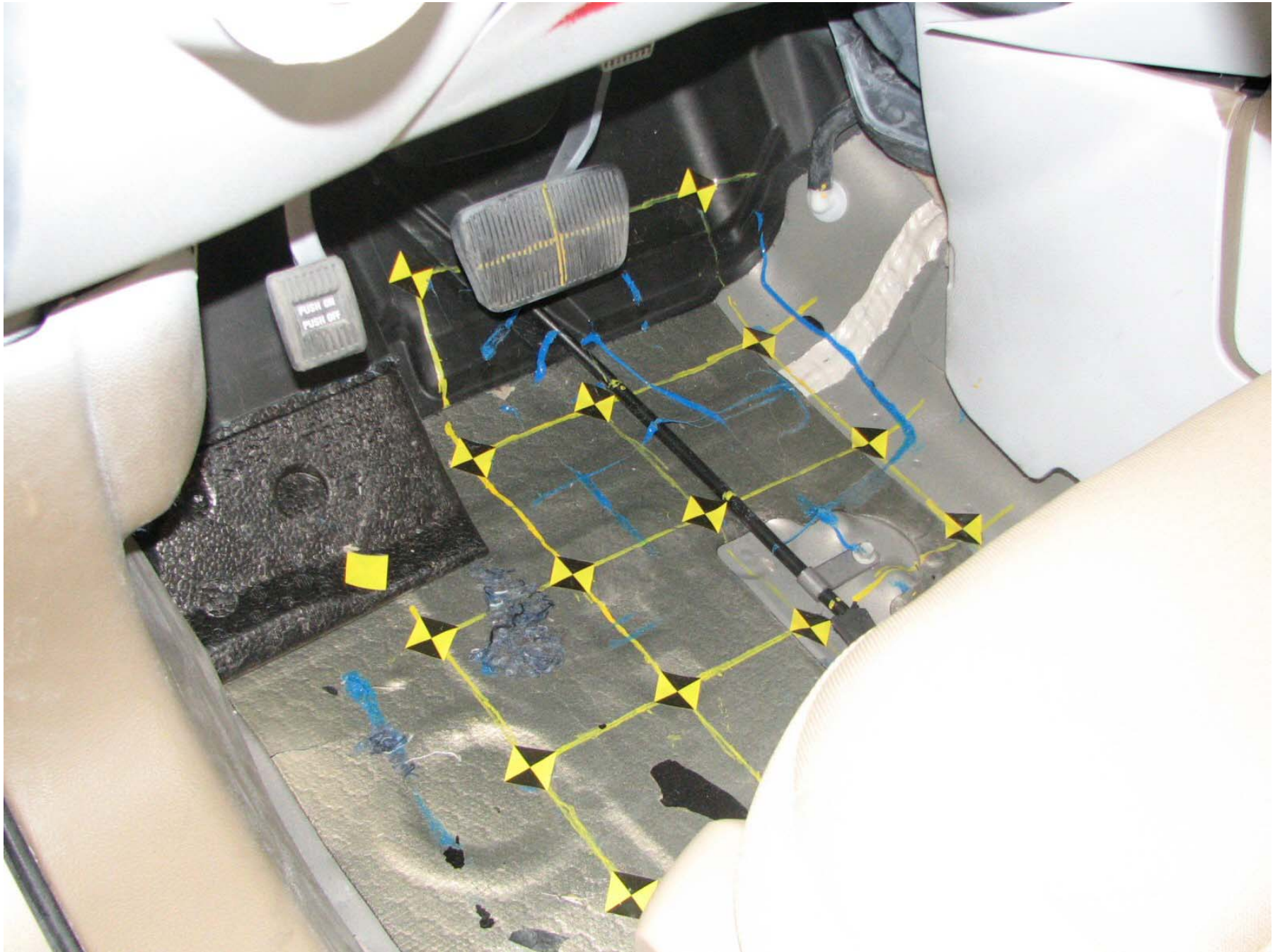
Figure A-41: Post-Test Driver Side Floor Pan
