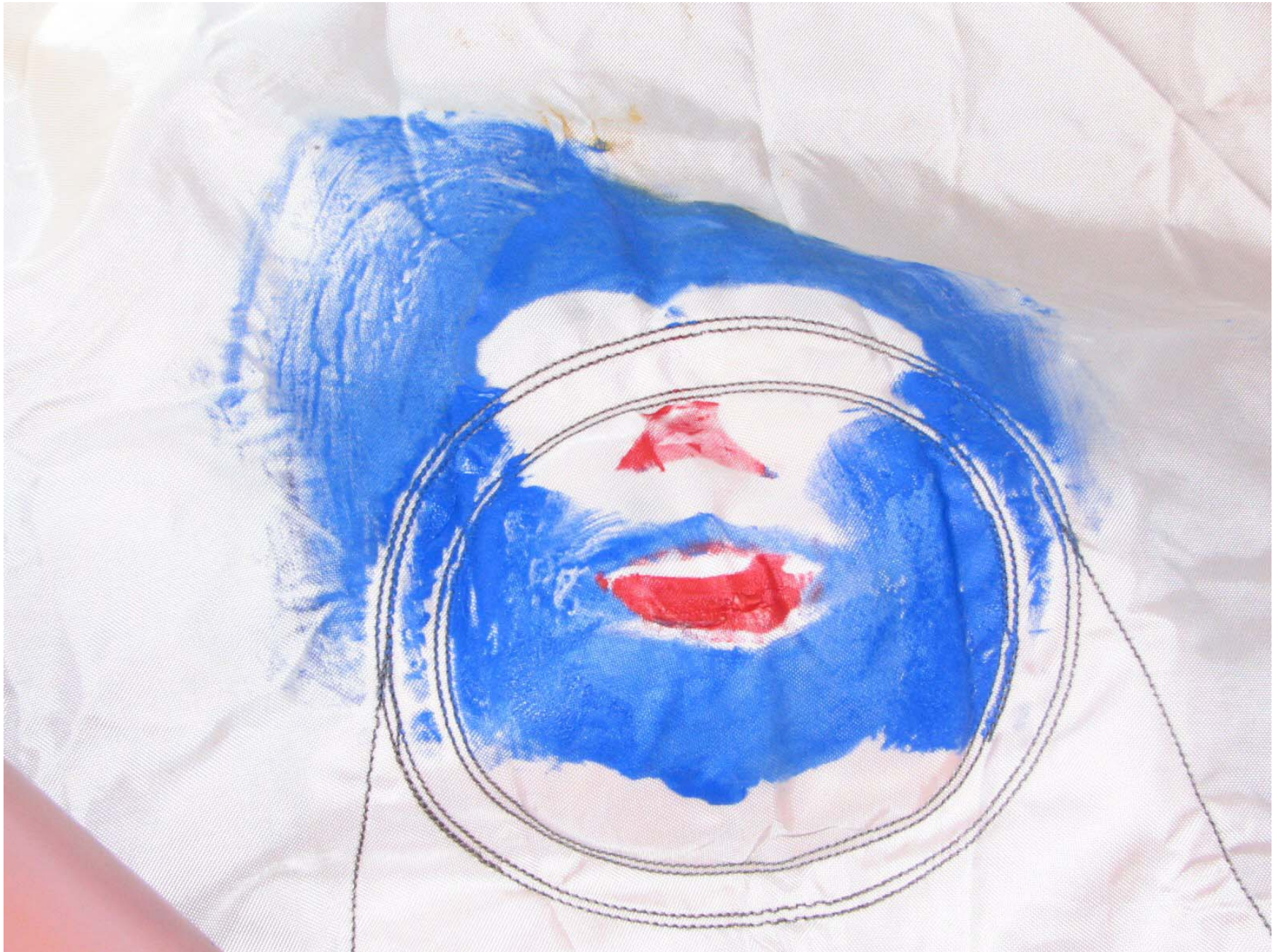
Figure A-43: Post-Test Driver Dummy Airbag Contact
