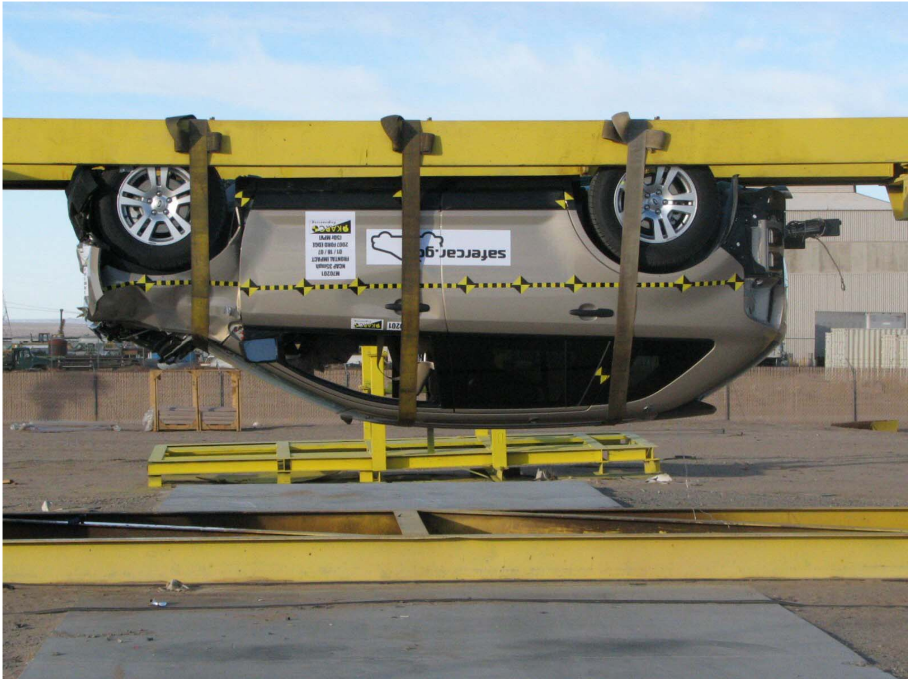
Figure A-60: Vehicle on Rollover Device (180°)
