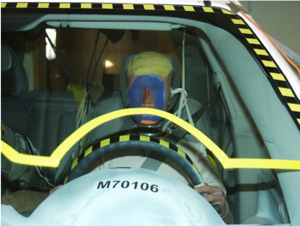
Figure A-30: Pre-Test Driver Head Location
