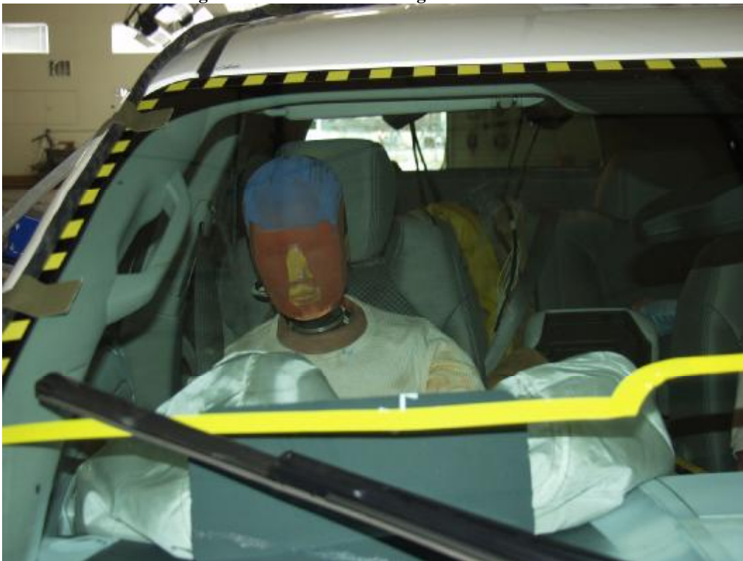
Figure A-45: Post-Test Passenger Head Location
