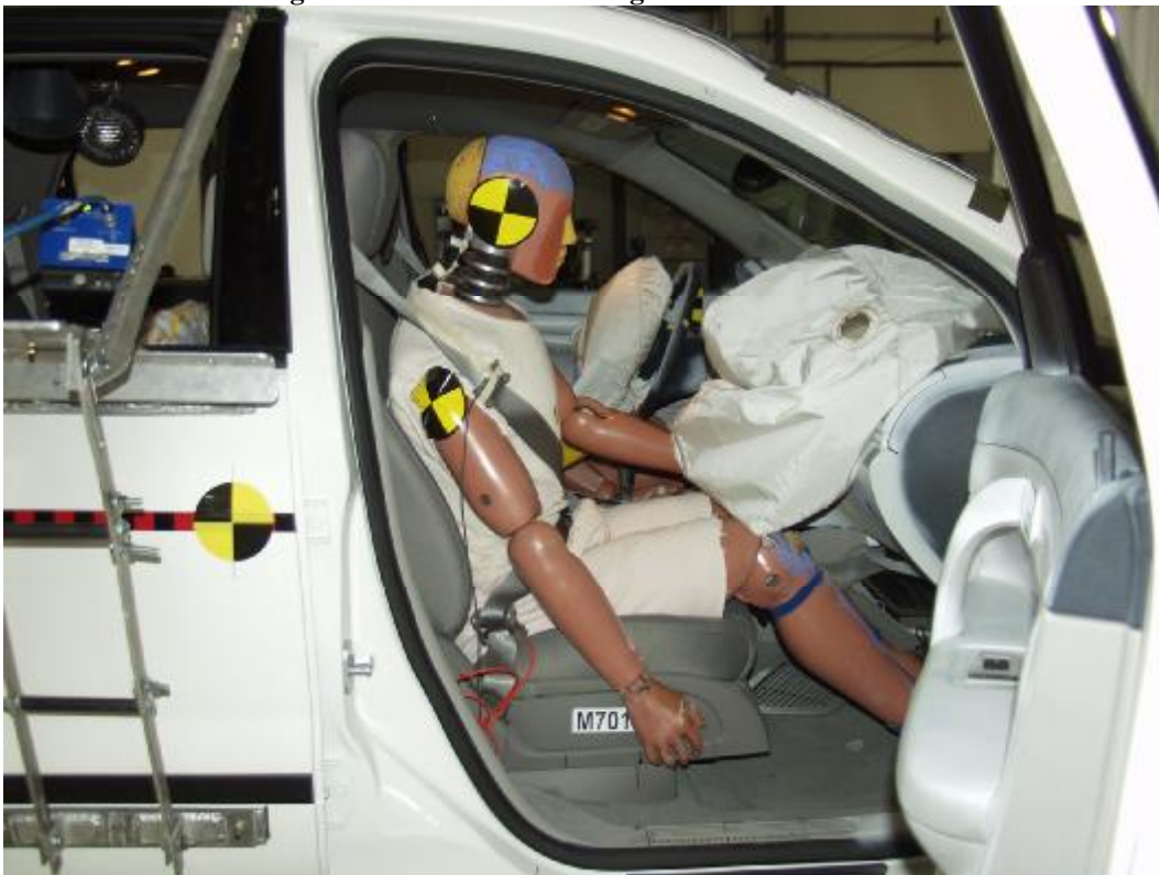
Figure A-49: Post-Test Passenger and Interior View
