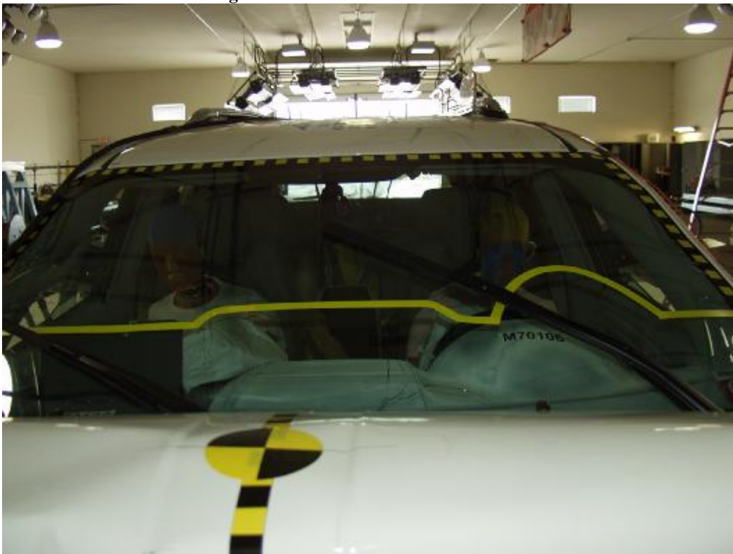
Figure A-19: Post-Test Windshield View
