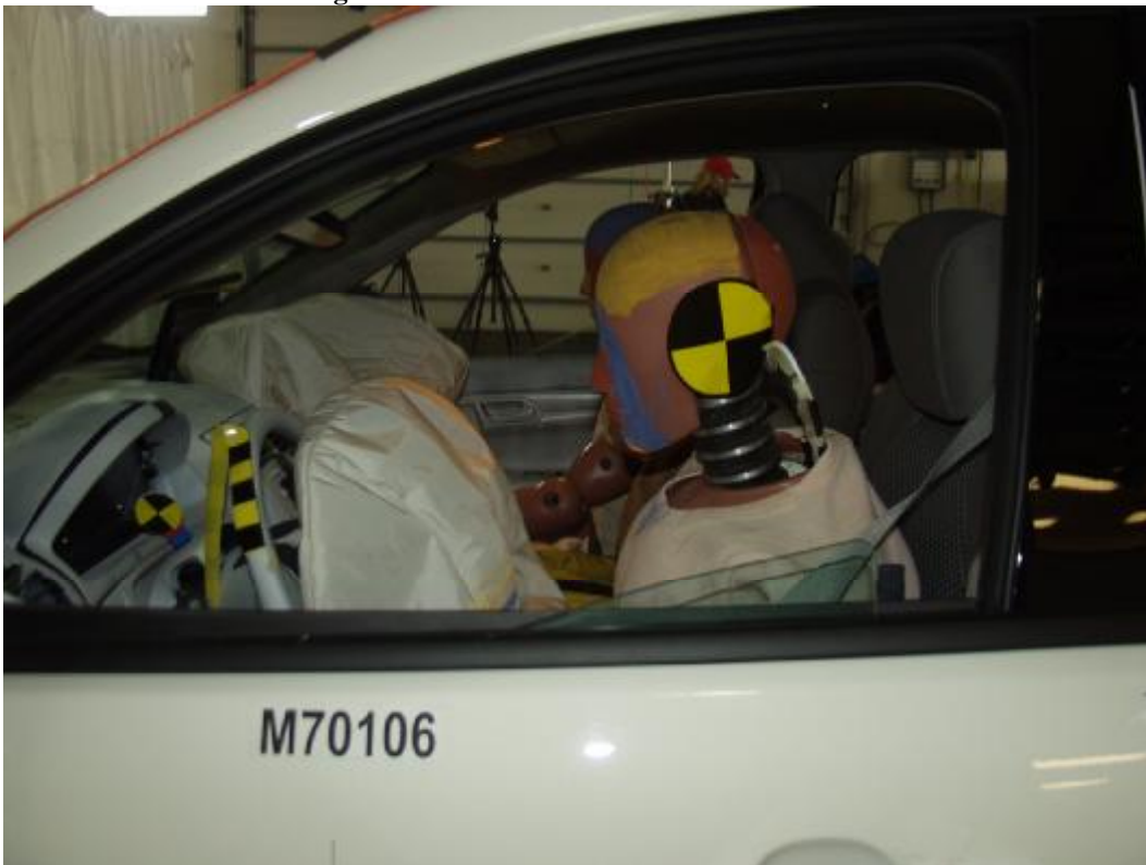
Figure A-33: Post-Test Driver Position View
