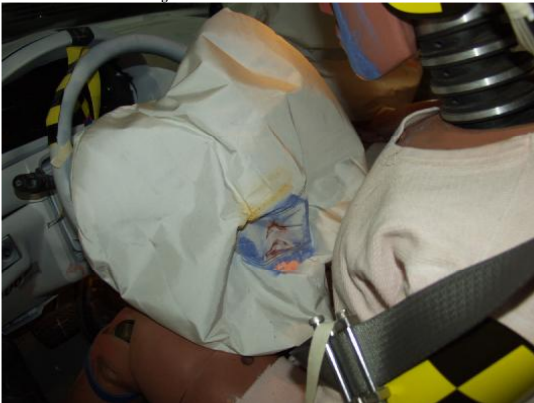
Figure A-43: Post-Test Driver Contact to Airbag
