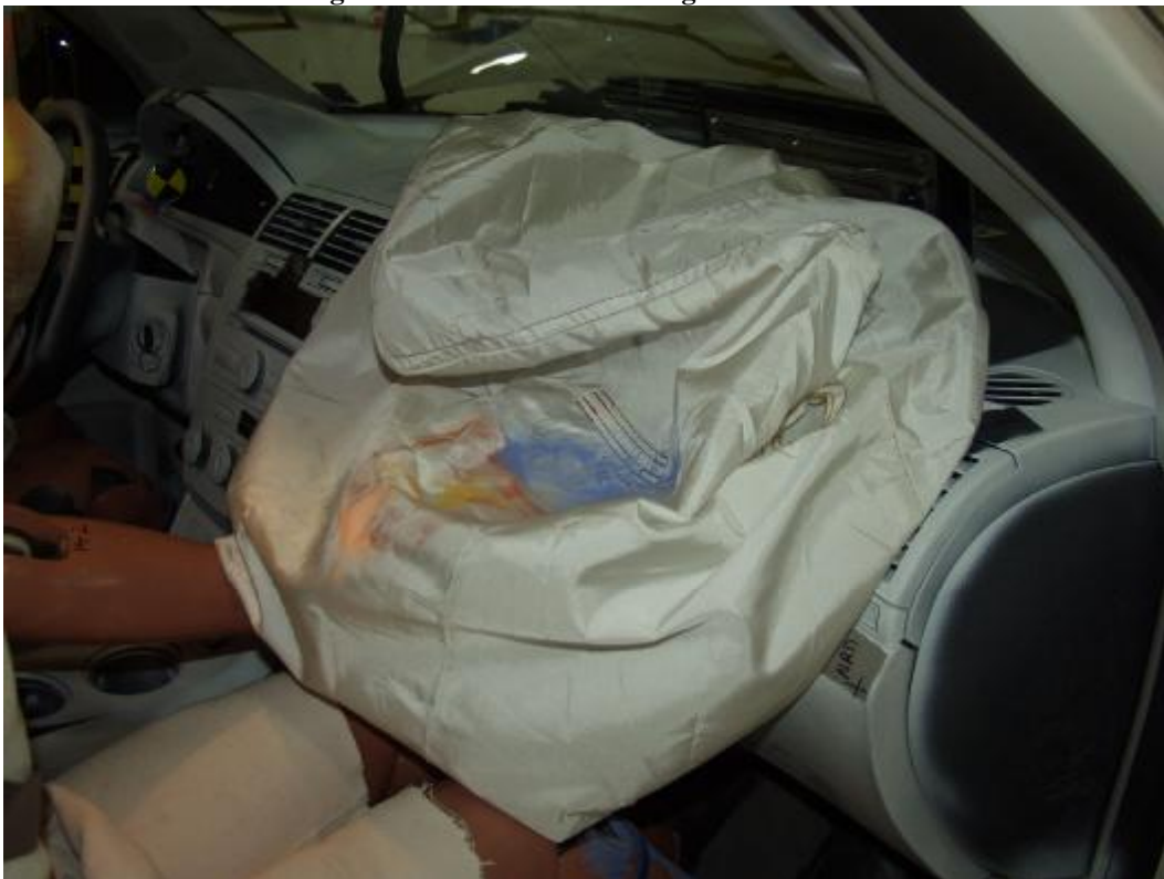
Figure A-57: Post-Test Passenger Contact to Airbag
