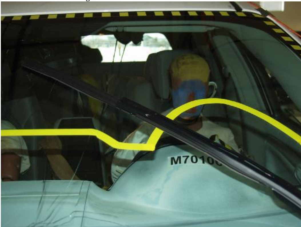
Figure A-31: Post-Test Driver Head Location
