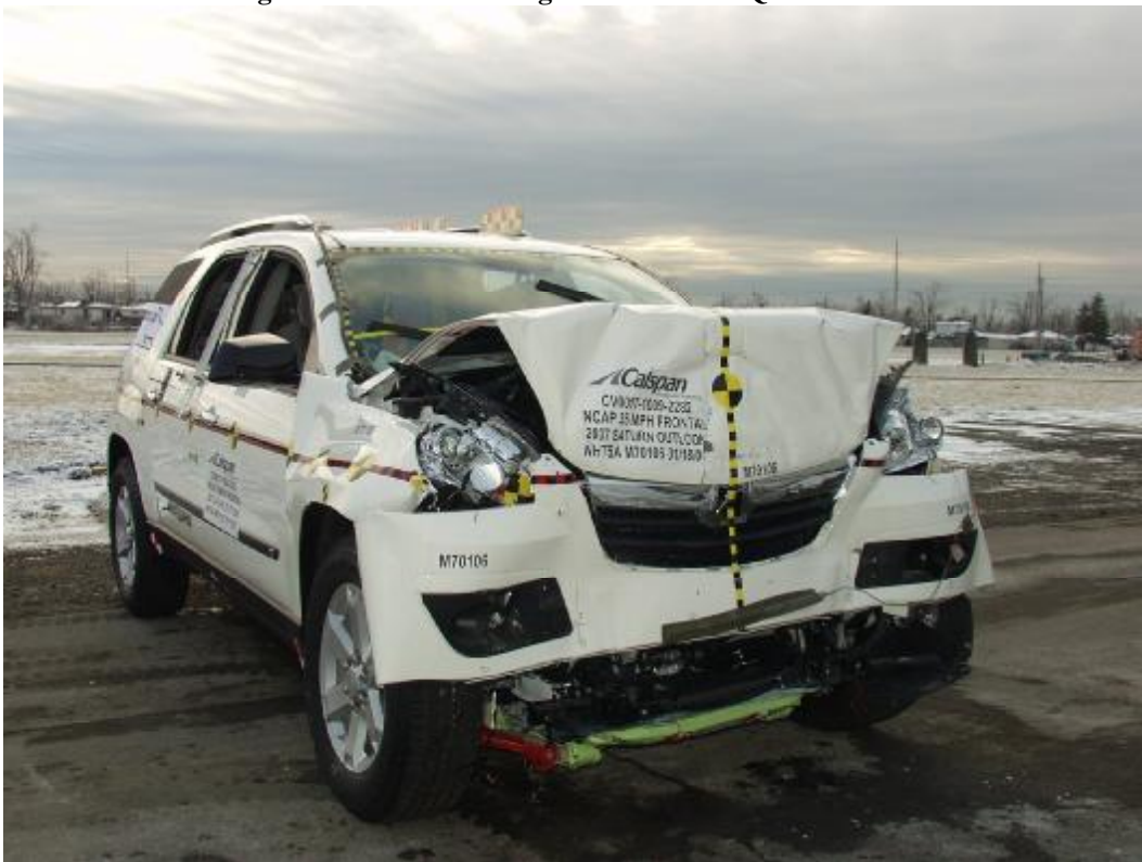
Figure A-13: Post-Test Right Front Three-Quarter View
