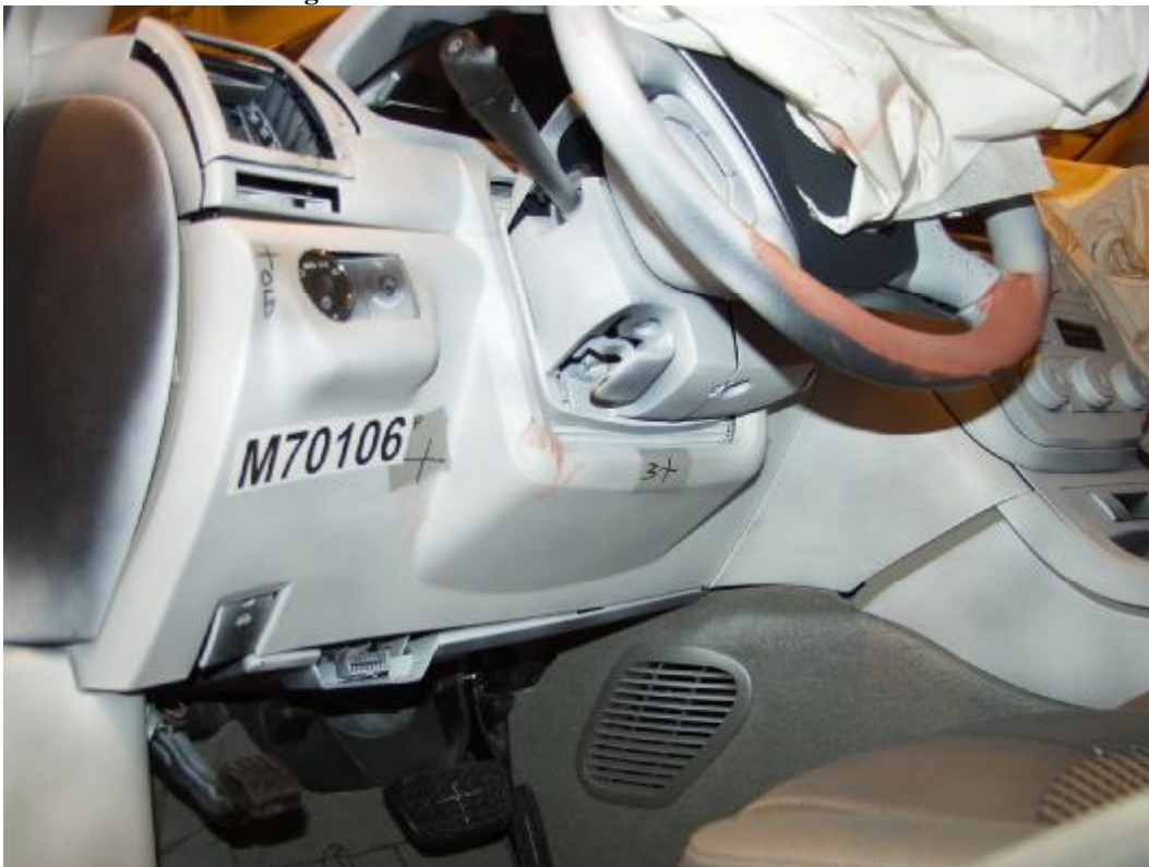
Figure A-39: Post-Test Driver Knee Bolster View
