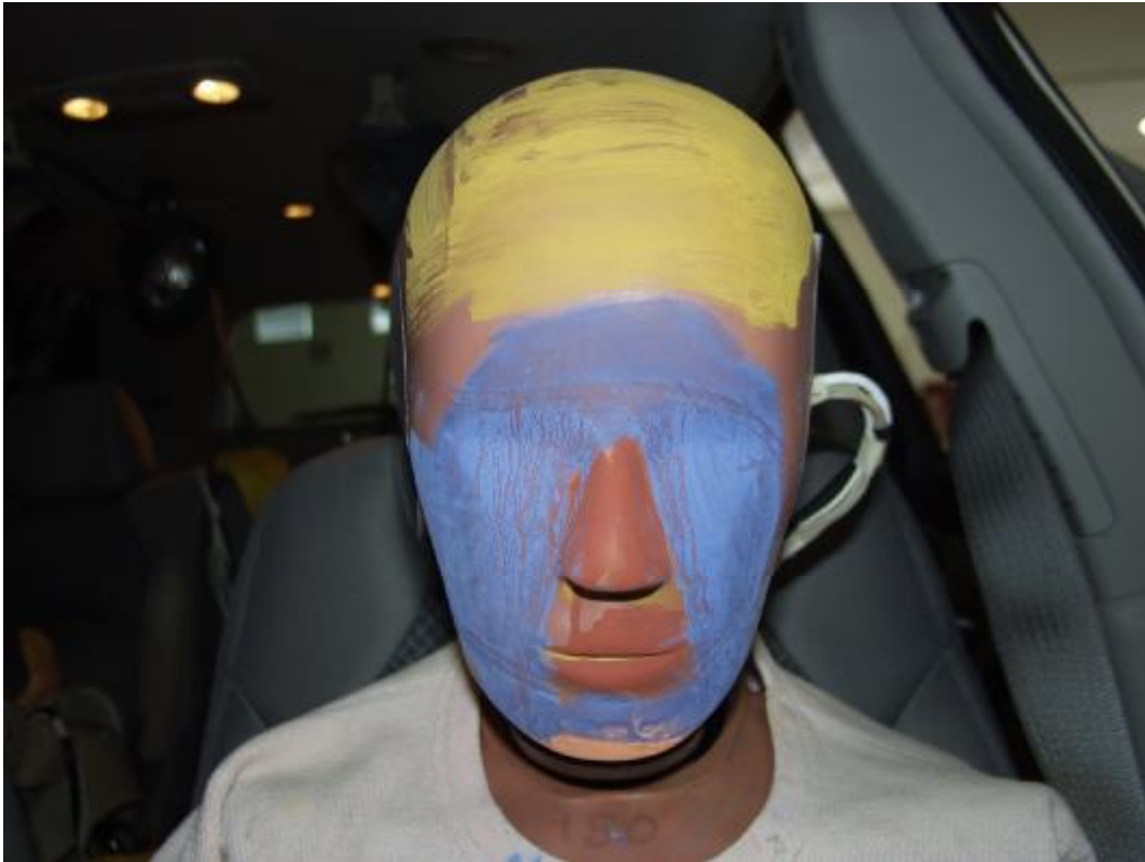
Figure A-42: Post-Test Driver Head View
