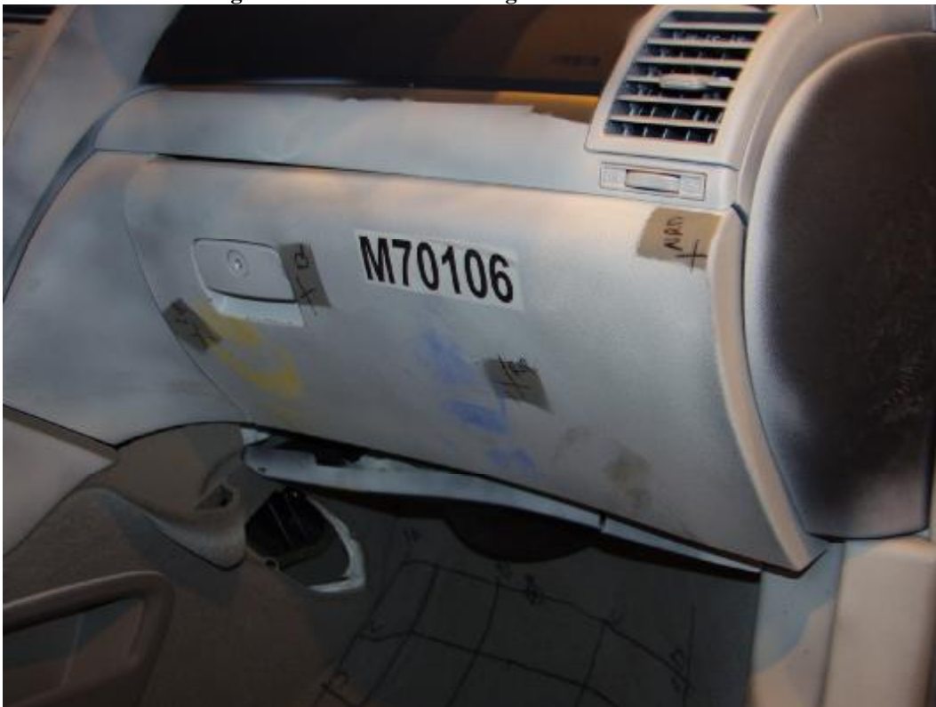
Figure A-53: Post-Test Passenger Knee Bolster View
