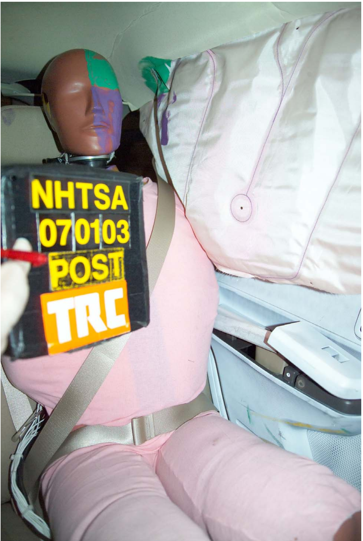
Figure A-52 Post-Test Left View of Rear SID HIII and Door Clearance
