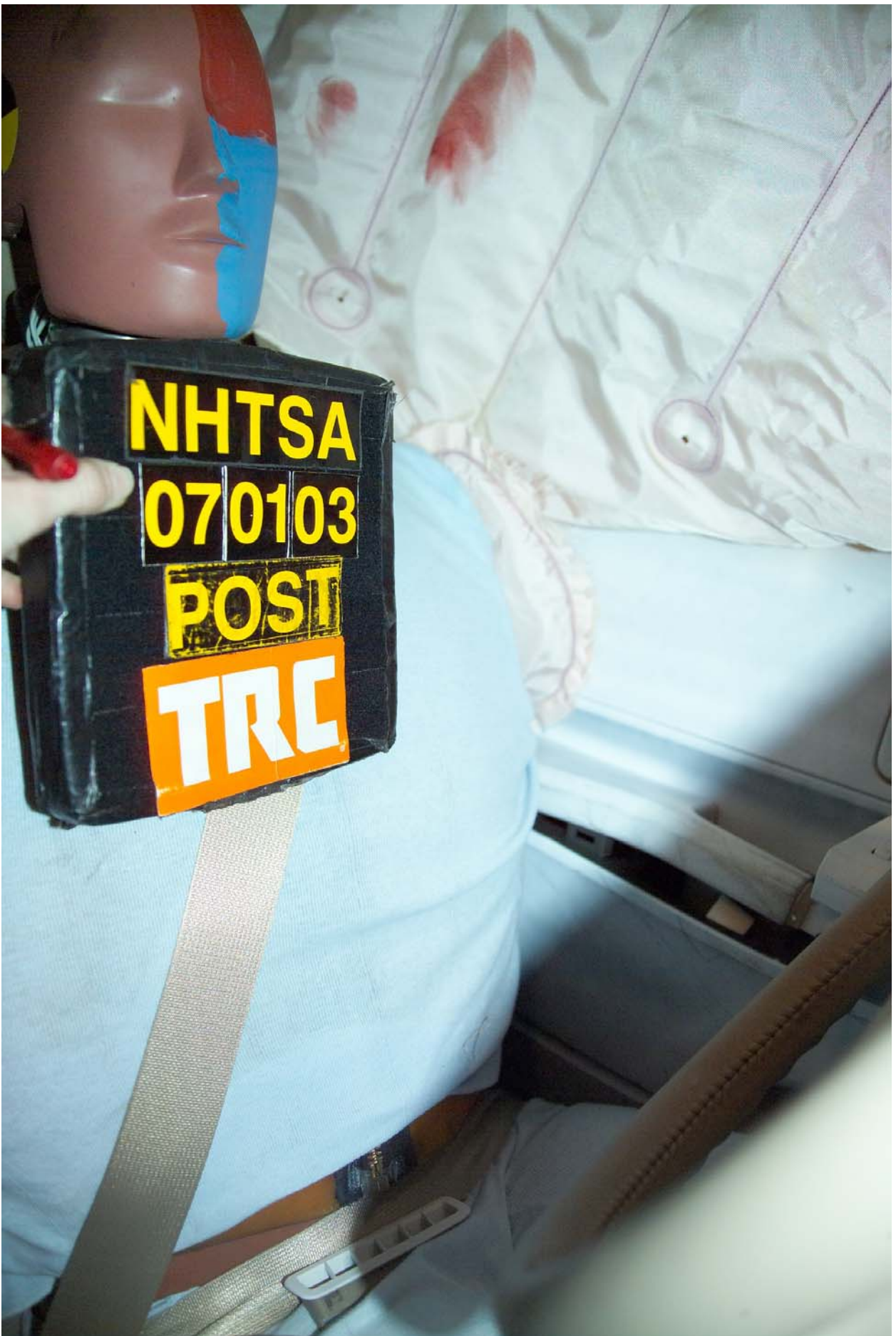
Figure A-47 Post-Test Left View of Front SID HIII and Door Clearance
