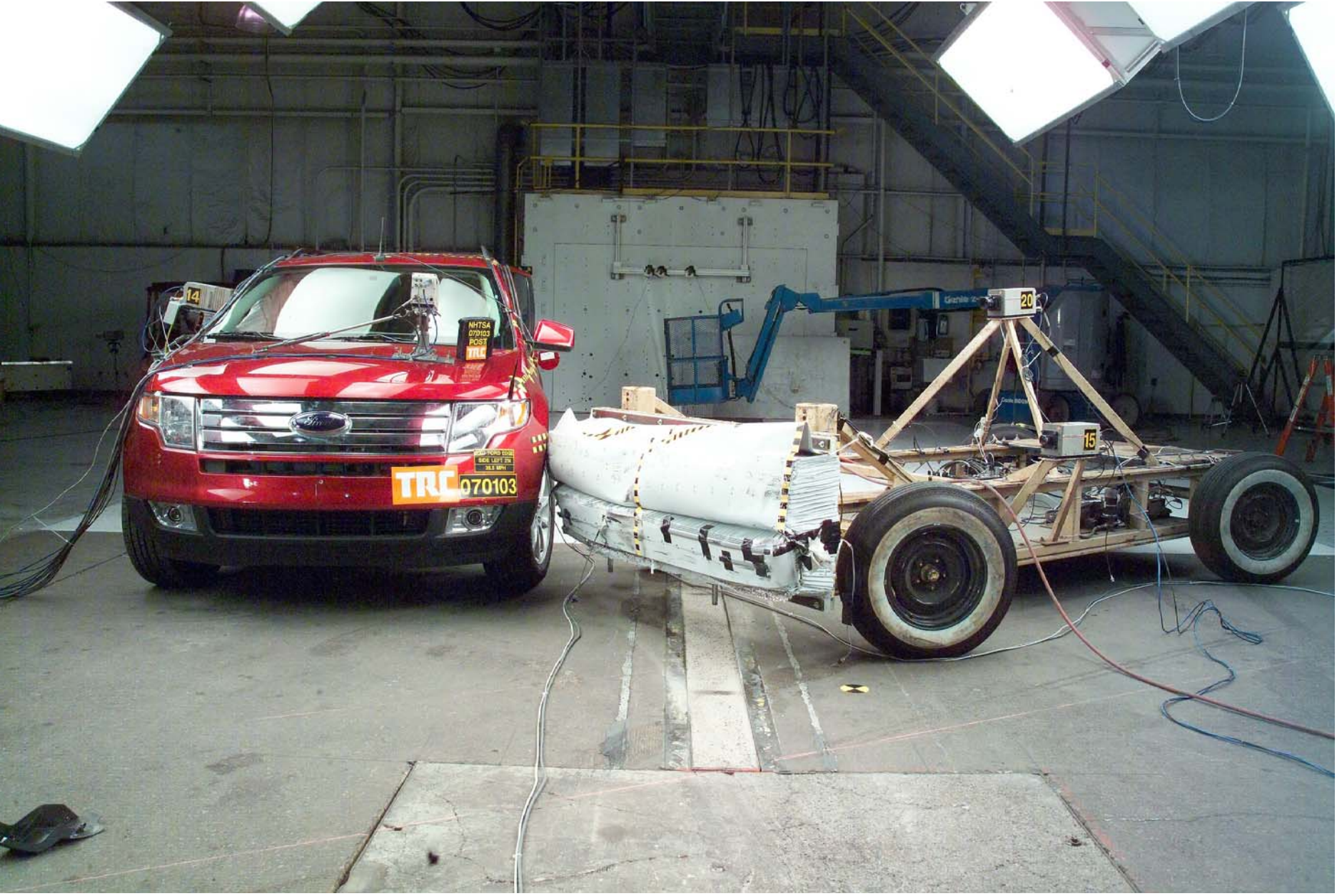
Figure A-64 Post-Test Left Side View of MDB With Impactor Face in Position
