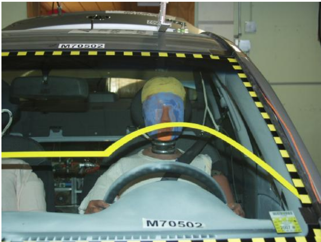
Figure A-30: Pre-Test Driver Head Location
