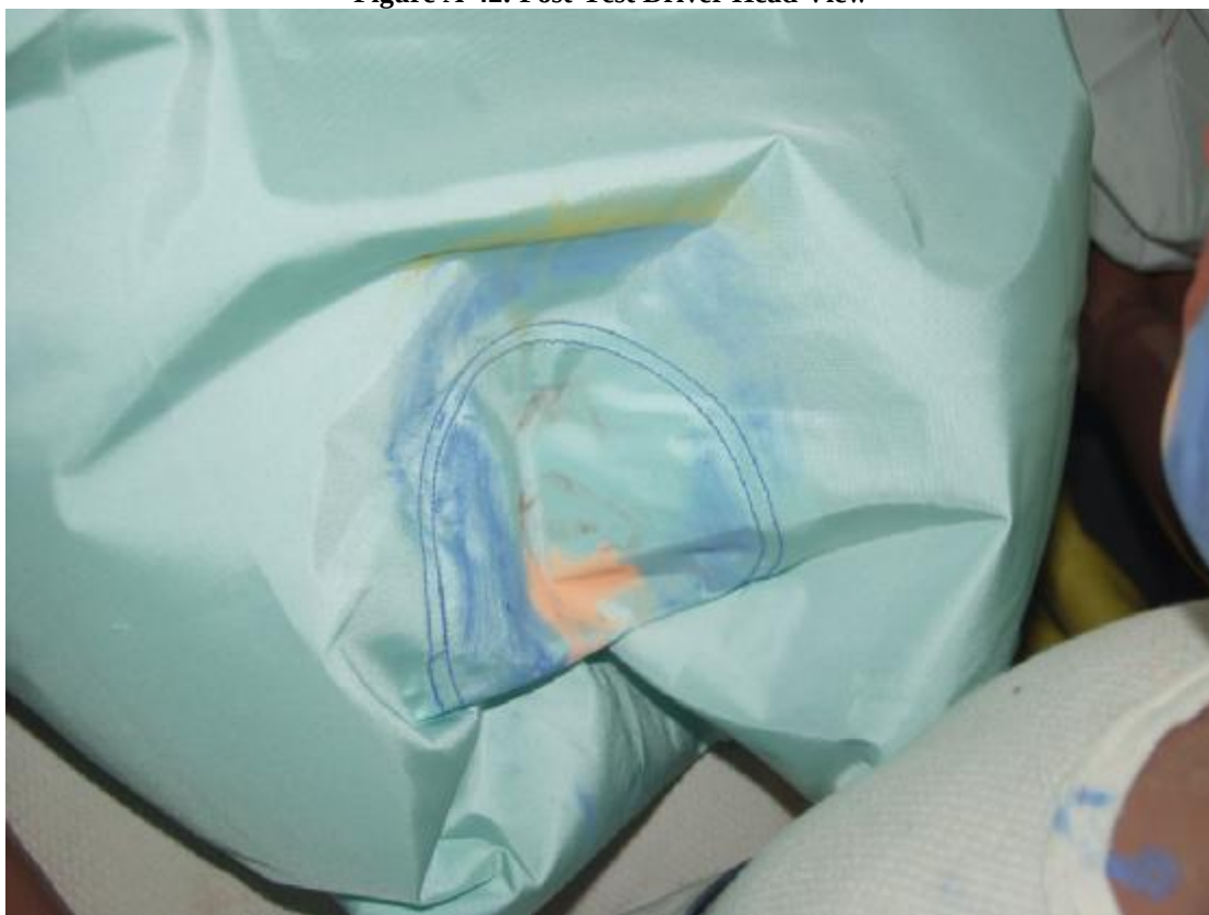
Figure A-43: Post-Test Driver Contact to Airbag
