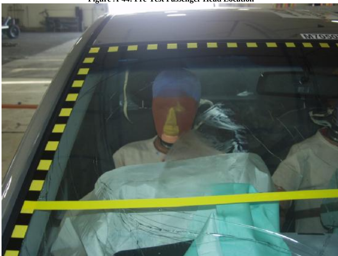
Figure A-45: Post-Test Passenger Head Location
