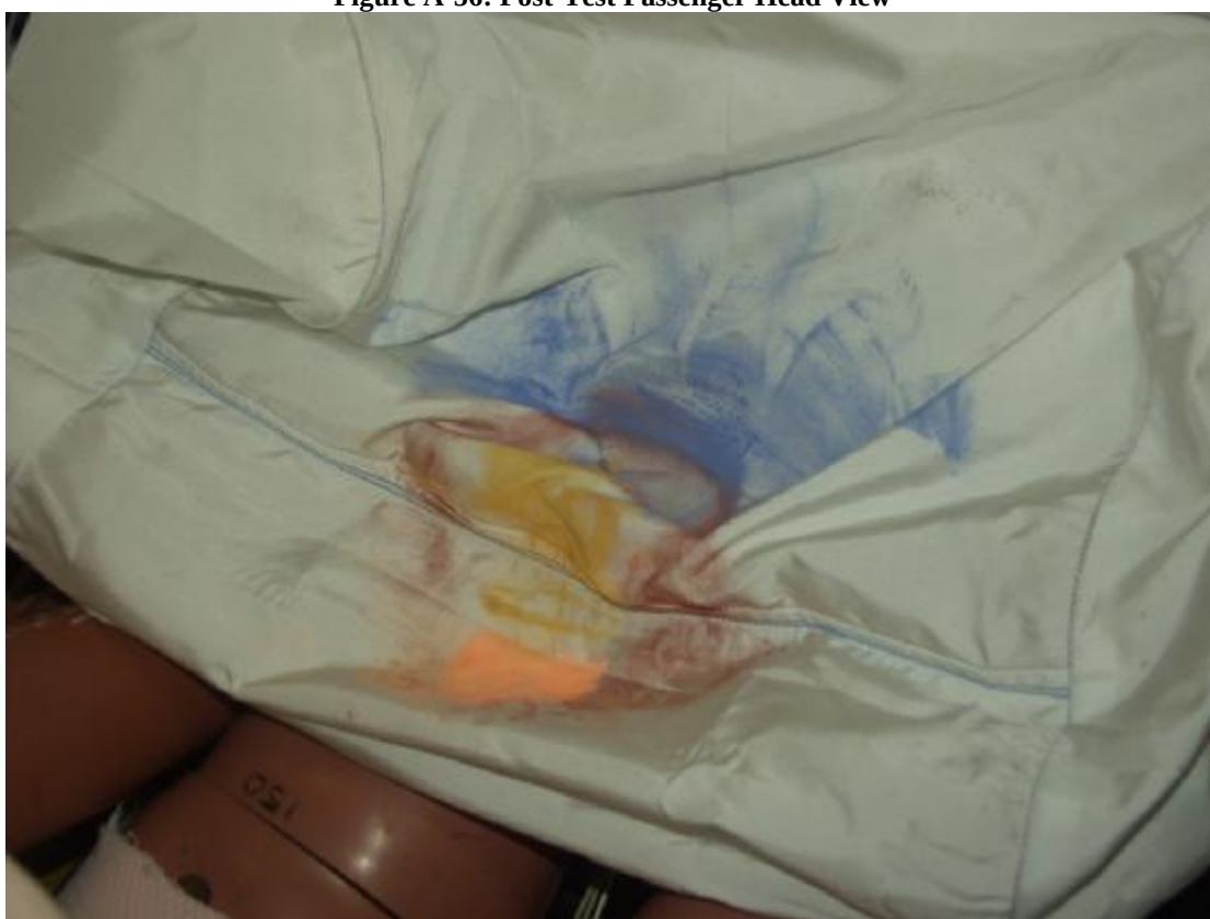
Figure A-57: Post-Test Passenger Contact to Airbag
