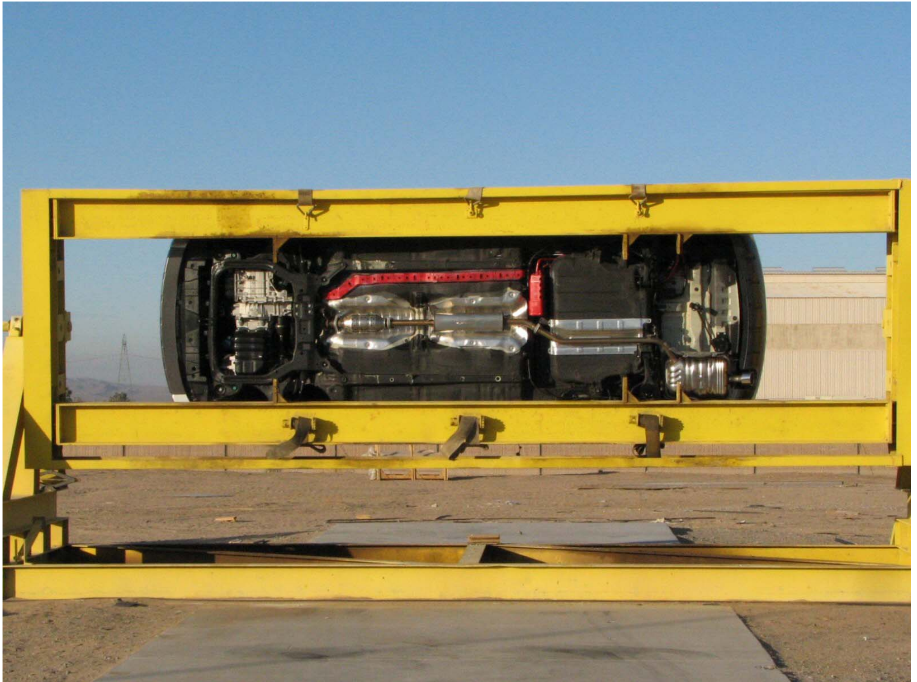
Figure A-64: Vehicle on Rollover Device (270°)
