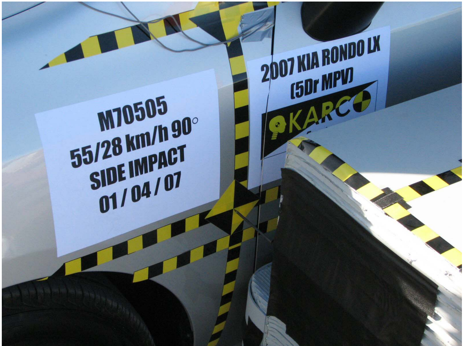
Figure A-25: Pre-Test Left Impact Point
