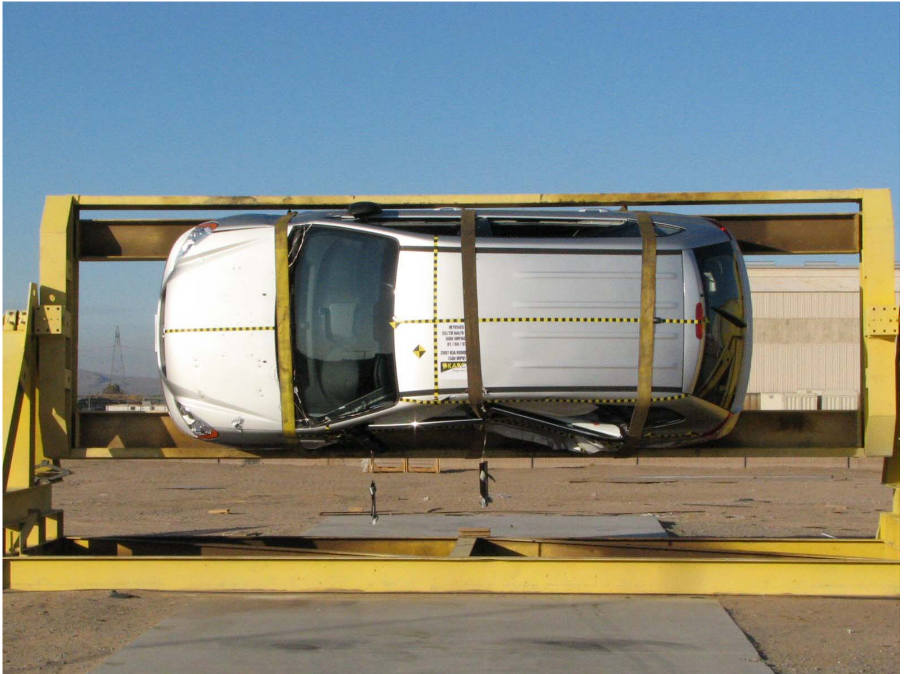
Figure A-62: Vehicle on Rollover Device (90°)
