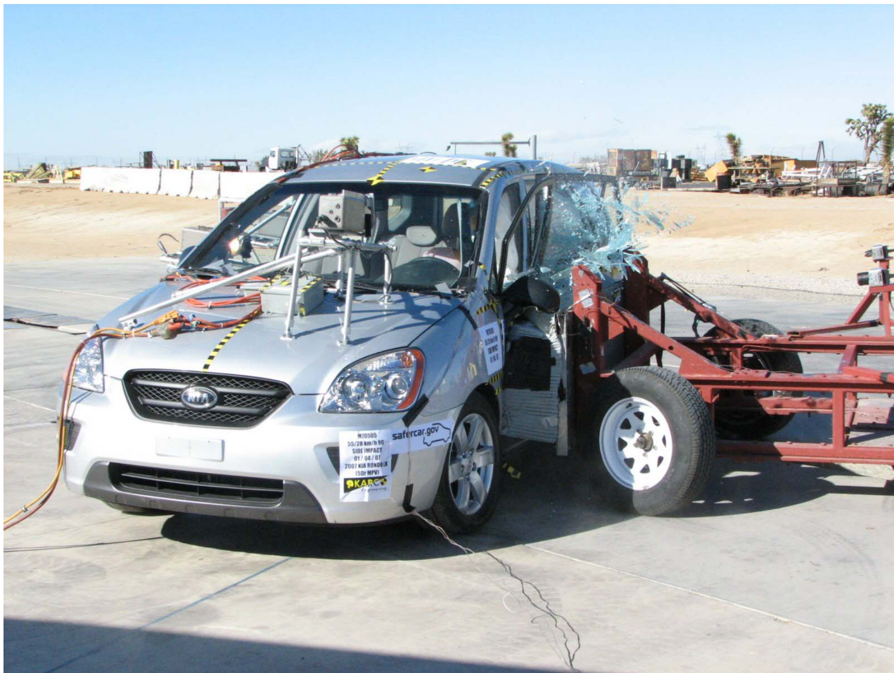
Figure A-65: Vehicle Impact
