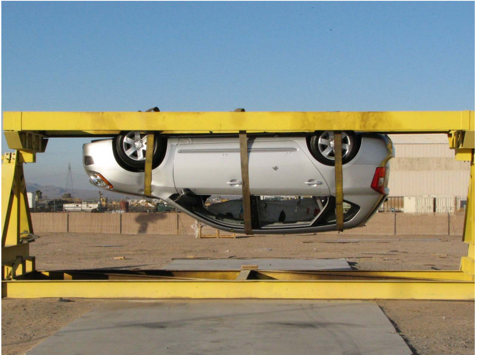
Figure A-63: Vehicle on Rollover Device (180°)
