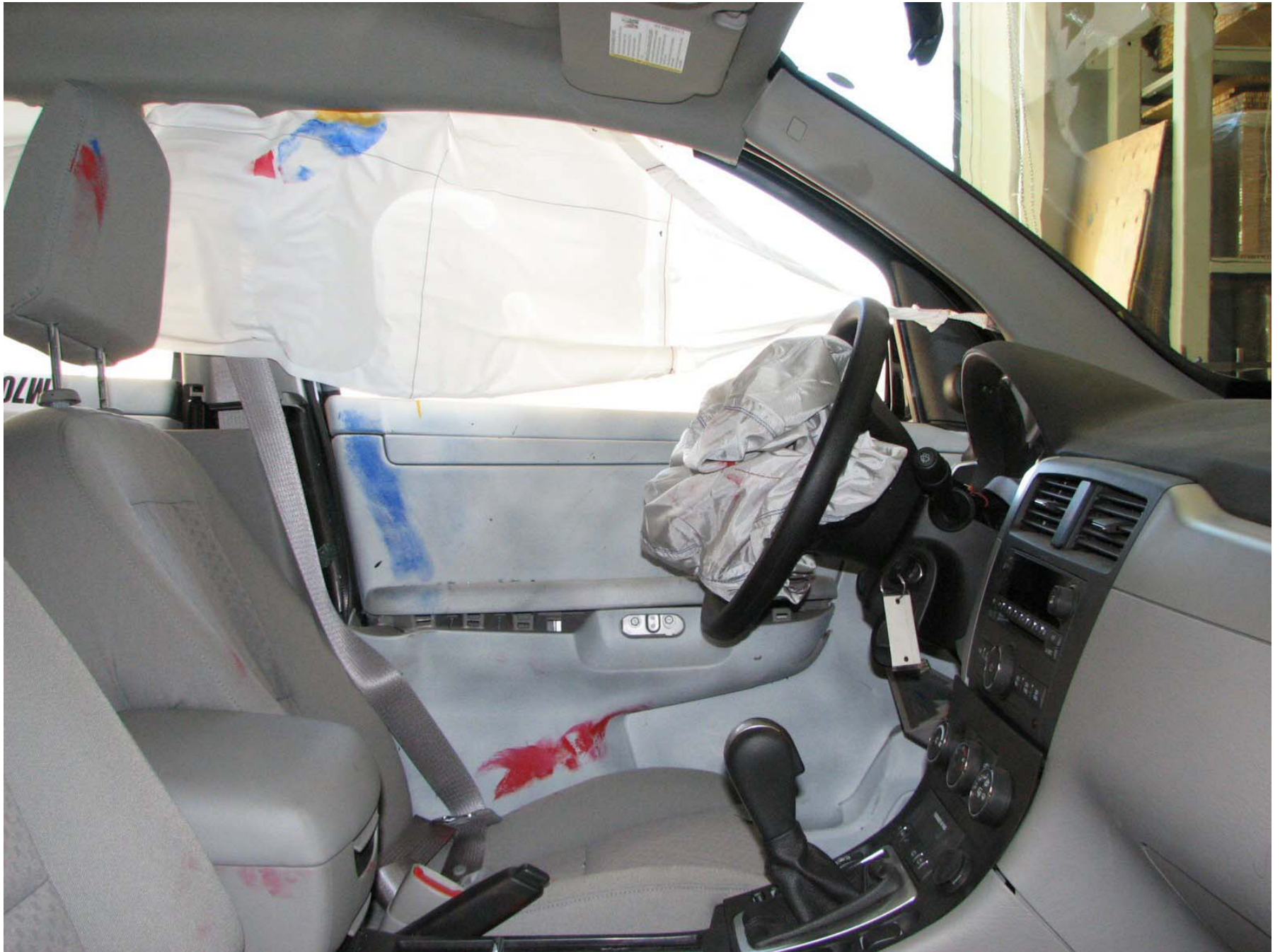
Figure A-43: Post-Test Front Door Panel (Interior)
