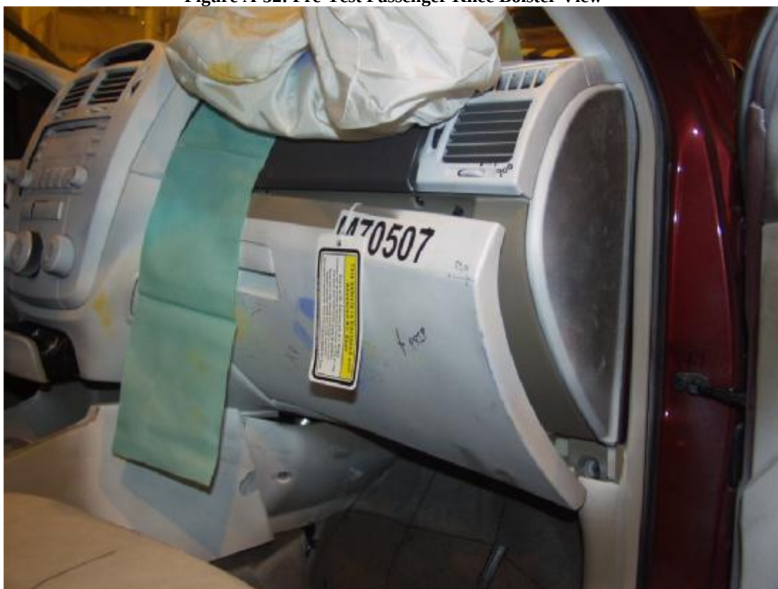
Figure A-53: Post-Test Passenger Knee Bolster View
