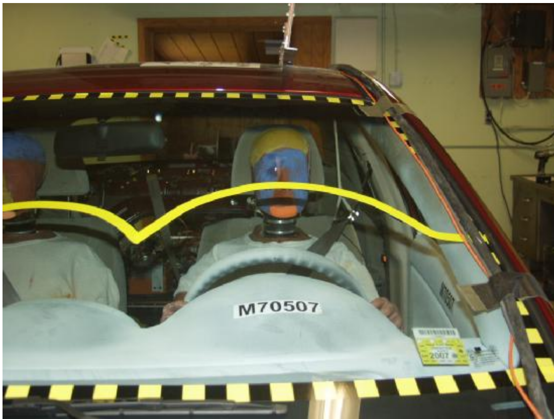
Figure A-30: Pre-Test Driver Head Location
