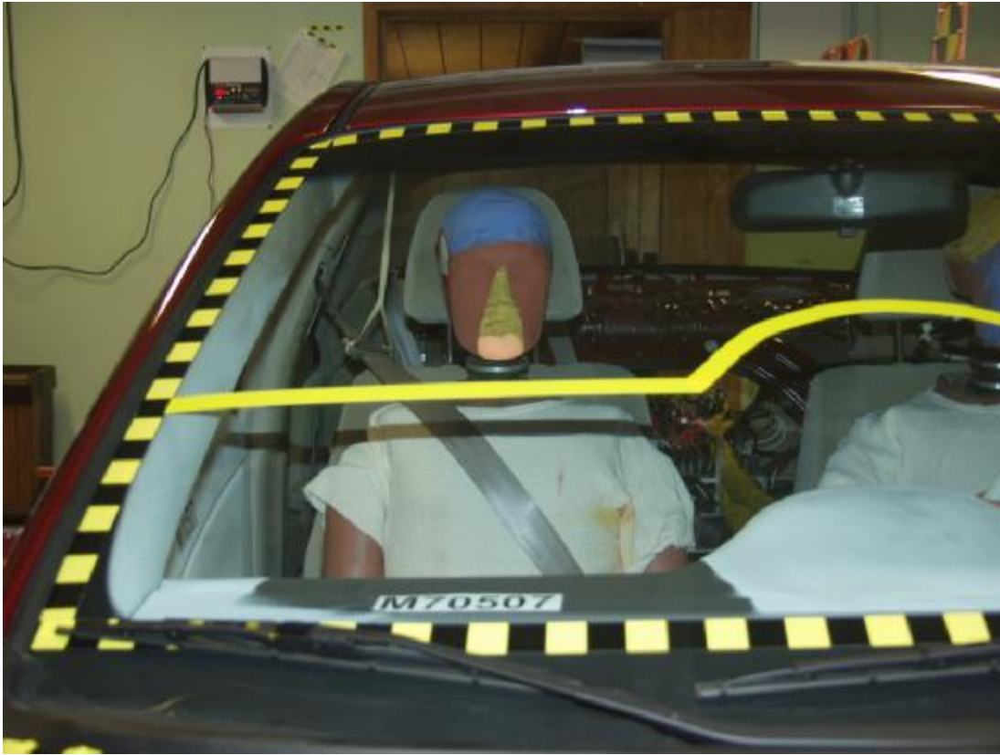
Figure A-44: Pre-Test Passenger Head Location
