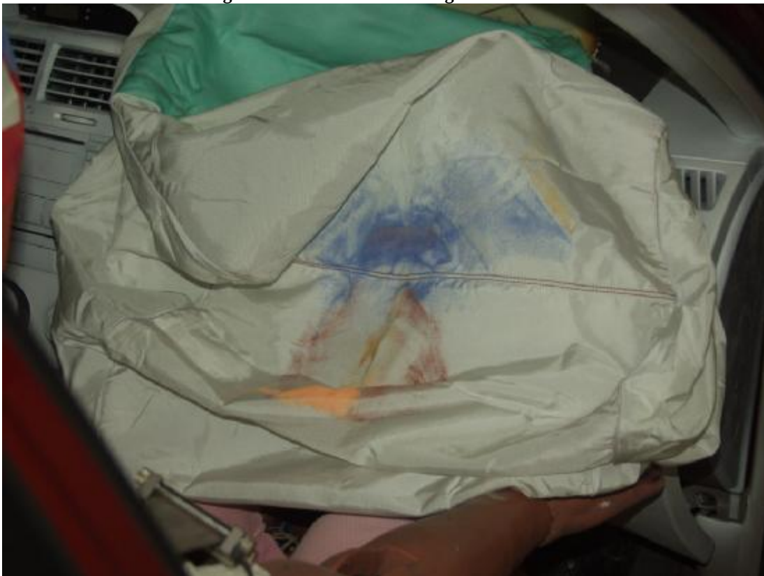
Figure A-57: Post-Test Passenger Contact to Airbag
