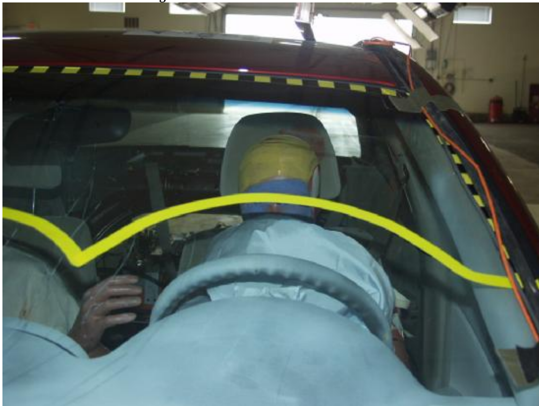
Figure A-31: Post-Test Driver Head Location
