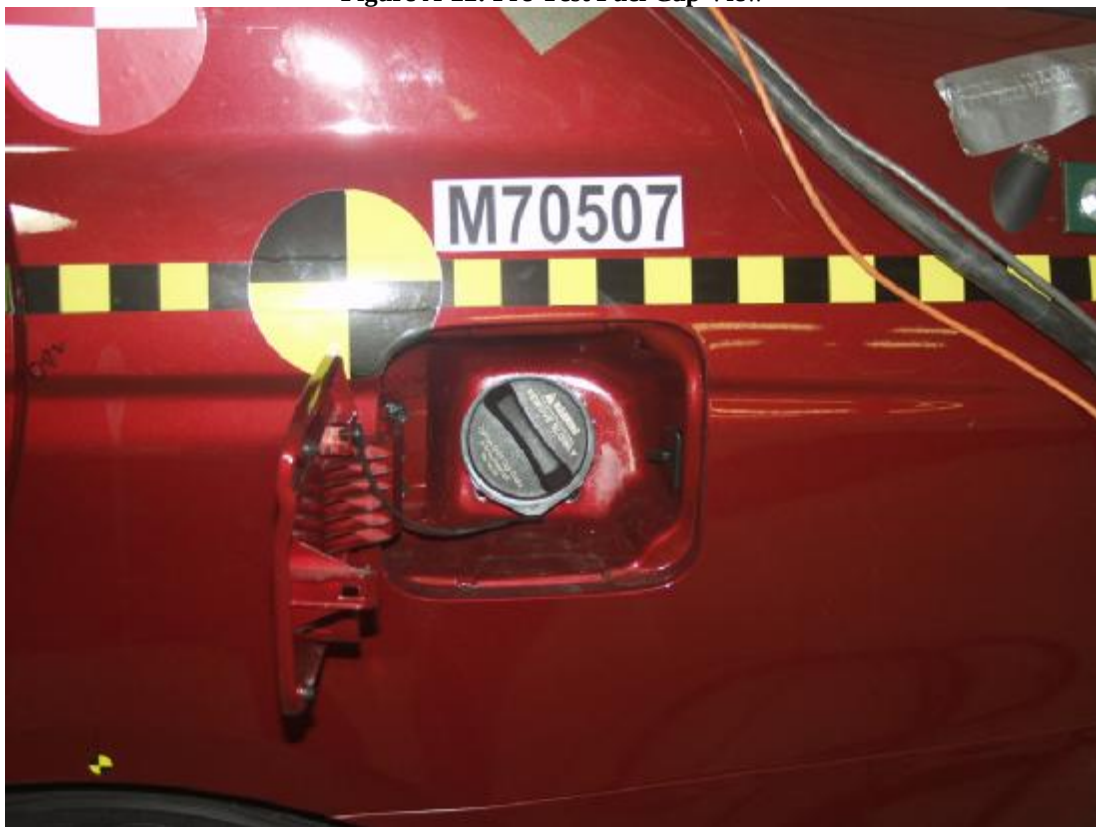
Figure A-23: Post-Test Fuel Cap View
