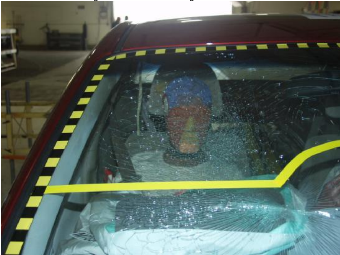
Figure A-45: Post-Test Passenger Head Location
