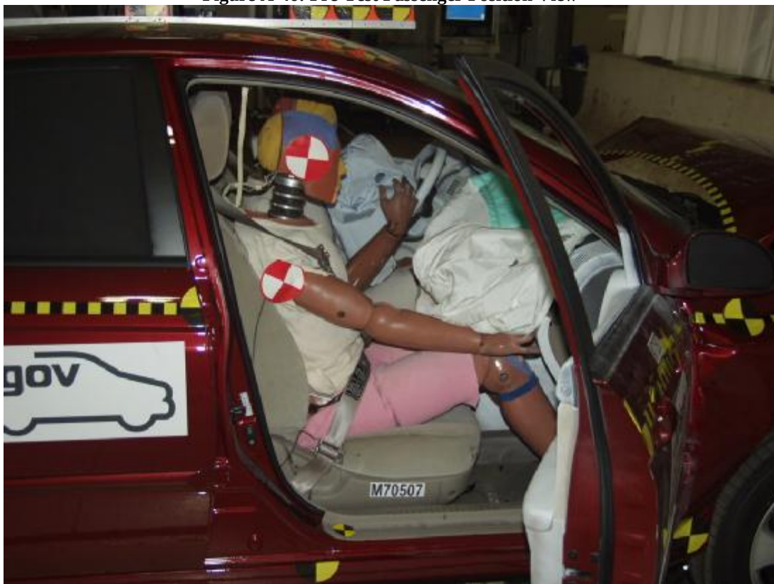
Figure A-47: Post-Test Passenger Position View
