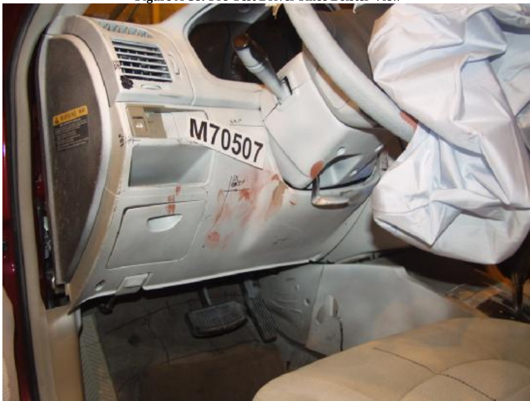
Figure A-39: Post-Test Driver Knee Bolster View
