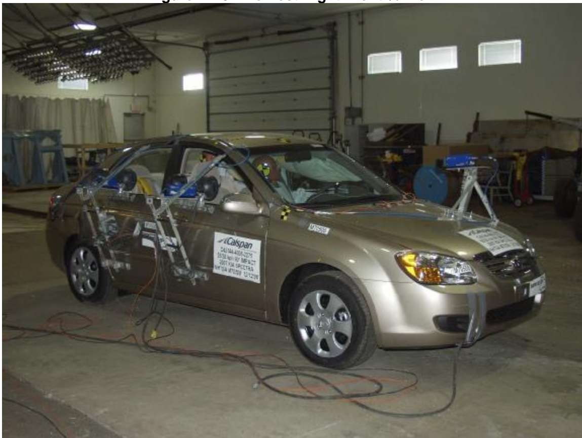
Figure A-20: Post-Test Right Front ¾ View
