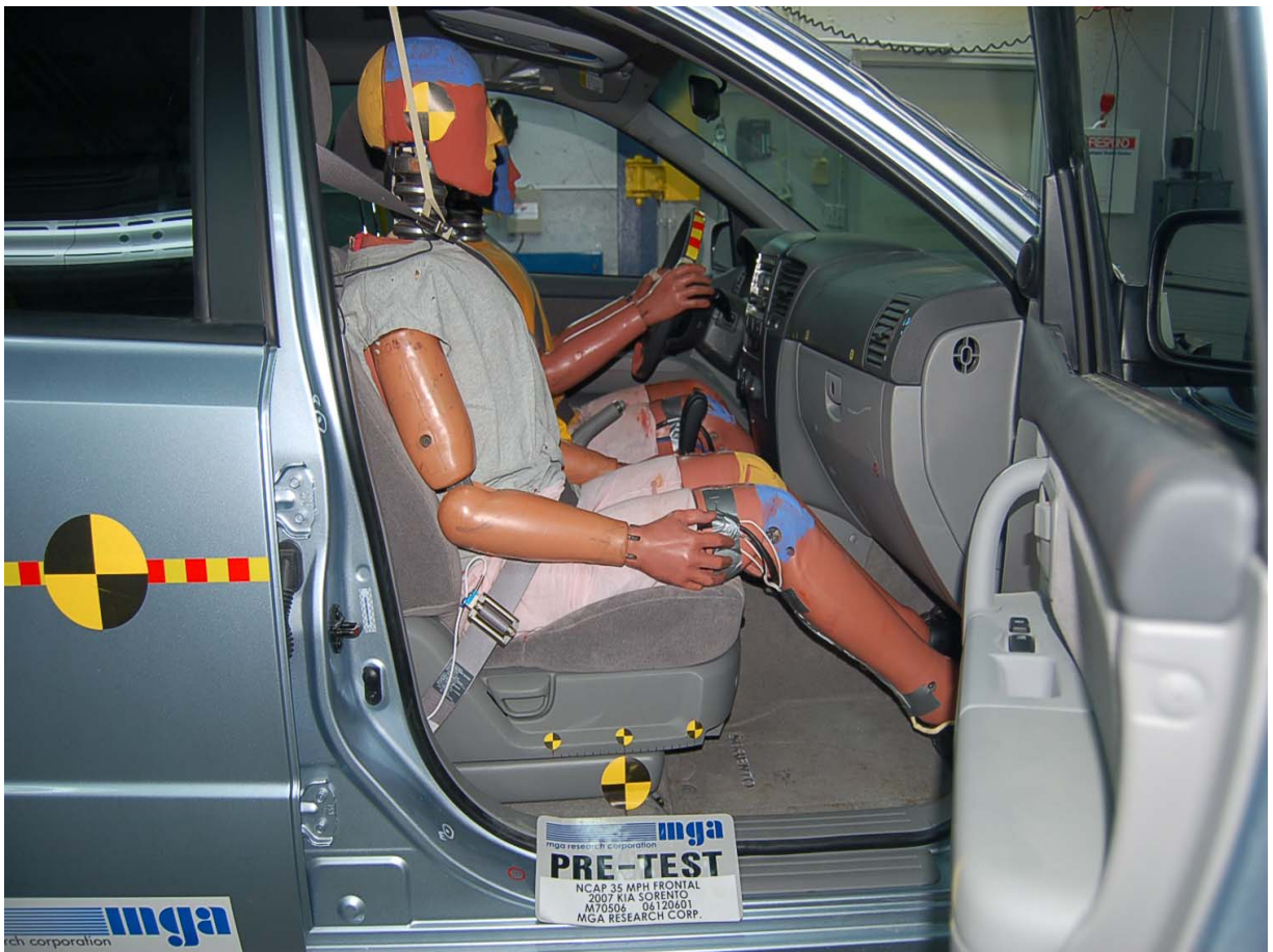
Pre-Test Passenger Dummy (Door Open)
