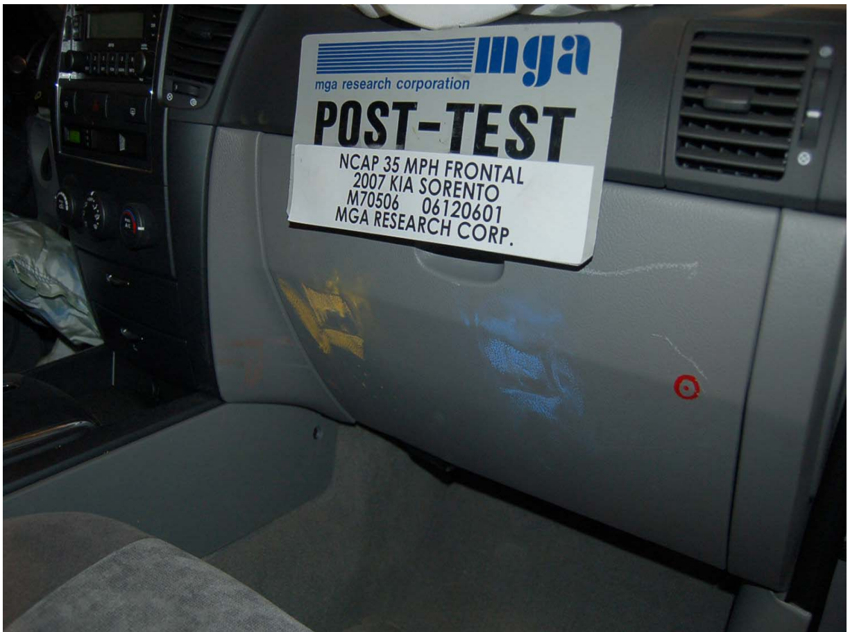
Post-Test Passenger Dummy Knee Contact
