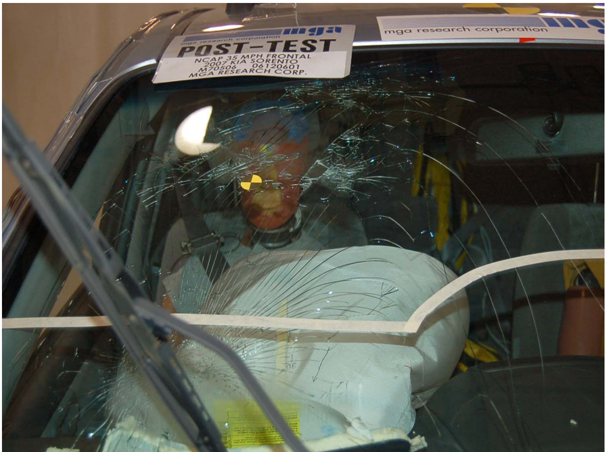
Post-Test Passenger Dummy Front View (Head Position)
