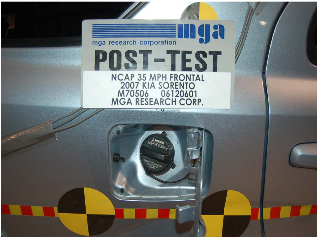
Post-Test Fuel Cap View
