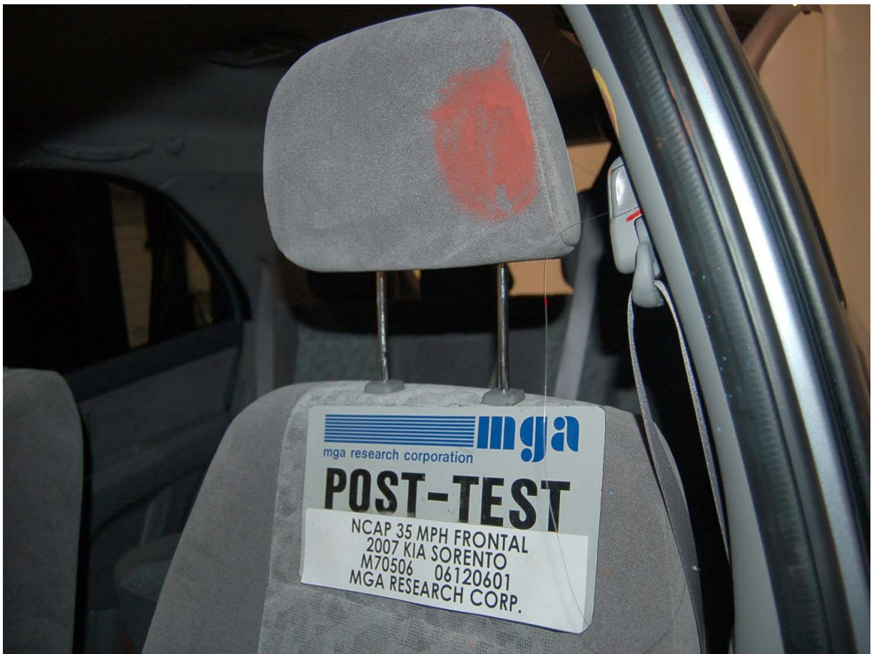
Post-Test Driver Dummy Head Contact (headrest)
