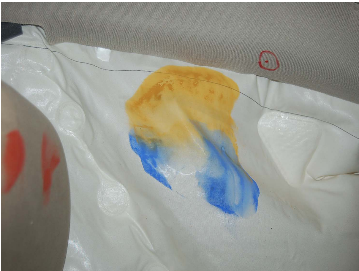
Post-Test Driver Dummy Head Contact (airbag)
