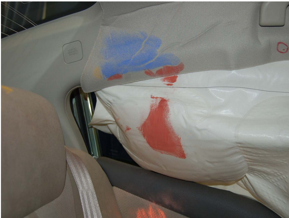
Post-Test Passenger Dummy Head Contact (airbag)
