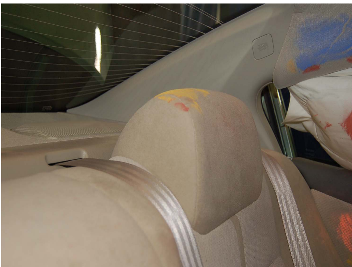
Post-Test Passenger Dummy Head Contact (headrest)
