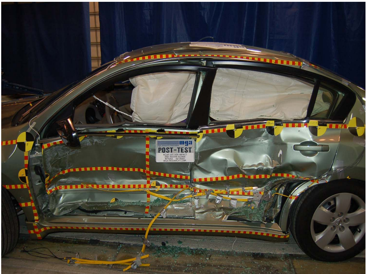
Post-Test Left Side Impact Close-up
