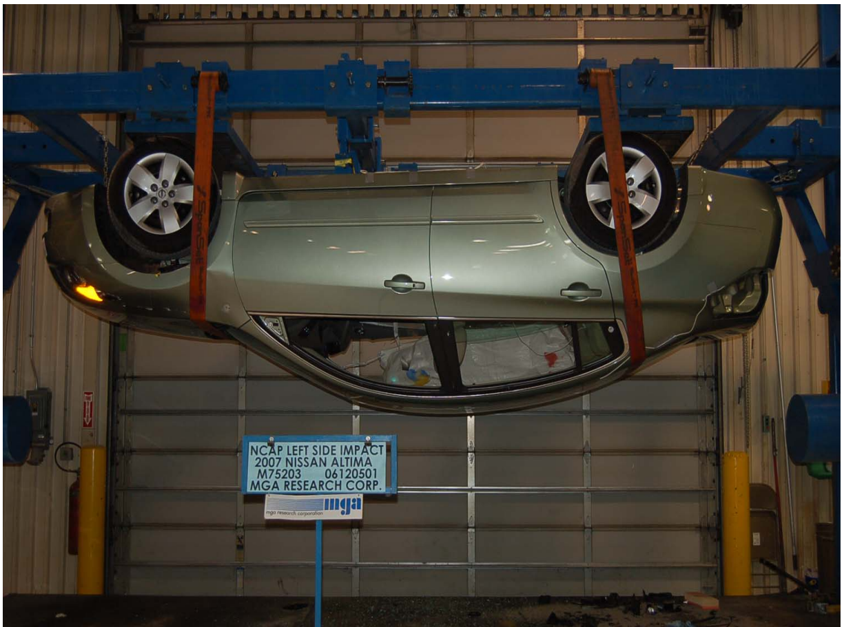
Vehicle on Rollover Device (180 Degrees)
