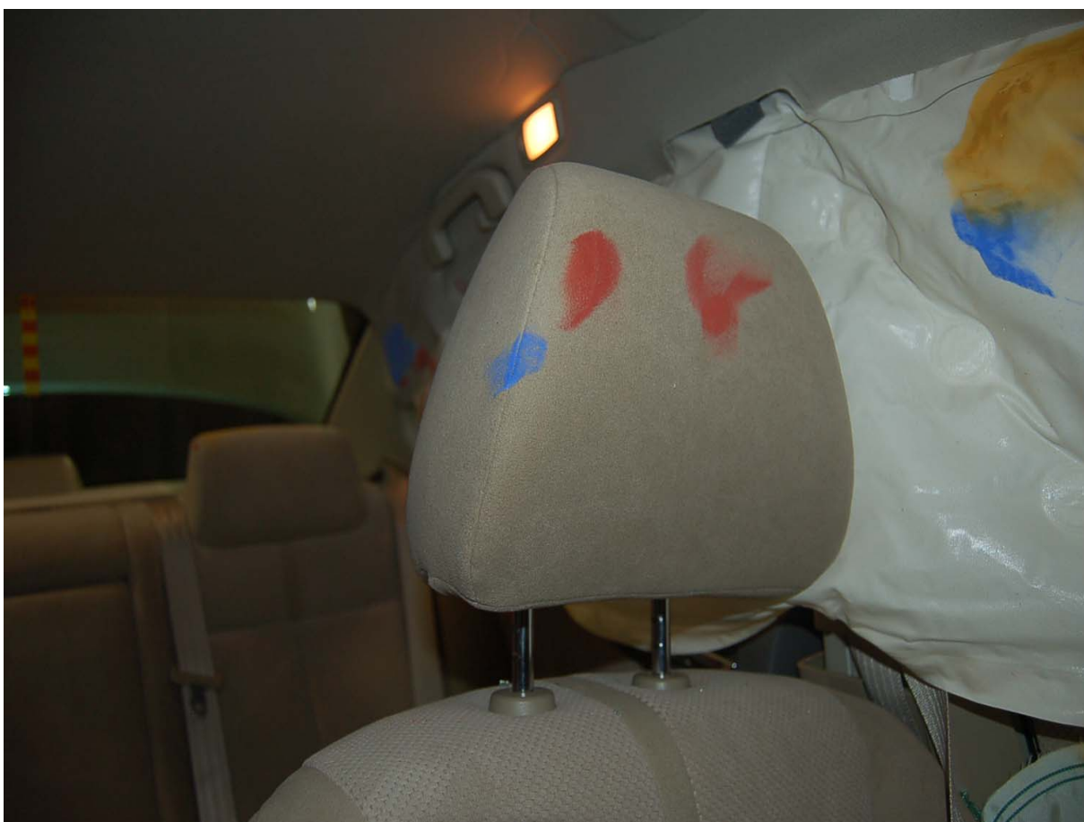
Post-Test Driver Dummy Head Contact (headrest)
