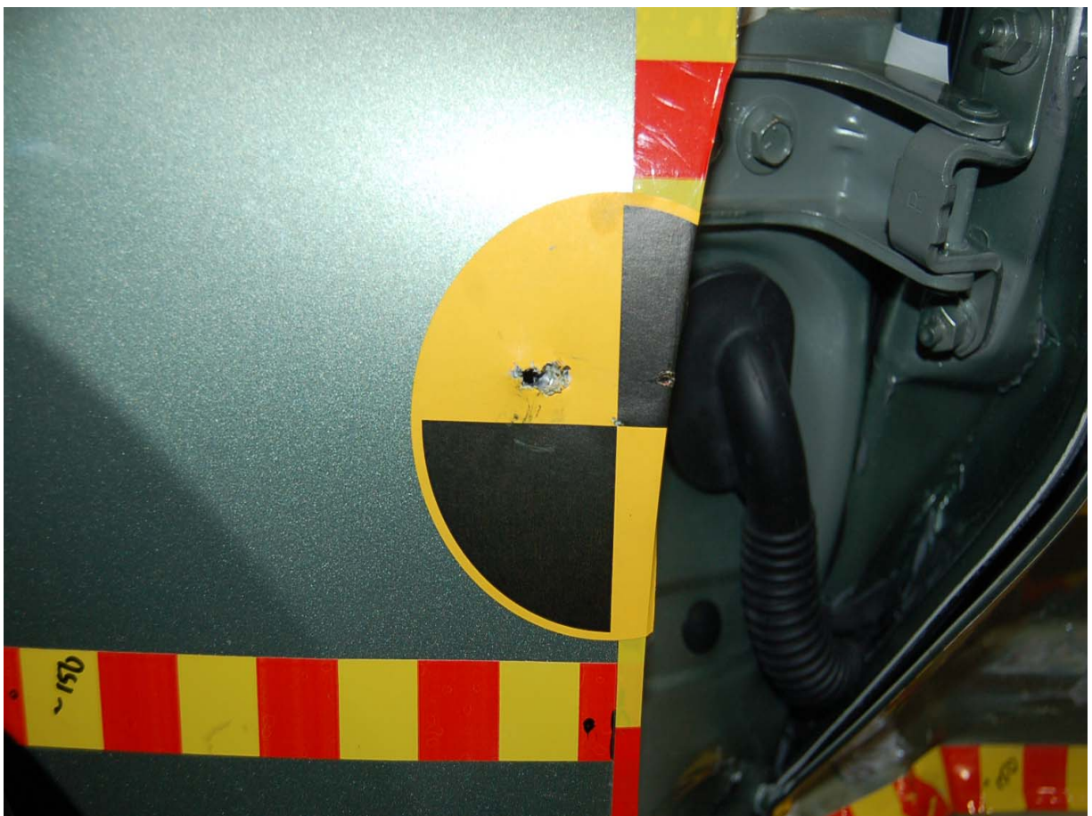
Post-Test Left Impact Point
