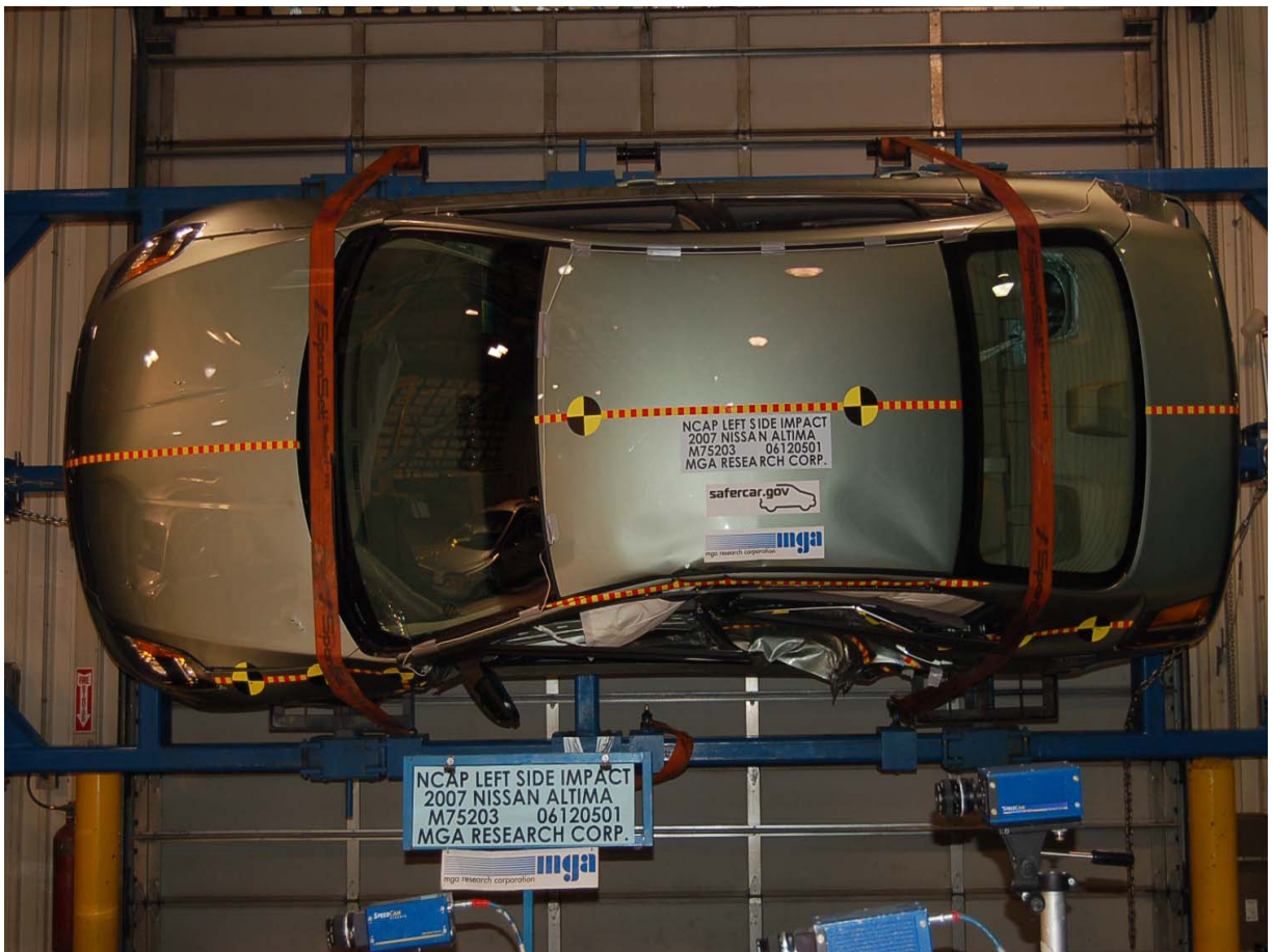
Vehicle on Rollover Device (90 Degrees)
