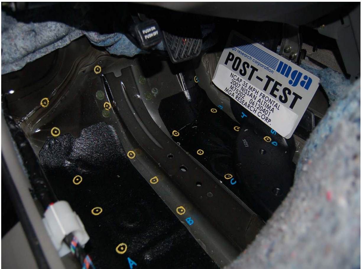
Post-Test Driver Side Floor Pan
