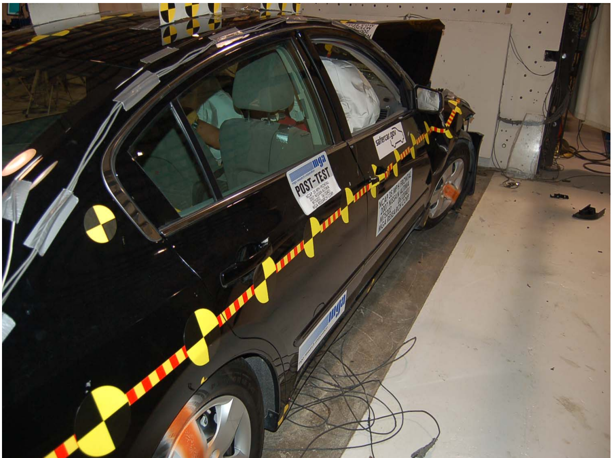
Post-Test Right Side ¾ View of Doors After Impact
