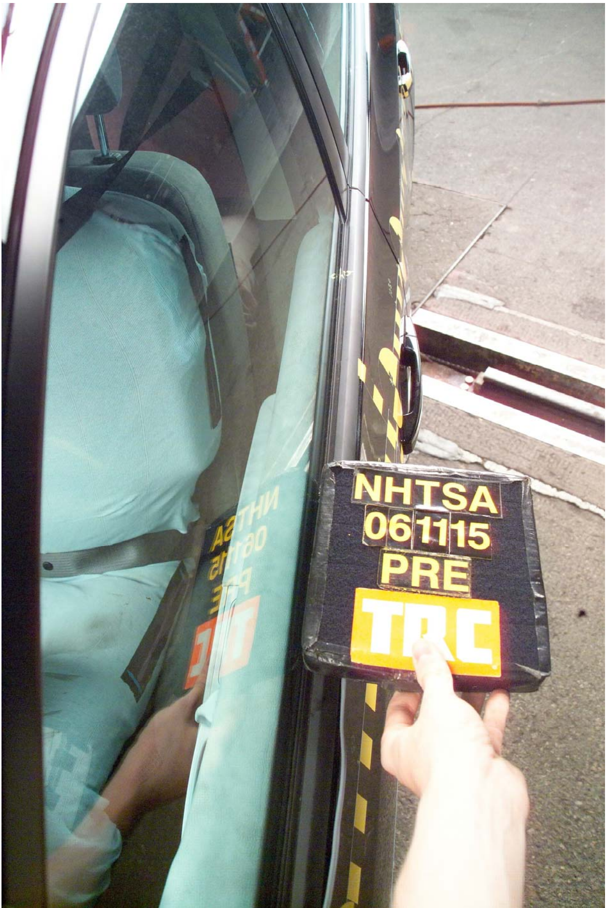
Figure A-52 Pre-Test Left View of Front SID HIII and Door Clearance
