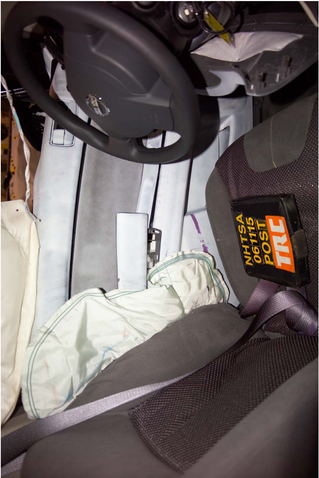
Figure A-60 Post-Test Interior of Front Door Showing SID HIII Impact Locations
