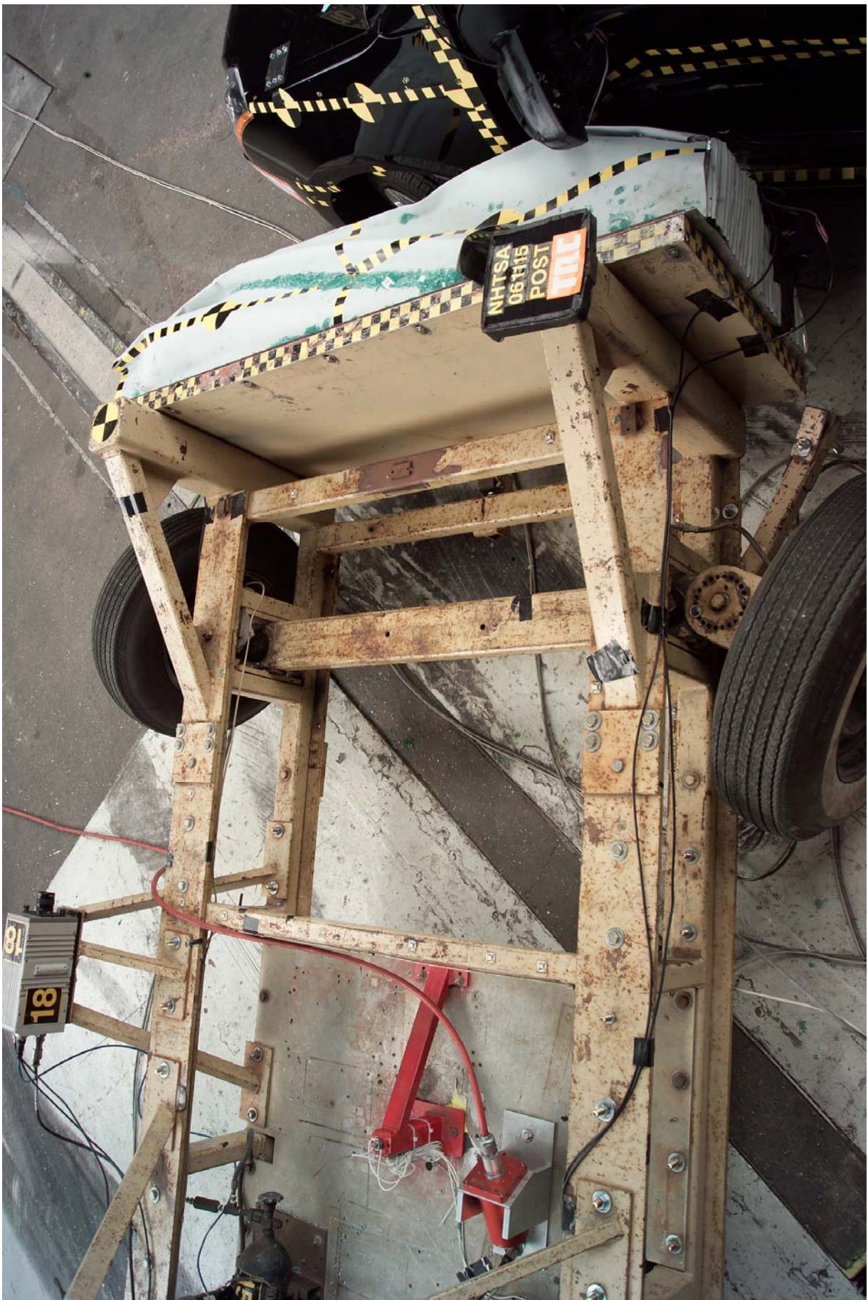
Figure A-78 Post-Test Overhead View of MDB With Impactor Face in Position
