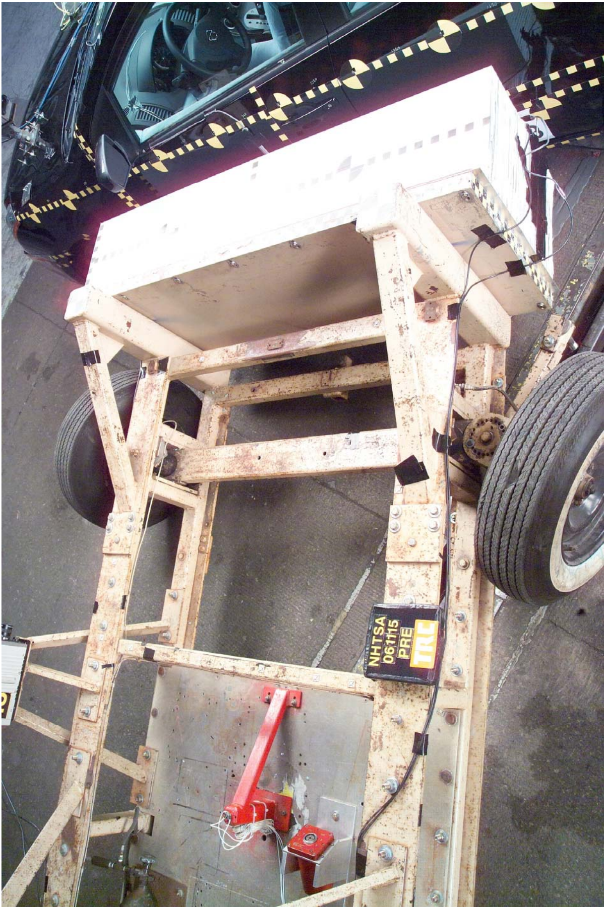
Figure A-77 Pre-Test Overhead View of MDB With Impactor Face in Position
