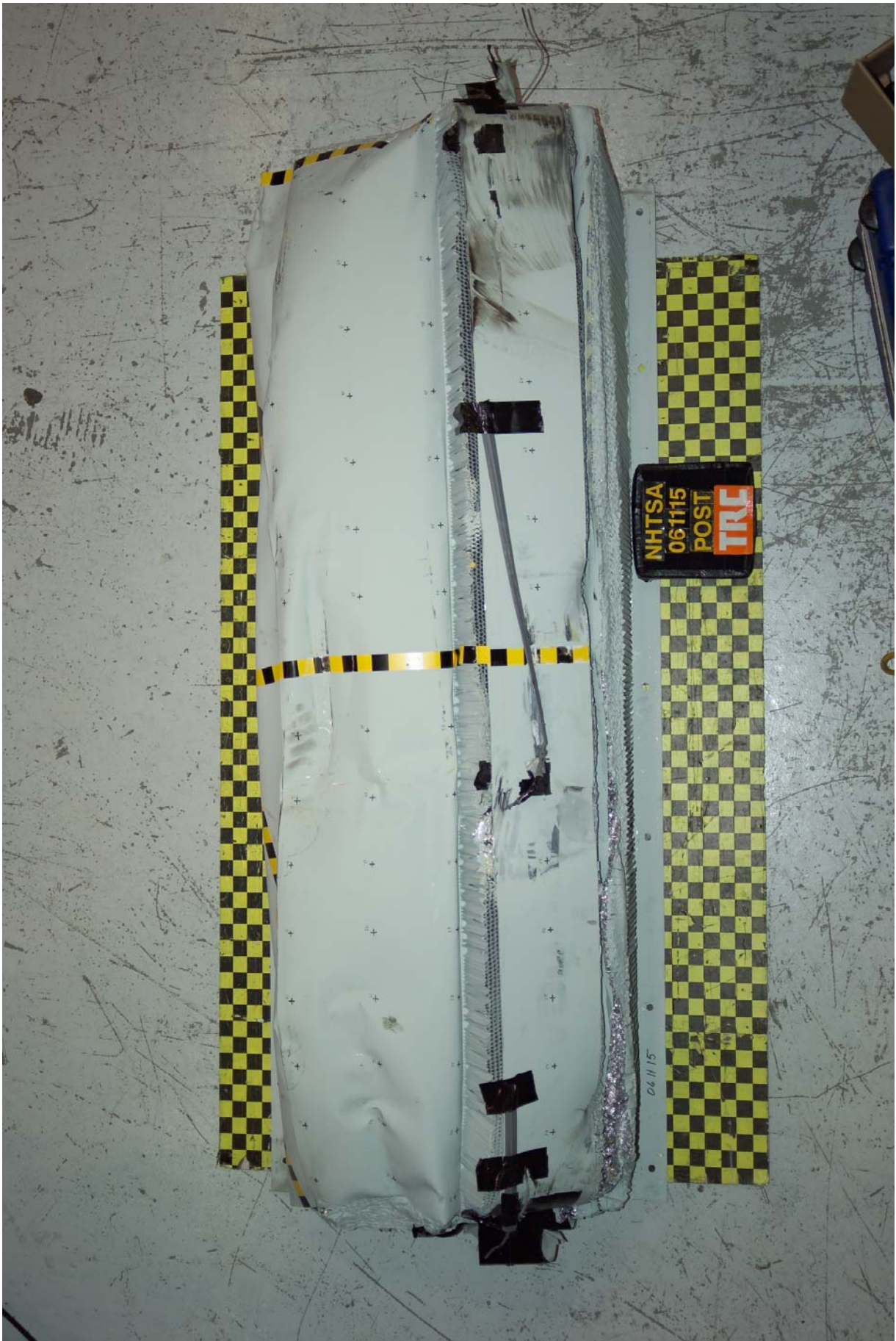
Figure A-18 Post-Test Frontal View of Impactor Face
