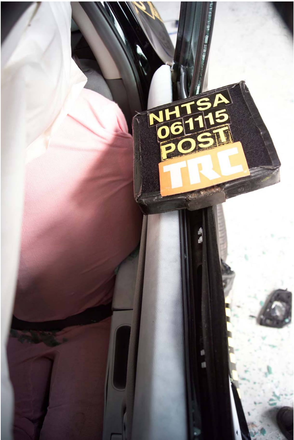
Figure A-58 Post-Test Left View of Rear SID HIII and Door Clearance
