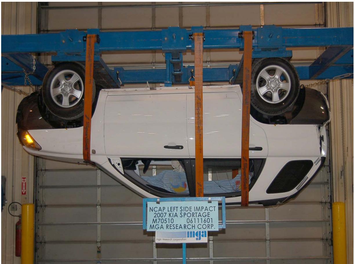
Vehicle on Rollover Device (180 Degrees)
