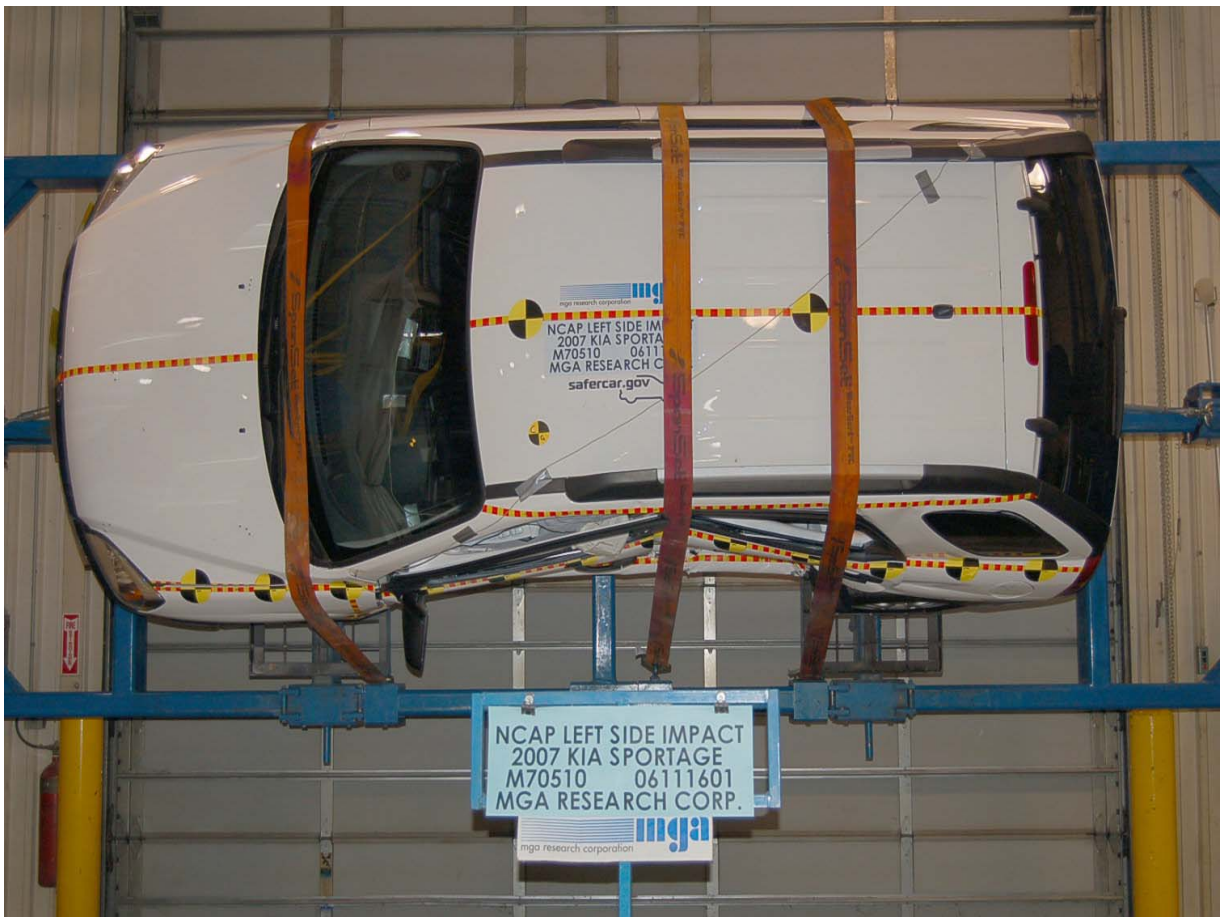
Vehicle on Rollover Device (90 Degrees)
