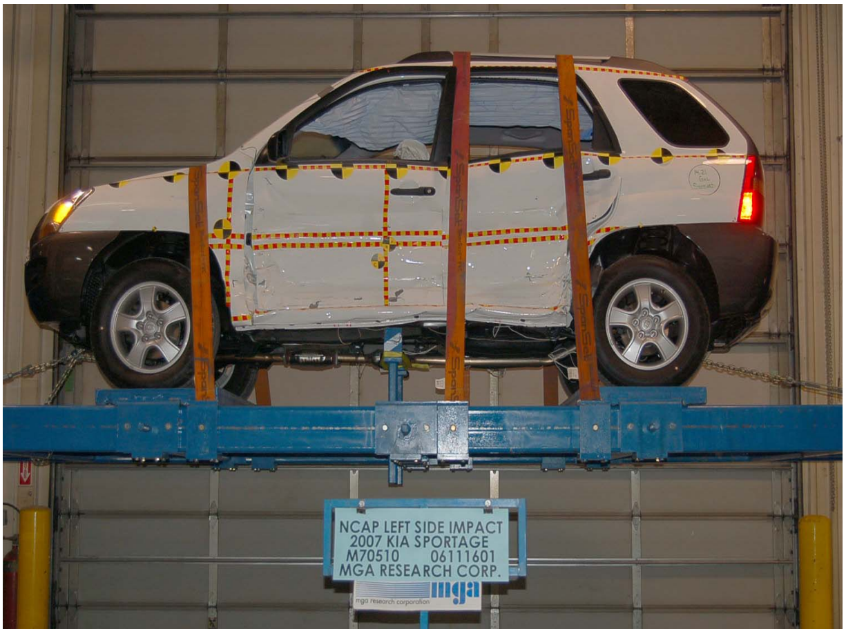
Vehicle on Rollover Device (360 Degrees)
