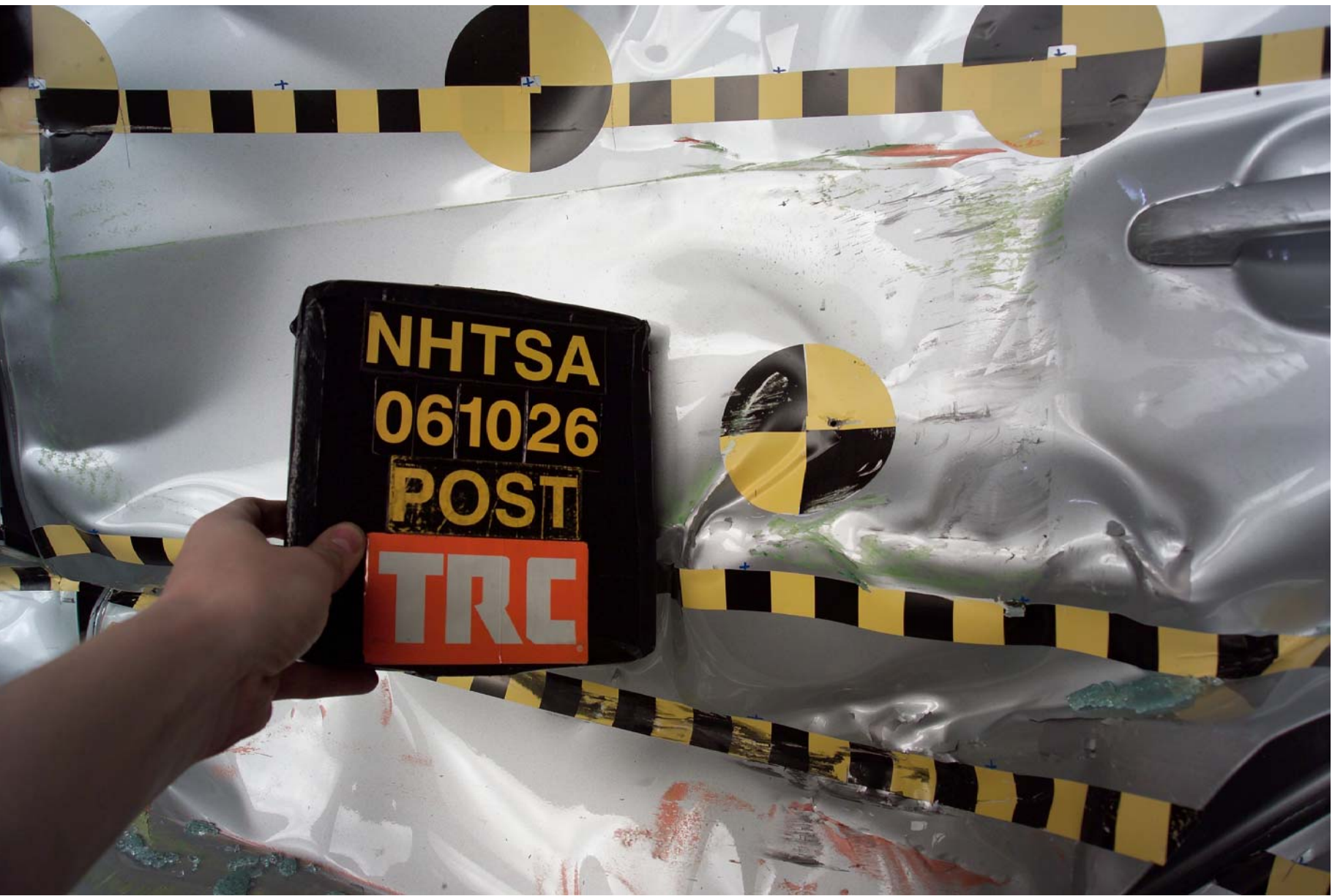
Figure A-66 Post-Test Secondary Impact Point View
