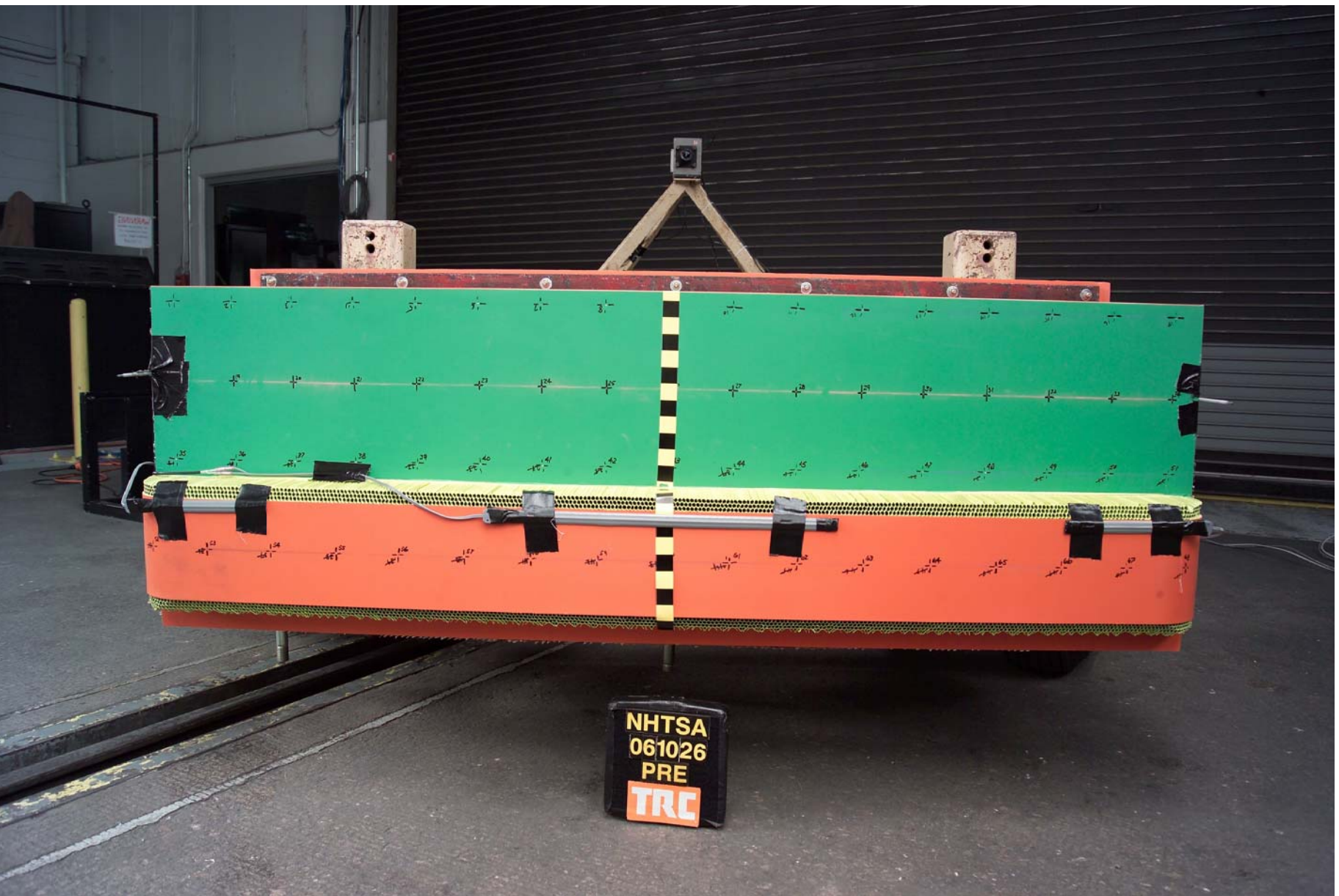
Figure A-33 Pre-Test View of MDB Showing Contact Switches in Place
