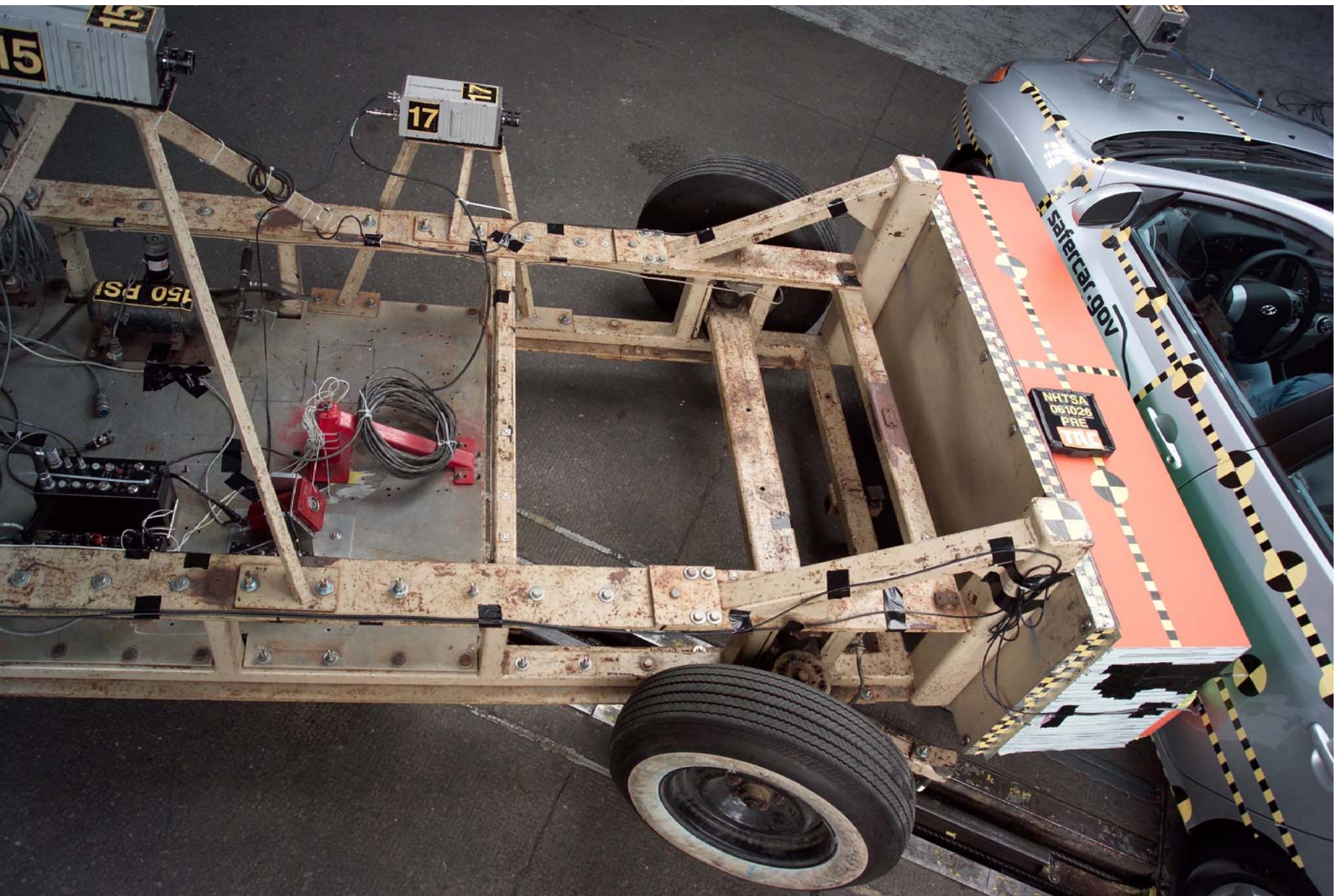
Figure A-67 Pre-Test Overhead View of MDB With Impactor Face in Position
