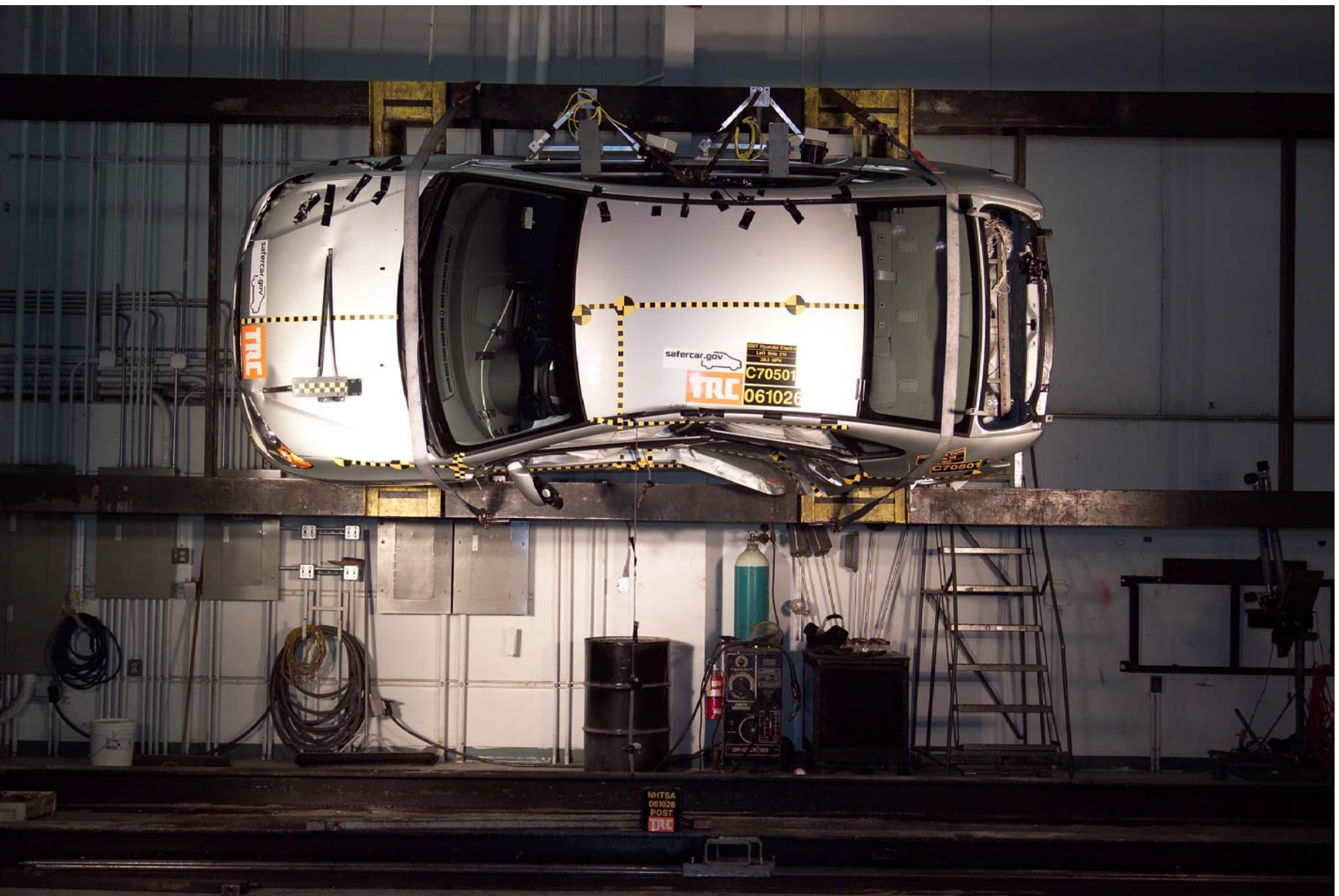
Figure A-76 FMVSS 301 Rollover View at 90°
