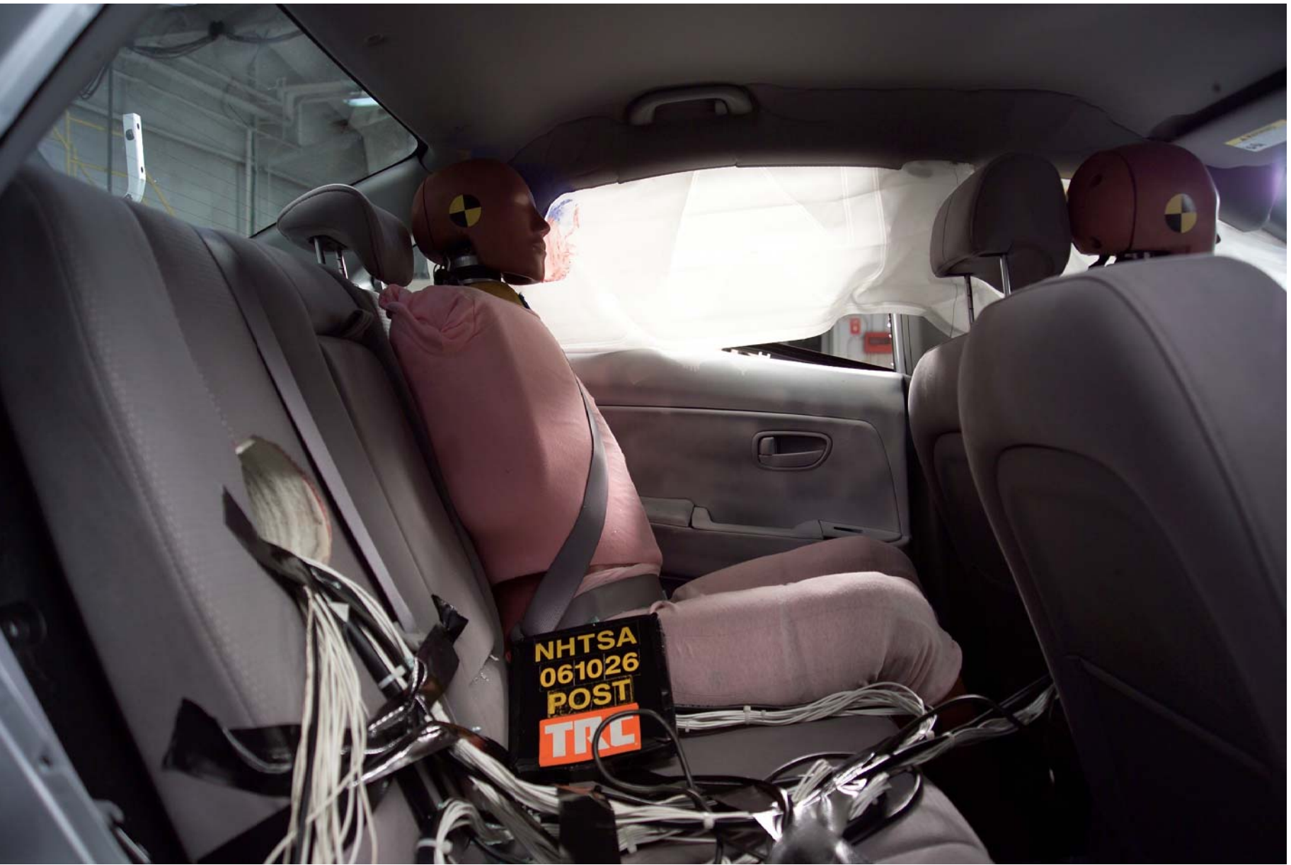
Figure A-40 Post-Test Right Occupant Compartment View of Rear SID HIII
