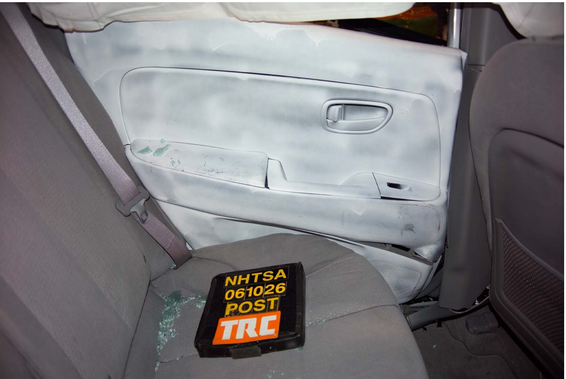
Figure A-58 Post-Test Rear SID HII Contact - View 2
