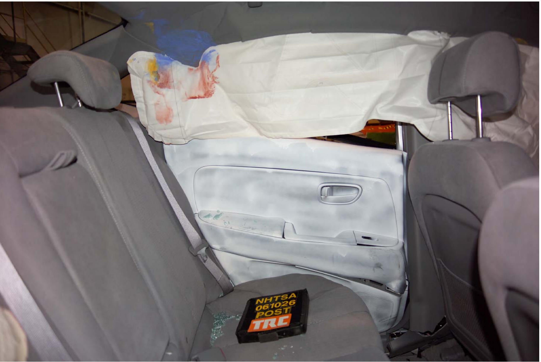
Figure A-56 Post-Test Interior of Rear Panel Showing SID HIII Impact Locations
