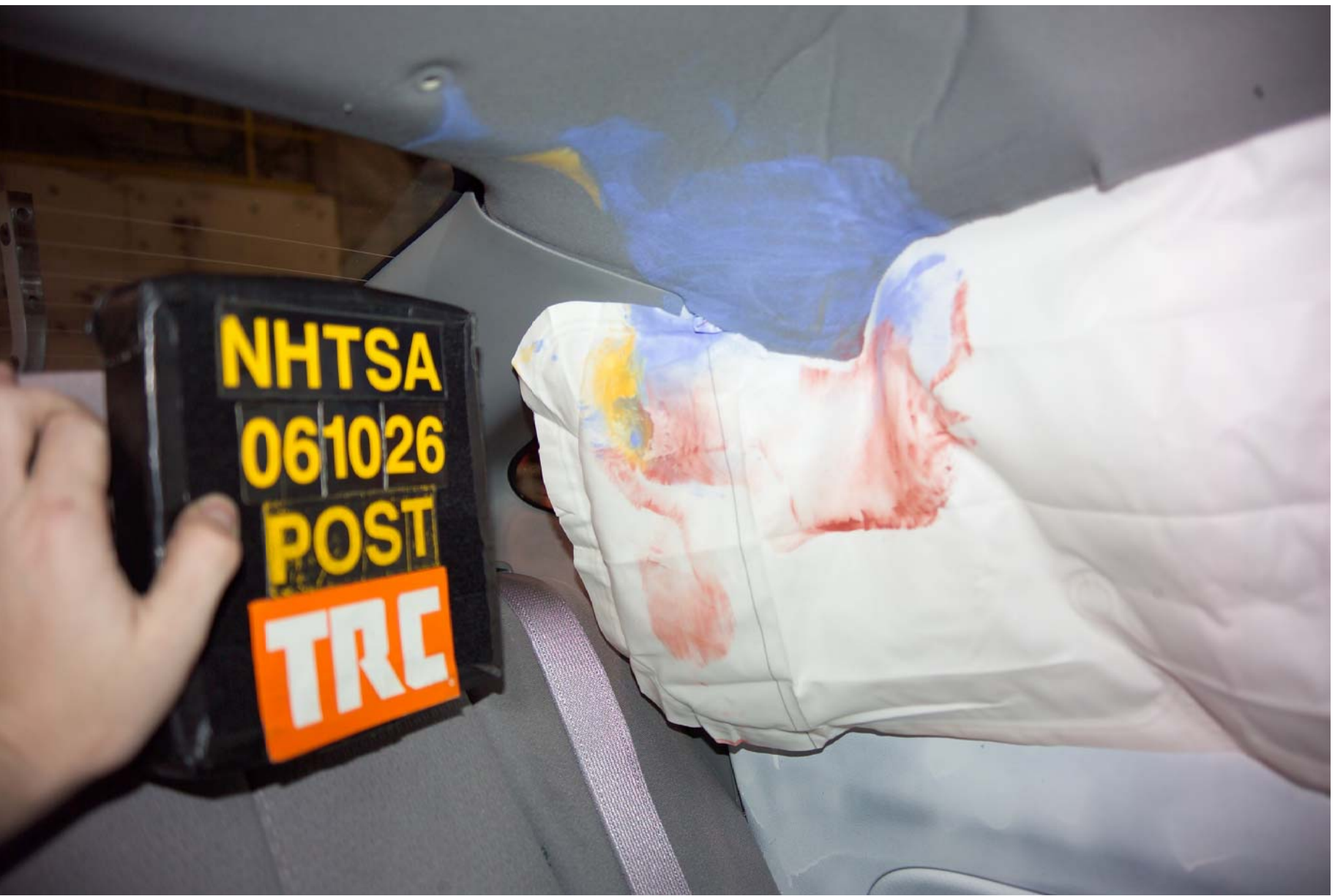
Figure A-57 Post-Test Rear SID HIII Contact - View 1
