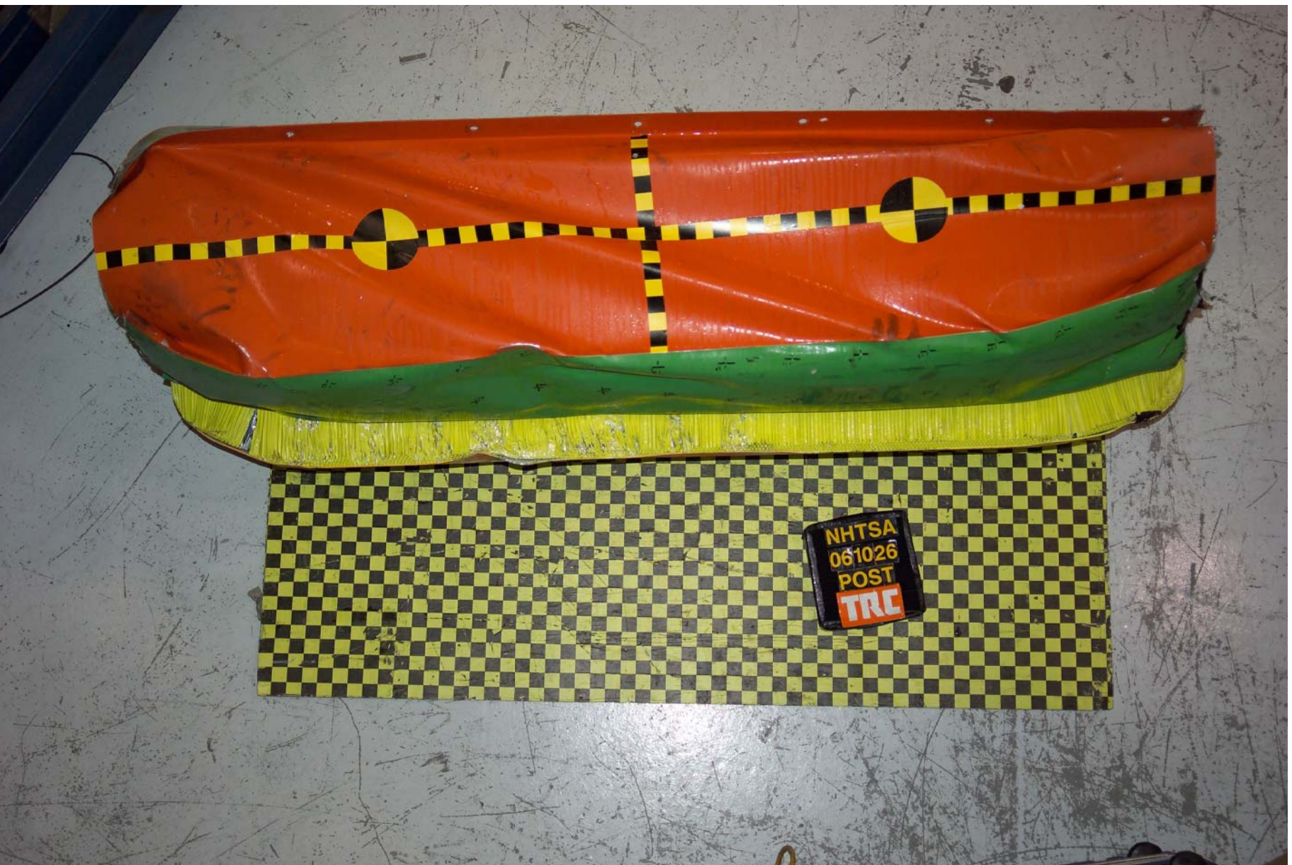
Figure A-20 Post-Test Top View of Impactor Face
