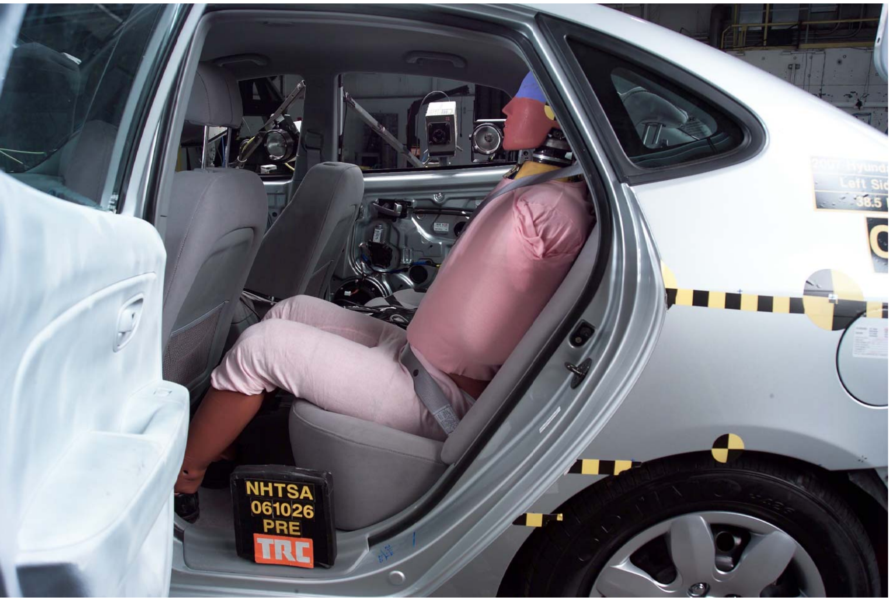
Figure A-48 Pre-Test Left of Rear SID HII and Belt Position
