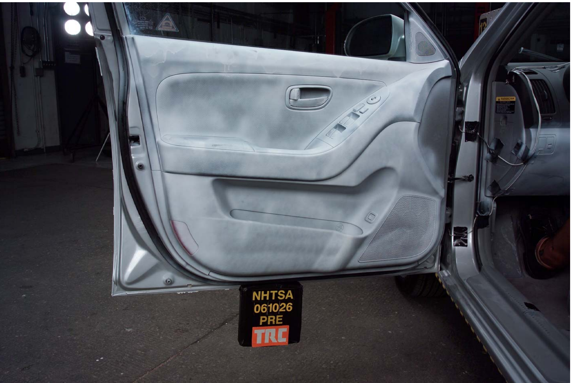
Figure A-51 Pre-Test Interior of Front Door
