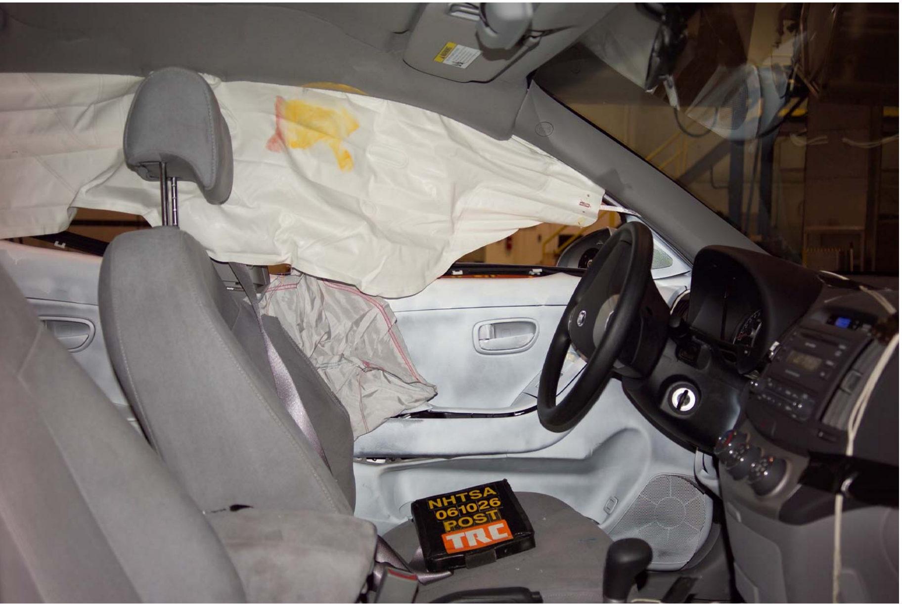
Figure A-52 Post-Test Interior of Front Door Showing SID HIII Impact Locations
