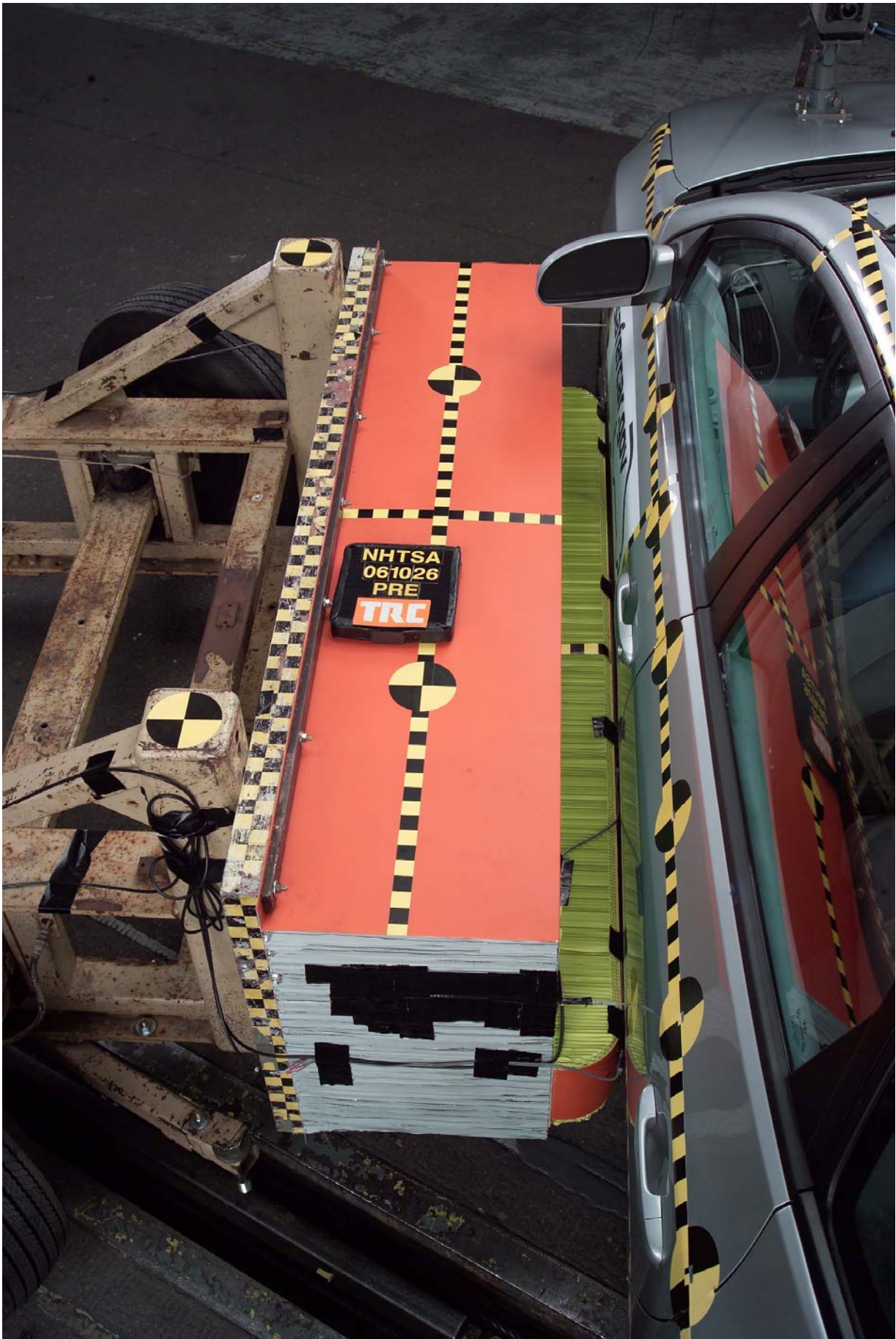
Figure A-35 Pre-Test Overhead View of MDB Aligned with Vehicle
