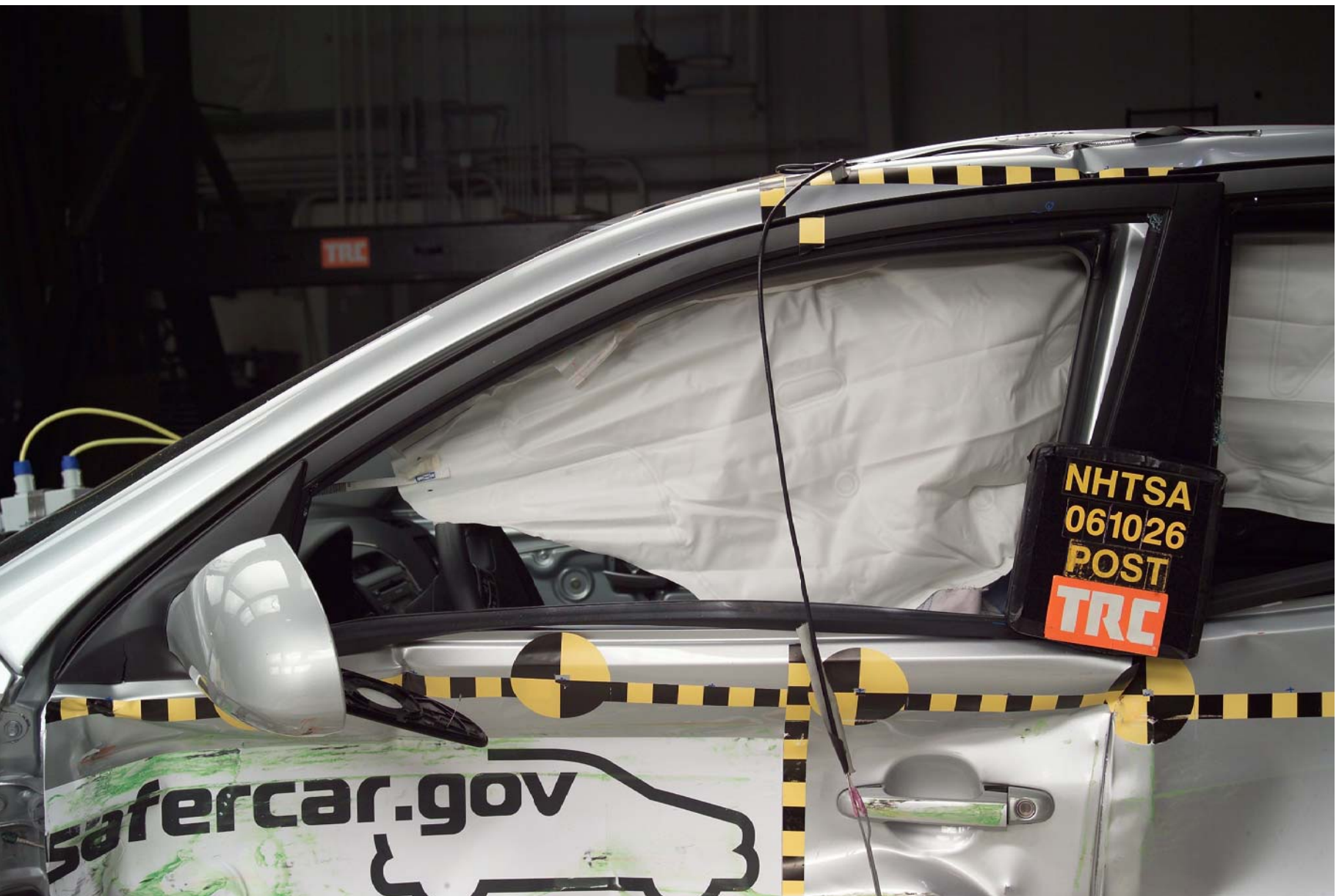
Figure A-42 Post-Test Left View of Front SID HIII
