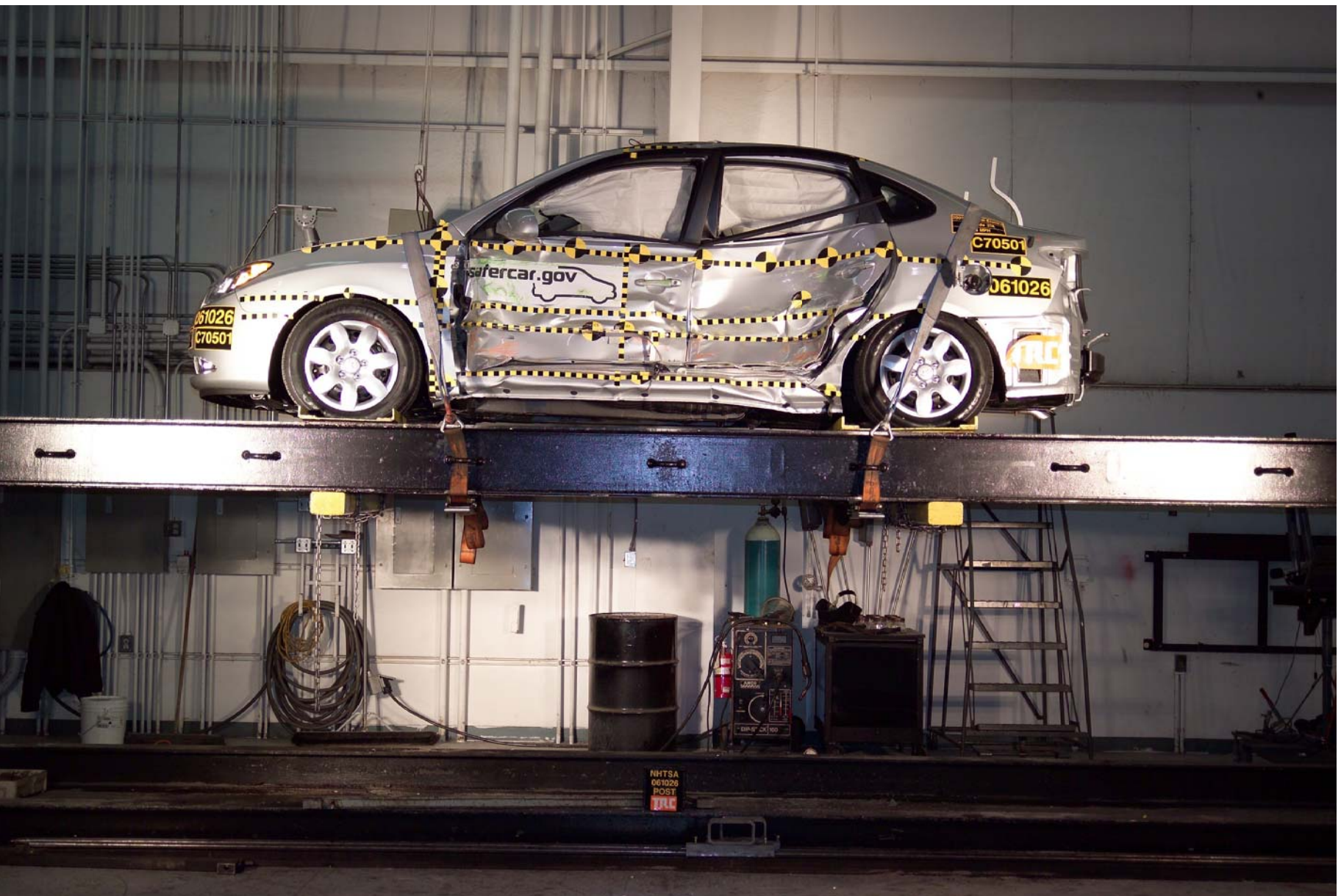
Figure A-79 FMVSS 301 Rollover View at 360°
