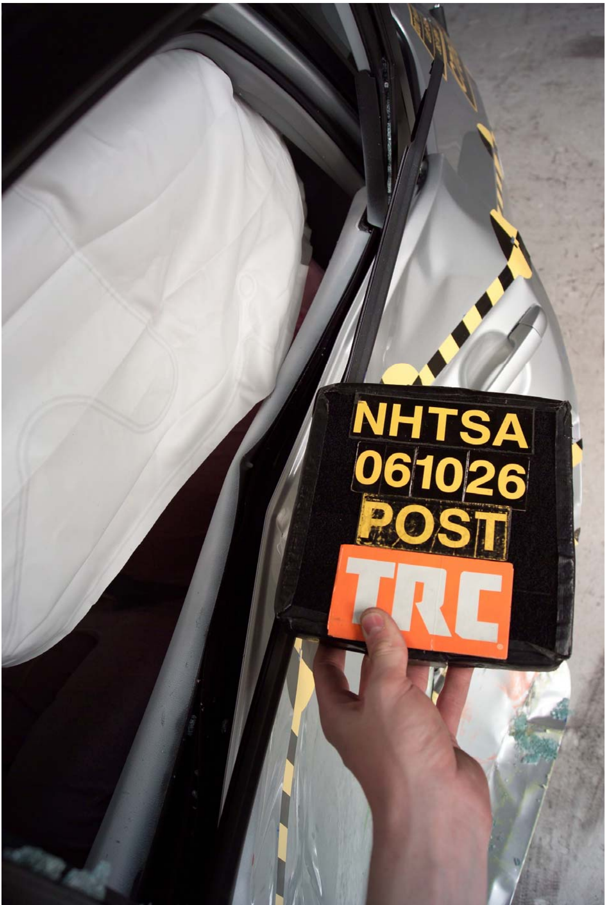
Figure A-50 Post-Test Left View of Rear SID HIII and Door Clearance
