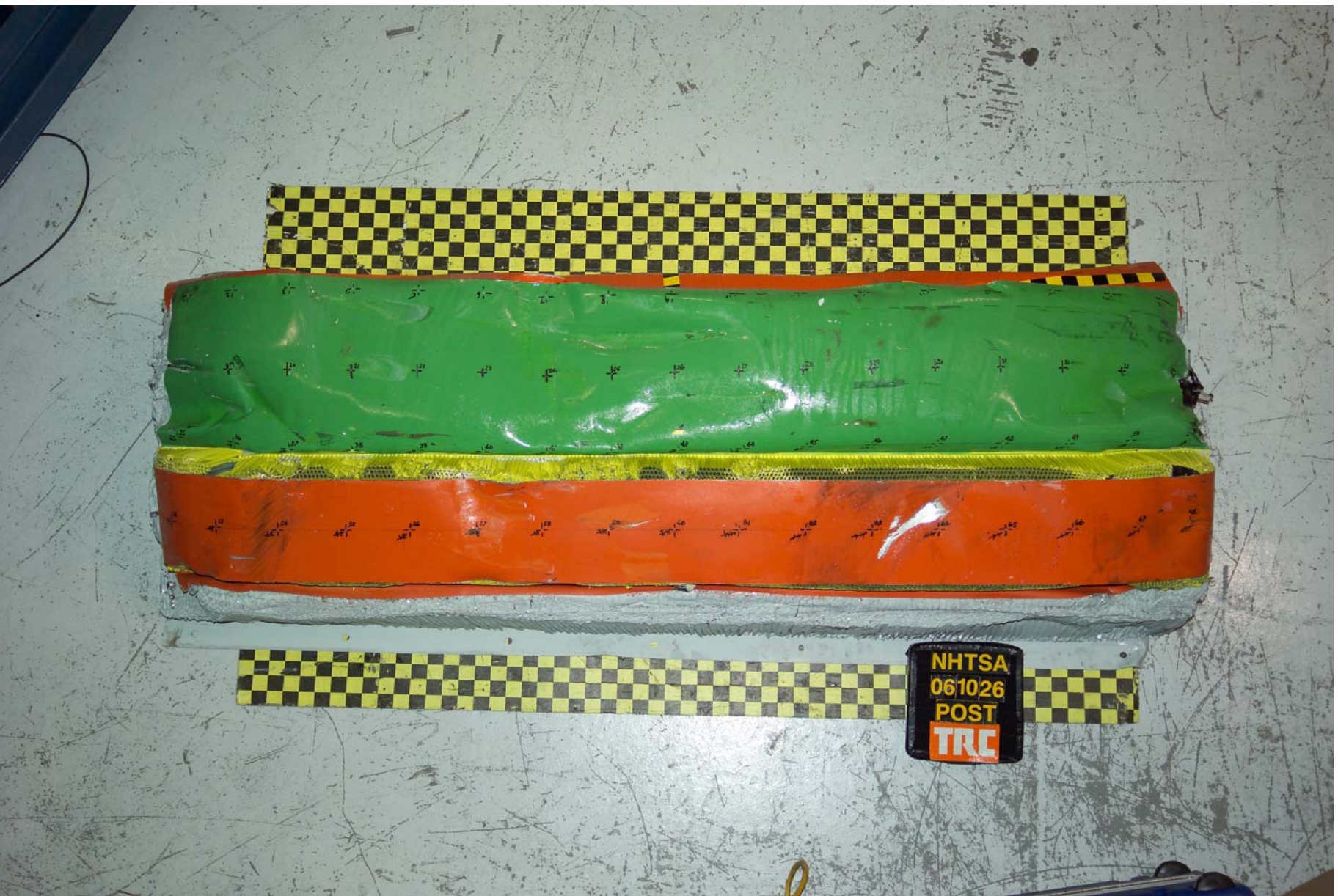
Figure A-17 Post-Test Frontal View of Impactor Face
