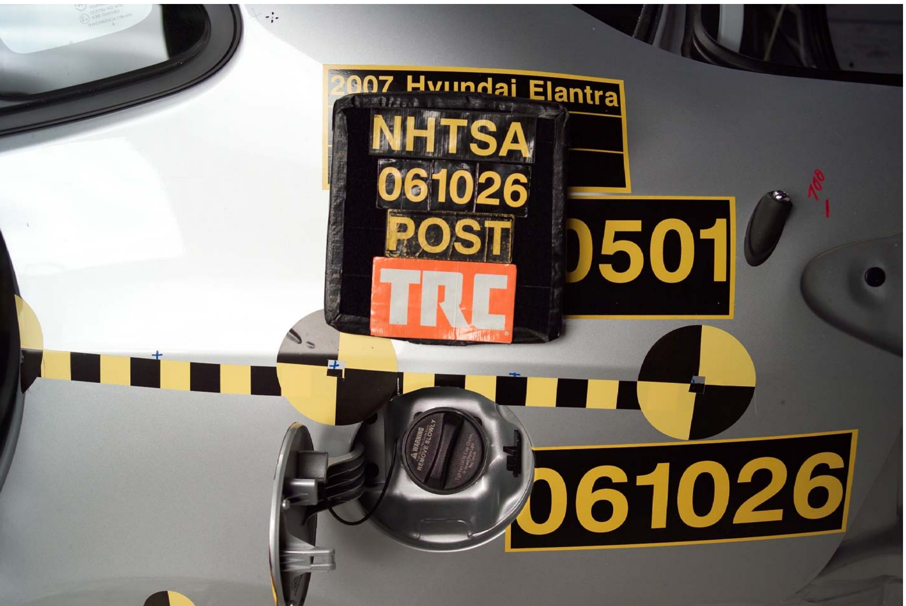
Figure A-75 Post-Test Fuel Cap
