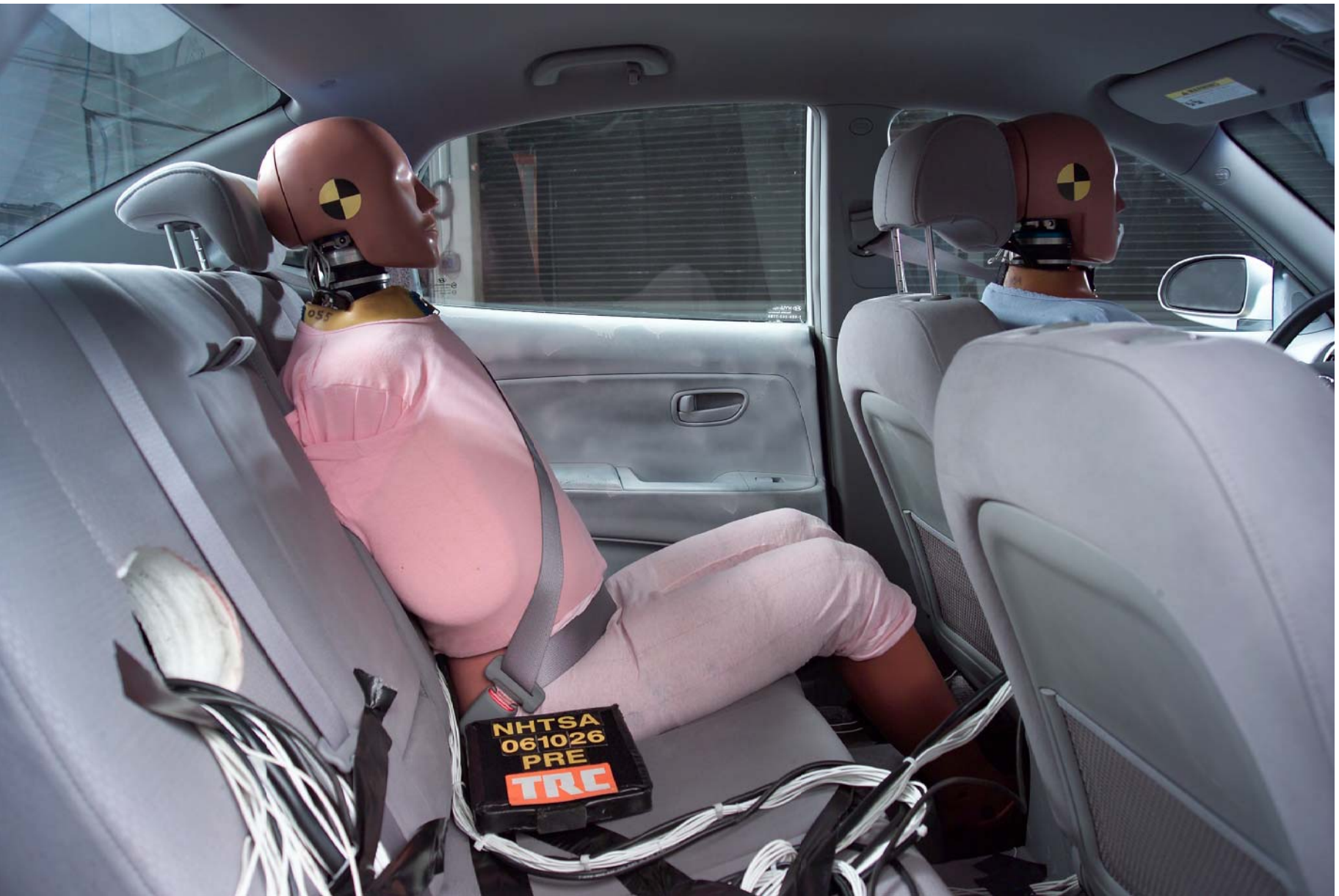
Figure A-39 Pre-Test Right Occupant Compartment View of Rear SID HIIII
