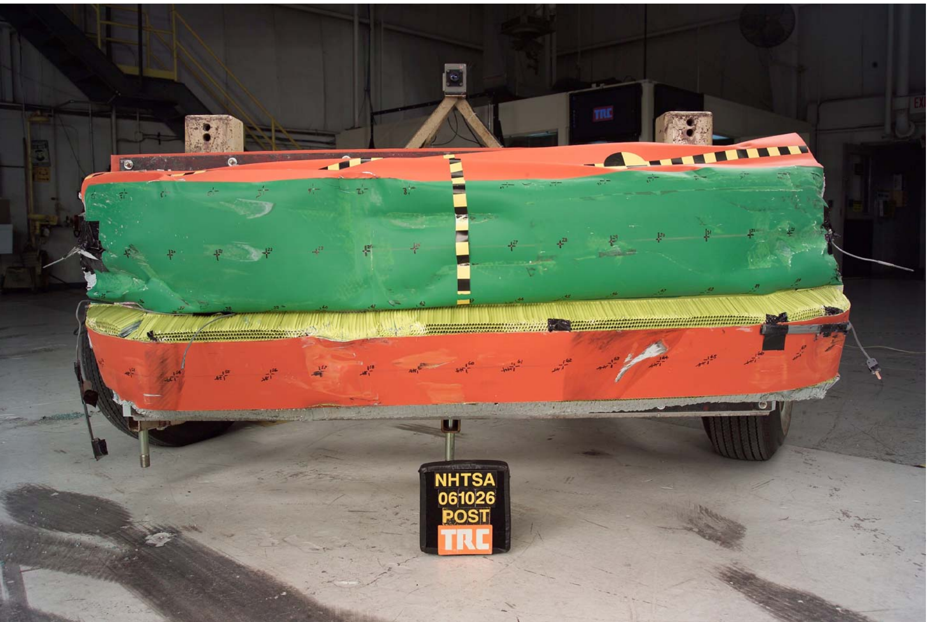
Figure A-34 Post-Test View of MDB Showing Contact Switches in Place
