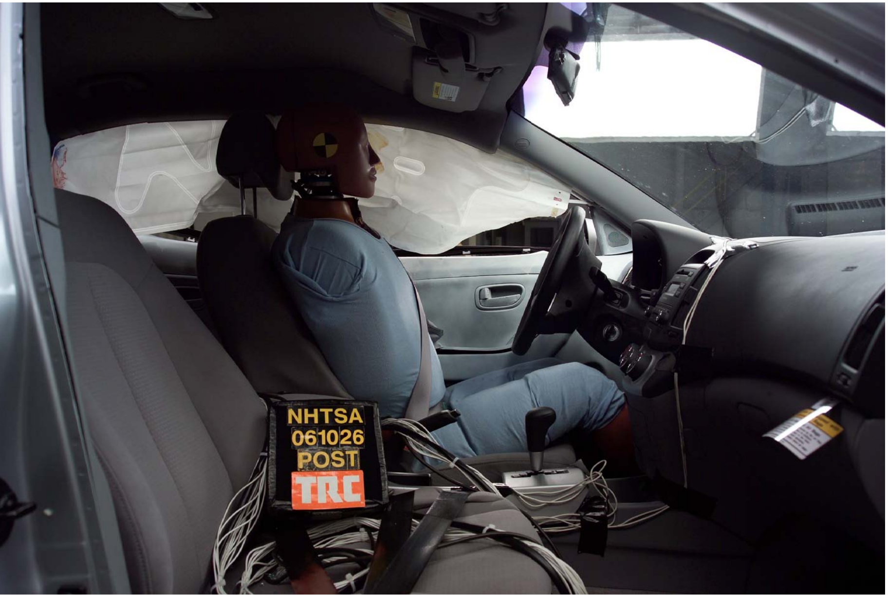
Figure A-38 Post-Test Right Occupant Compartment View of Front SID HII
