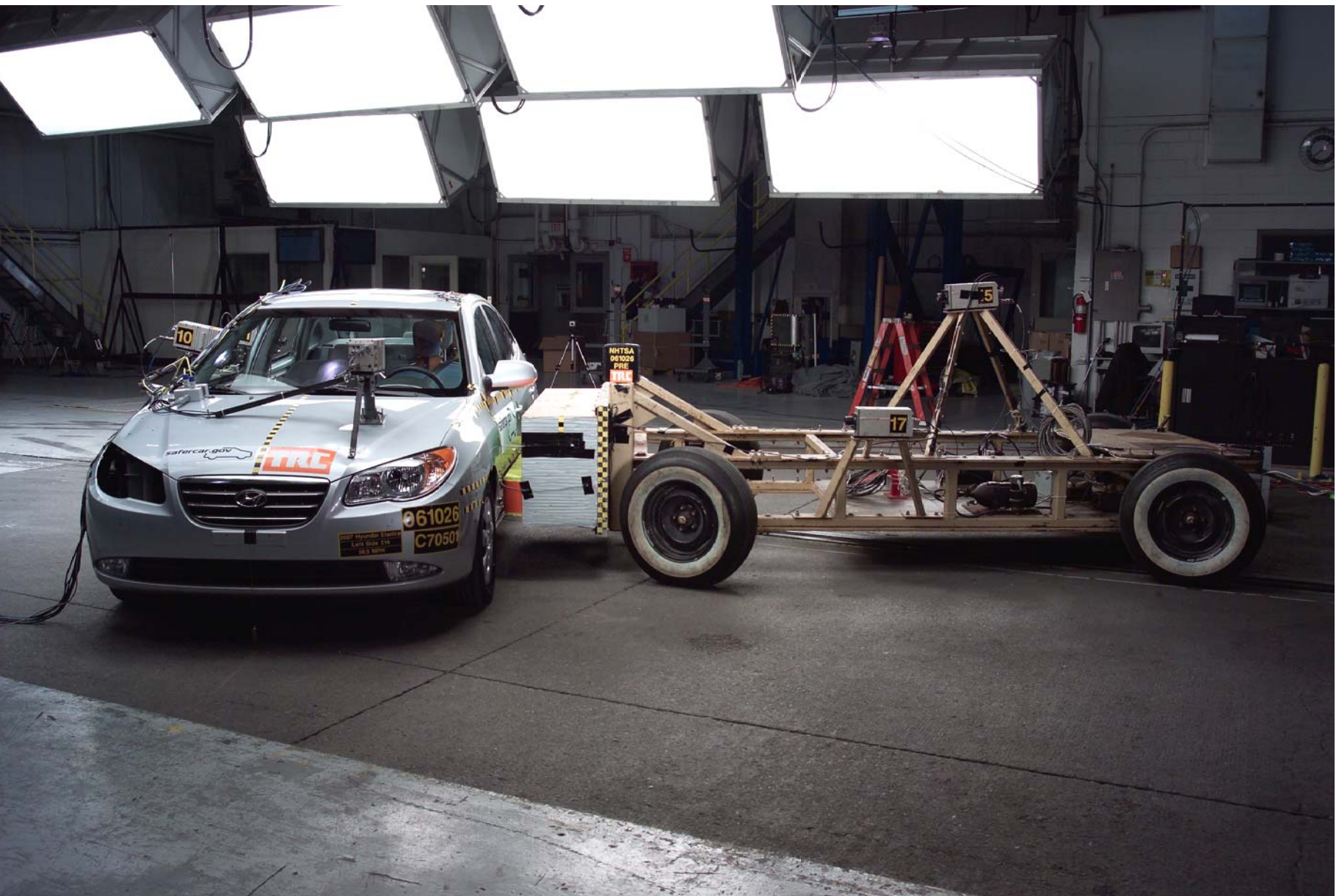
Figure A-59 Pre-Test Left Side View of MDB With Impactor Face in Position
