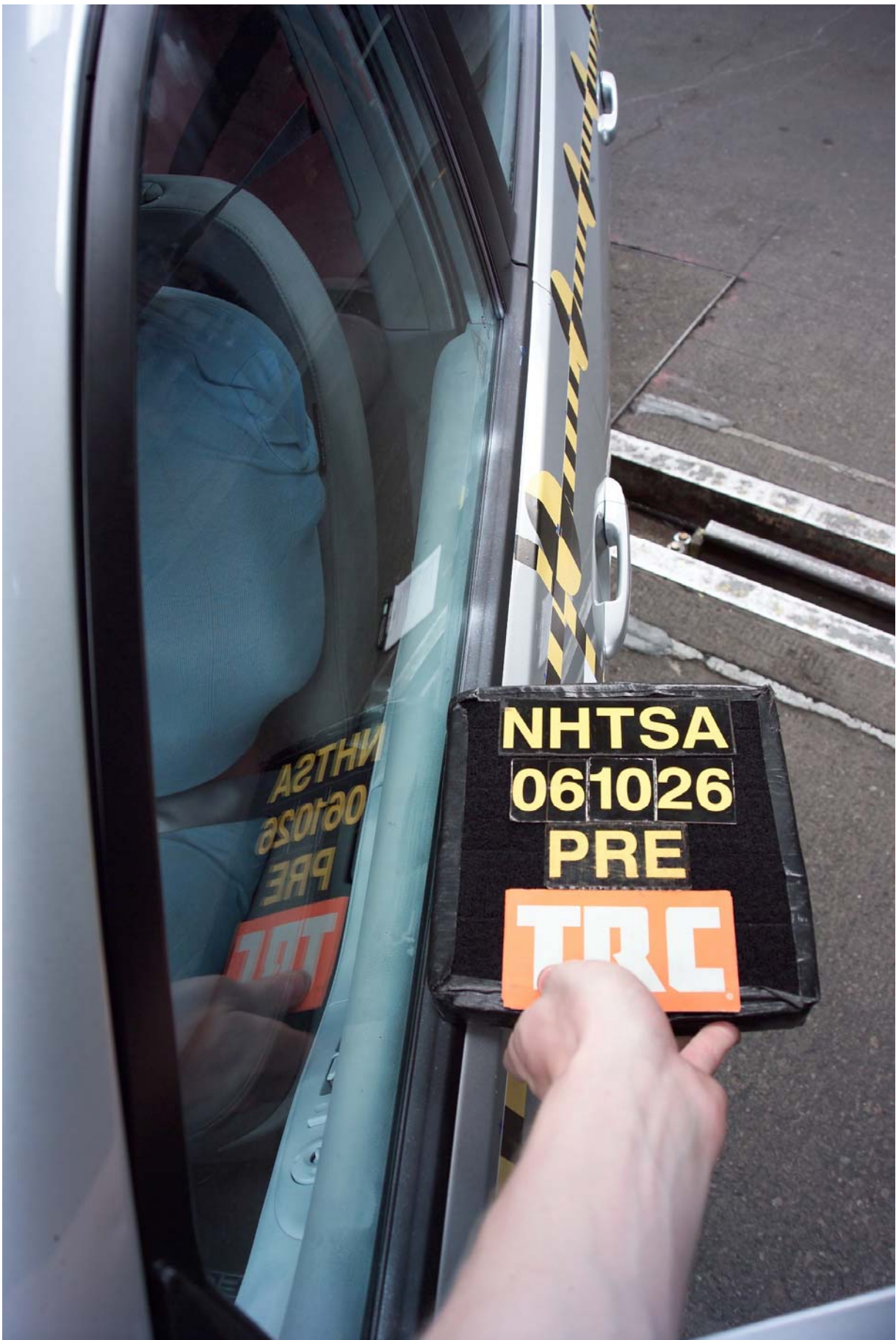
Figure A-44 Pre-Test Left View of Front SID HIII and Door Clearance
