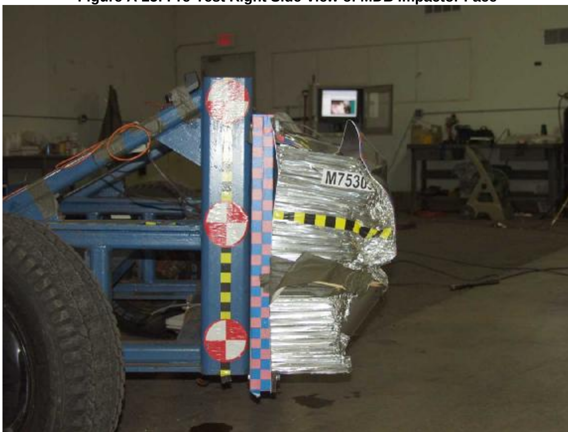
Figure A-26: Post-Test Right Side View of MDB Impactor Face
