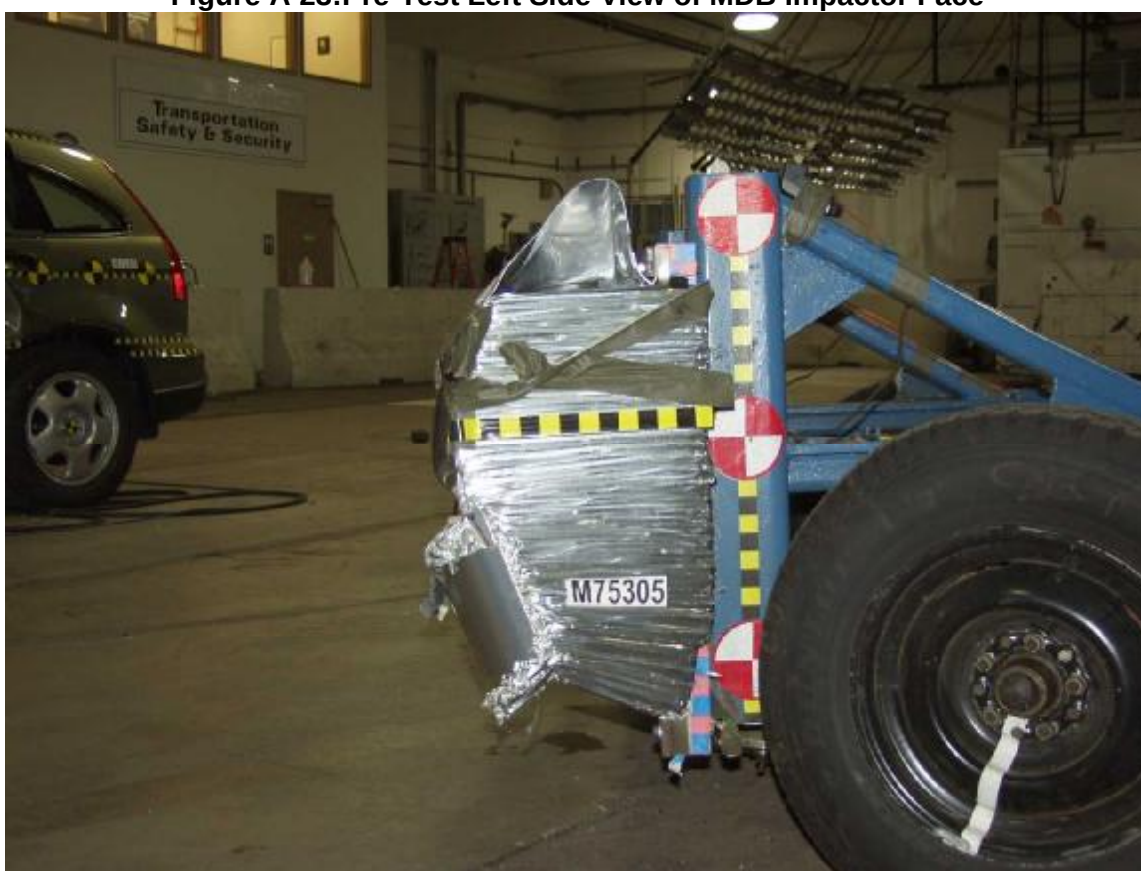
Figure A-24: Post-Test Left Side View of MDB Impactor Face
