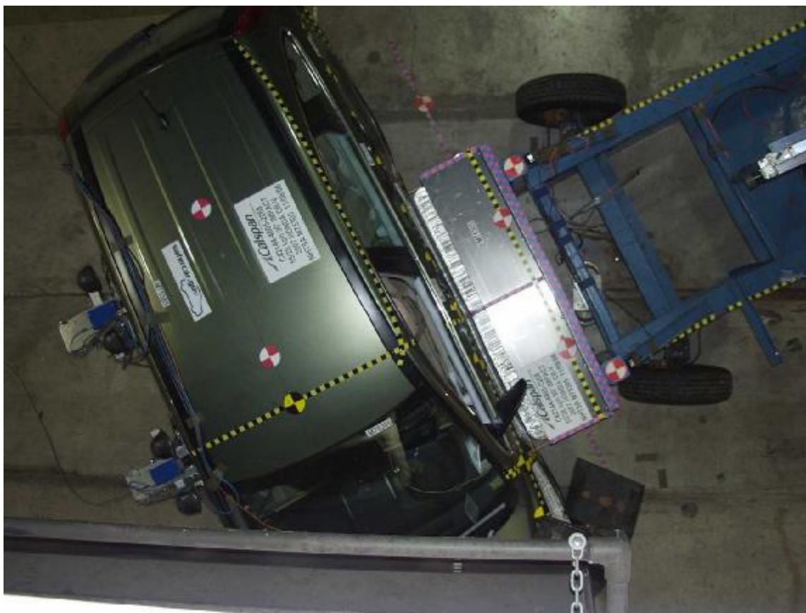
Figure A-31: Pre-Test Overhead View of Aligned MDB and Vehicle
