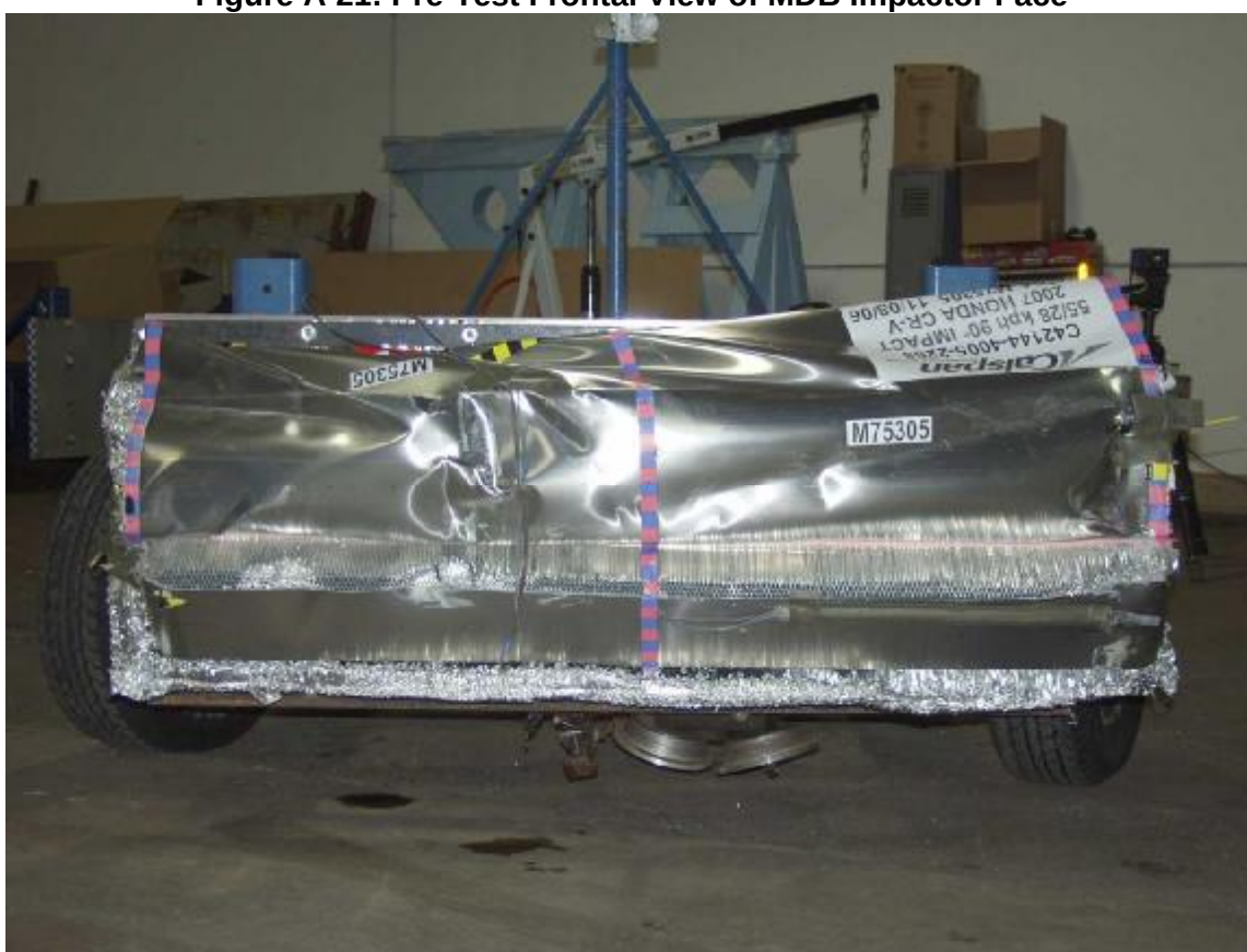
Figure A-22: Post-Test Frontal View of MDB Impactor Face
