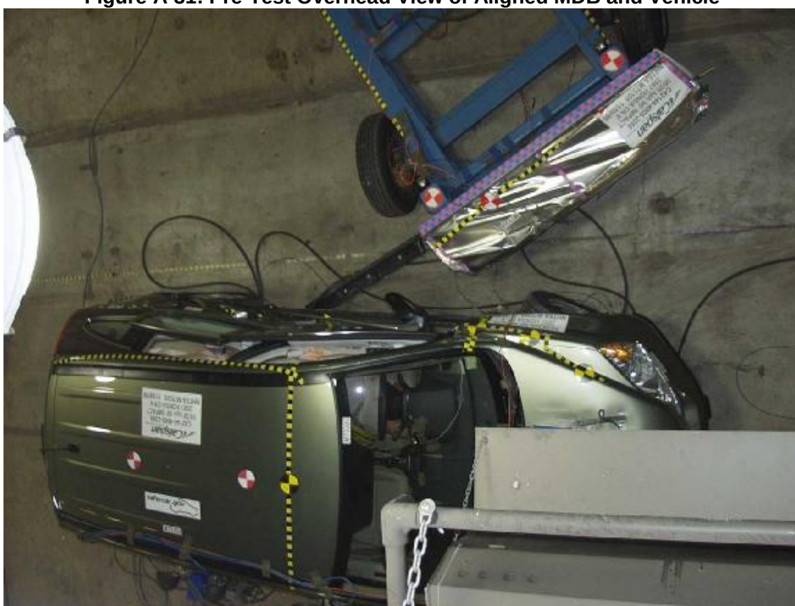
Figure A-32: Post-Test Overhead View of MDB and Vehicle
