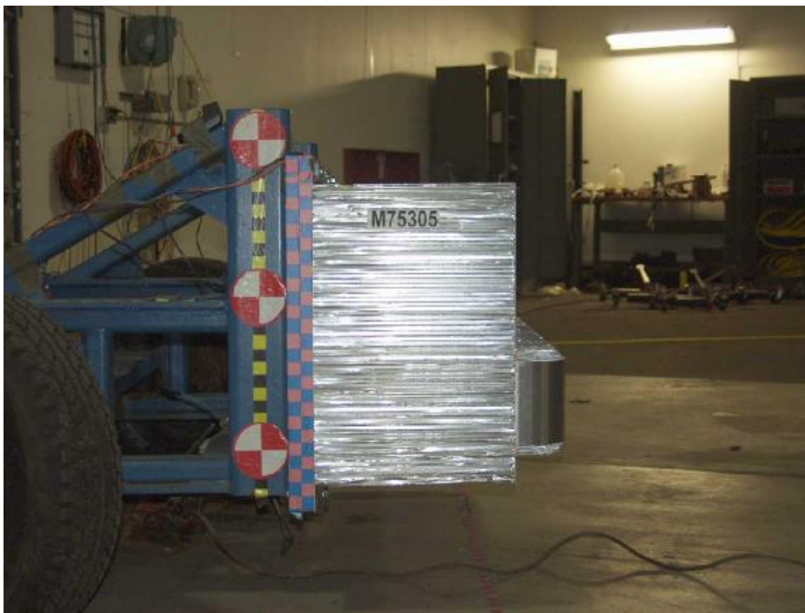
Figure A-25: Pre-Test Right Side View of MDB Impactor Face
