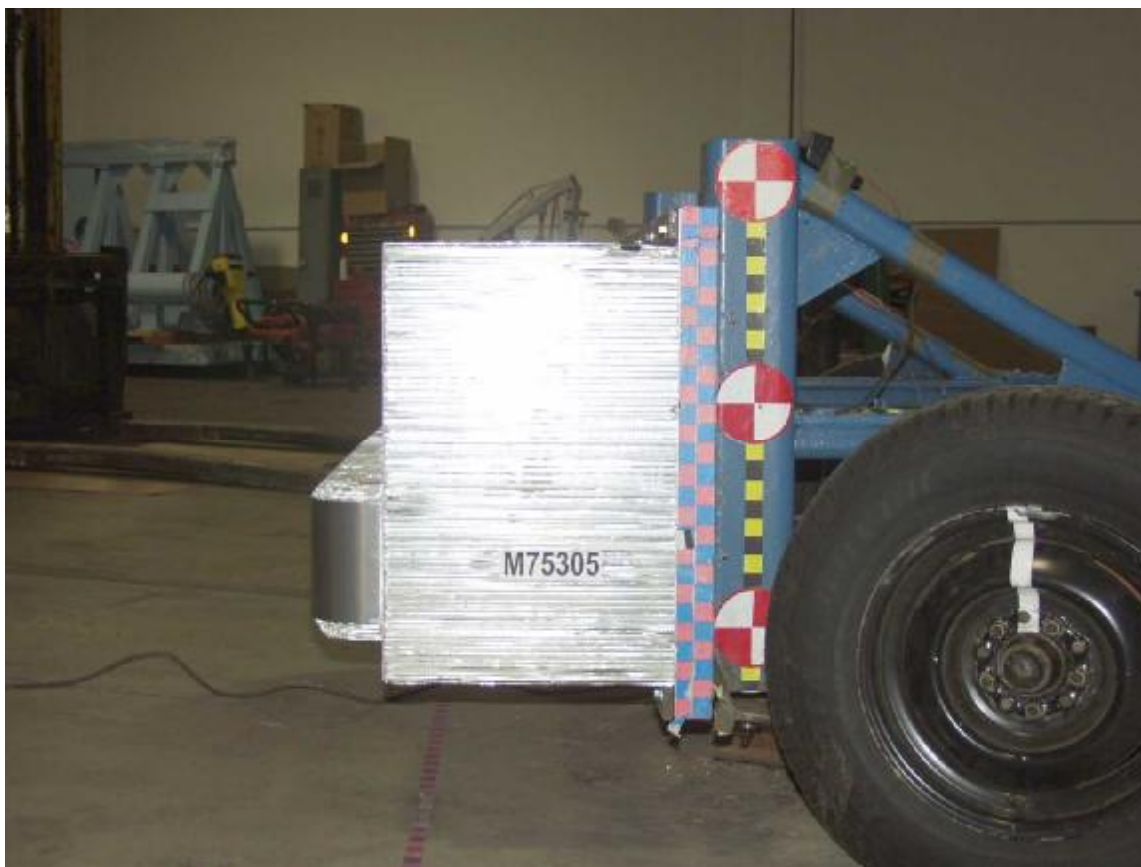
Figure A-23: Pre-Test Left Side View of MDB Impactor Face
