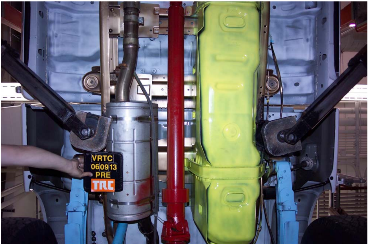
Figure A-33 Pre-Test Fuel Tank View
