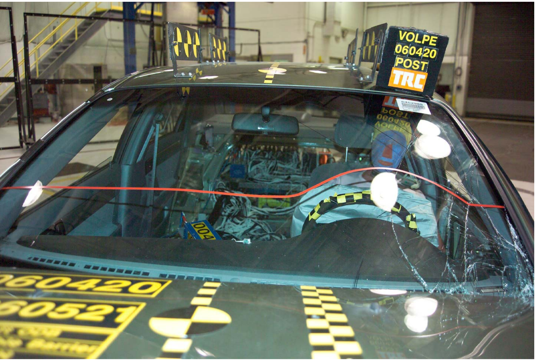
Figure A-42 Post-Test Windshield View
