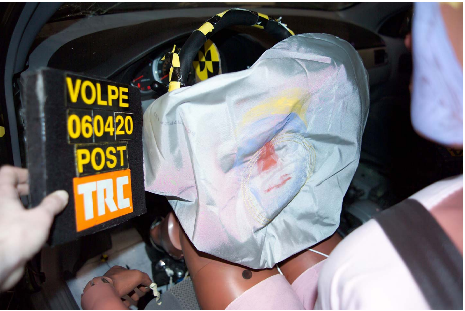
Figure A-48 Post-Test Driver Dummy Head Contact - View 1
