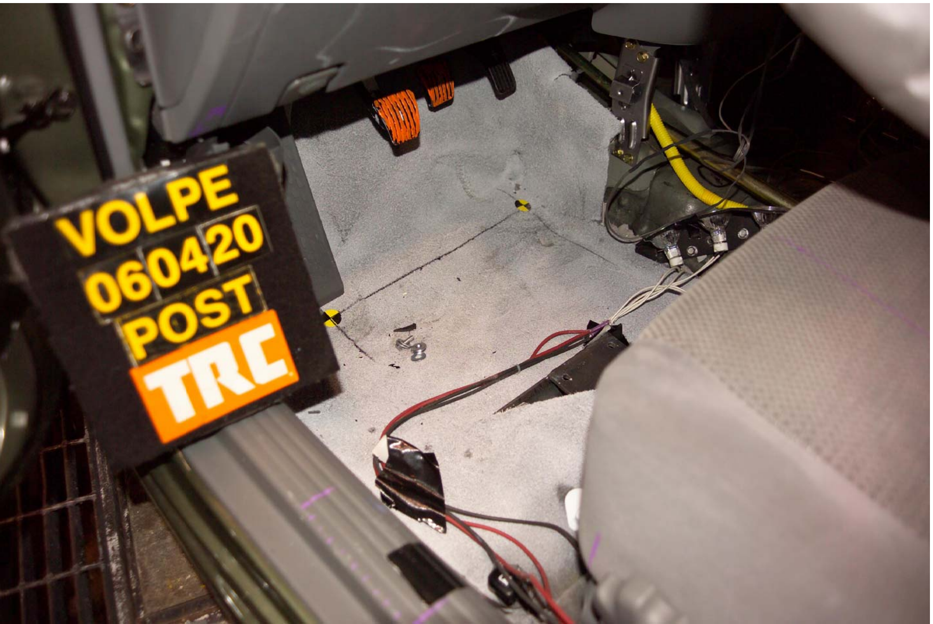
Figure A-54 Post-Test Driver Floorboard Deformation - View 1
