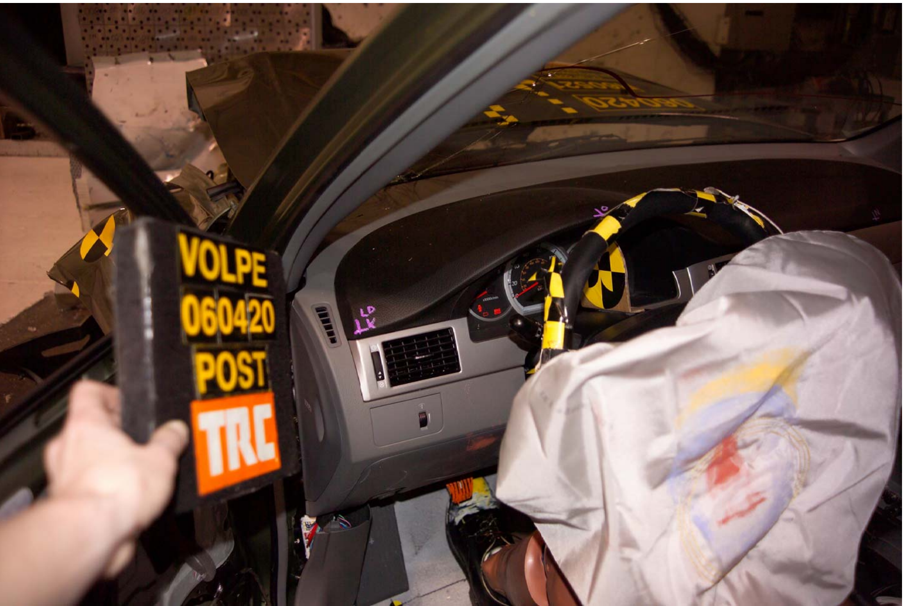
Figure A-58 Post-Test Driver Instrument Panel Damage View
