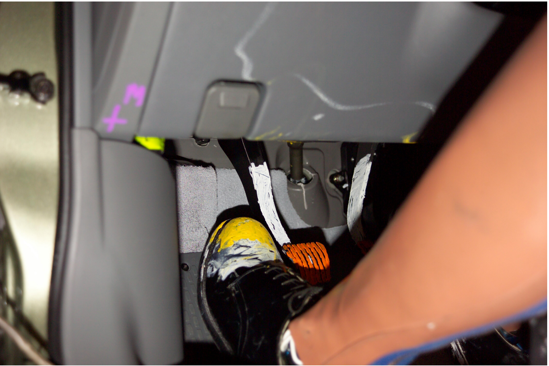
Figure A-56 Pre-Test Driver Toeboard Deformation View
