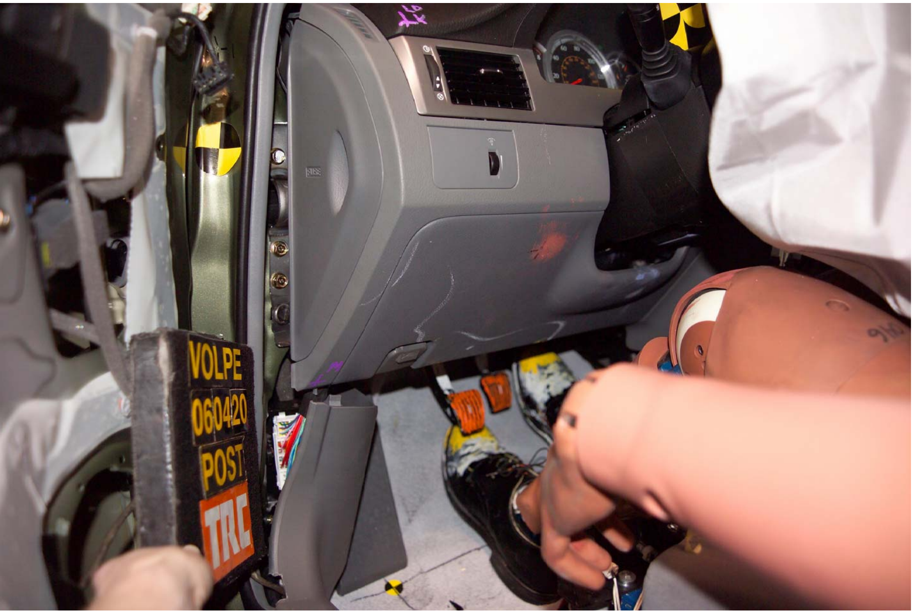
Figure A-51 Post-Test Driver Dummy Knee Contact - View 2
