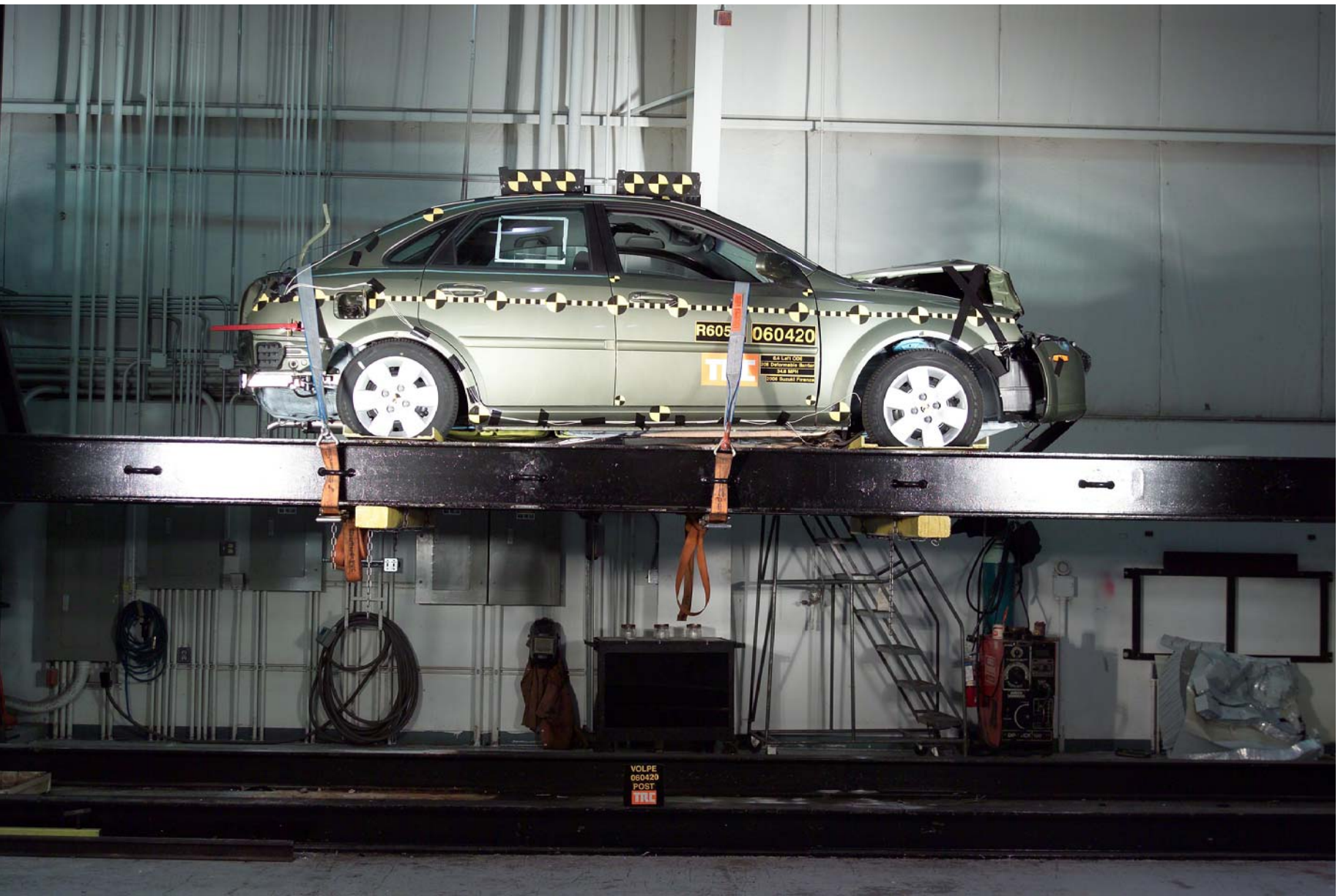
Figure A-70 Vehicle on Rollover Device - 360°
