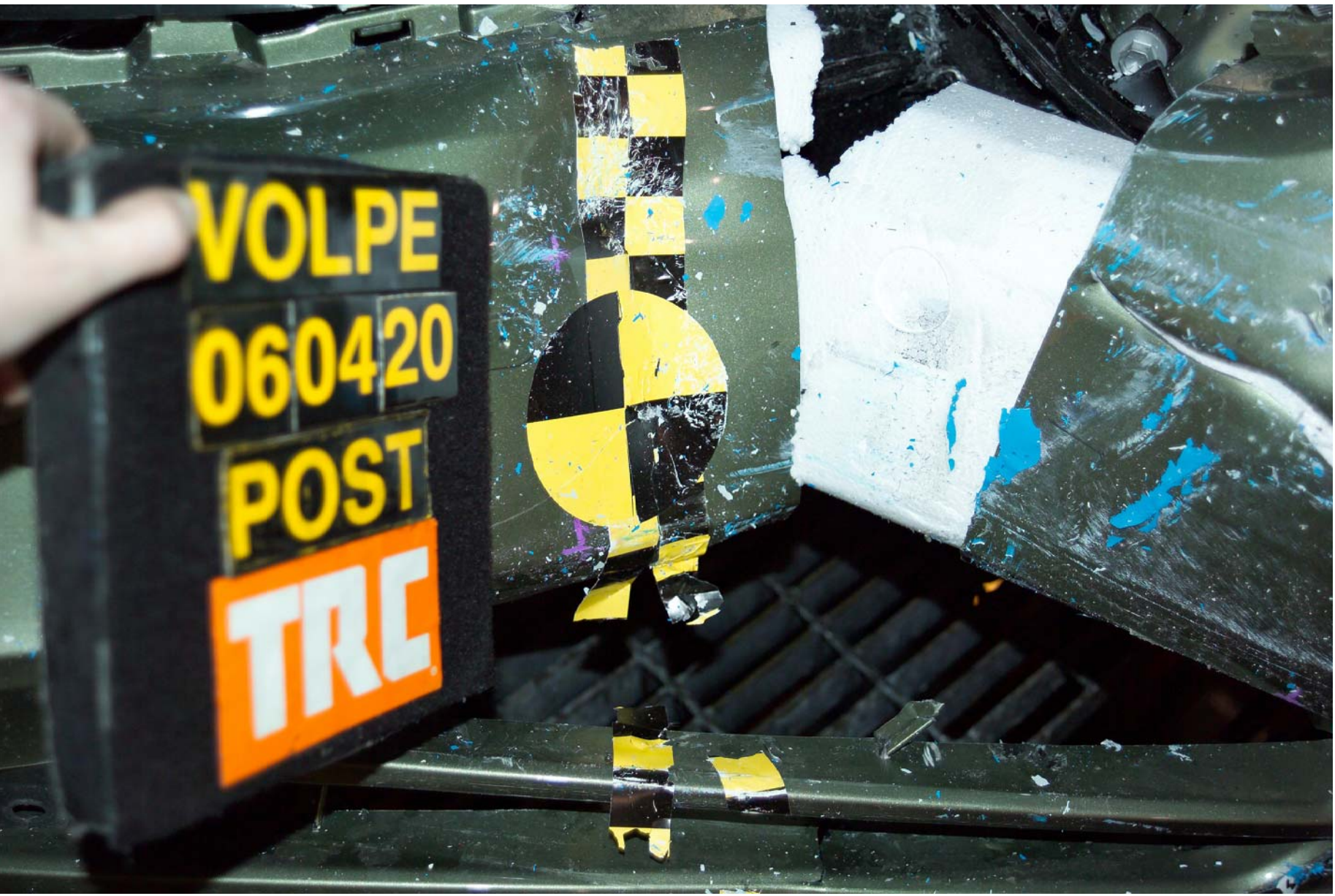
Figure A-20 Post-Test Primary Impact Point View
