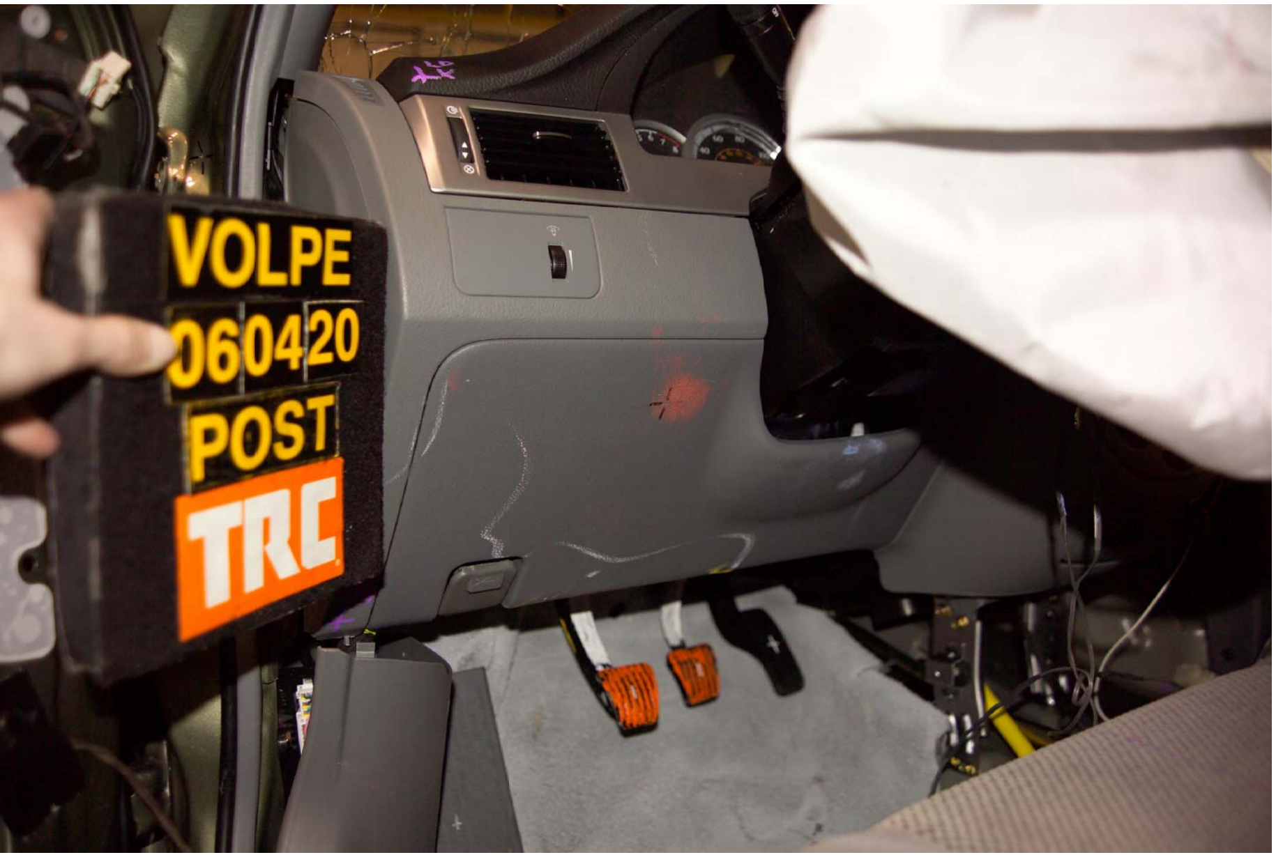
Figure A-52 Post-Test Driver Dummy Knee Bolster View
