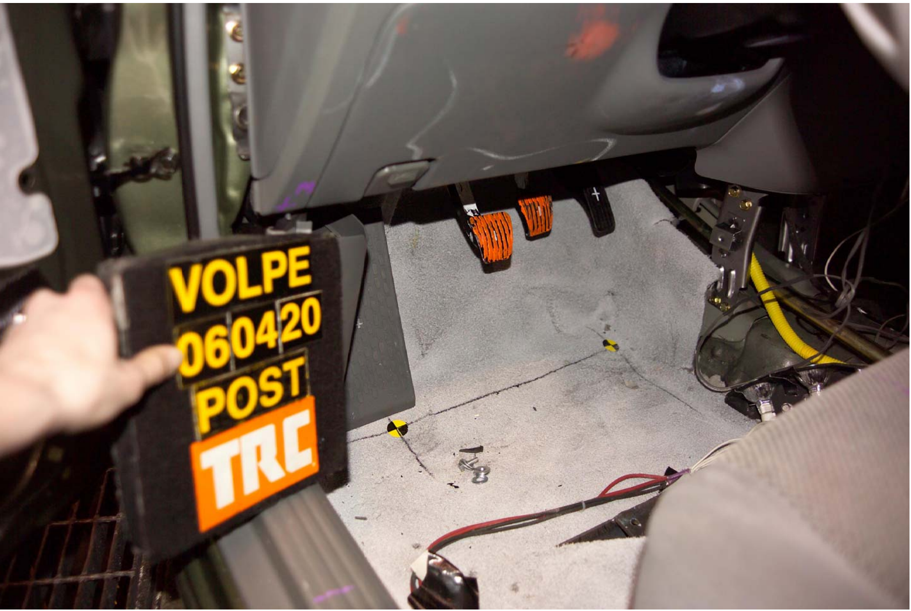
Figure A-55 Post-Test Driver Floorboard Deformation - View 2
