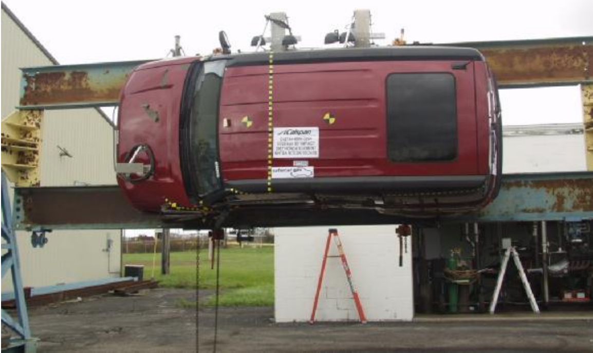
Figure A-51: Rollover 90 Degrees
