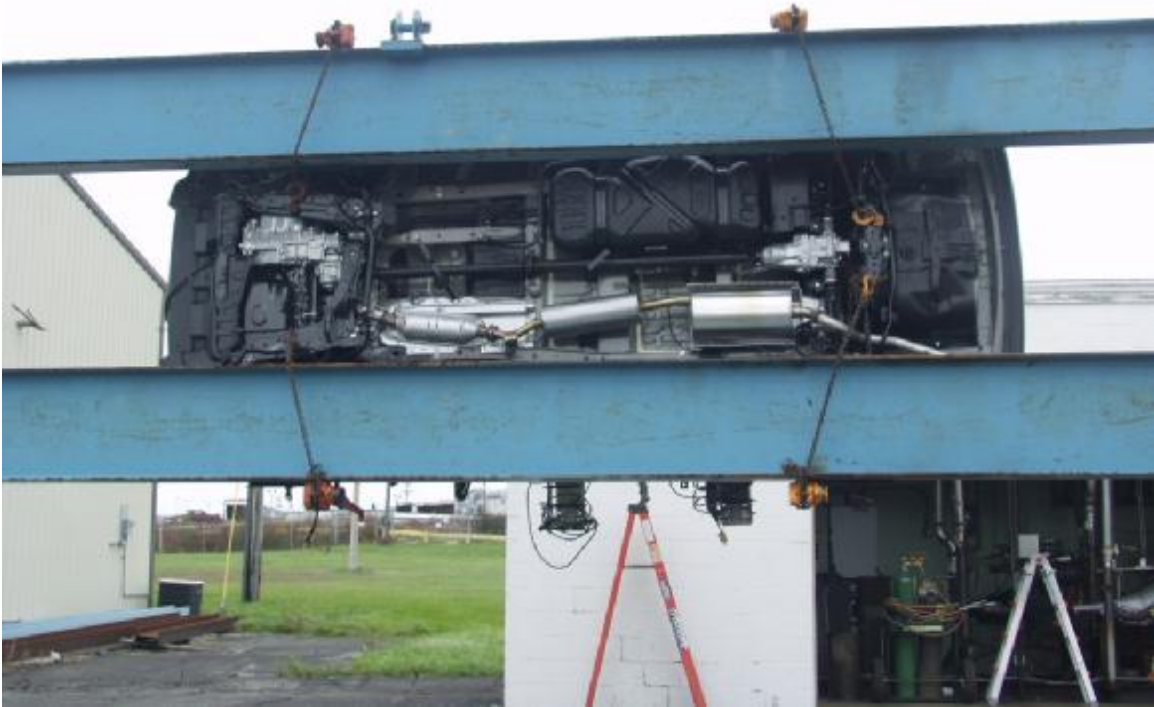
Figure A-53: Rollover 270 Degrees
