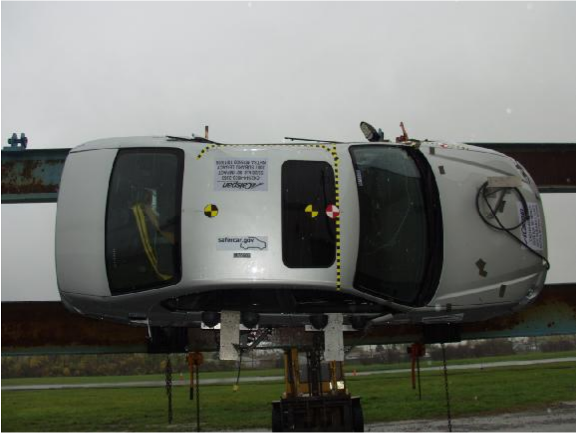
Figure A-51: Rollover 90 Degrees
