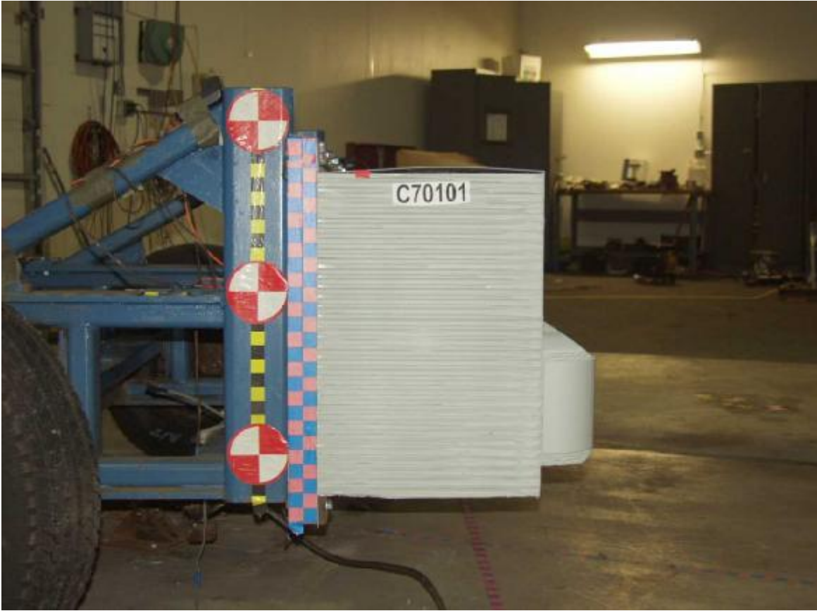
Figure A-25: Pre-Test Right Side View of MDB Impactor Face
